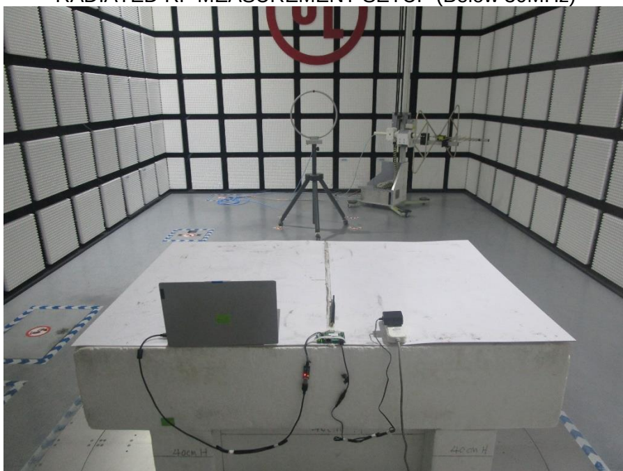
RADIATED RF MEASUREMENT SETUP (Below 30MHz)
