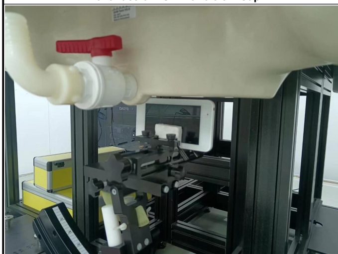
Left Side of EUT with 0.5 cm Gap
