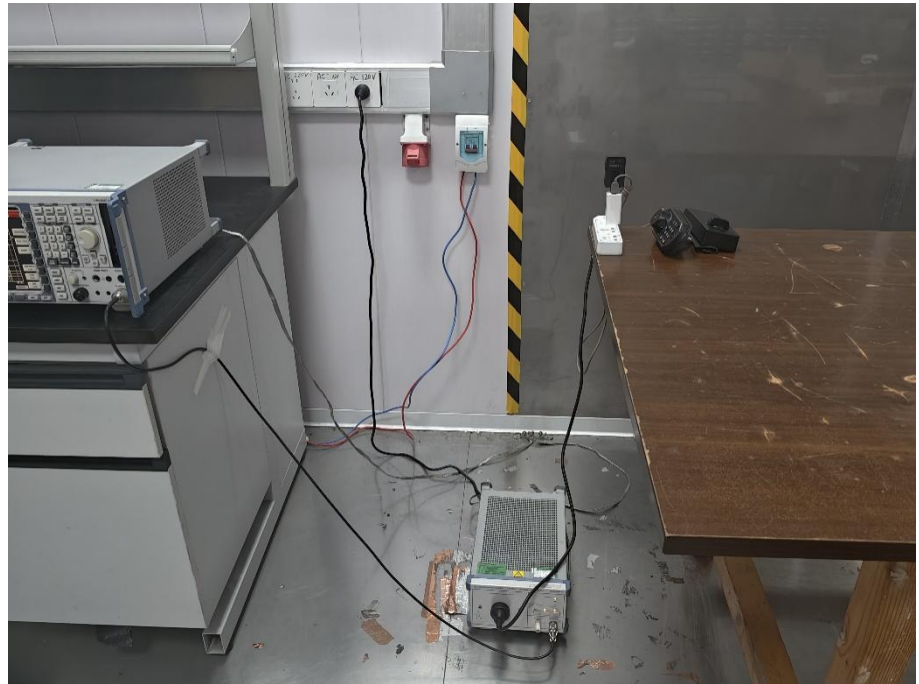
Conducted Emission Test Setup
