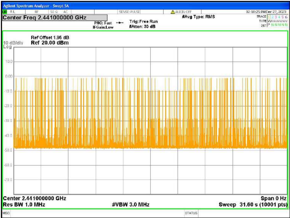
Dwell NVNT 1-DH5 2441MHz Ant1 Accumulated
