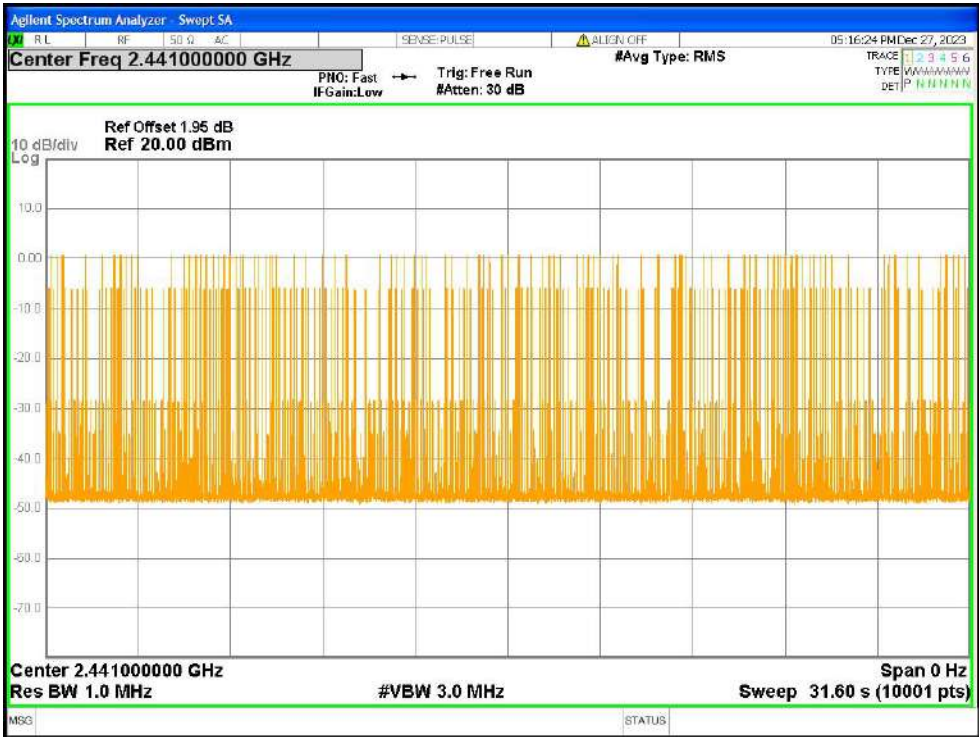
Dwell NVNT 2-DH5 2441MHz Ant1 Accumulated
