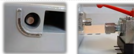
Align device onto plate to fit with the mounting holes with rivet nuts. Use the attached screws M5x12 to attach the device to plate.
