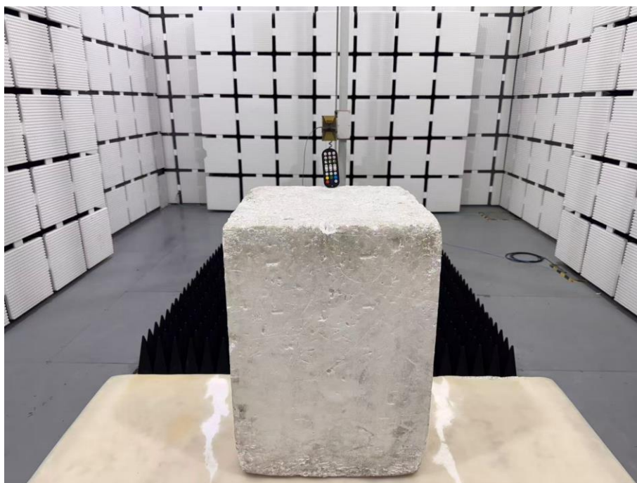
Set-up for Radiated Spurious Emission, Above 1GHz
