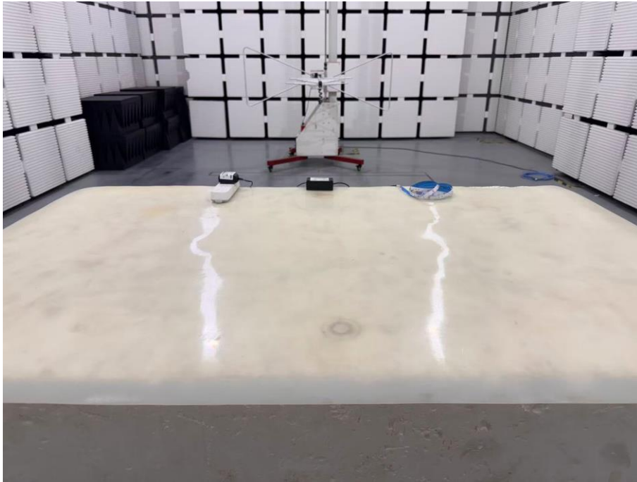
Set-up for Radiated Spurious Emission, Above 1GHz
