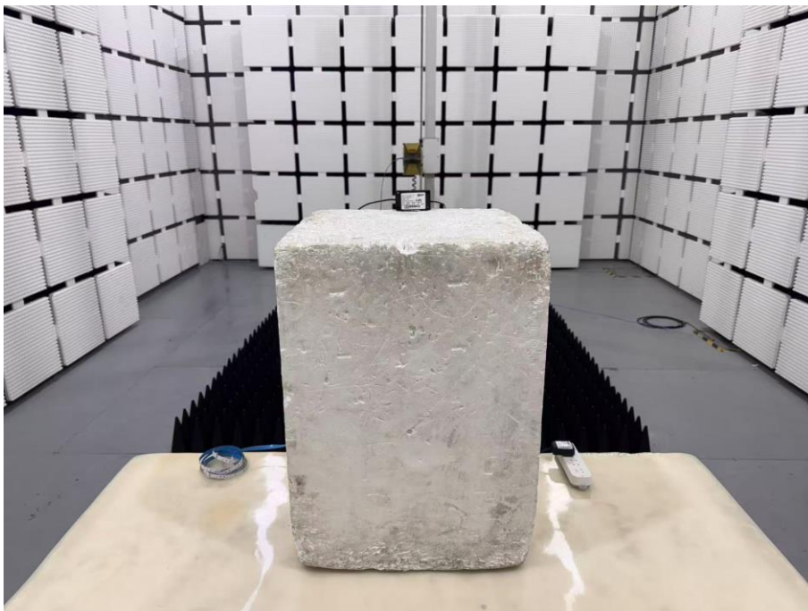
Set-up for Radiated Spurious Emission, Above 1GHz
