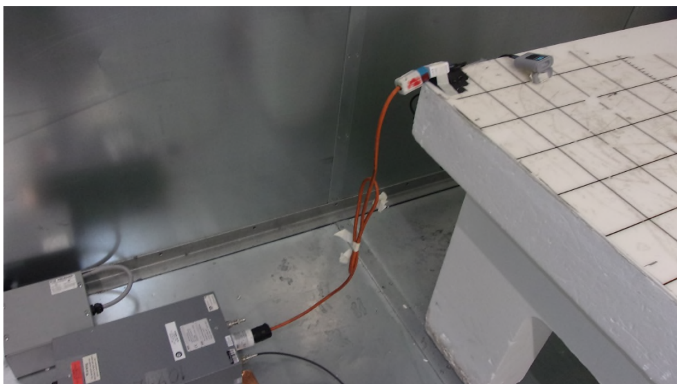
Photo 1.3-1 – Conducted AC Emissions
