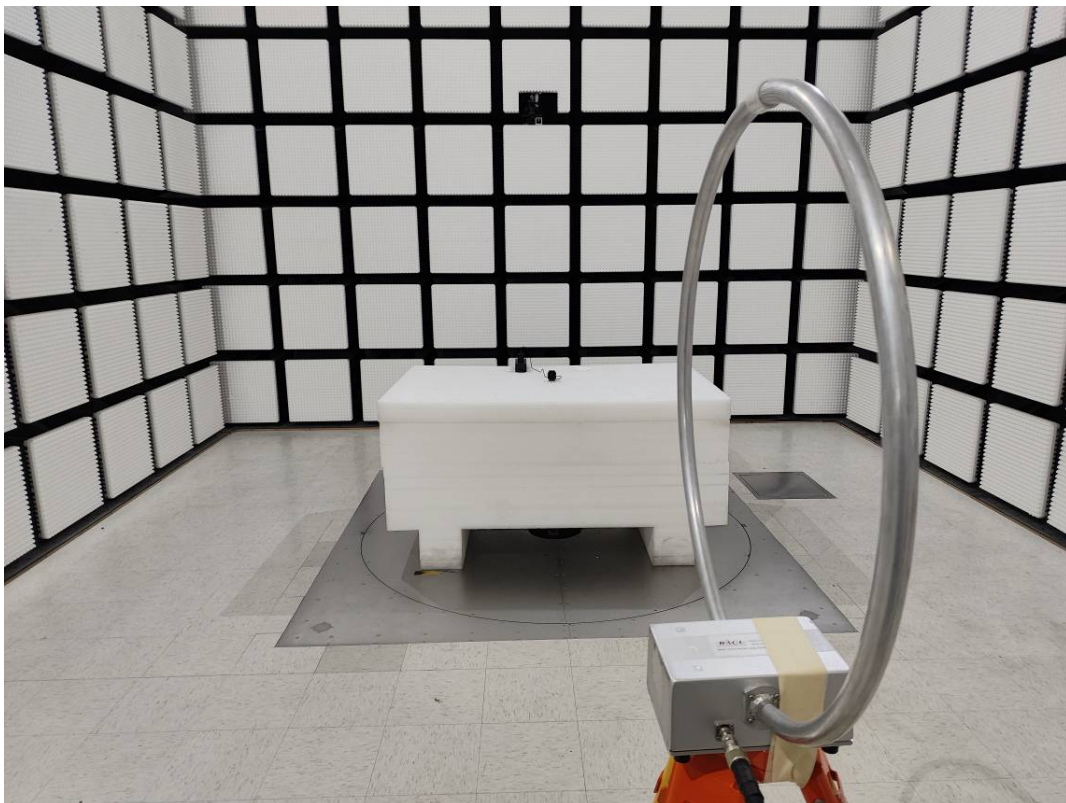
Radiated Emission Below 30MHz View Perpendicular
