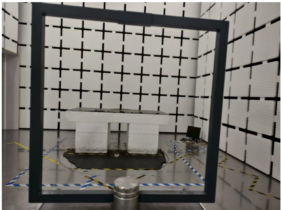
Radiation Emission Test Setup (Below 30MHz)
