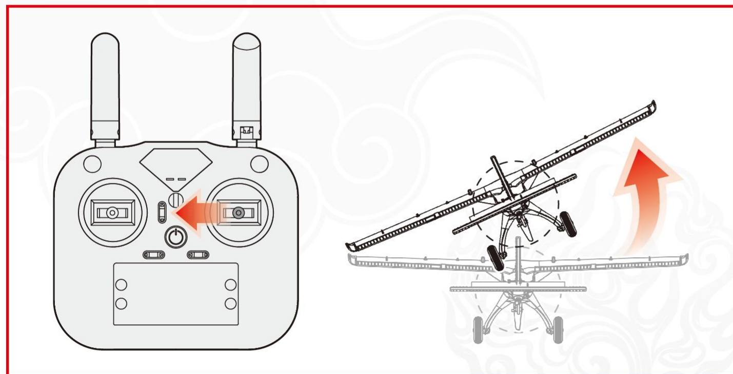
(9). 左倾斜：将遥控器右操纵杆向左移动时，飞机随之向左倾斜。 Left tilt: When the right joystick of the remote control is moved to the left, the aircraft will tilt to the left accordingly.
