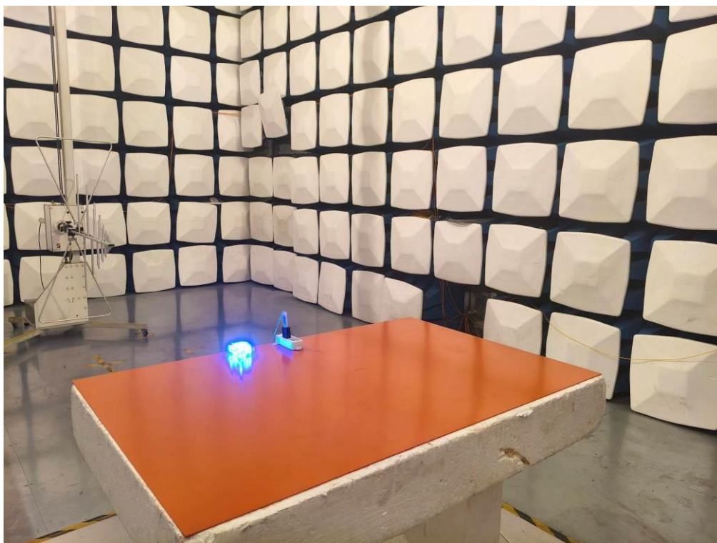
Test Setup Photo(s) of Radiated Emissions Measurement
