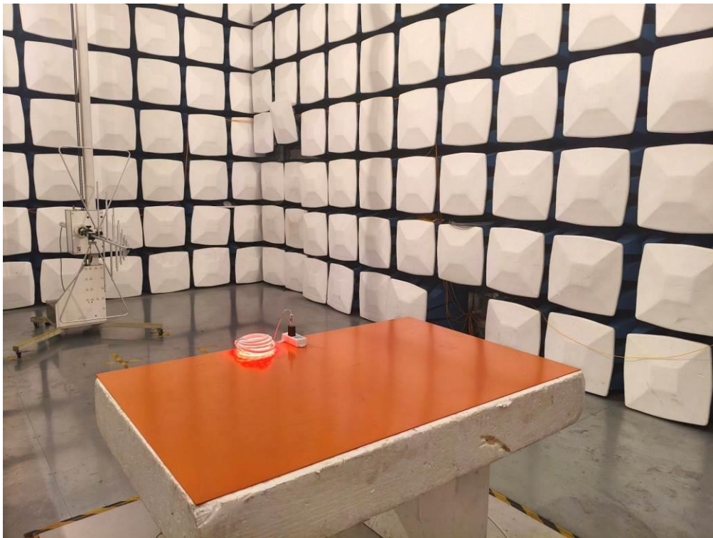
Test Setup Photo(s) of Radiated Emissions Measurement
