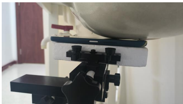
Left Cheek, Test Separation 0 mm
