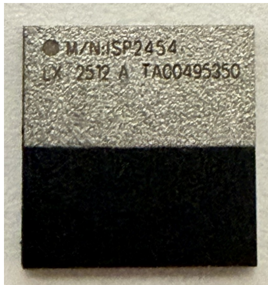
Module top view showing the manufacturer part marking, M/N ISP2454.
