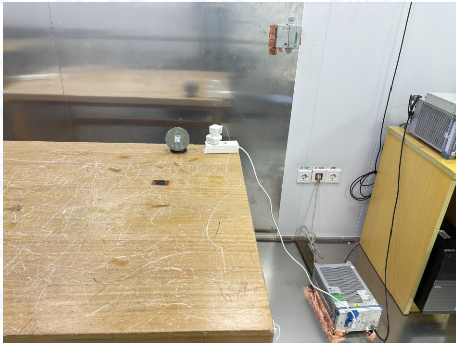
Photo of Setup for Conducted Emission
