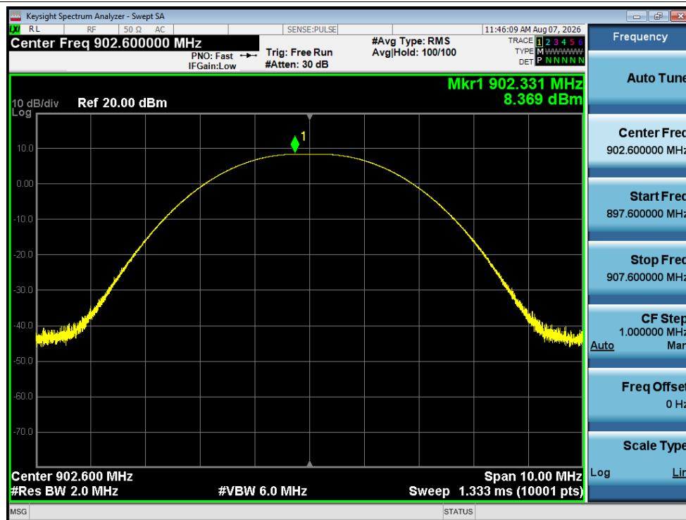
Peak Power NVNT 1M 902.6MHz Ant1
