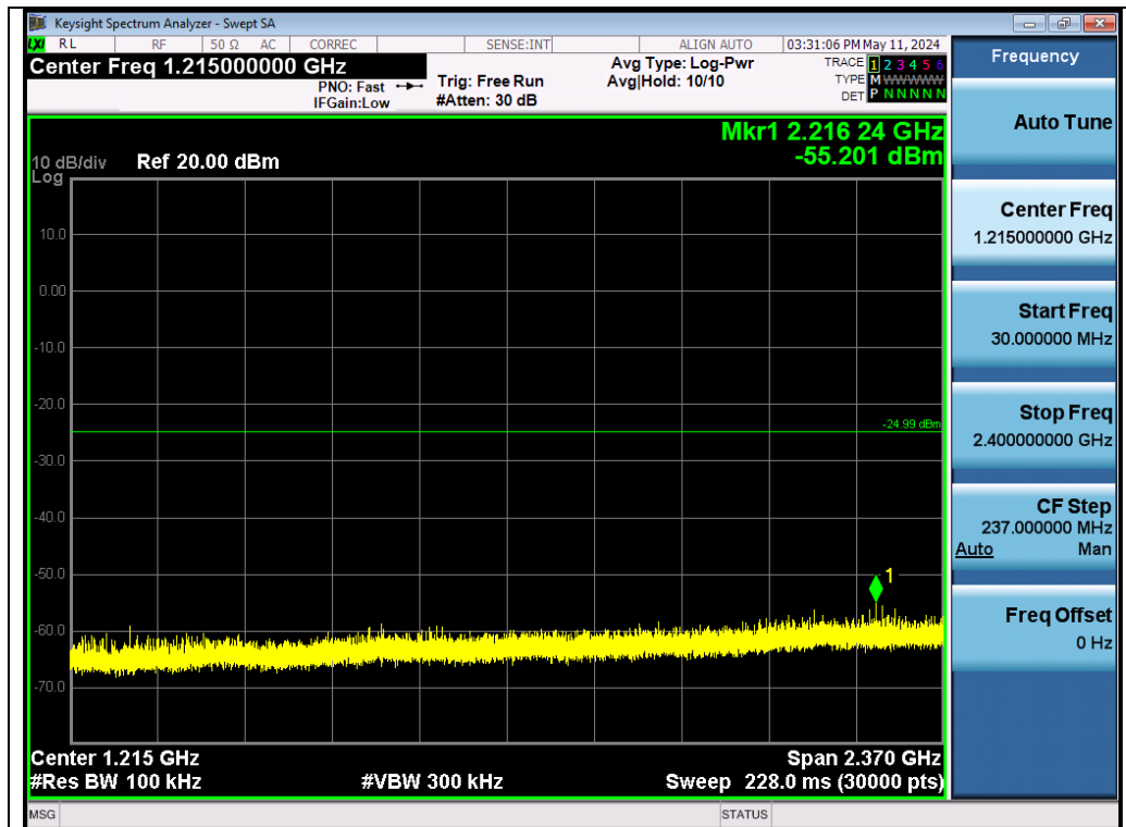
Test_Graph_GFSK_ANT1_2440_Lower Band Emissions
