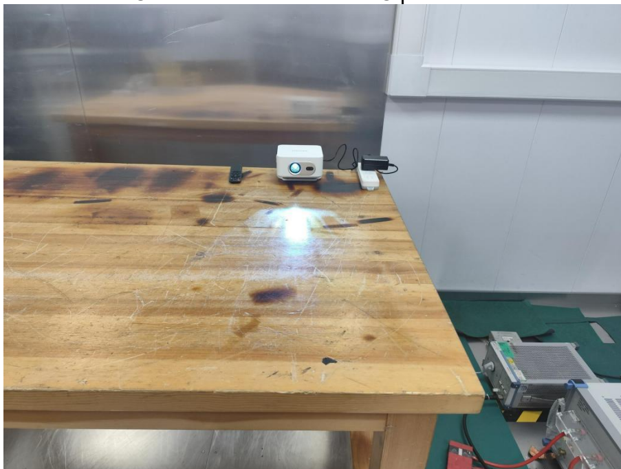
Conducted Emission at AC power line
