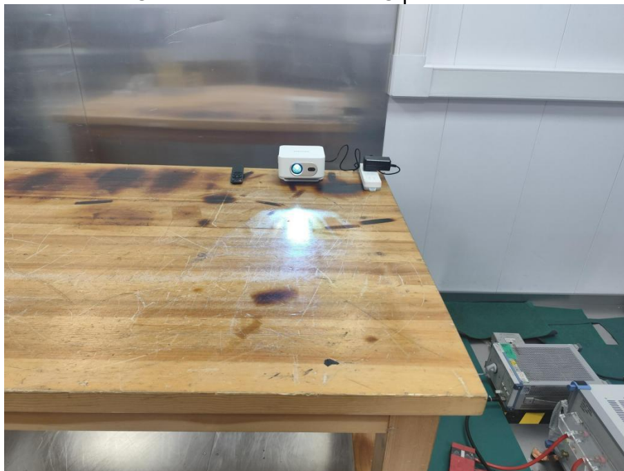
Conducted Emission at AC power line
