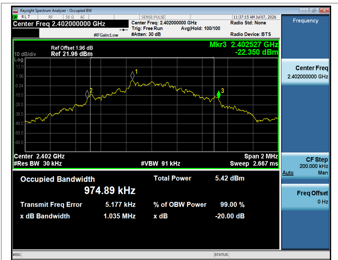
-20dB Bandwidth NVNT 1-DH1 2402MHz Ant1
