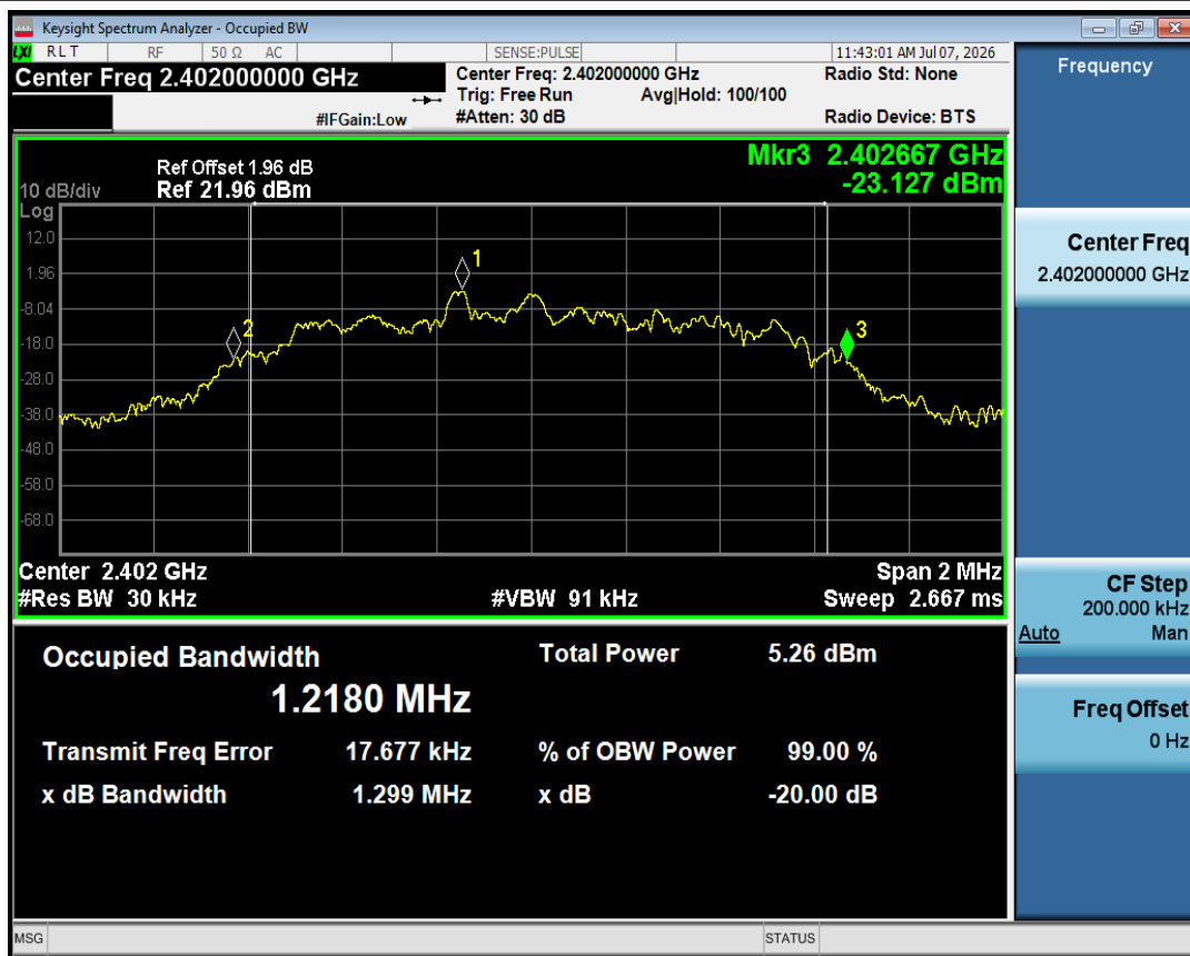
-20dB Bandwidth NVNT 2-DH1 2402MHz Ant1
