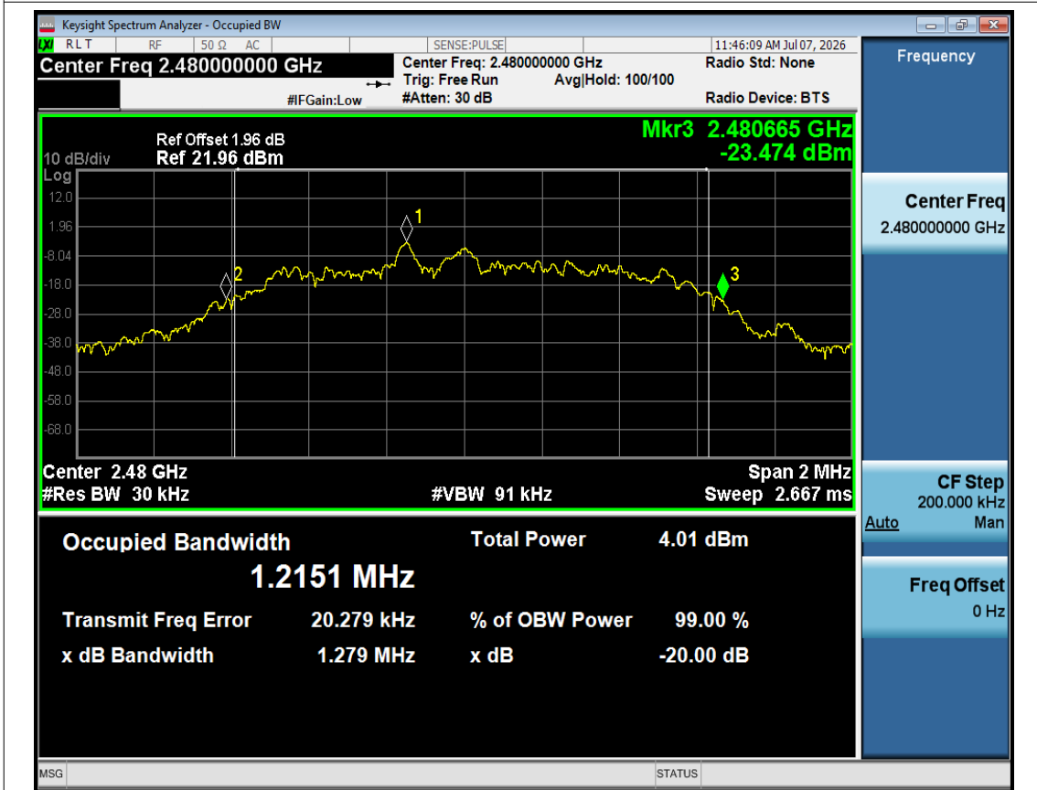
-20dB Bandwidth NVNT 2-DH1 2480MHz Ant1
