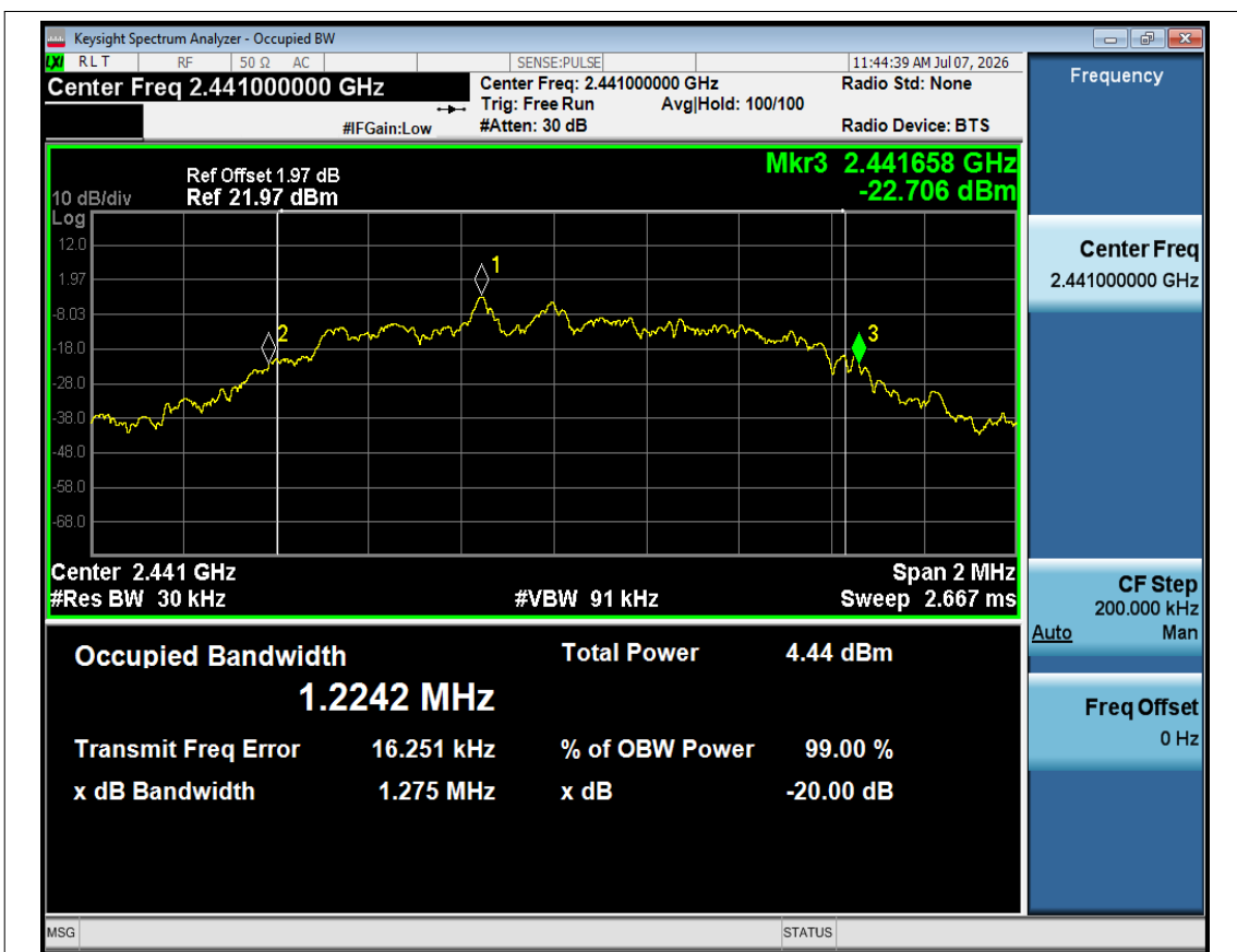
-20dB Bandwidth NVNT 2-DH1 2441MHz Ant1
