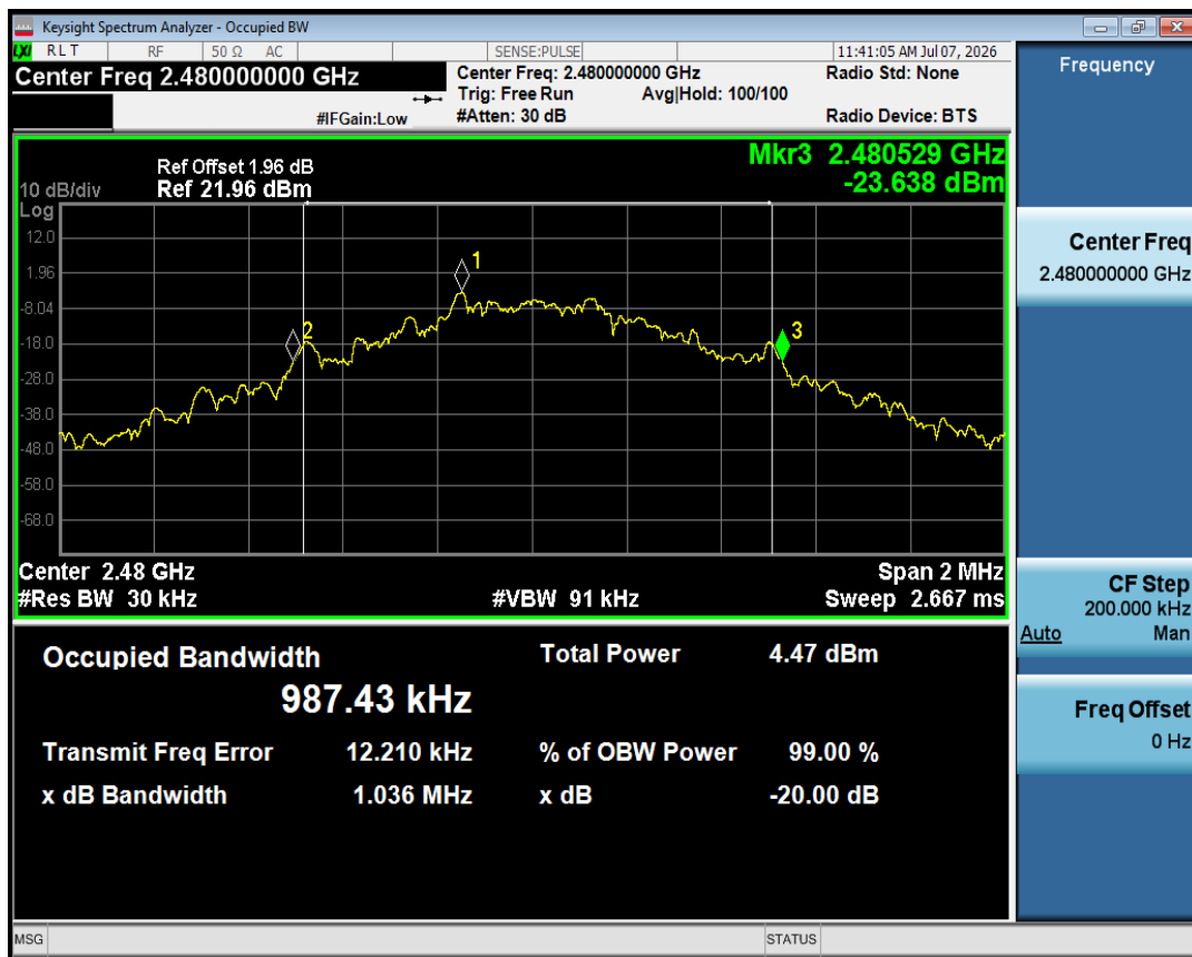
-20dB Bandwidth NVNT 1-DH1 2480MHz Ant1
