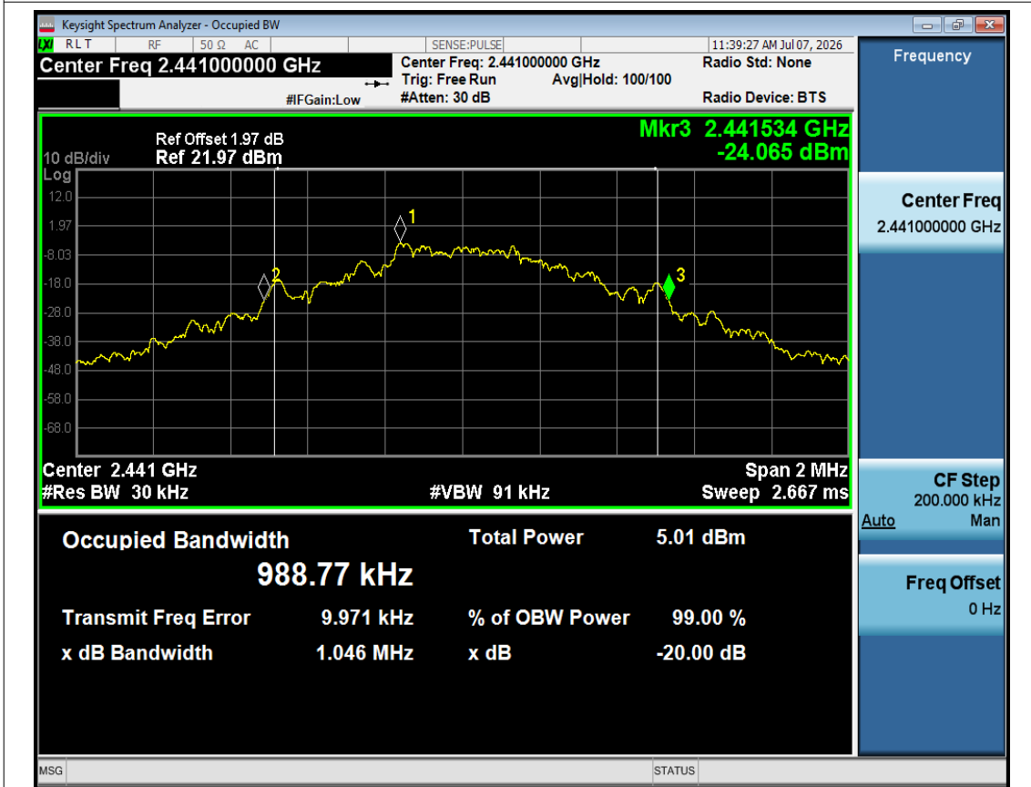
-20dB Bandwidth NVNT 1-DH1 2441MHz Ant1
