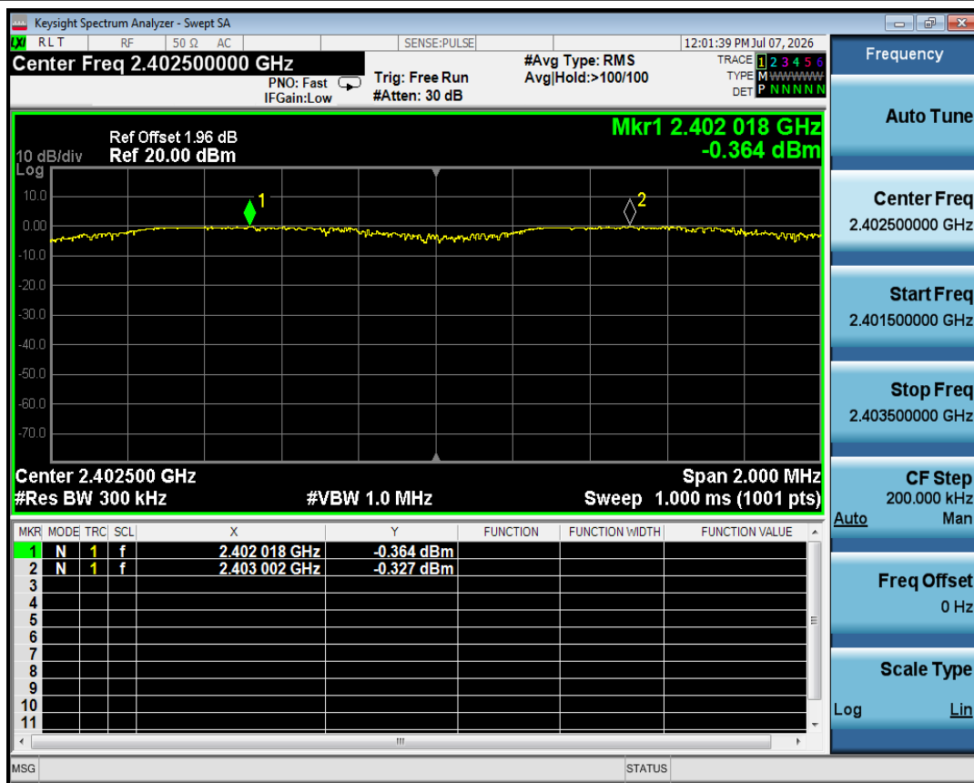
CFS NVNT 2-DH1 2402MHz Ant1
