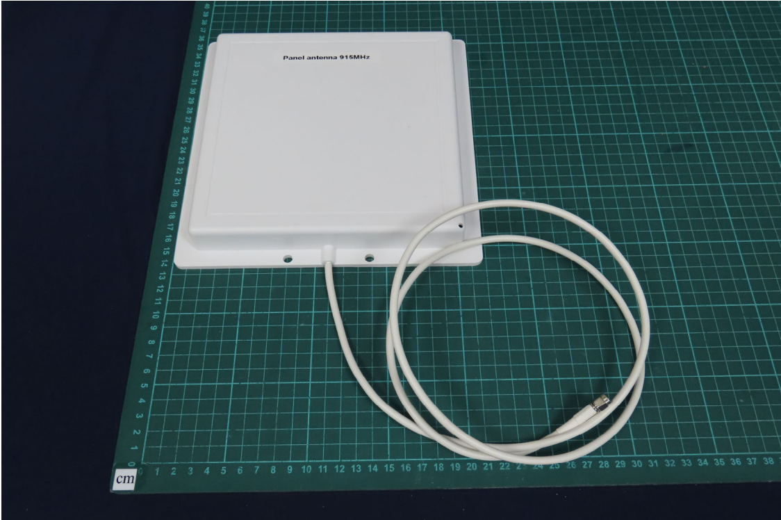
(27)EUT Photo- 915MHz Antenna
