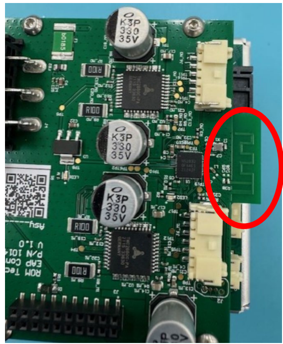
Figure 18; Trace antennae 10145-200 Rev 2 for Bluetooth
