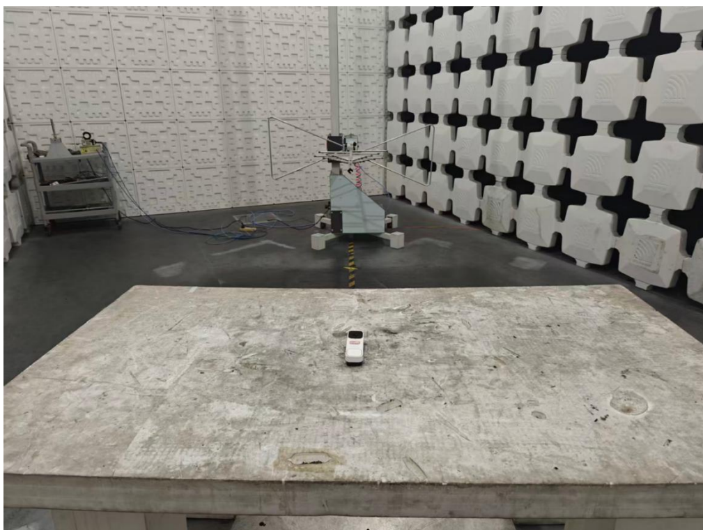
Radiated Setup for Above 1 GHz (433.92MHz)
