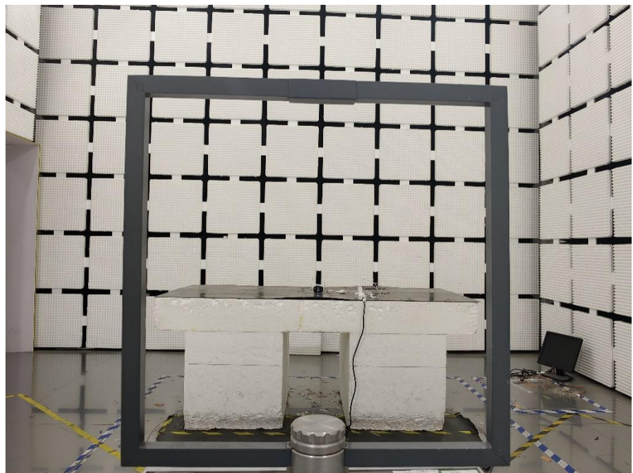
Radiation Emission Test Setup (Below 30MHz)
