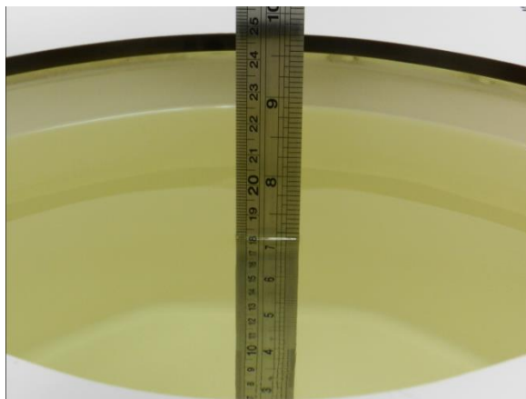
Fig 11.2 Photo of Liquid Height for Body SAR
