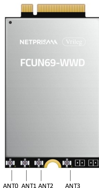
Figure 23: FCUN69-WWD Antenna Connectors
