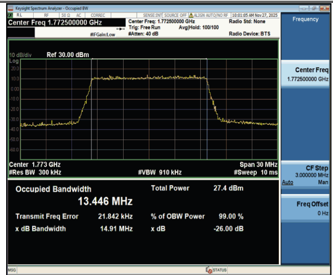
Band66-15MHz-256QAM-132597-75RB#0-PASS
