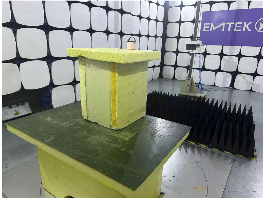
Spurious Emission Test Setup (30MHz-1GHz)
