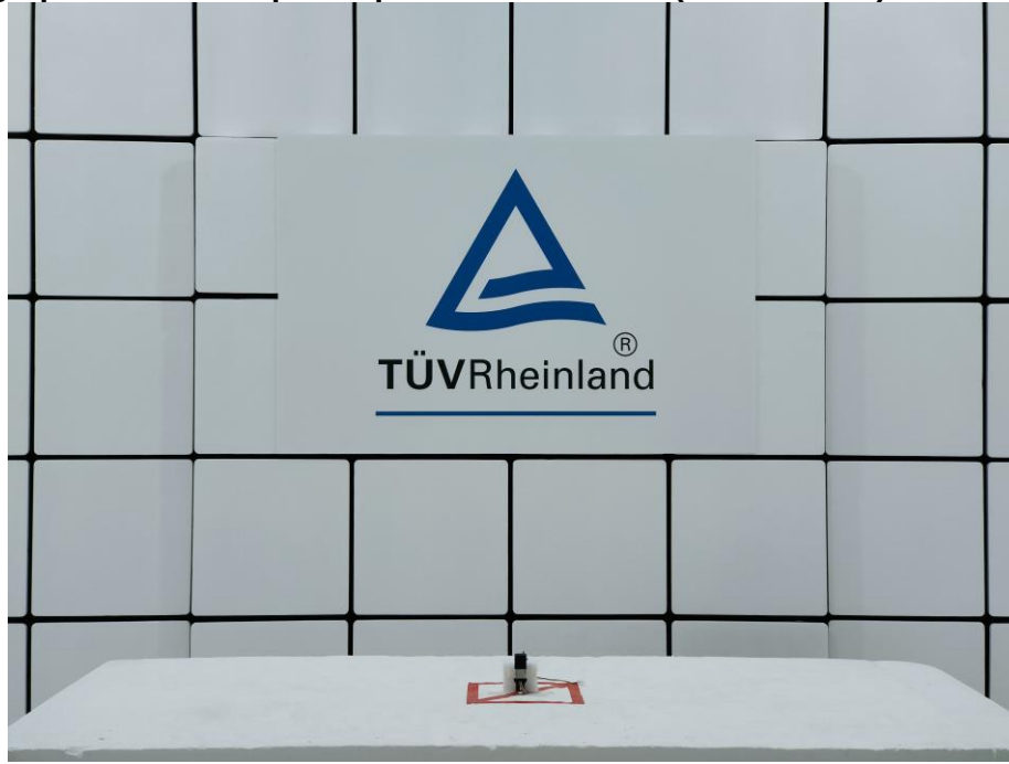
Photograph 2: Test Setup for Spurious Emissions (Front View 2)
