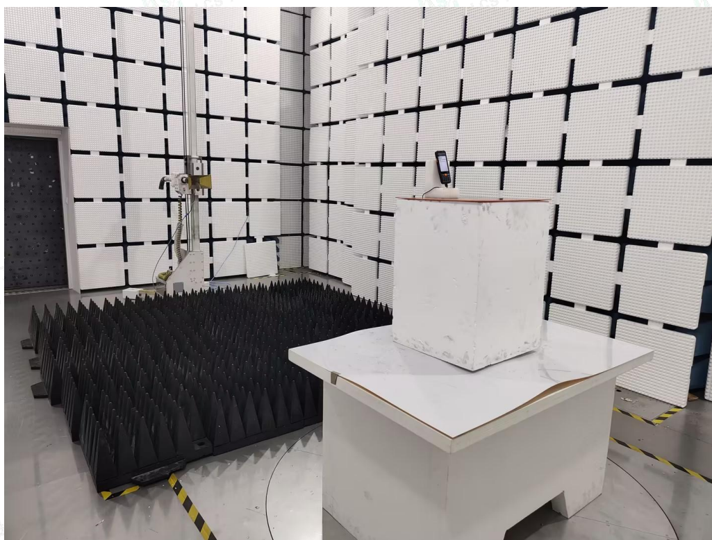
Radiated Emissions Measurement (Above 1GHz)
