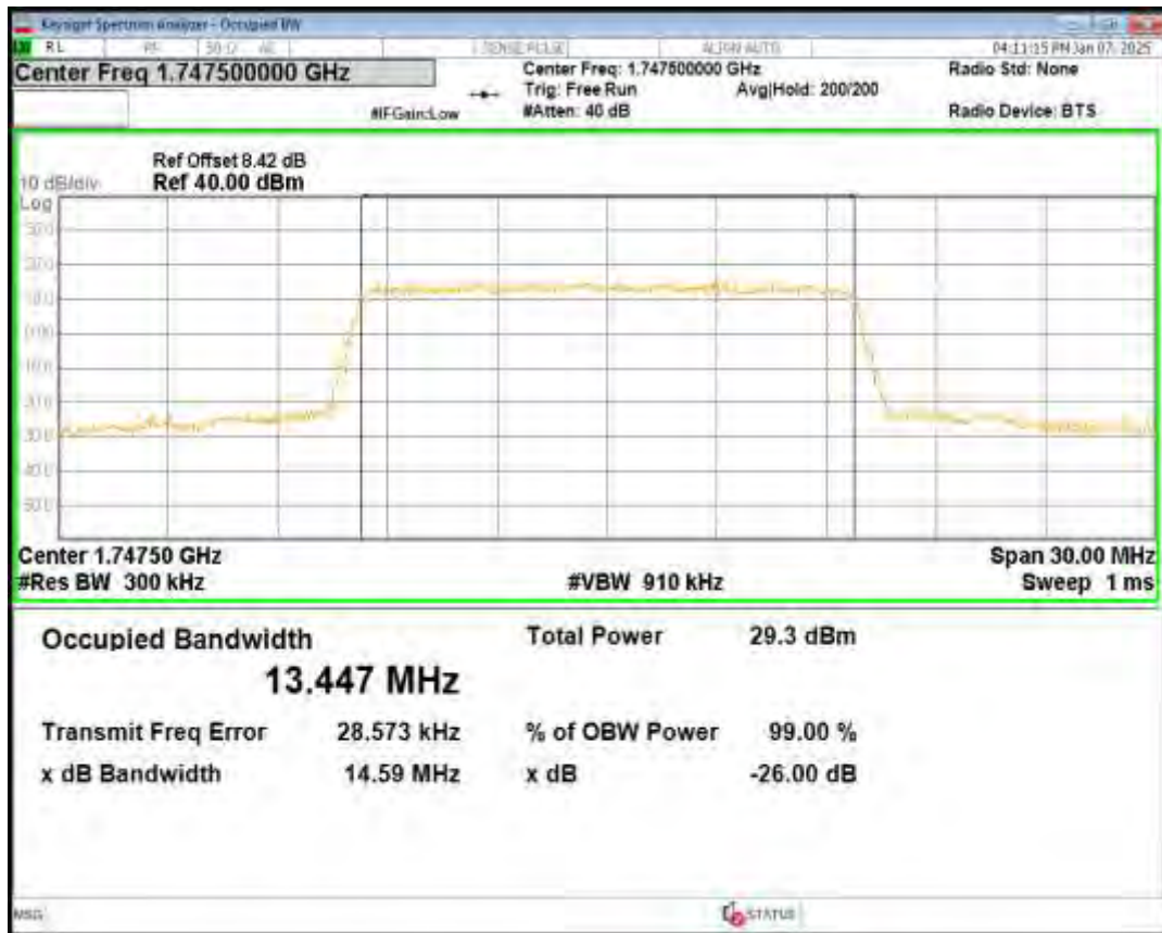
Band4 QPSK BW=20MHz Channel=20050 RB Size=100 Position=#0
