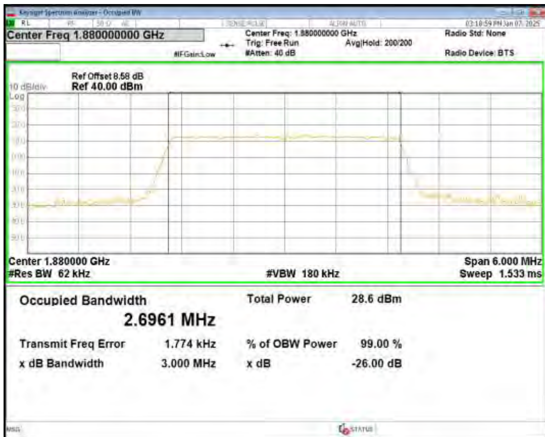
Band2 16QAM BW=20MHz Channel=18900 RB Size=100 Position=#0
