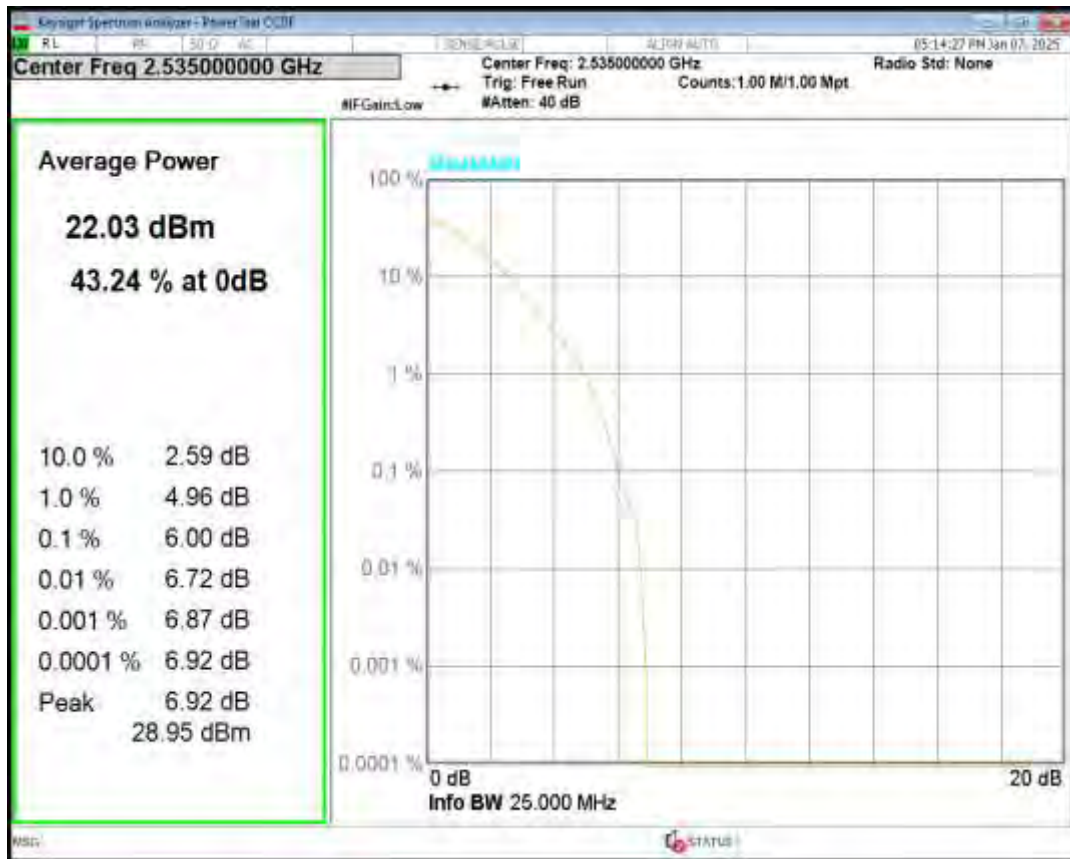
Band7 QPSK BW=5MHz Channel=21100 RB Size=1 Position=#0
