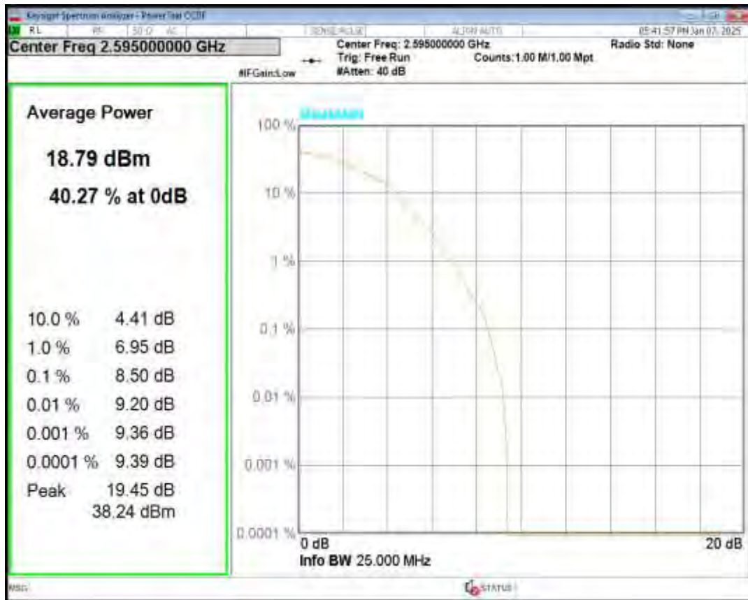
Band38 16QAM BW=20MHz Channel=38150 RB Size=1 Position=#0
