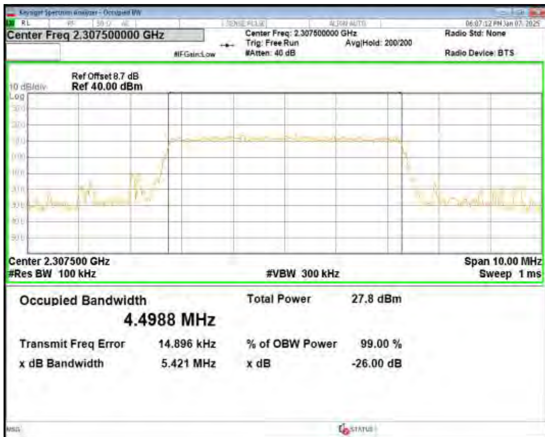
Band40(2305-2315) 16QAM BW=5MHz Channel=38750 RB Size=25 Position=#0
