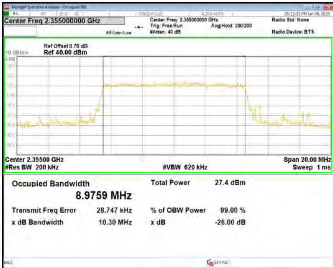
Band40(2350-2360) 16QAM BW=5MHz Channel=39175 RB Size=25 Position=#0
