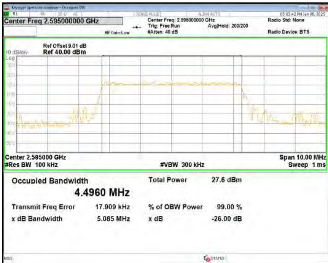
Band38 16QAM BW=5MHz Channel=37775 RB Size=25 Position=#0
