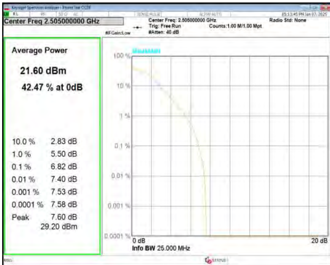
Band7 16QAM BW=10MHz Channel=21100 RB Size=1 Position=#0
