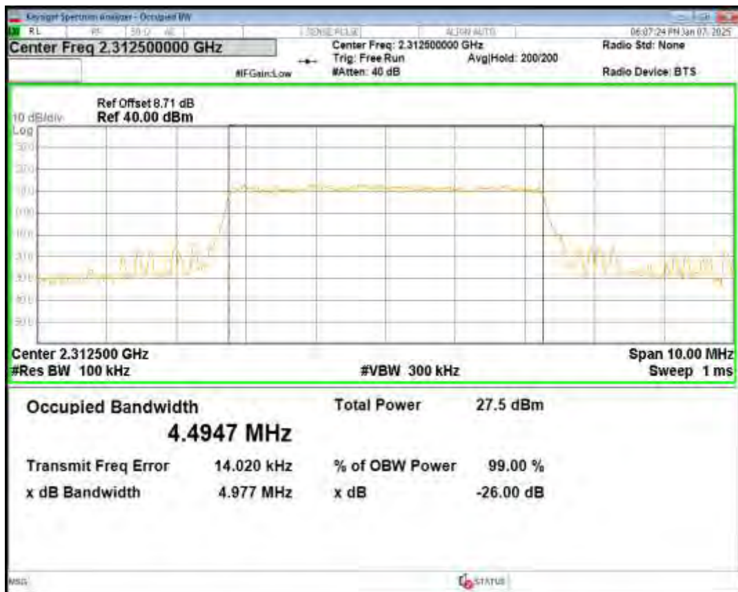
Band40(2305-2315) QPSK BW=10MHz Channel=38750 RB Size=50 Position=#0
