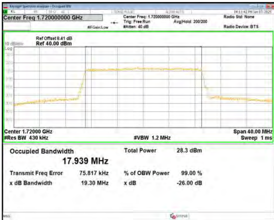
Band4 16QAM BW=20MHz Channel=20175 RB Size=100 Position=#0
