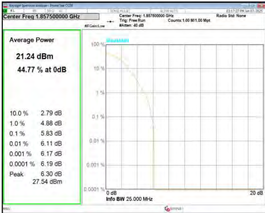
Band2 16QAM BW=20MHz Channel=18900 RB Size=1 Position=#0
