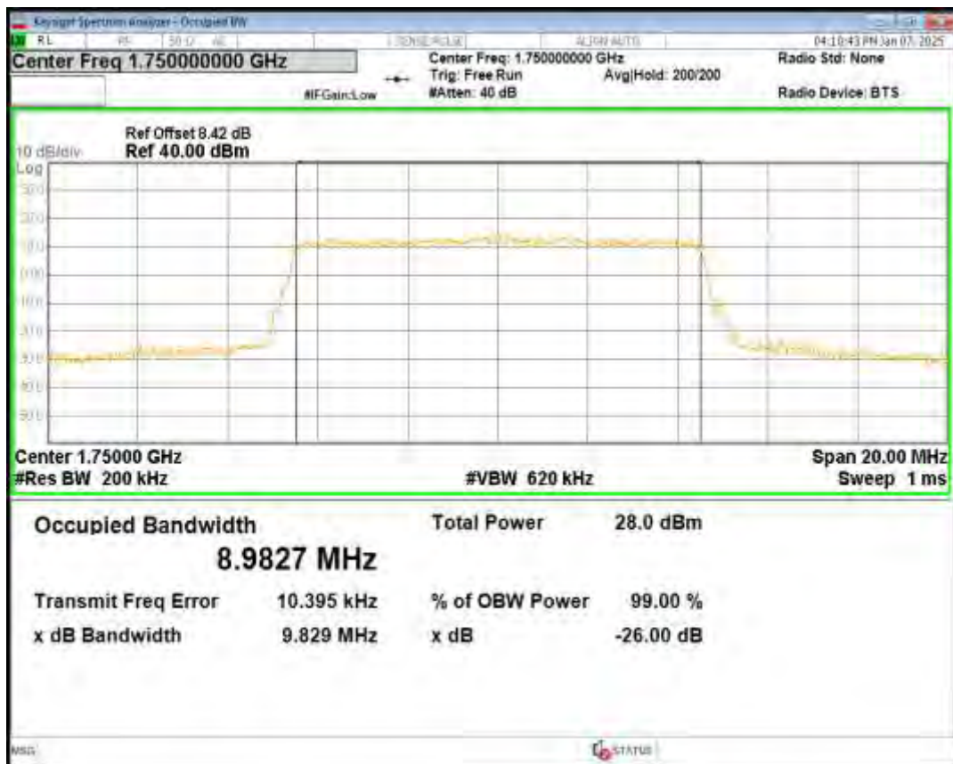
Band4 16QAM BW=15MHz Channel=20025 RB Size=75 Position=#0
