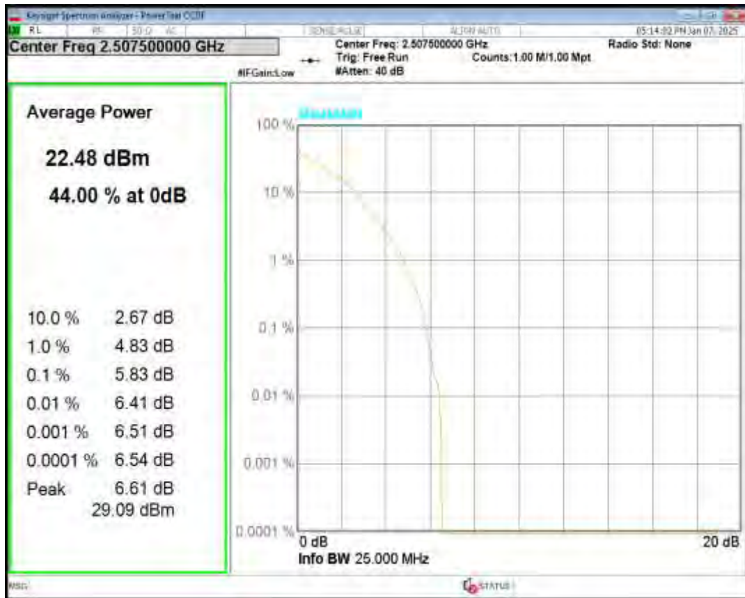
Band7 QPSK BW=15MHz Channel=21100 RB Size=1 Position=#0
