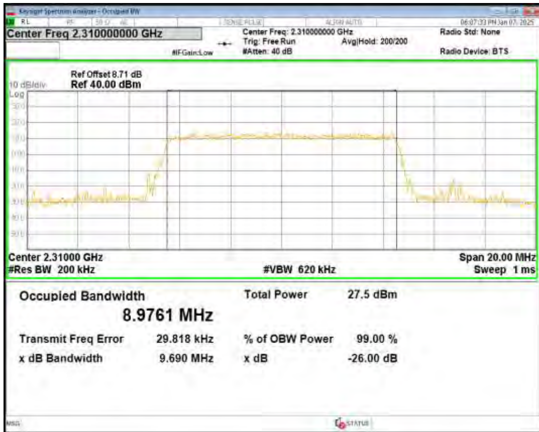
Band40(2305-2315) 16QAM BW=5MHz Channel=38725 RB Size=25 Position=#0
