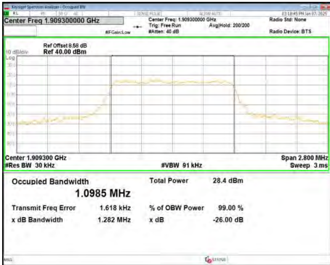
Band2 16QAM BW=10MHz Channel=18650 RB Size=50 Position=#0
