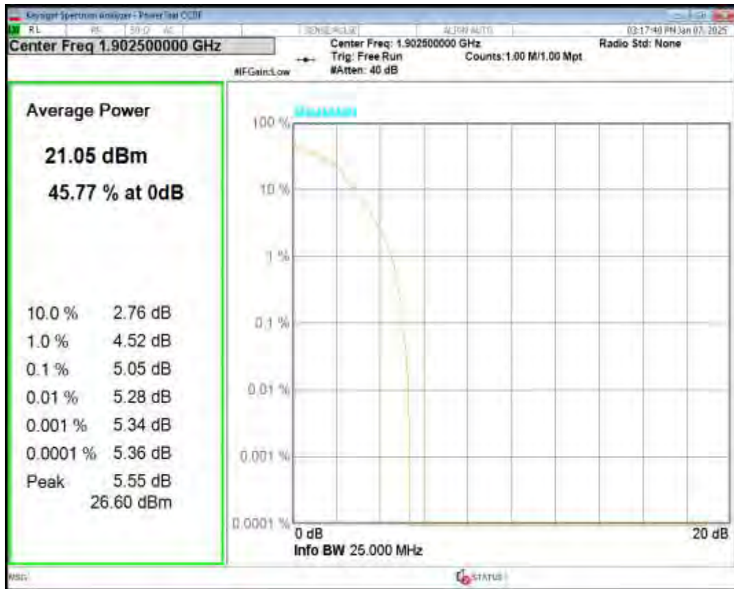
Band2 16QAM BW=15MHz Channel=18900 RB Size=1 Position=#0
