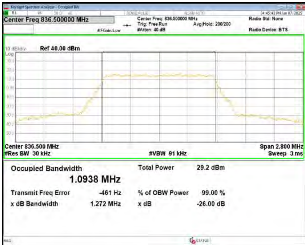
Band5 16QAM BW=1.4MHz Channel=20643 RB Size=6 Position=#0
