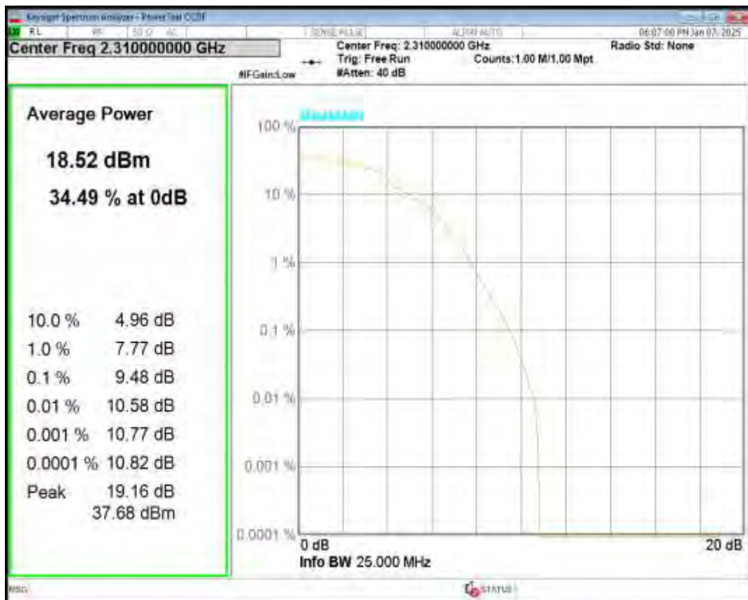
Band40(2305-2315) QPSK BW=5MHz Channel=38725 RB Size=1 Position=#0
