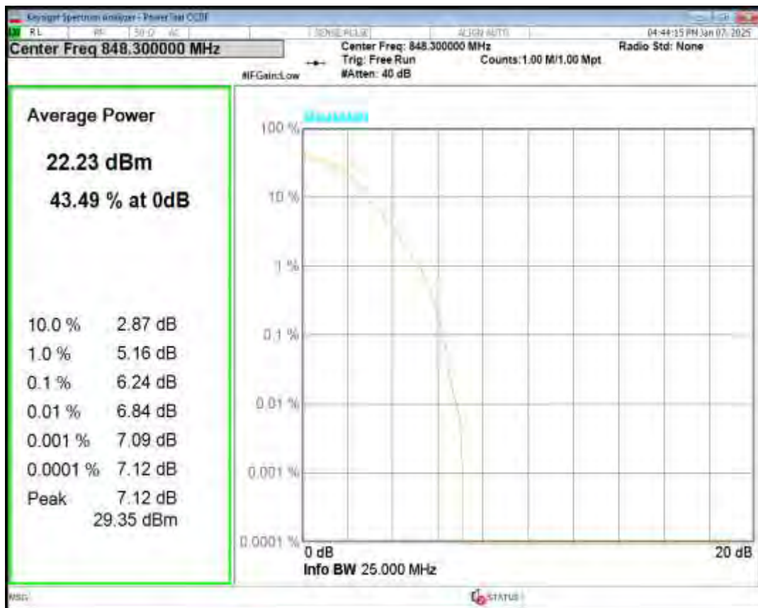
Band5 16QAM BW=10MHz Channel=20450 RB Size=1 Position=#0
