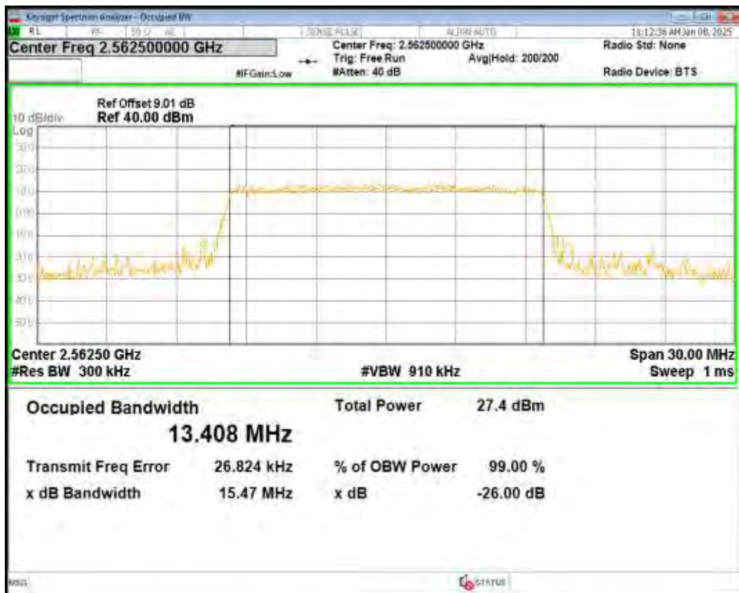
Band41(2555-2655) 16QAM BW=15MHz Channel=40740 RB Size=75 Position=#0
