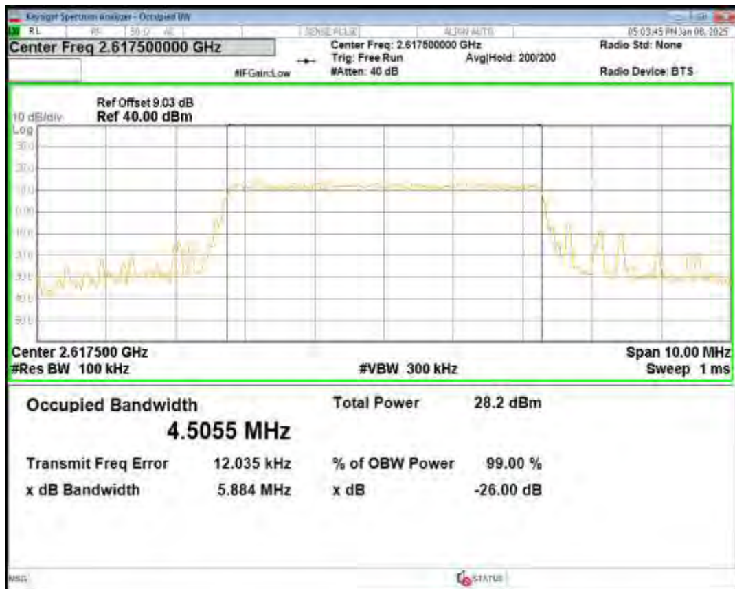
Band4 16QAM BW=1.4MHz Channel=19957 RB Size=6 Position=#0
