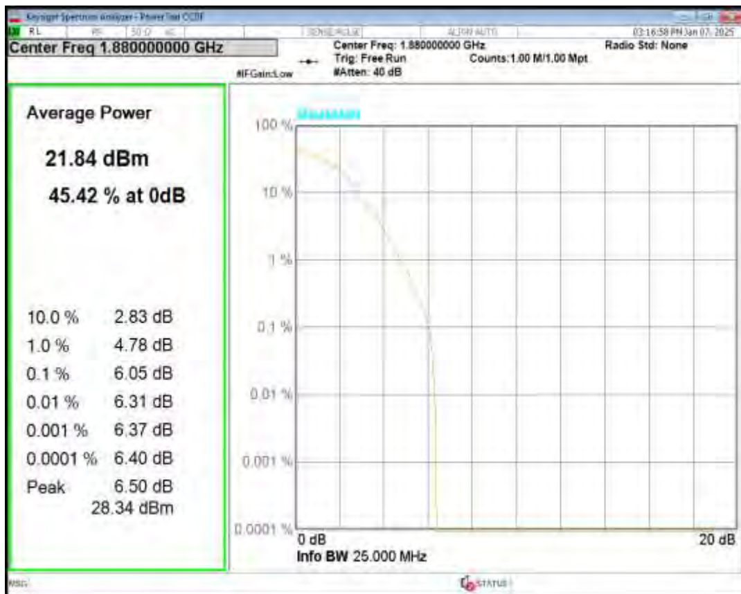
Band2 16QAM BW=10MHz Channel=19150 RB Size=1 Position=#0
