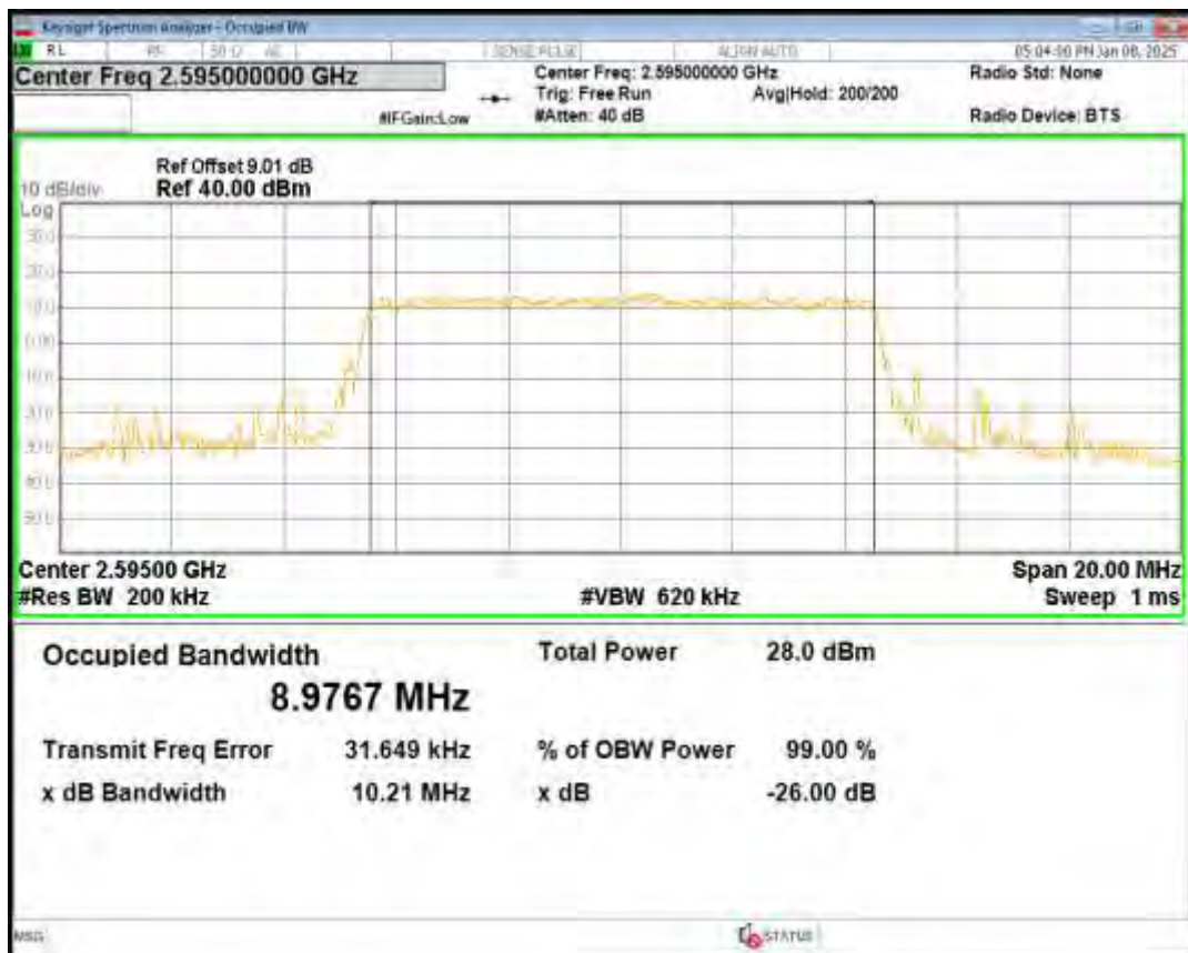
Band38 QPSK BW=10MHz Channel=38200 RB Size=50 Position=#0
