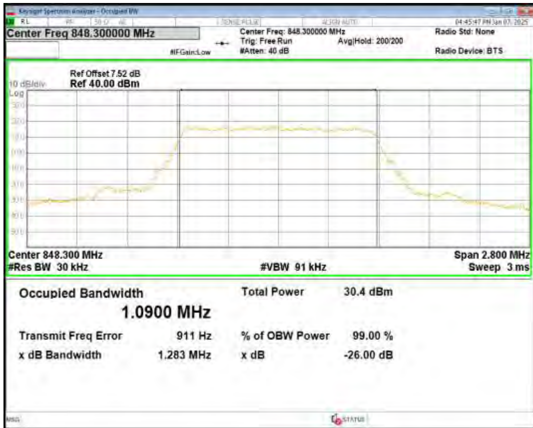
Band5 QPSK BW=5MHz Channel=20525 RB Size=25 Position=#0
