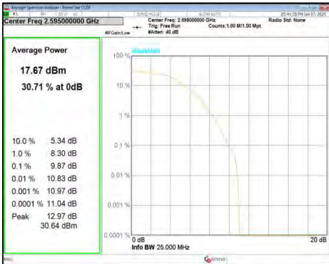
Band38 QPSK BW=15MHz Channel=38175 RB Size=1 Position=#0
