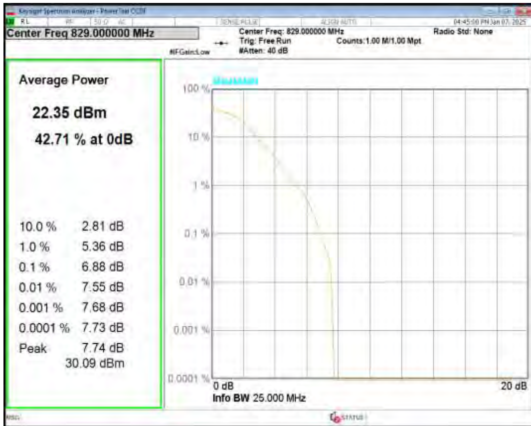
Band5 16QAM BW=5MHz Channel=20525 RB Size=1 Position=#0
