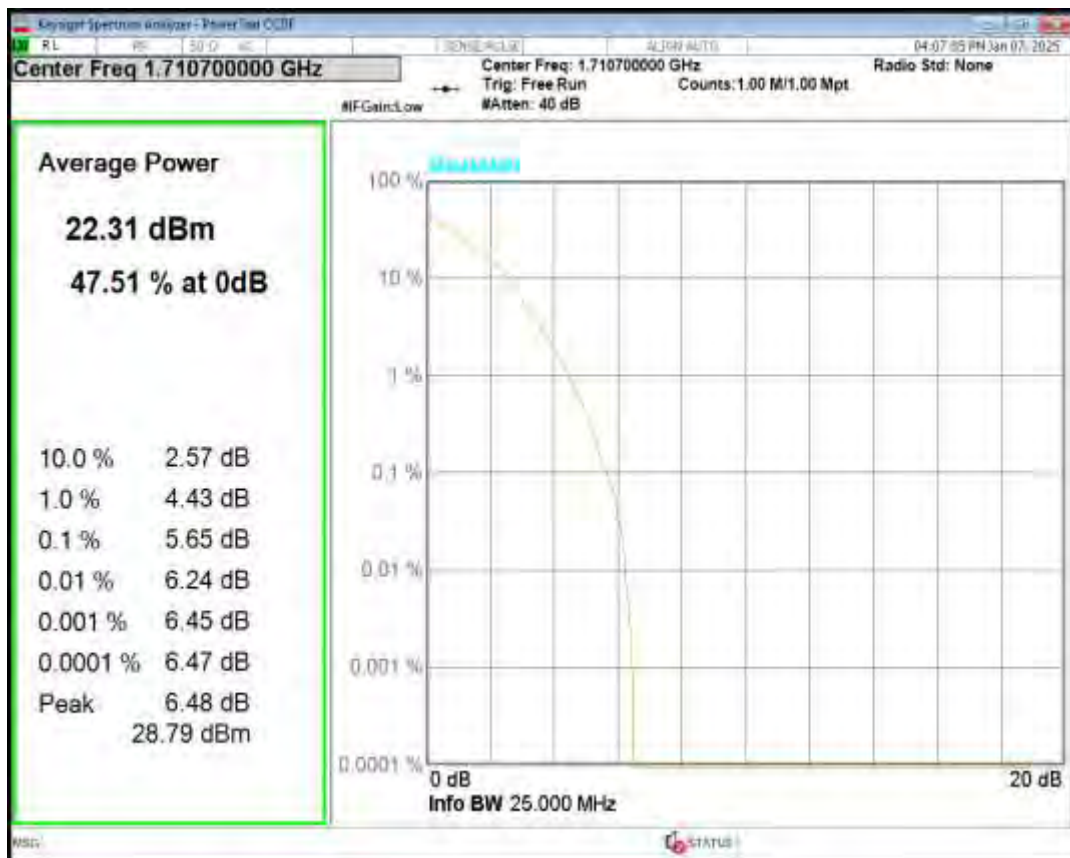
Band4 QPSK BW=1.4MHz Channel=20175 RB Size=1 Position=#0
