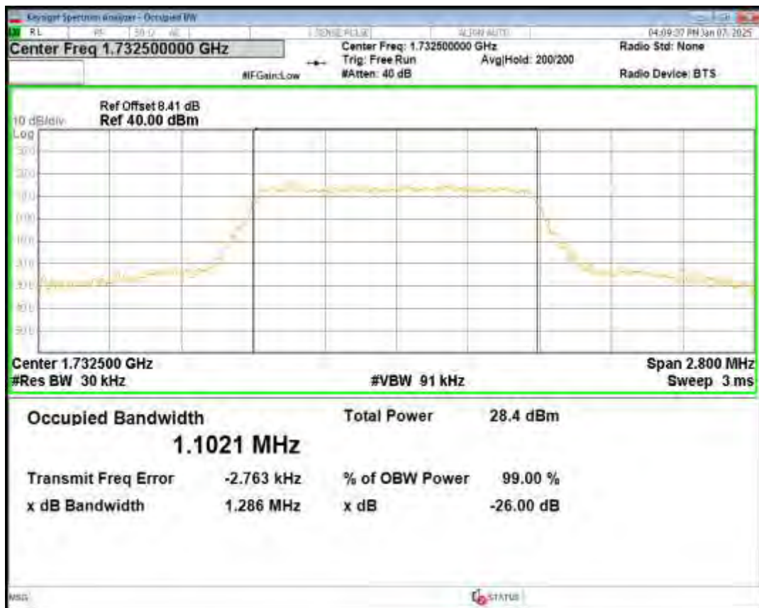
Band4 16QAM BW=1.4MHz Channel=20393 RB Size=6 Position=#0
