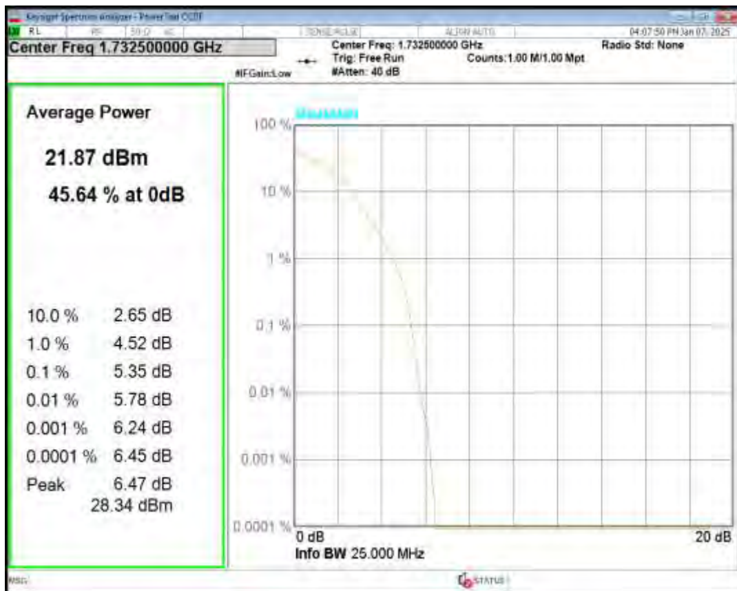
Band4 QPSK BW=5MHz Channel=20375 RB Size=1 Position=#0
