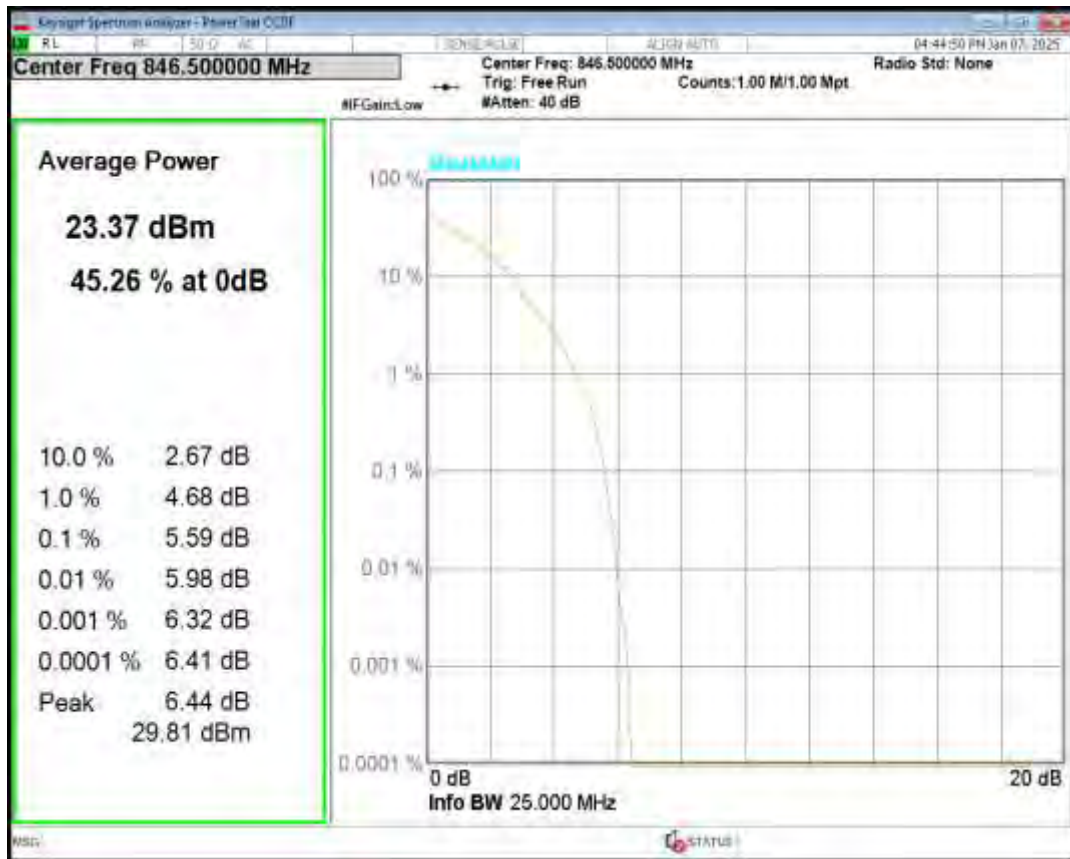
Band7 16QAM BW=10MHz Channel=20800 RB Size=1 Position=#0
