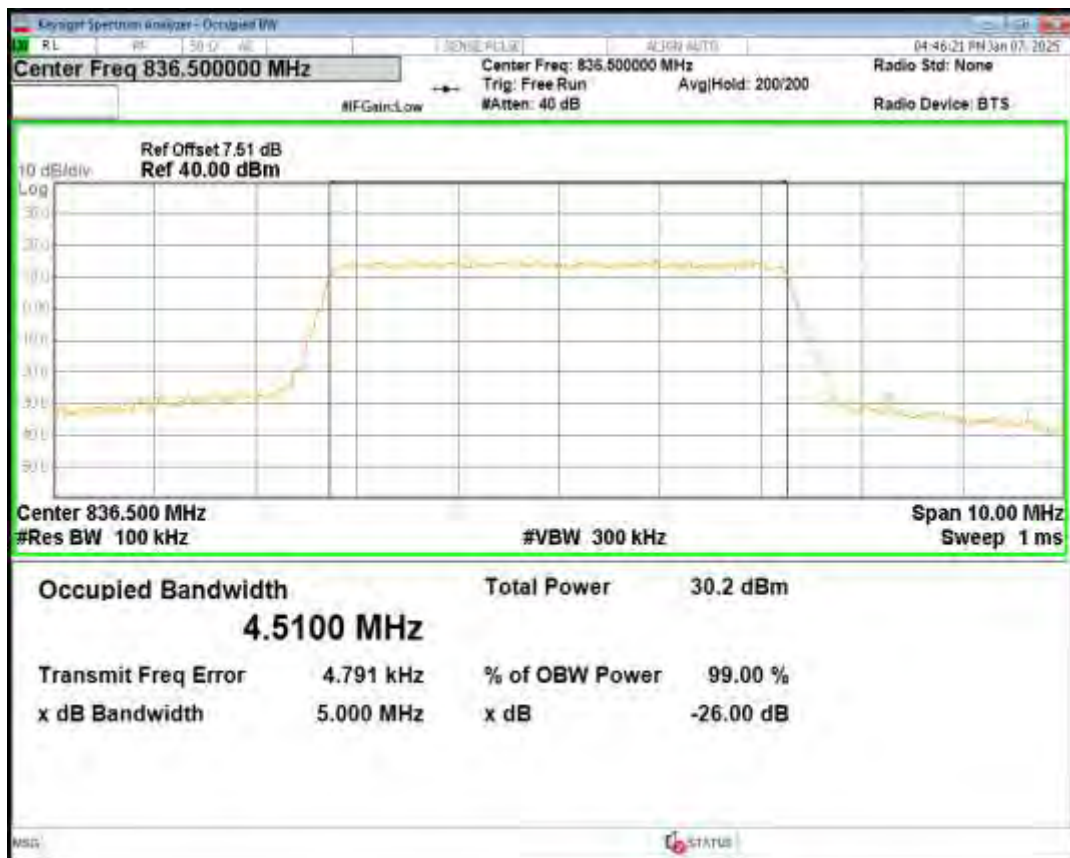
Band5 QPSK BW=3MHz Channel=20525 RB Size=15 Position=#0
