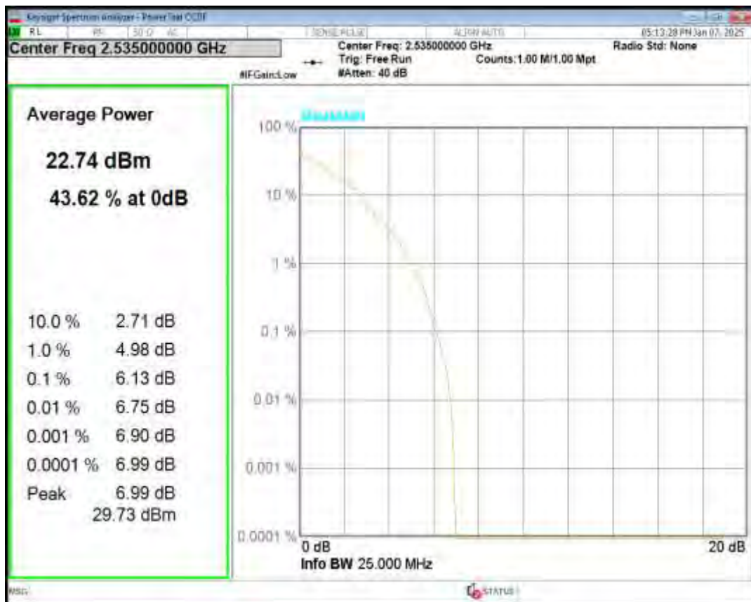
Band7 QPSK BW=20MHz Channel=21350 RB Size=1 Position=#0
