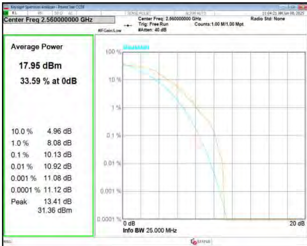
Band41(2555-2655) QPSK BW=10MHz Channel=40740 RB Size=1 Position=#0
