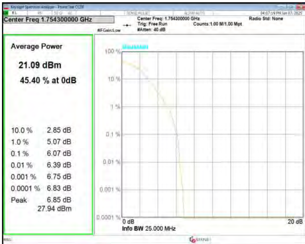
Band4 16QAM BW=10MHz Channel=20000 RB Size=1 Position=#0
