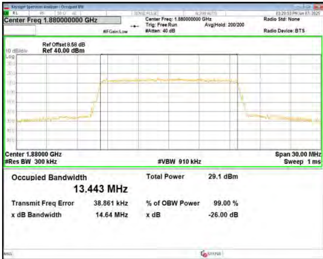
Band2 QPSK BW=1.4MHz Channel=19193 RB Size=6 Position=#0
