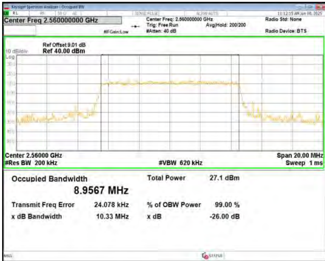
Band41(2555-2655) 16QAM BW=10MHz Channel=40740 RB Size=50 Position=#0
