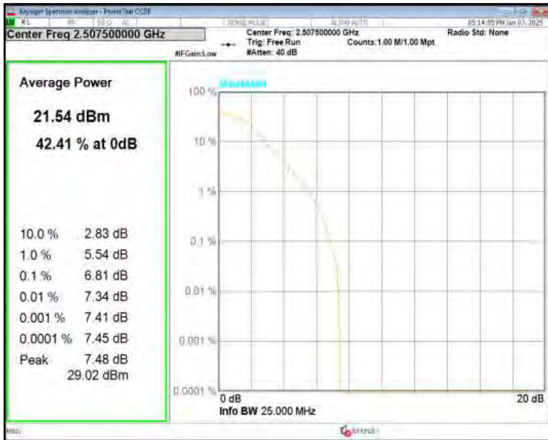
Band7 16QAM BW=5MHz Channel=21100 RB Size=1 Position=#0
