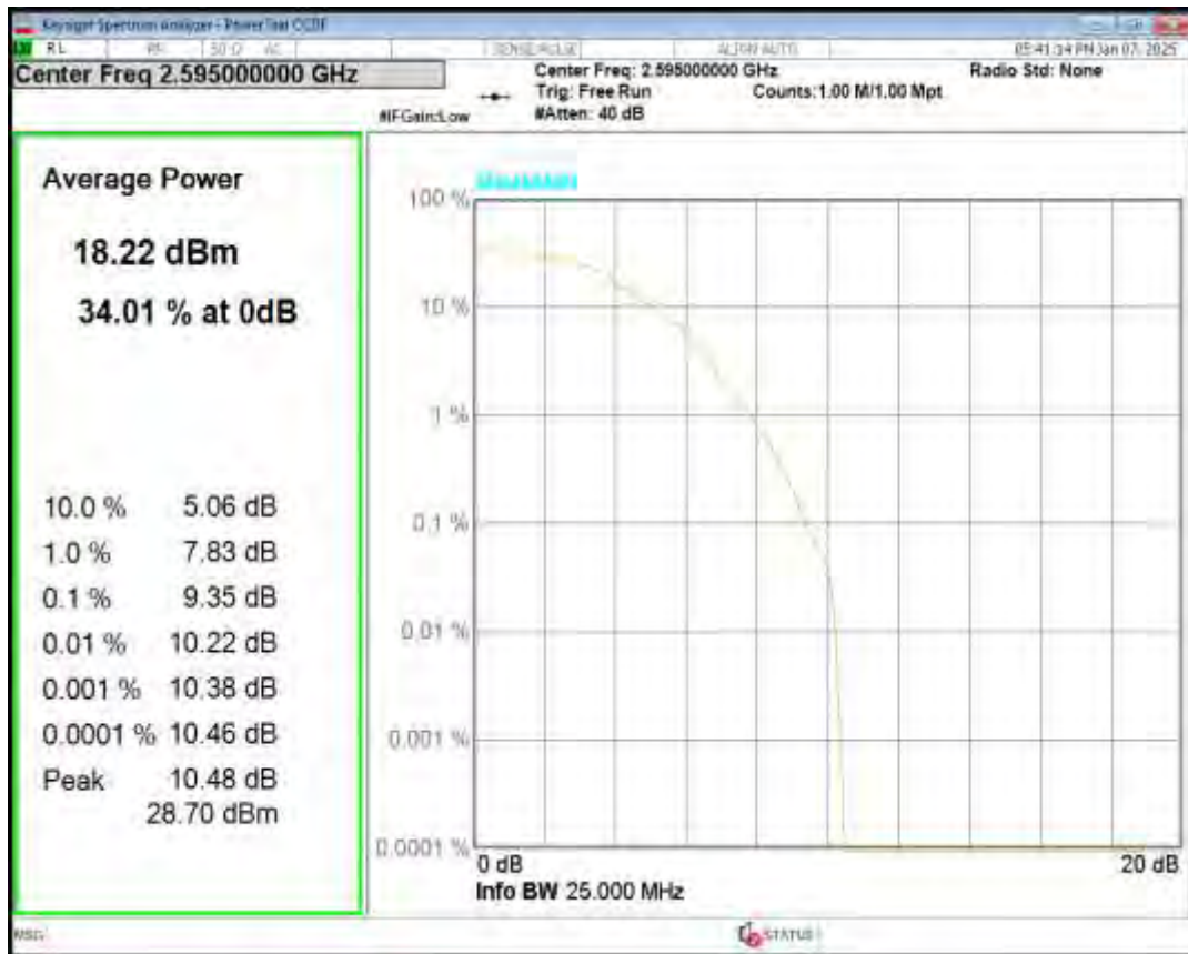
Band38 QPSK BW=10MHz Channel=38200 RB Size=1 Position=#0
