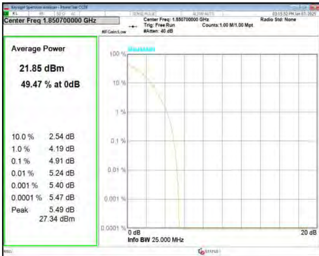
Band2 QPSK BW=10MHz Channel=19150 RB Size=1 Position=#0
