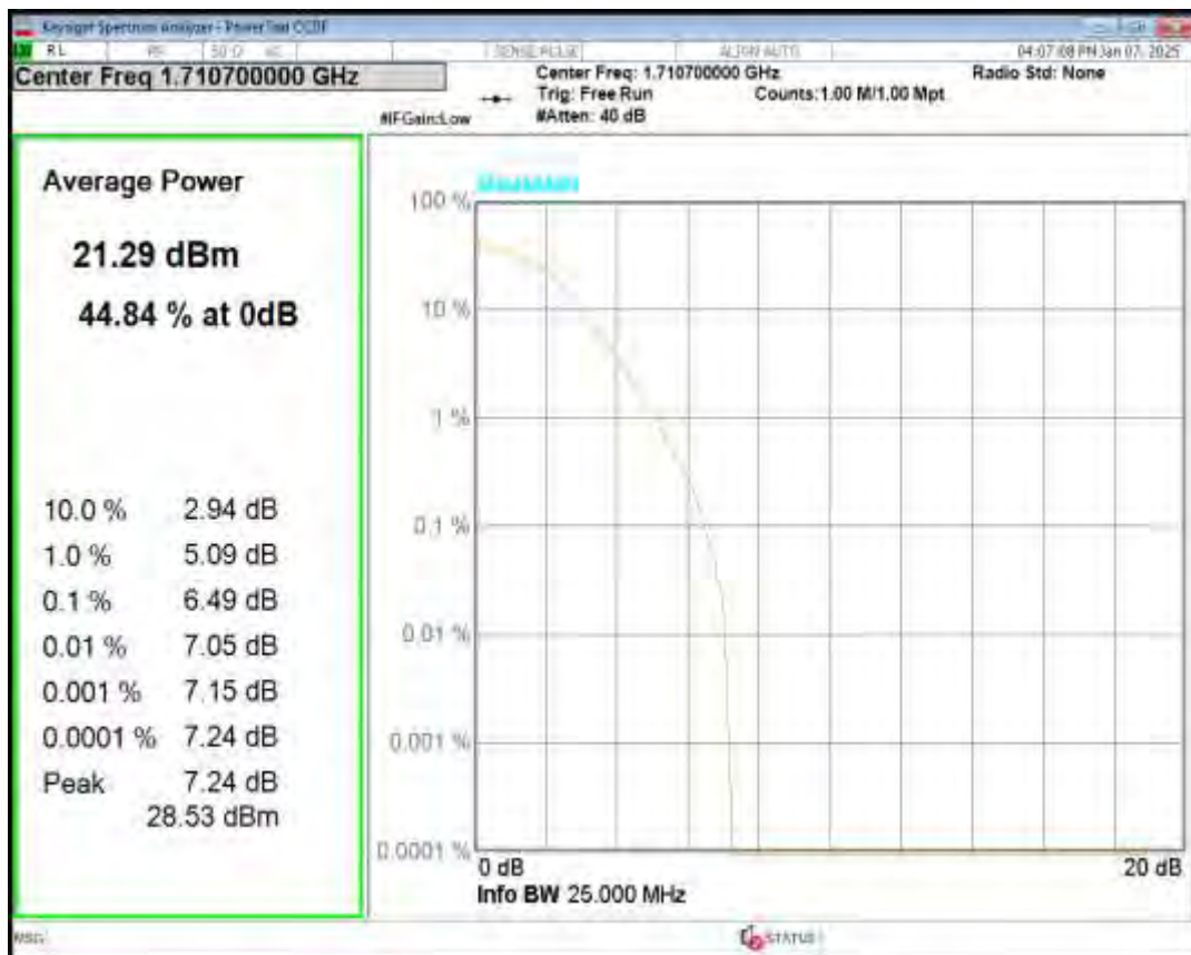
Band4 16QAM BW=1.4MHz Channel=20175 RB Size=1 Position=#0
