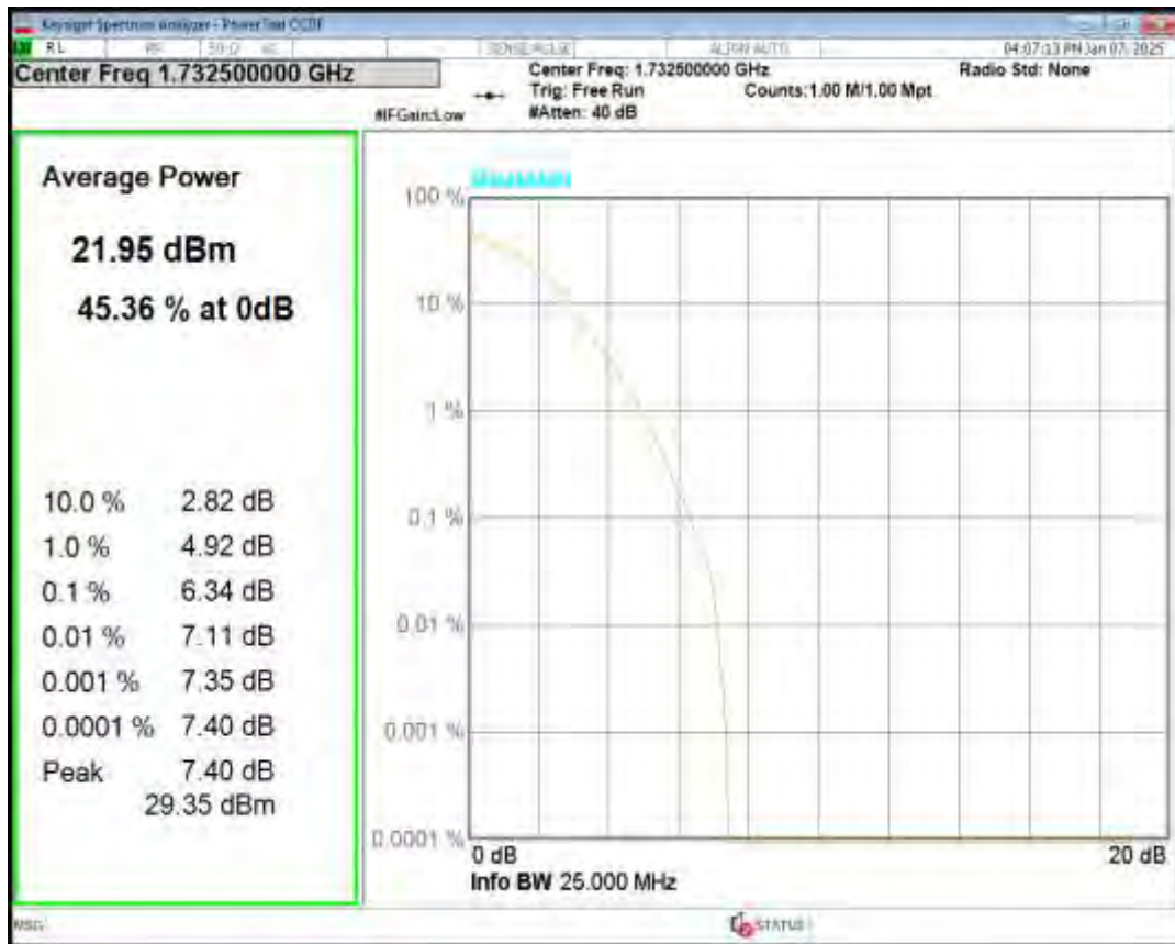
Band4 16QAM BW=1.4MHz Channel=20393 RB Size=1 Position=#0
