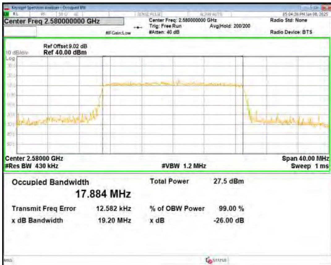
Band38 16QAM BW=15MHz Channel=38175 RB Size=75 Position=#0
