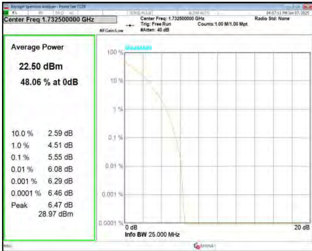
Band4 QPSK BW=1.4MHz Channel=20393 RB Size=1 Position=#0
