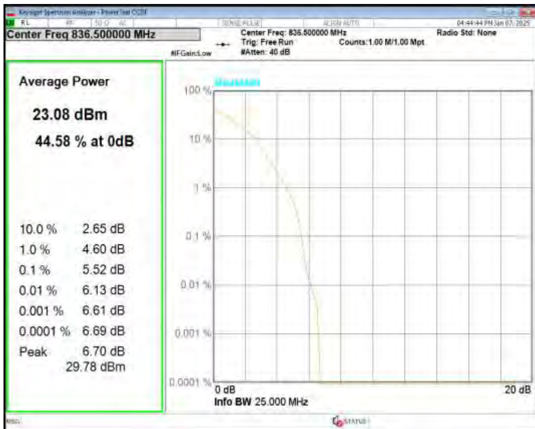
Band5 QPSK BW=3MHz Channel=20635 RB Size=1 Position=#0
