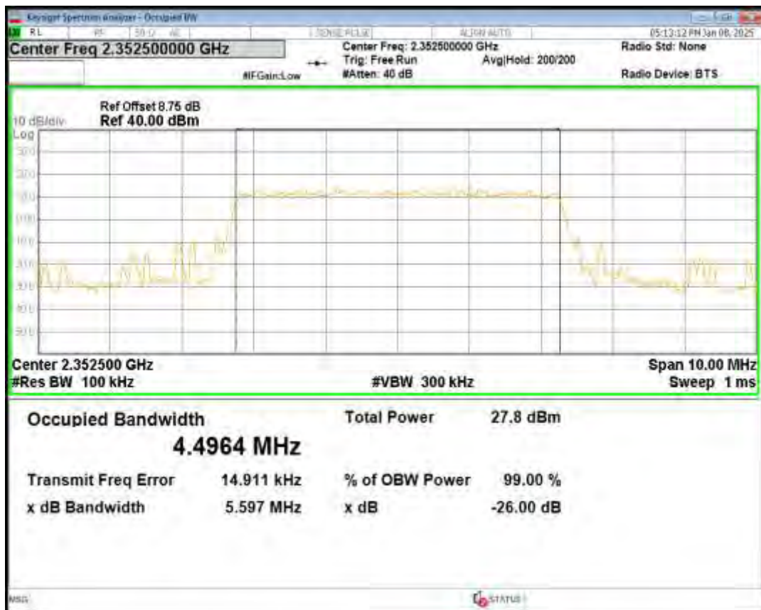
Band40(2350-2360) 16QAM BW=5MHz Channel=39200 RB Size=25 Position=#0
