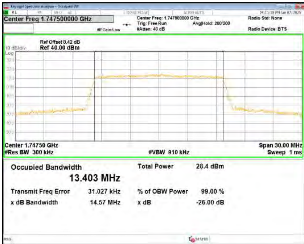
Band4 16QAM BW=20MHz Channel=20050 RB Size=100 Position=#0
