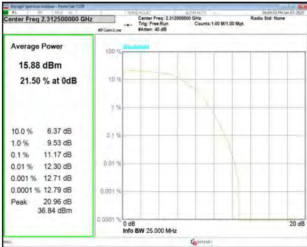
Band40(2350-2360) 16QAM BW=10MHz Channel=39200 RB Size=1 Position=#0
