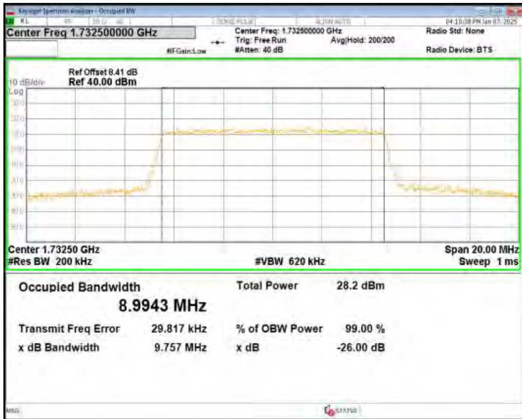
Band4 16QAM BW=10MHz Channel=20350 RB Size=50 Position=#0
