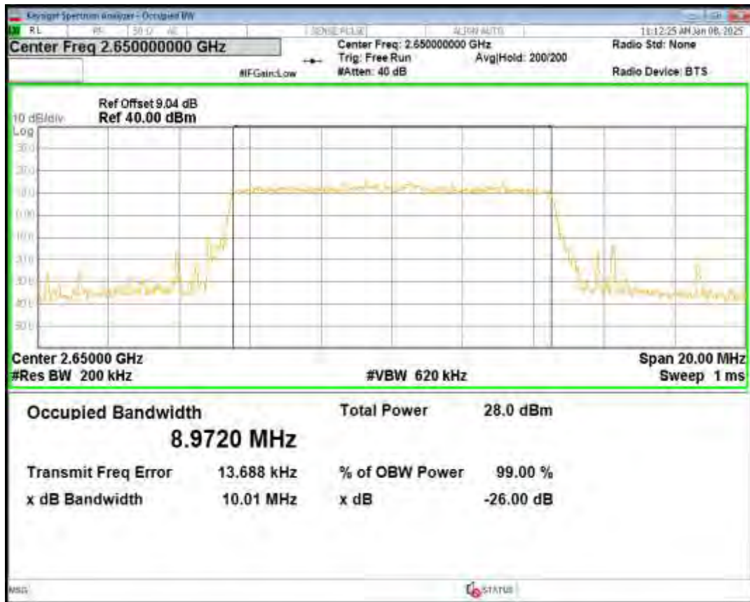
Band41(2555-2655) QPSK BW=15MHz Channel=40315 RB Size=75 Position=#0
