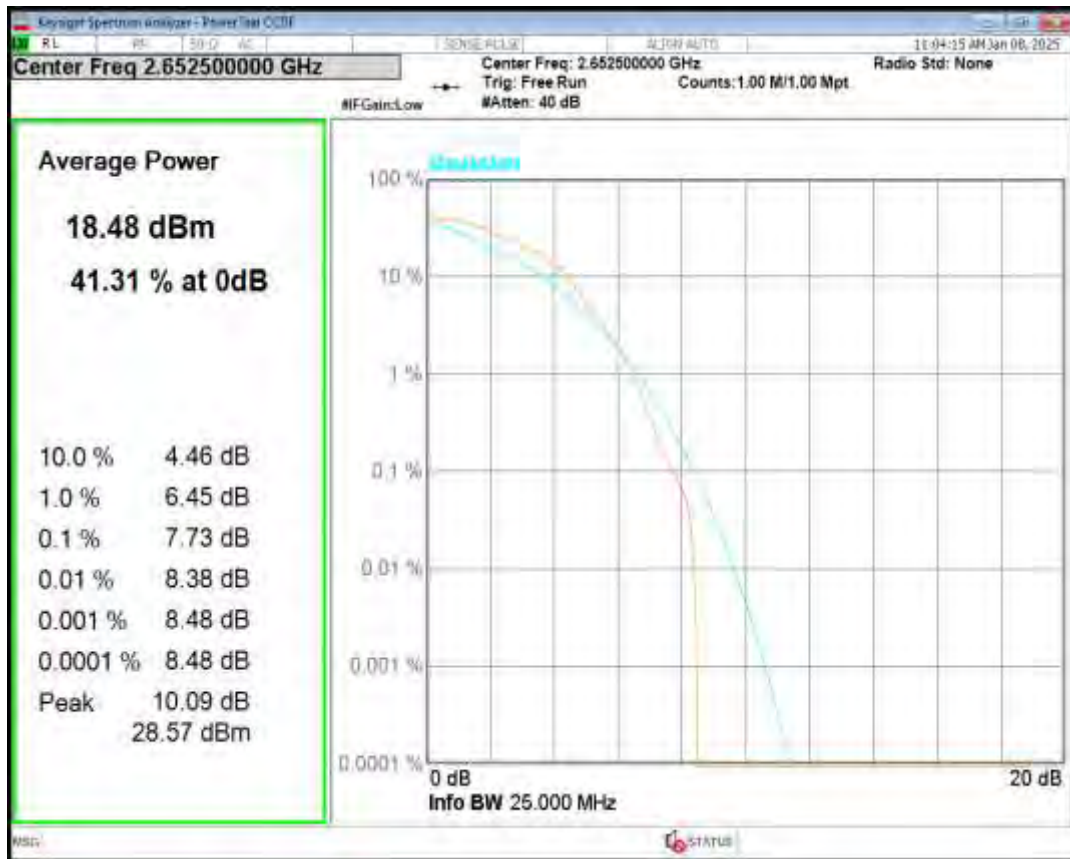
Band41(2555-2655) 16QAM BW=20MHz Channel=40340 RB Size=1 Position=#0
