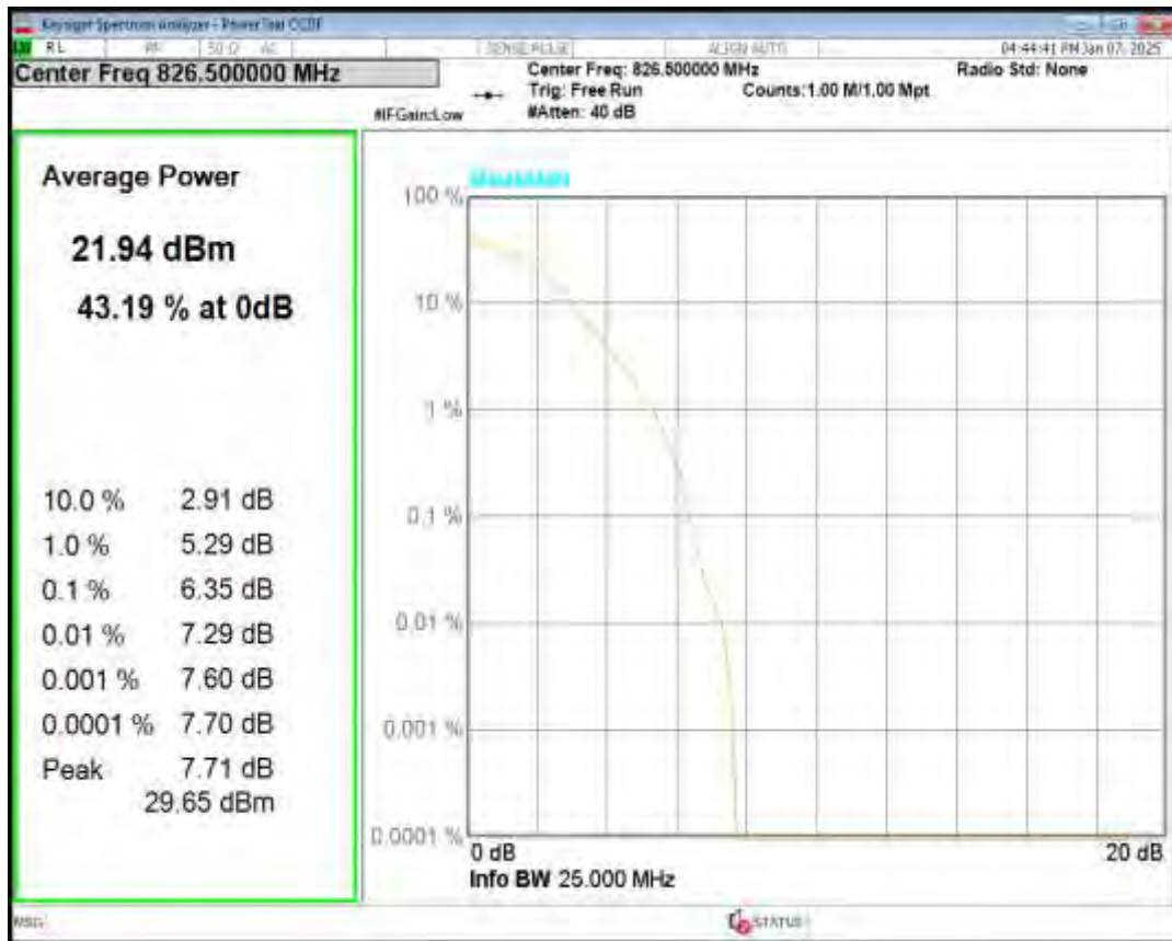
Band5 16QAM BW=3MHz Channel=20635 RB Size=1 Position=#0
