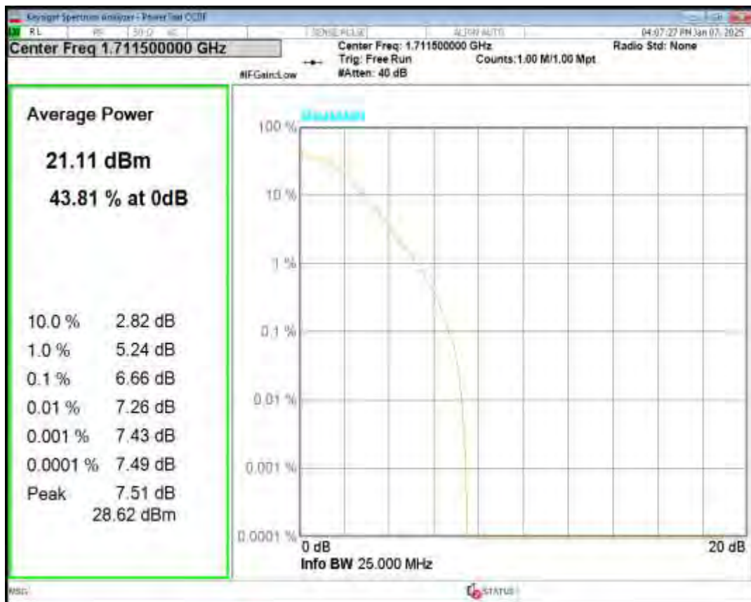
Band4 16QAM BW=3MHz Channel=20175 RB Size=1 Position=#0
