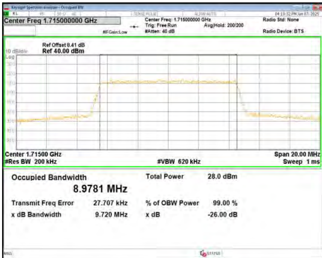
Band4 16QAM BW=10MHz Channel=20175 RB Size=50 Position=#0
