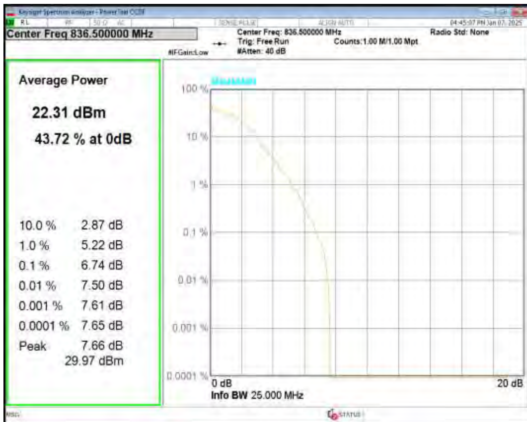
Band5 16QAM BW=3MHz Channel=20525 RB Size=1 Position=#0
