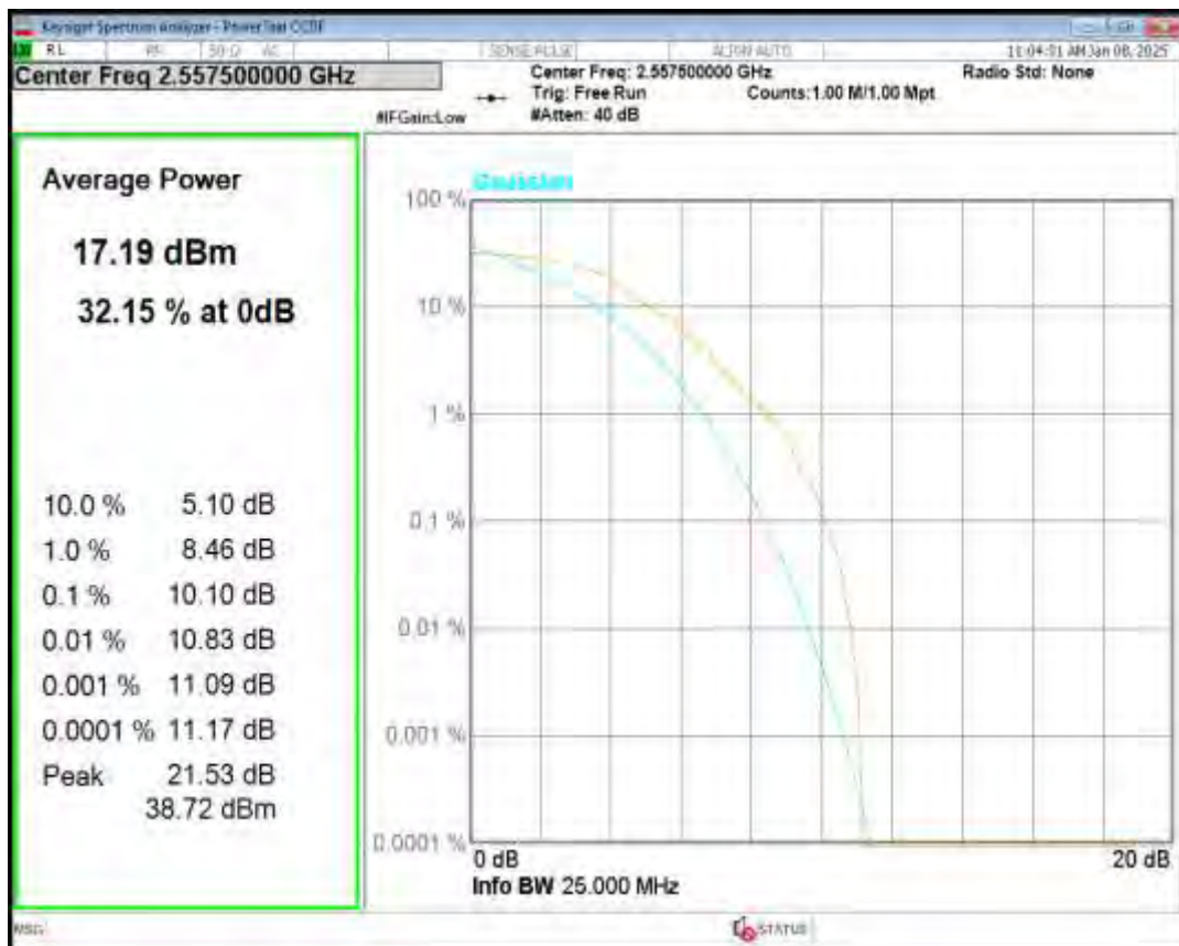
Band41(2555-2655) QPSK BW=5MHz Channel=41215 RB Size=1 Position=#0
