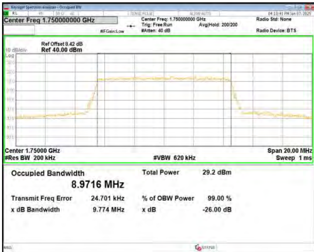
Band4 QPSK BW=15MHz Channel=20025 RB Size=75 Position=#0
