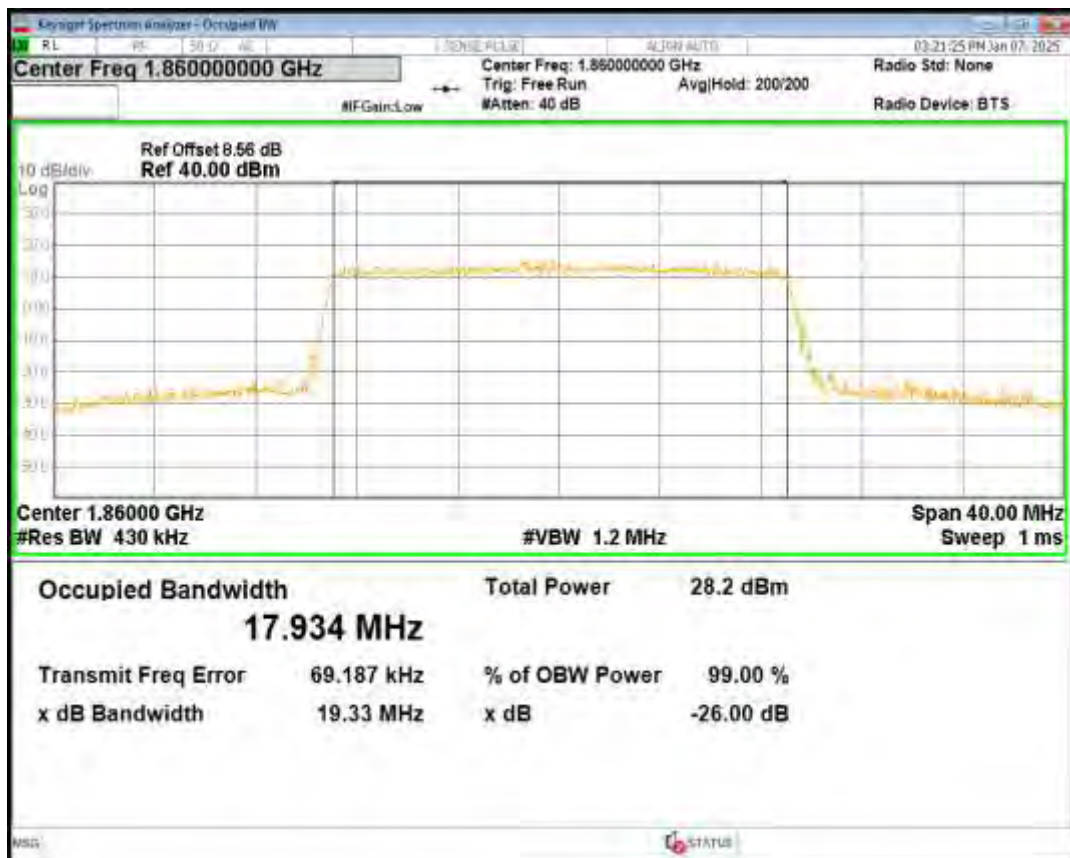
Band2 QPSK BW=1.4MHz Channel=18607 RB Size=6 Position=#0
