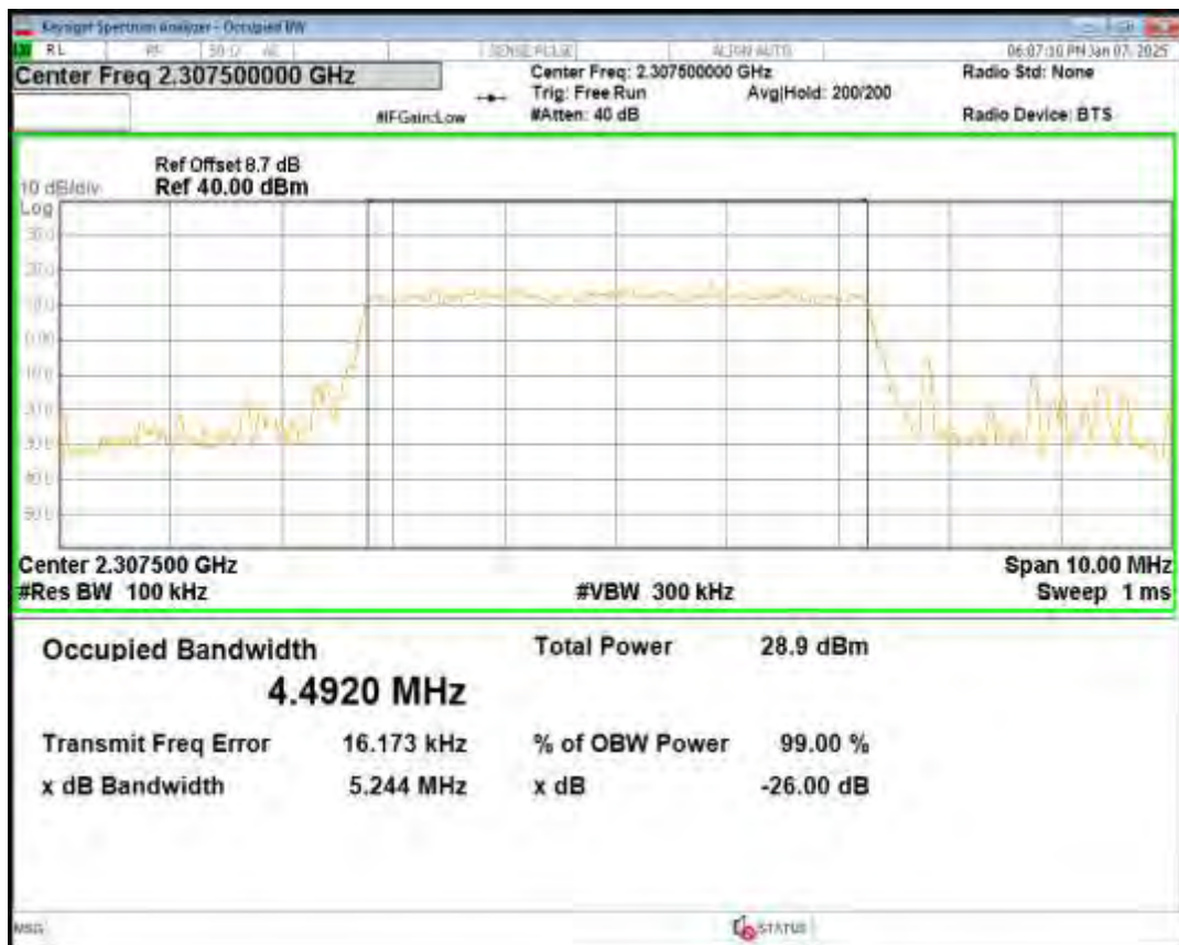
Band40(2305-2315) QPSK BW=5MHz Channel=38750 RB Size=25 Position=#0
