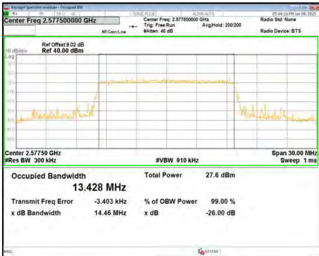
Band38 QPSK BW=10MHz Channel=37800 RB Size=50 Position=#0
