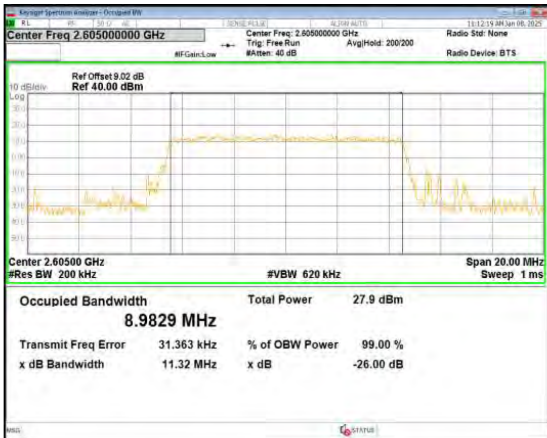
Band41(2555-2655) QPSK BW=10MHz Channel=41190 RB Size=50 Position=#0
