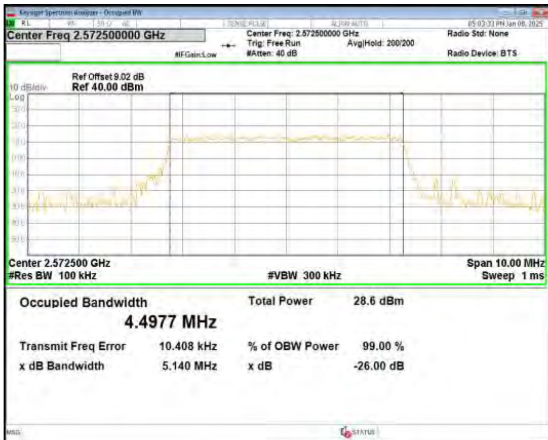
Band38 QPSK BW=5MHz Channel=38000 RB Size=25 Position=#0
