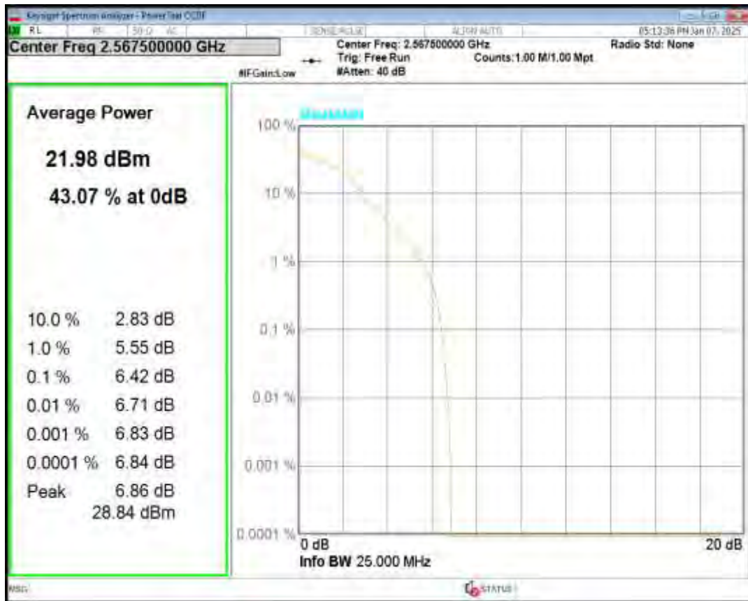
Band7 16QAM BW=20MHz Channel=20850 RB Size=1 Position=#0
