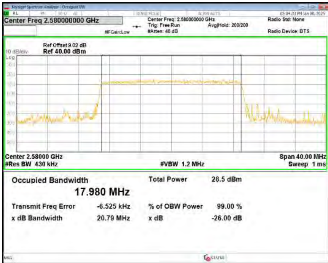
Band38 QPSK BW=20MHz Channel=38000 RB Size=100 Position=#0
