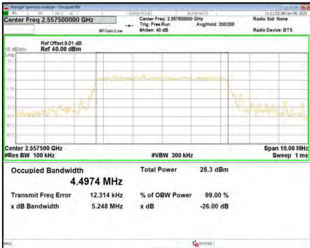
Band41(2555-2655) QPSK BW=5MHz Channel=40740 RB Size=25 Position=#0
