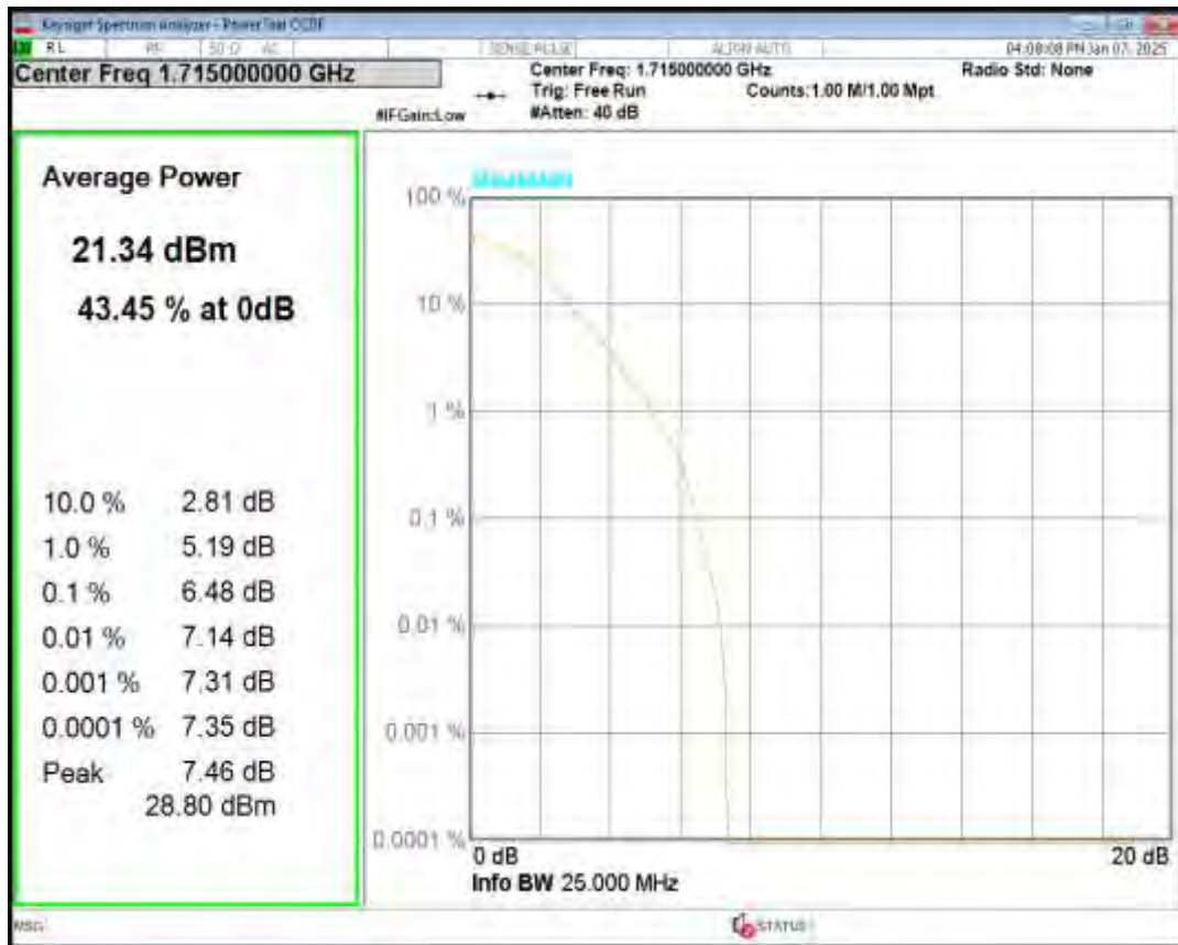
Band4 16QAM BW=10MHz Channel=20175 RB Size=1 Position=#0
