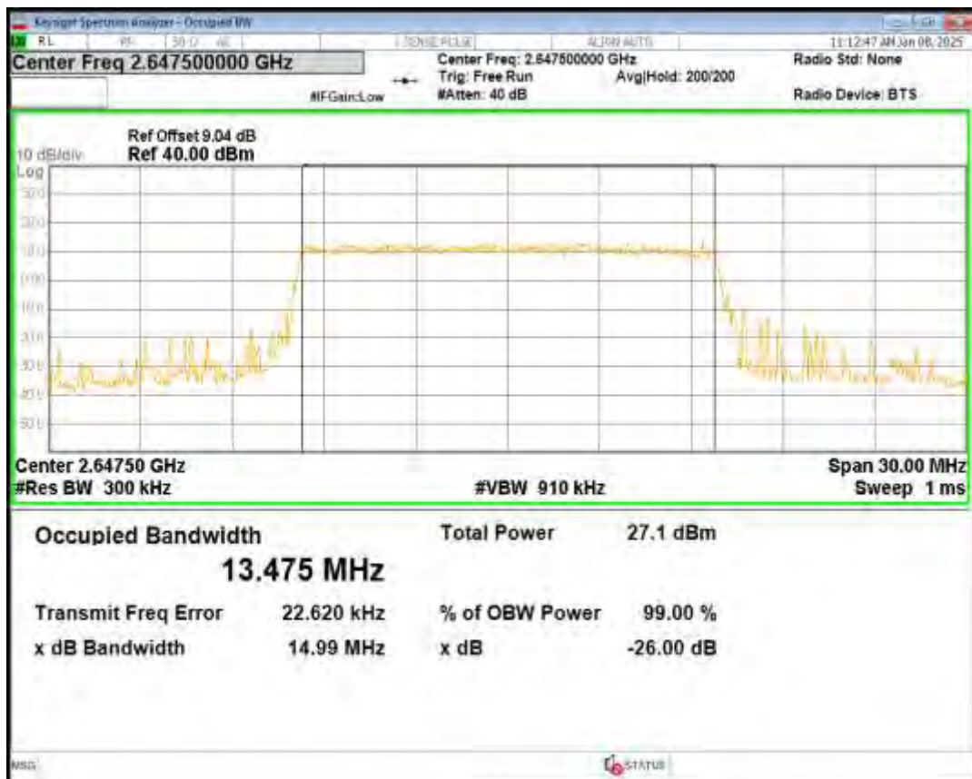
Band41(2555-2655) 16QAM BW=20MHz Channel=40340 RB Size=100 Position=#0
