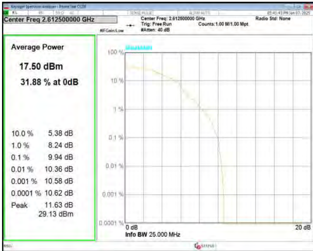
Band38 16QAM BW=20MHz Channel=37850 RB Size=1 Position=#0
