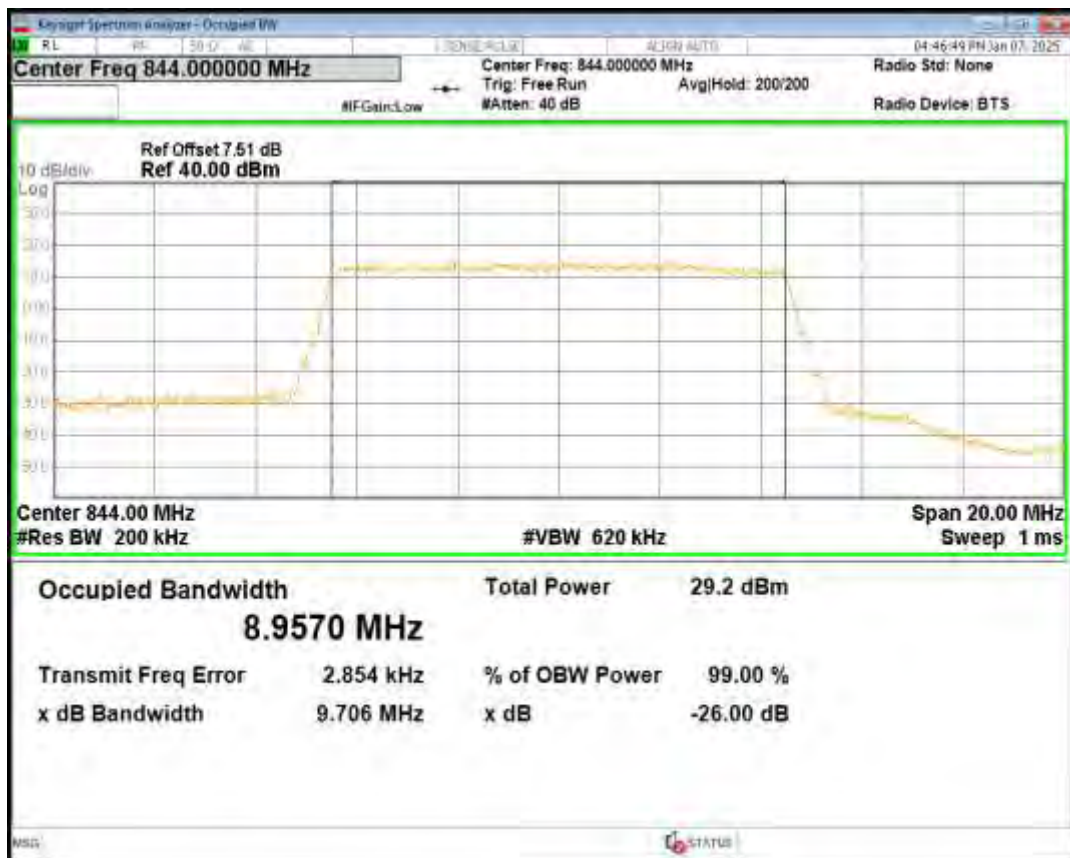
Band5 16QAM BW=3MHz Channel=20415 RB Size=15 Position=#0
