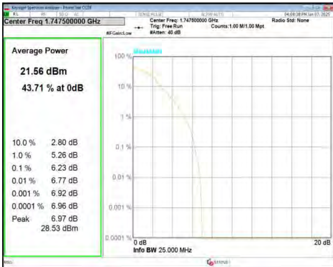
Band4 16QAM BW=20MHz Channel=20050 RB Size=1 Position=#0
