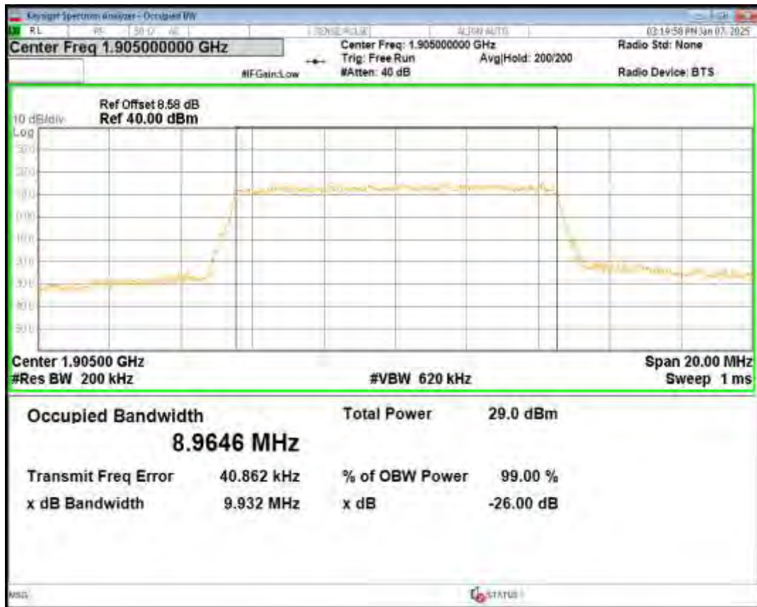
Band2 QPSK BW=10MHz Channel=18900 RB Size=50 Position=#0
