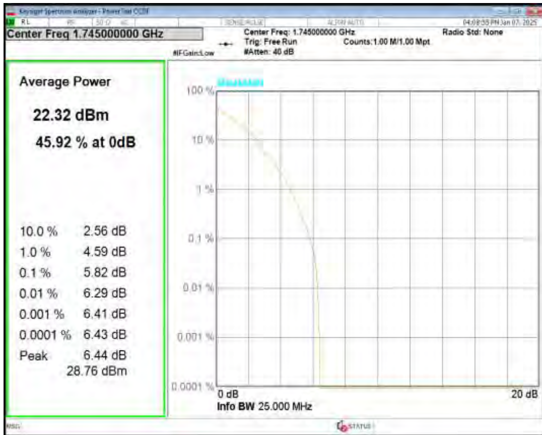
Band4 QPSK BW=20MHz Channel=20175 RB Size=1 Position=#0
