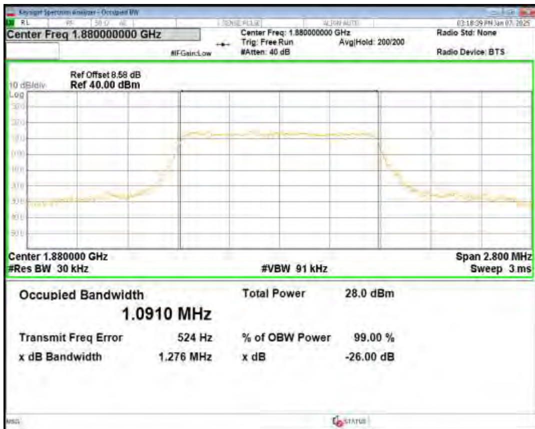
Band2 16QAM BW=1.4MHz Channel=19193 RB Size=6 Position=#0
