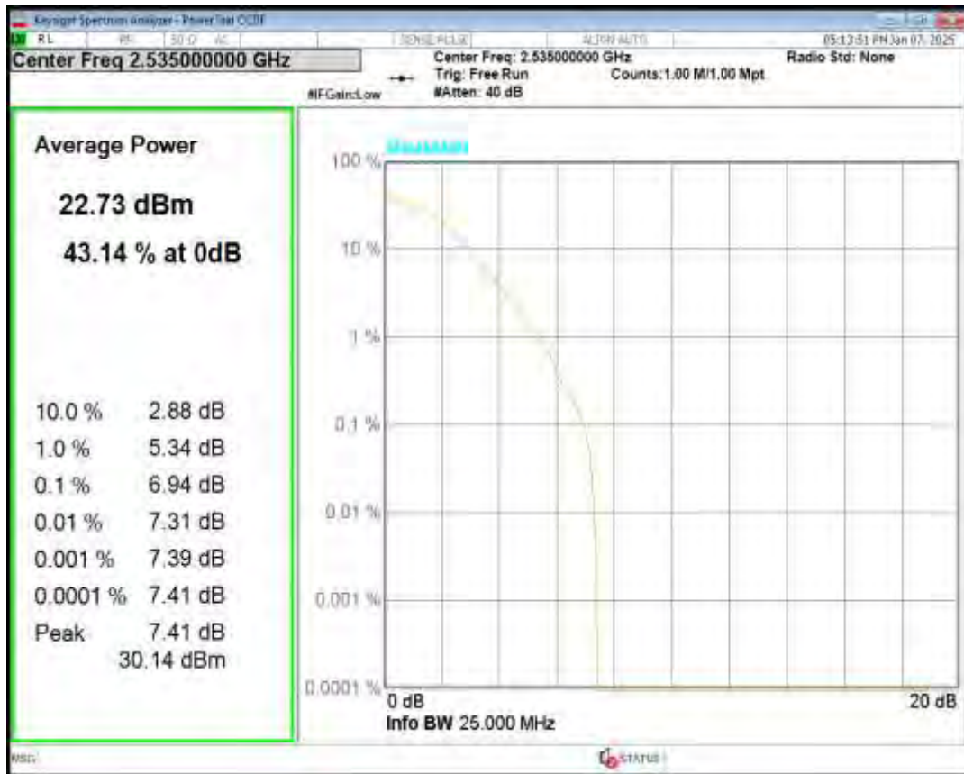
Band7 16QAM BW=10MHz Channel=21400 RB Size=1 Position=#0
