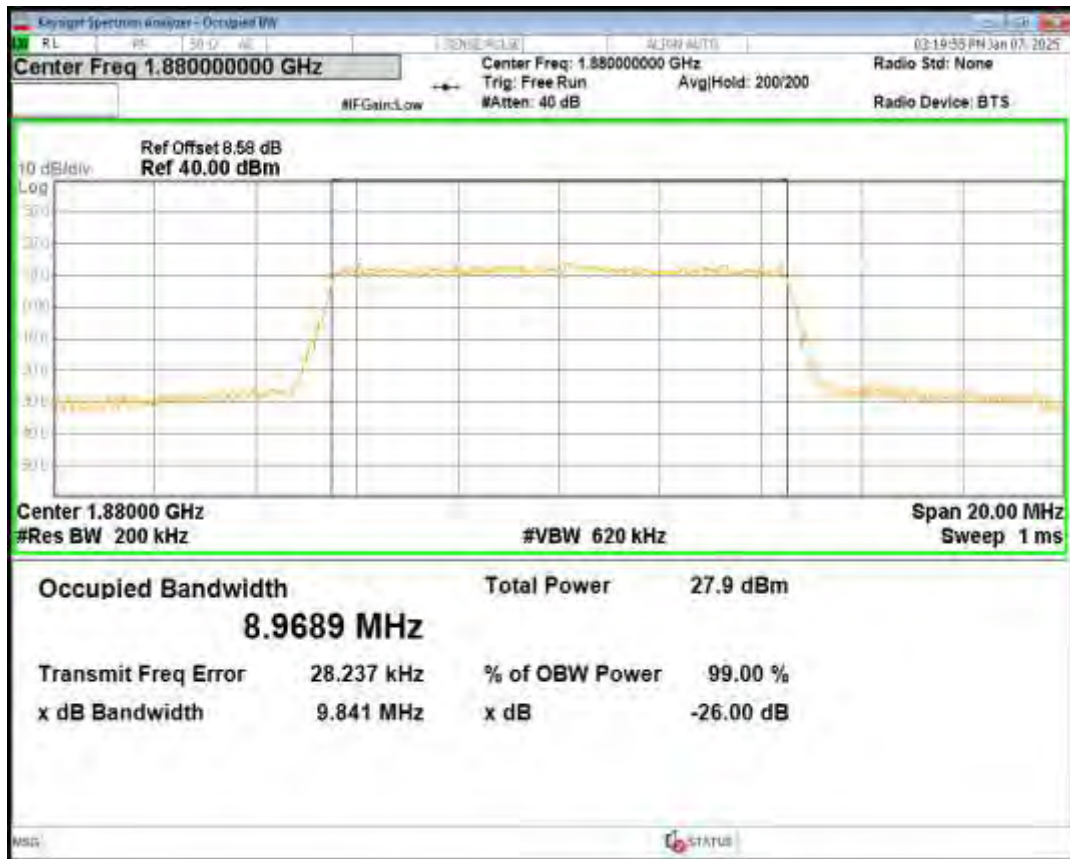
Band2 16QAM BW=10MHz Channel=19150 RB Size=50 Position=#0
