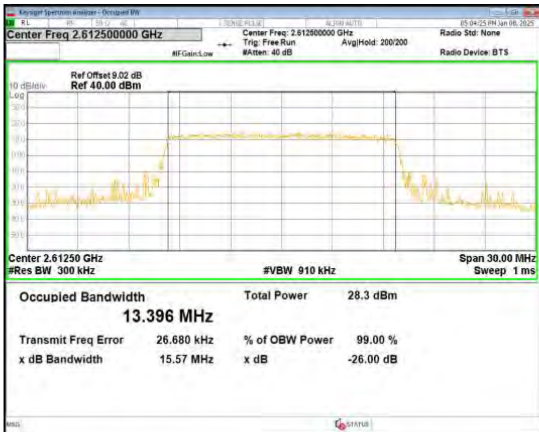
Band38 QPSK BW=20MHz Channel=37850 RB Size=100 Position=#0
