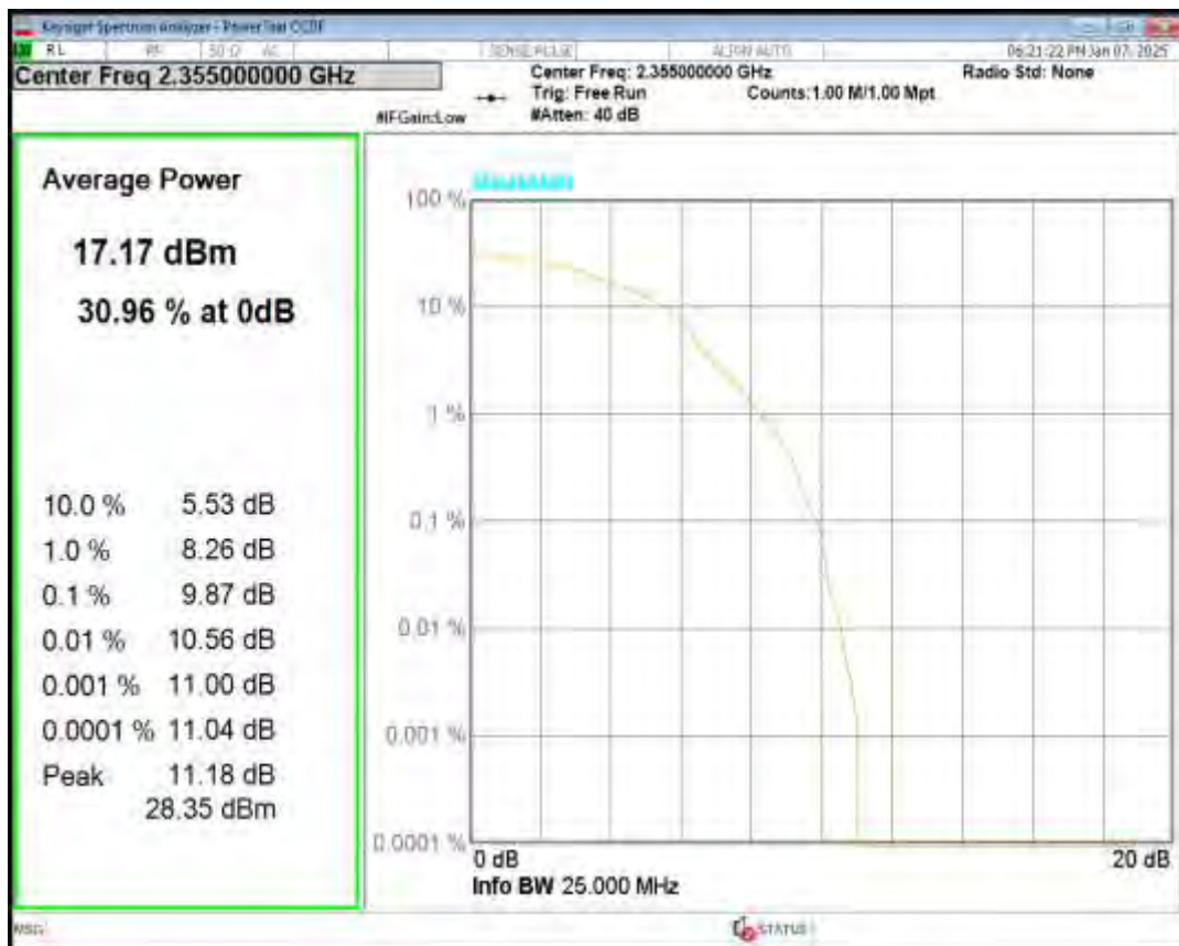
Band40(2350-2360) 16QAM BW=5MHz Channel=39175 RB Size=1 Position=#0
