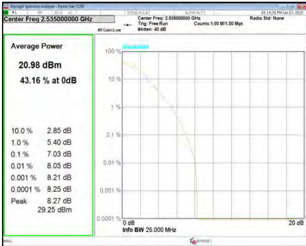
Band7 QPSK BW=10MHz Channel=20800 RB Size=1 Position=#0
