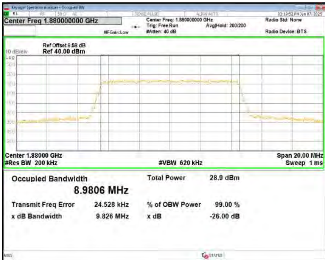
Band2 QPSK BW=15MHz Channel=18900 RB Size=75 Position=#0
