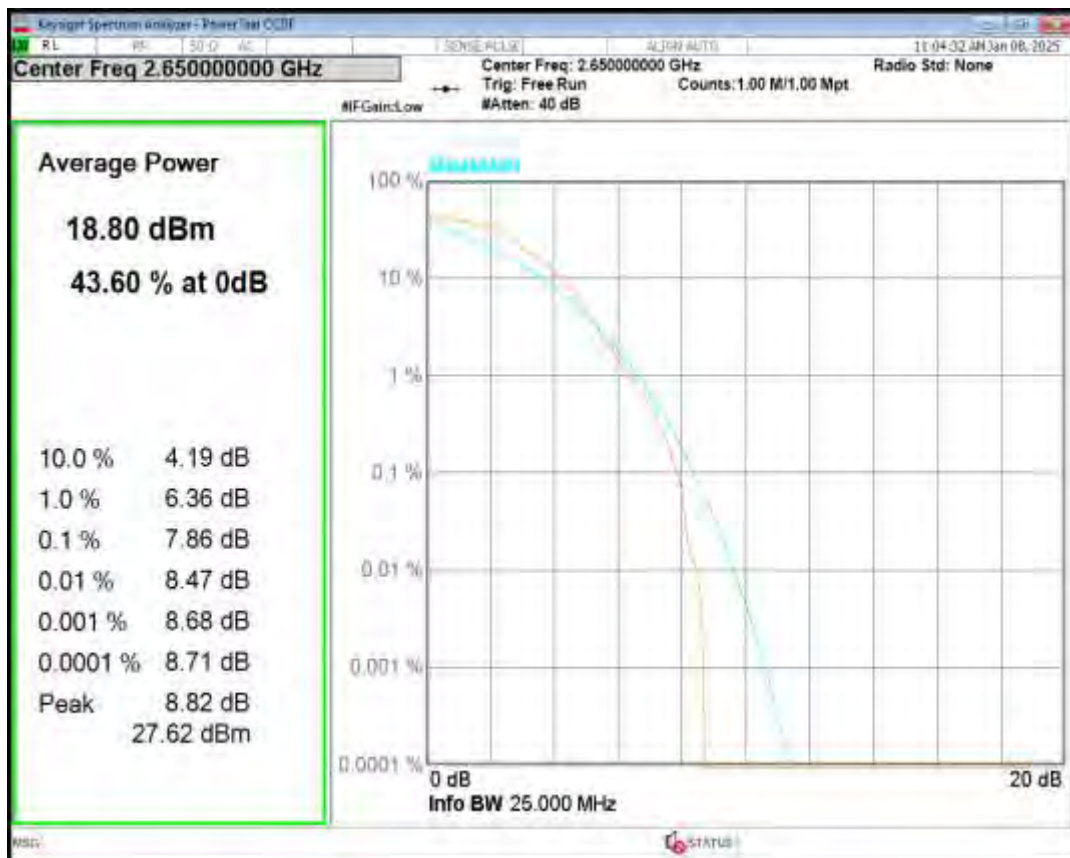
Band41(2555-2655) QPSK BW=15MHz Channel=40315 RB Size=1 Position=#0
