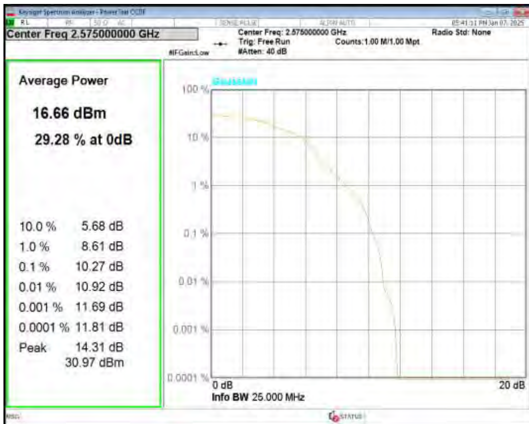
Band38 16QAM BW=10MHz Channel=38000 RB Size=1 Position=#0
