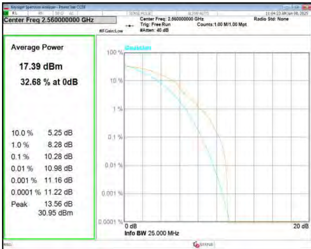
Band41(2555-2655) 16QAM BW=10MHz Channel=40740 RB Size=1 Position=#0
