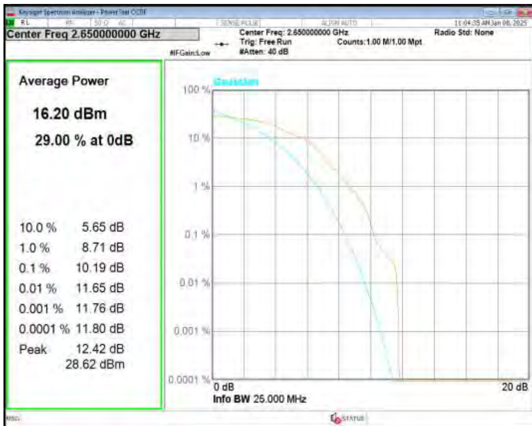
Band41(2555-2655) 16QAM BW=15MHz Channel=40315 RB Size=1 Position=#0
