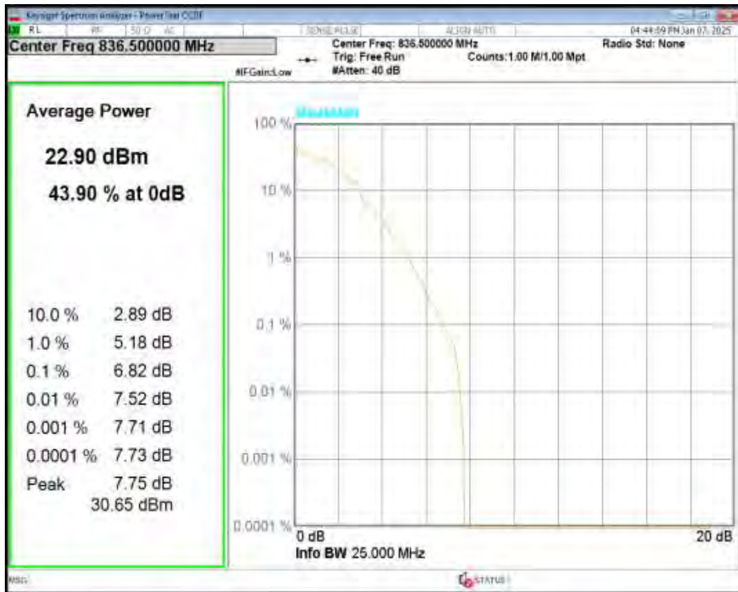
Band5 16QAM BW=1.4MHz Channel=20643 RB Size=1 Position=#0
