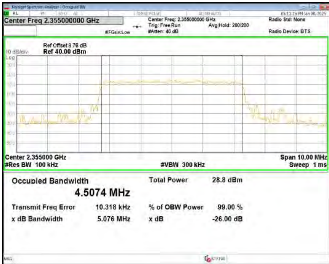
Band40(2350-2360) QPSK BW=5MHz Channel=39225 RB Size=25 Position=#0
