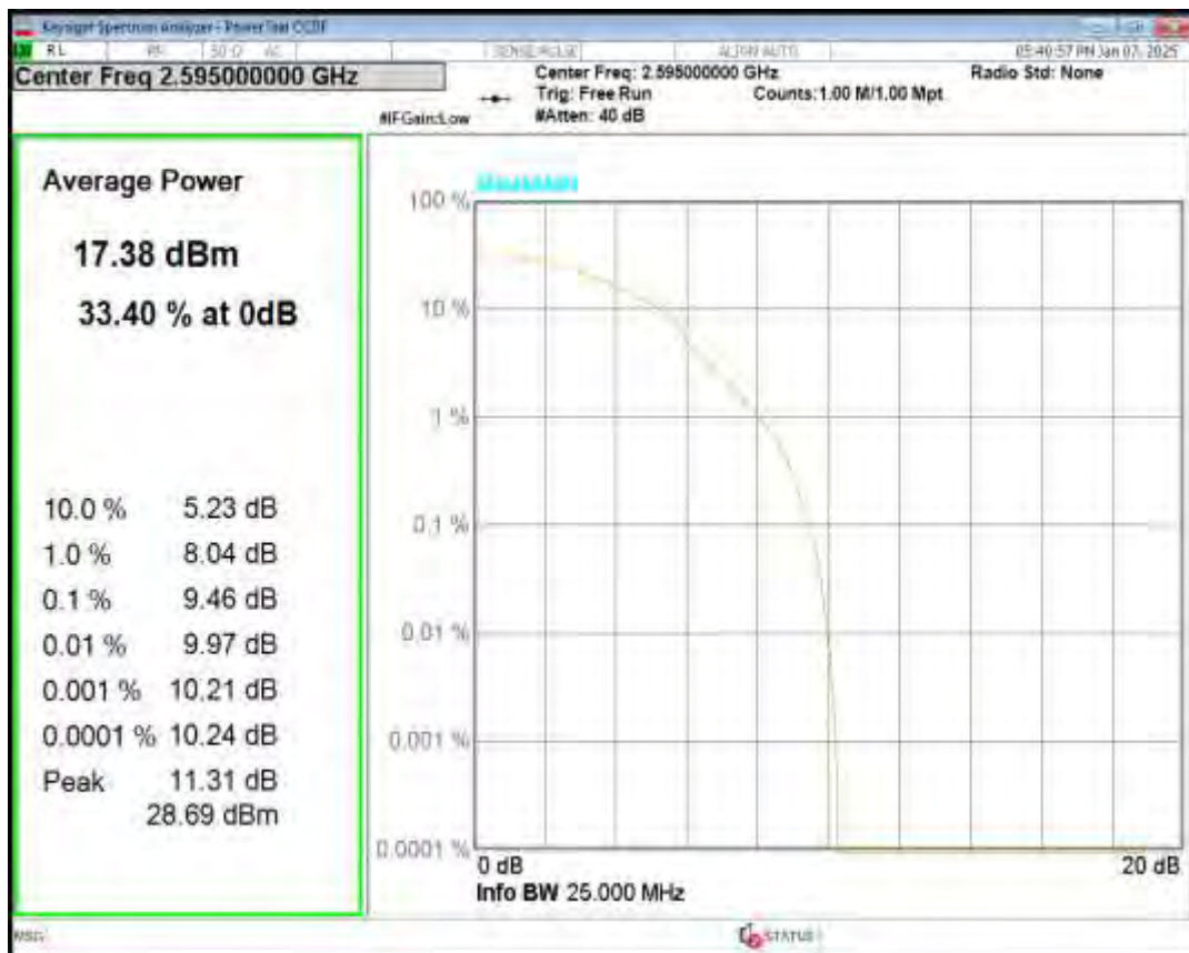
Band38 16QAM BW=5MHz Channel=38225 RB Size=1 Position=#0
