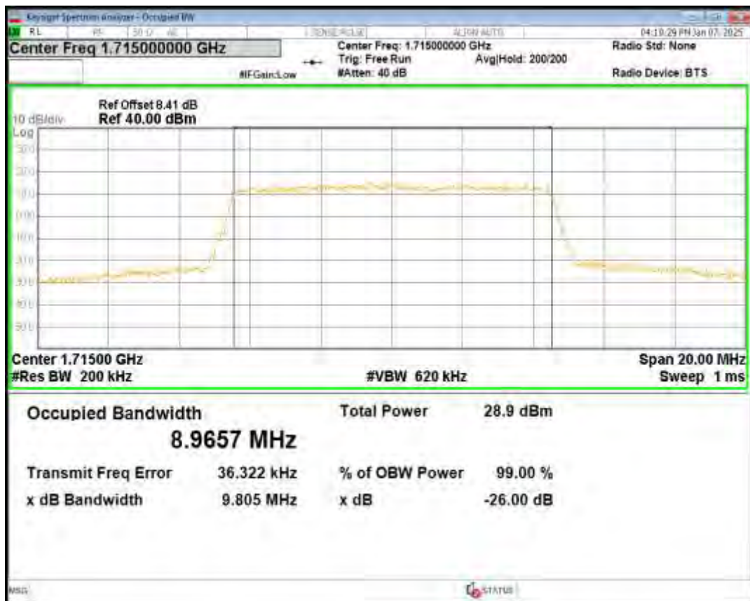
Band4 QPSK BW=10MHz Channel=20175 RB Size=50 Position=#0
