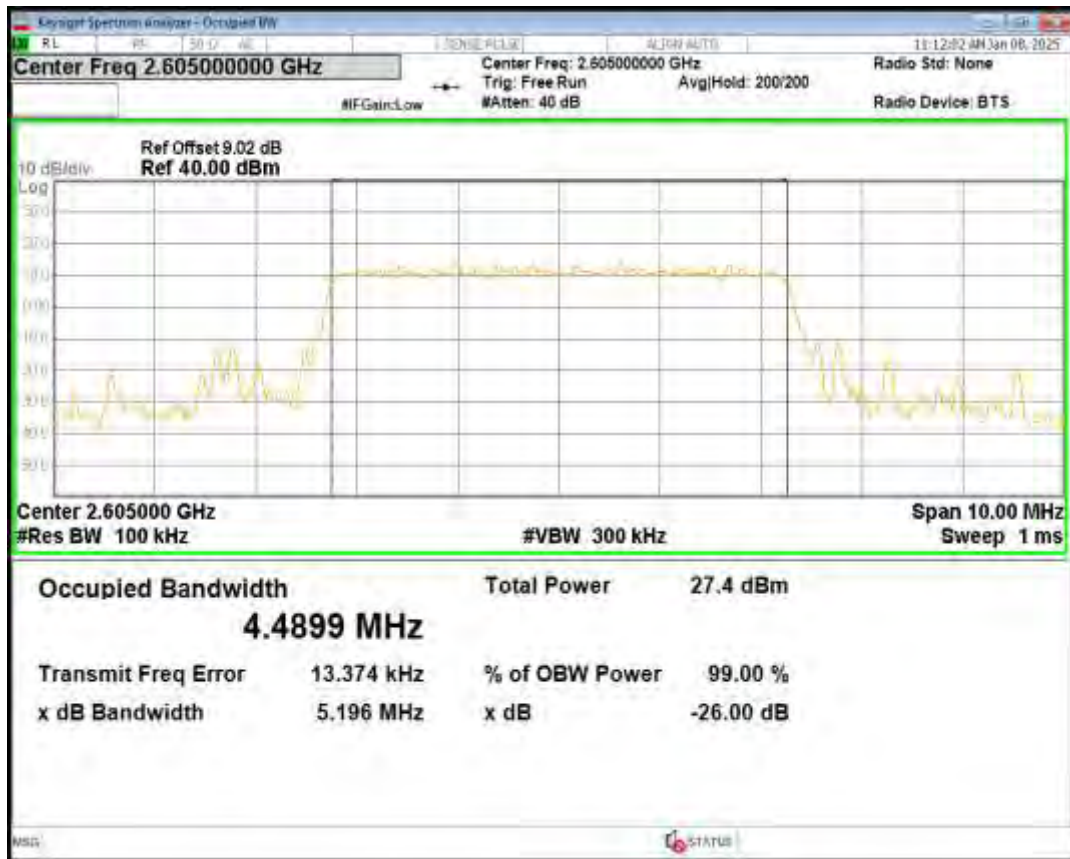
Band41(2555-2655) 16QAM BW=5MHz Channel=41215 RB Size=25 Position=#0
