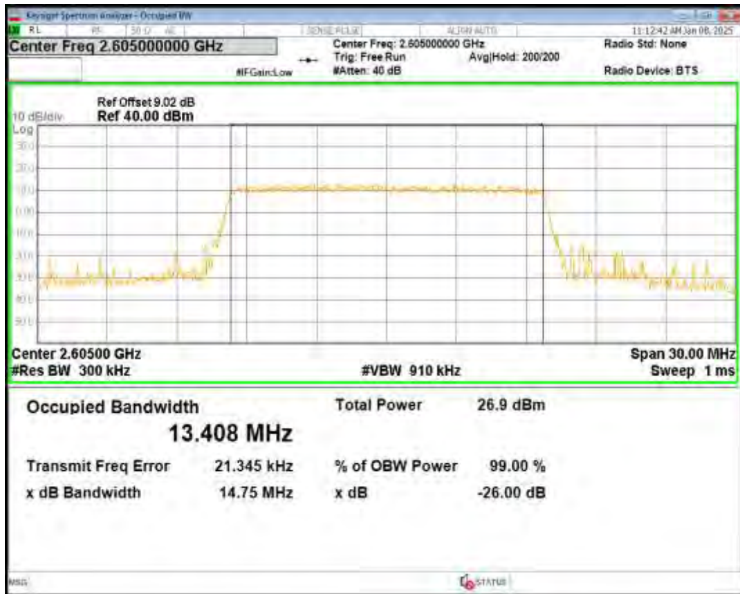
Band41(2555-2655) 16QAM BW=15MHz Channel=41165 RB Size=75 Position=#0
