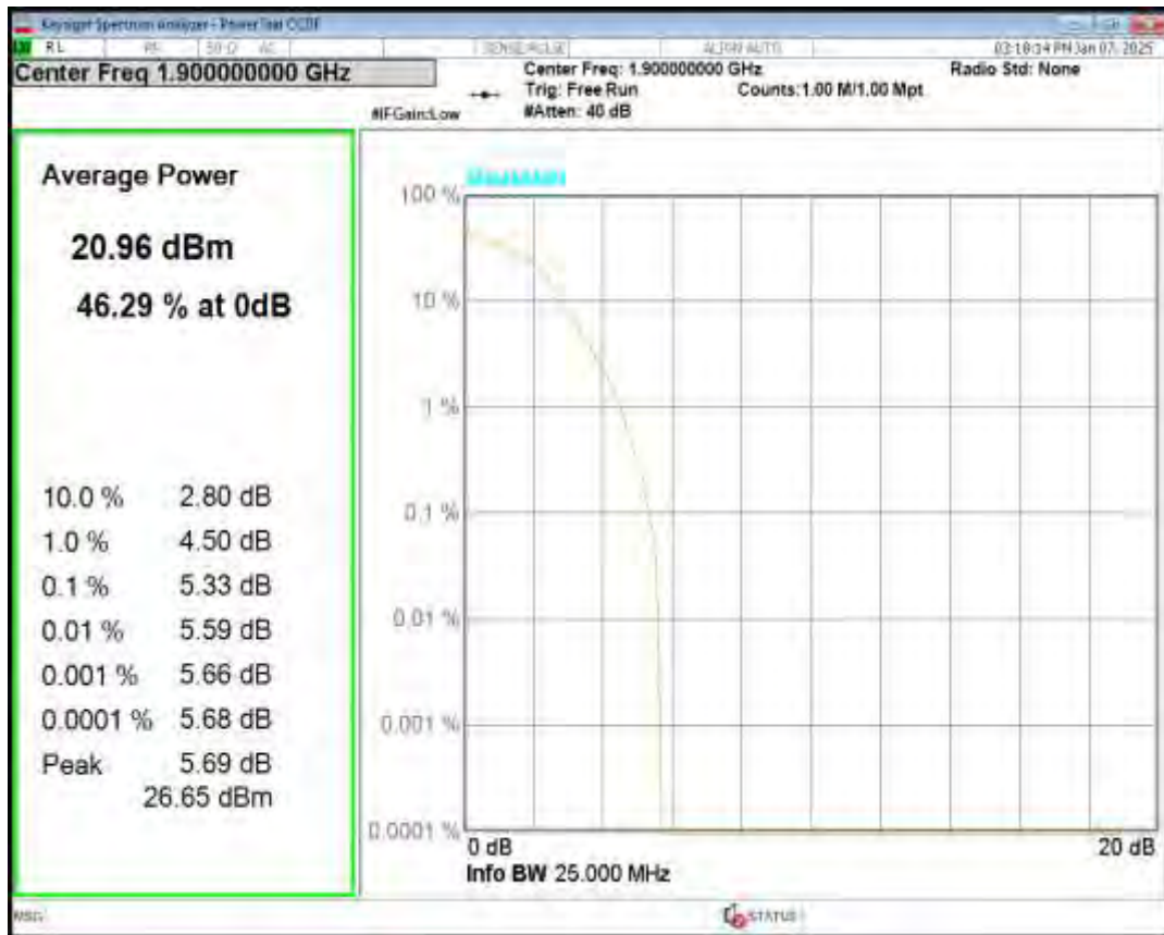
Band2 16QAM BW=20MHz Channel=18700 RB Size=1 Position=#0
