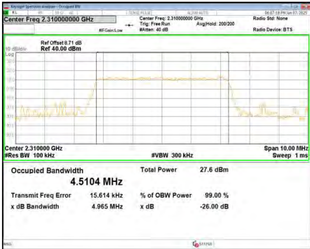
Band40(2305-2315) 16QAM BW=5MHz Channel=38775 RB Size=25 Position=#0
