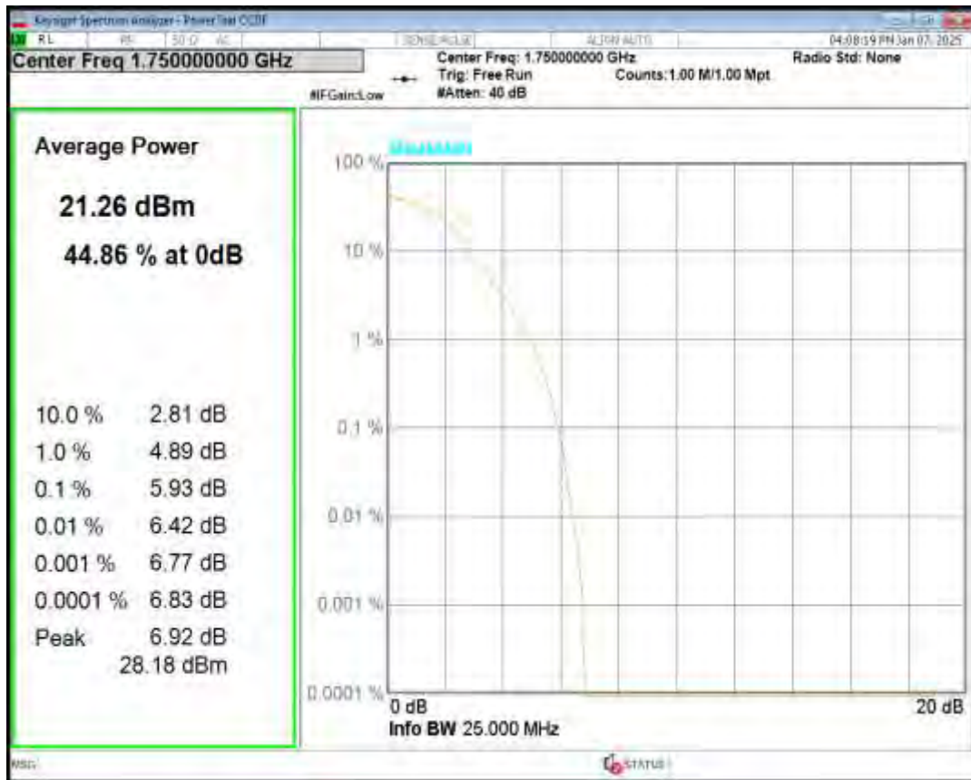
Band4 16QAM BW=15MHz Channel=20025 RB Size=1 Position=#0
