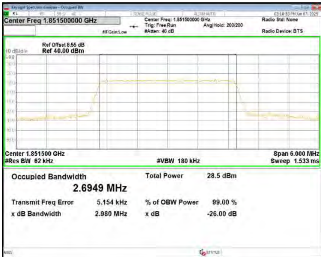
Band2 16QAM BW=20MHz Channel=19100 RB Size=100 Position=#0
