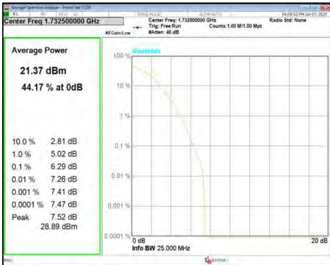
Band4 16QAM BW=20MHz Channel=20300 RB Size=1 Position=#0
