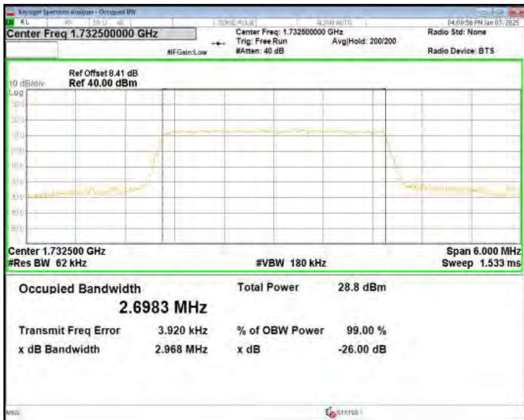
Band4 16QAM BW=3MHz Channel=20385 RB Size=15 Position=#0
