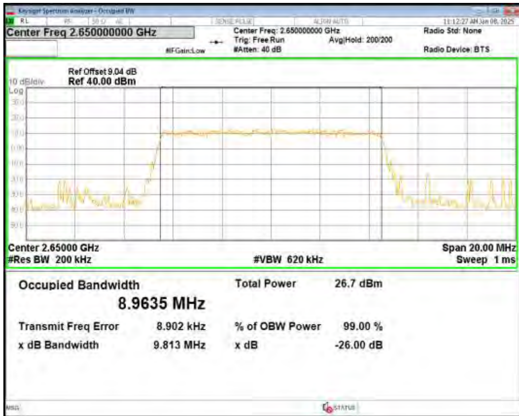
Band41(2555-2655) 16QAM BW=15MHz Channel=40315 RB Size=75 Position=#0
