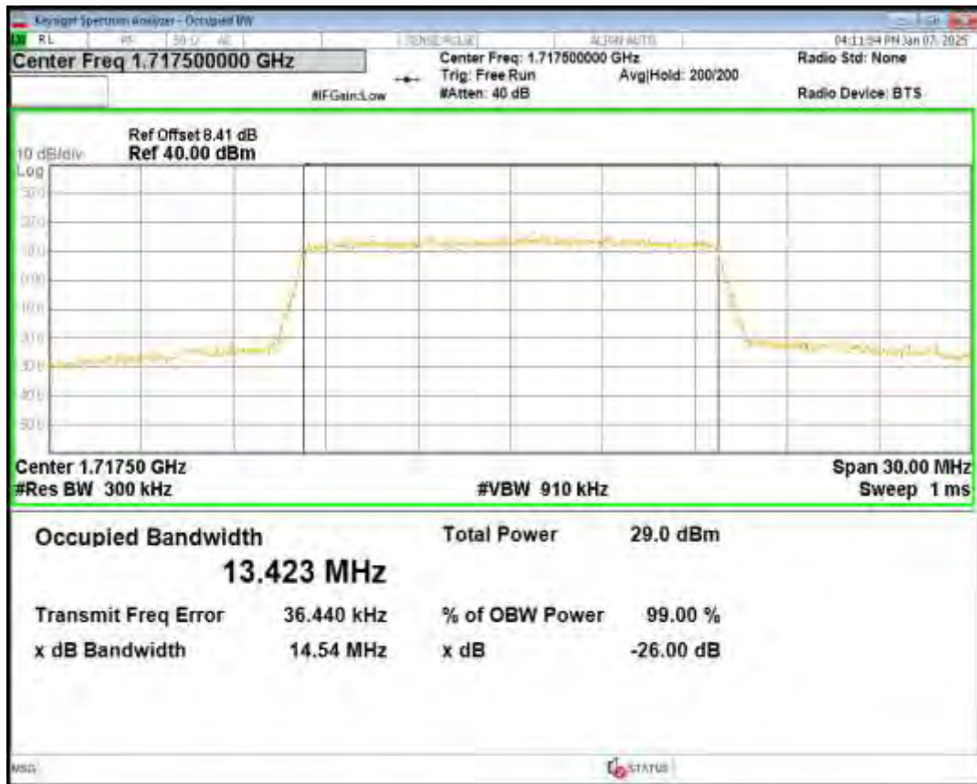
Band4 QPSK BW=15MHz Channel=20175 RB Size=75 Position=#0
