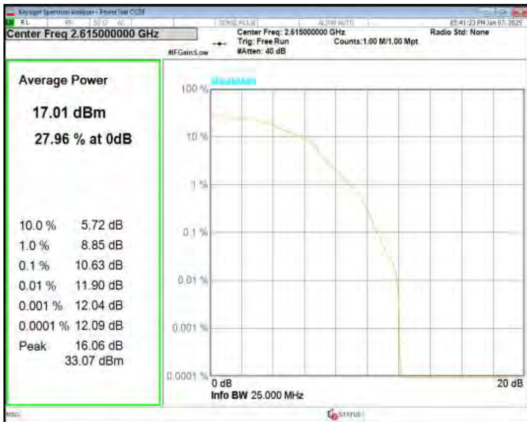
Band38 16QAM BW=15MHz Channel=37825 RB Size=1 Position=#0
