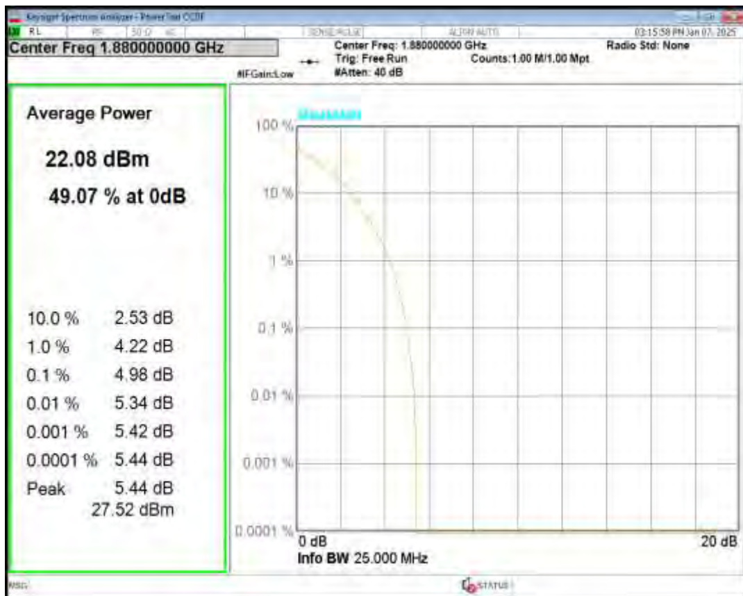
Band2 16QAM BW=5MHz Channel=19175 RB Size=1 Position=#0
