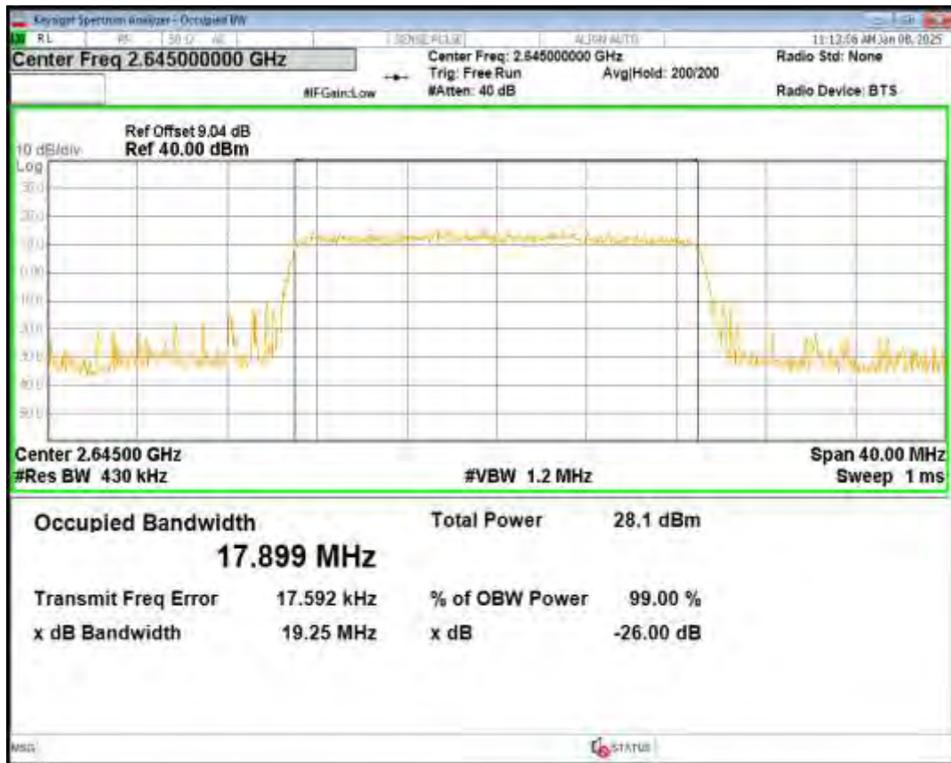
Band41(2555-2655) QPSK BW=5MHz Channel=40265 RB Size=25 Position=#0
