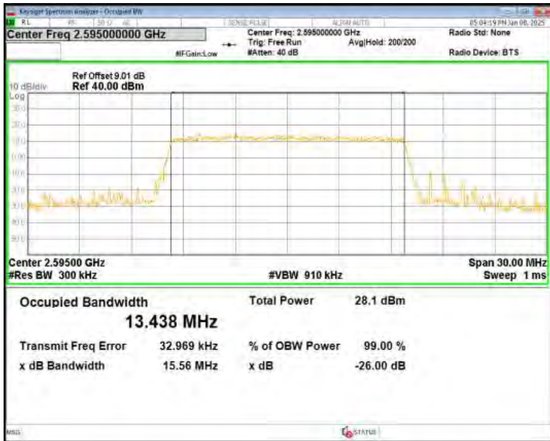
Band38 QPSK BW=15MHz Channel=38175 RB Size=75 Position=#0
