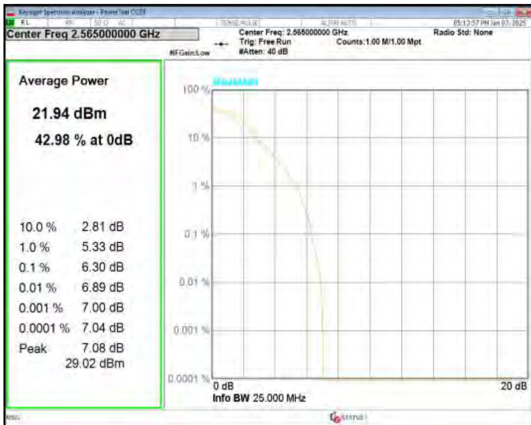
Band7 16QAM BW=15MHz Channel=20825 RB Size=1 Position=#0
