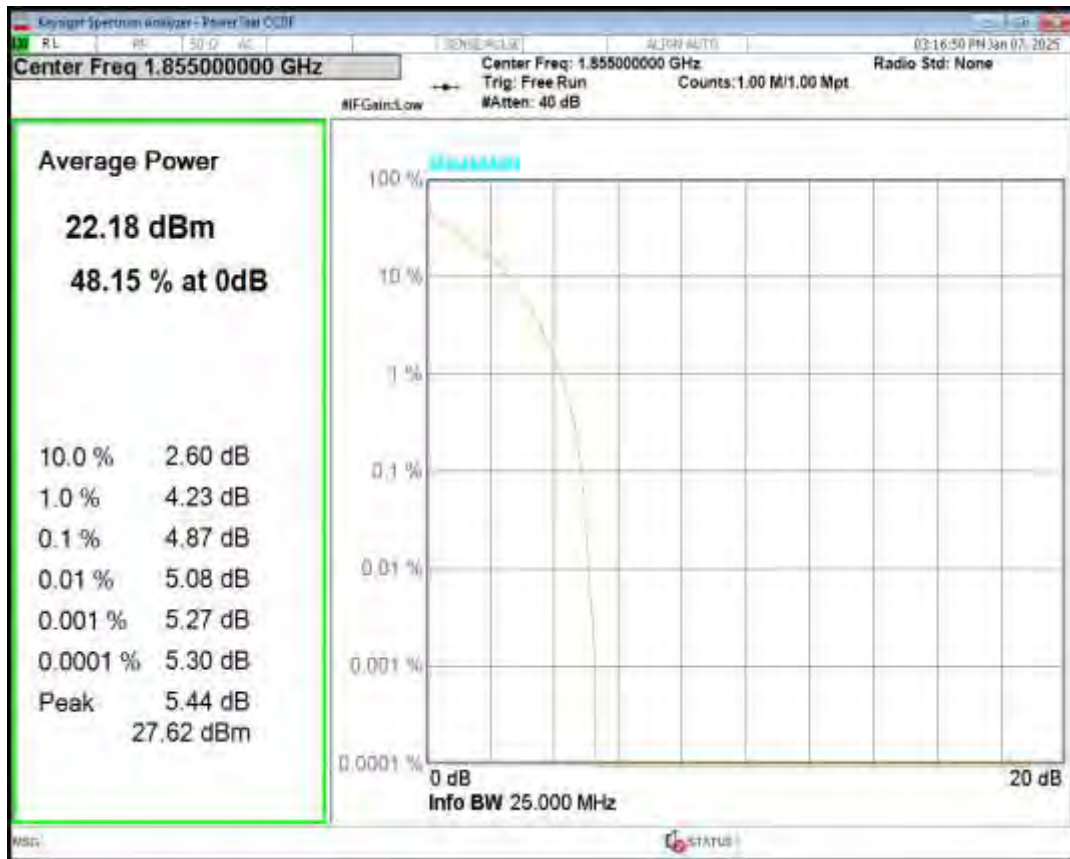
Band2 QPSK BW=1.4MHz Channel=18900 RB Size=1 Position=#0
