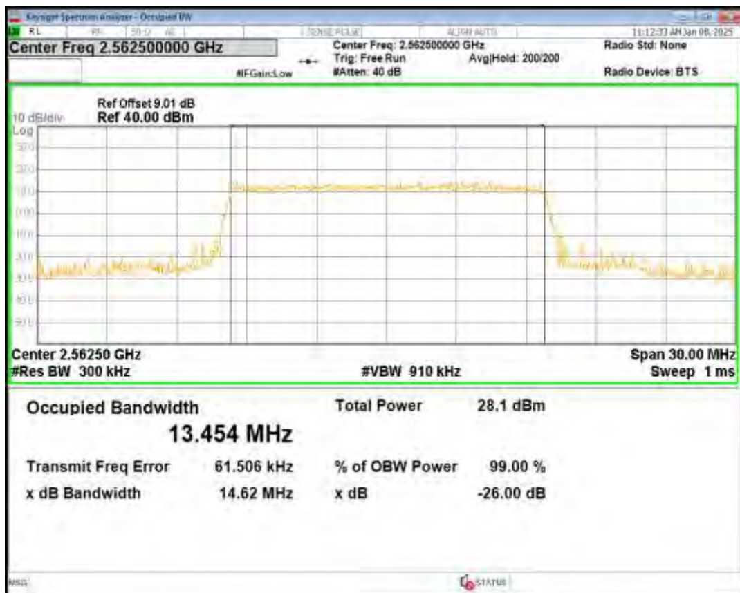
Band41(2555-2655) QPSK BW=15MHz Channel=40740 RB Size=75 Position=#0
