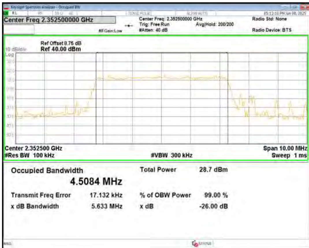
Band40(2350-2360) QPSK BW=5MHz Channel=39200 RB Size=25 Position=#0
