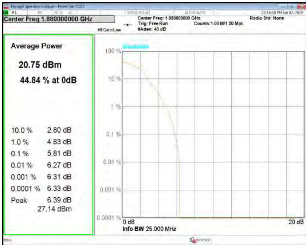
Band2 16QAM BW=1.4MHz Channel=19193 RB Size=1 Position=#0
