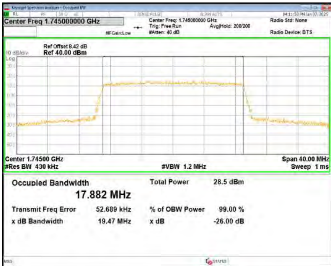
Band4 16QAM BW=3MHz Channel=19965 RB Size=15 Position=#0
