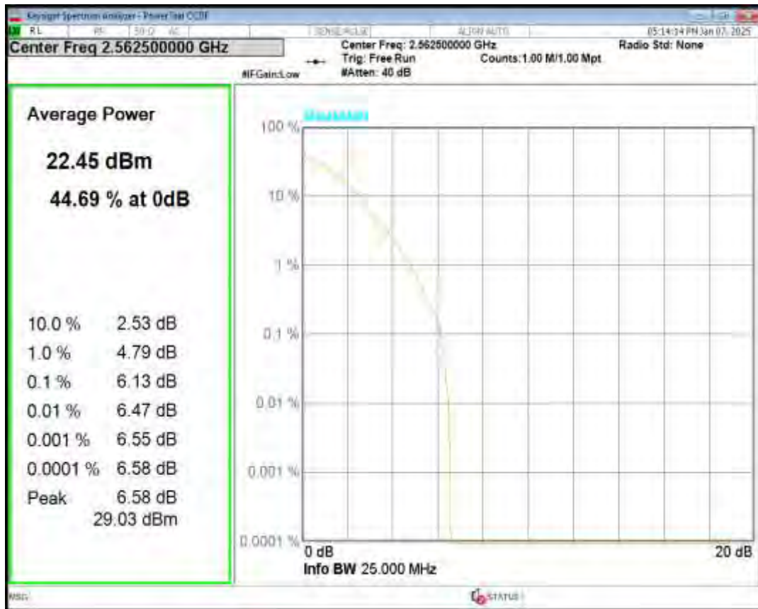
Band7 QPSK BW=20MHz Channel=20850 RB Size=1 Position=#0
