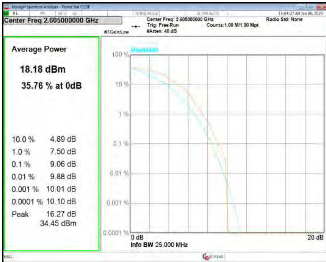
Band41(2555-2655) QPSK BW=10MHz Channel=41190 RB Size=1 Position=#0
