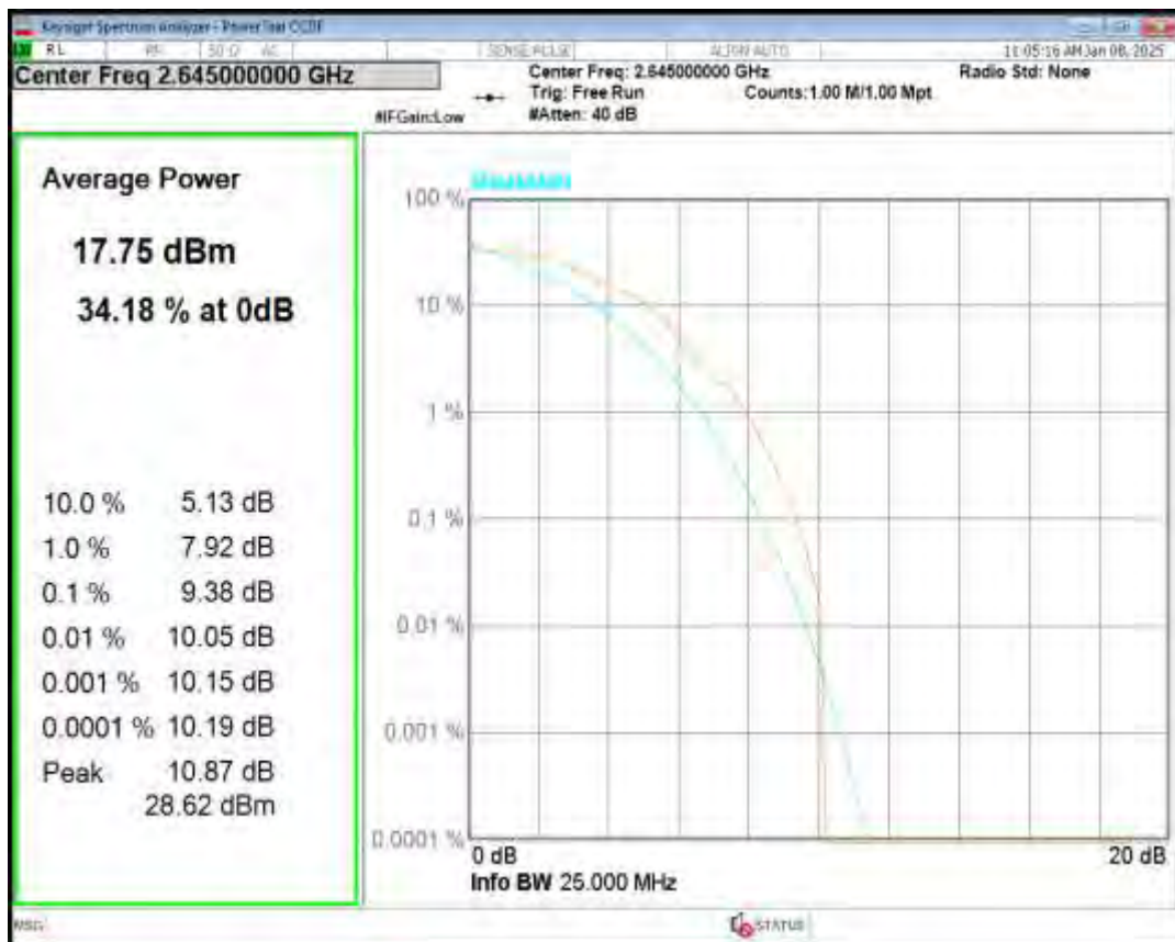
Band41(2555-2655) 16QAM BW=5MHz Channel=41215 RB Size=1 Position=#0
