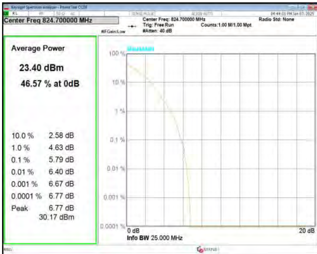
Band5 QPSK BW=1.4MHz Channel=20525 RB Size=1 Position=#0
