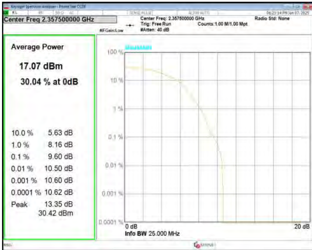
Band40(2350-2360) QPSK BW=10MHz Channel=39200 RB Size=1 Position=#0
