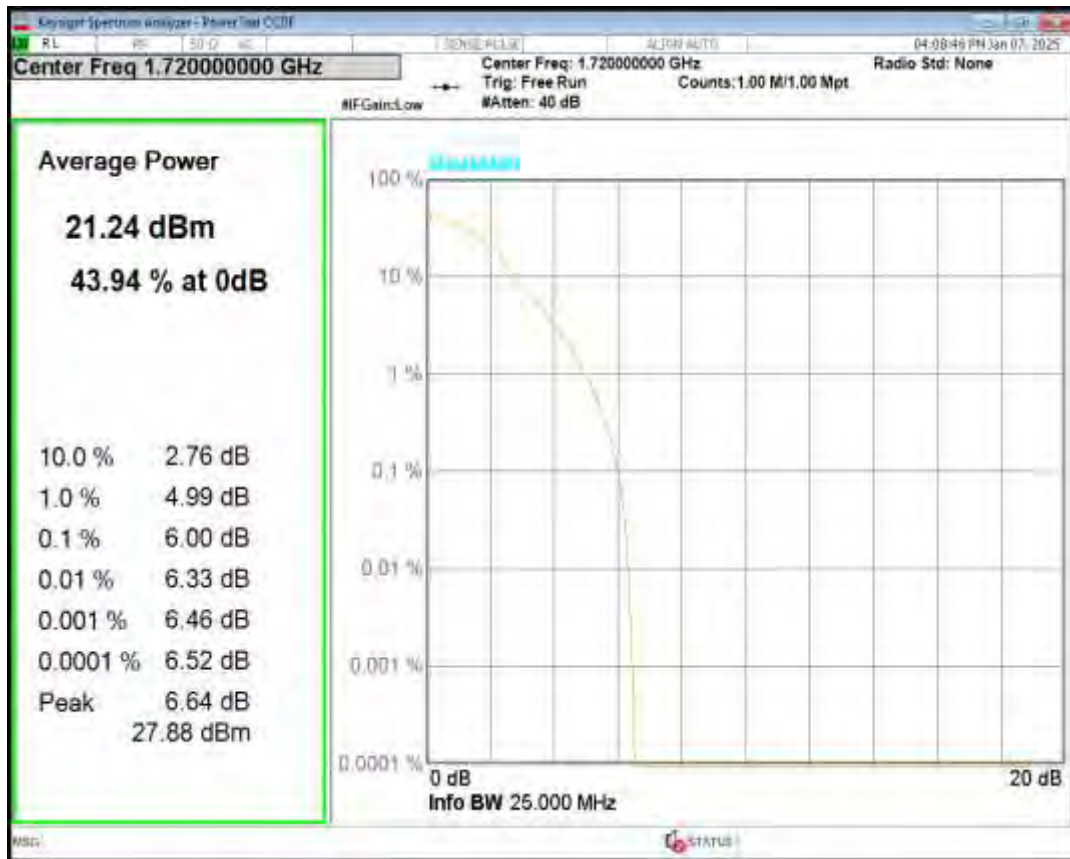
Band4 16QAM BW=20MHz Channel=20175 RB Size=1 Position=#0
