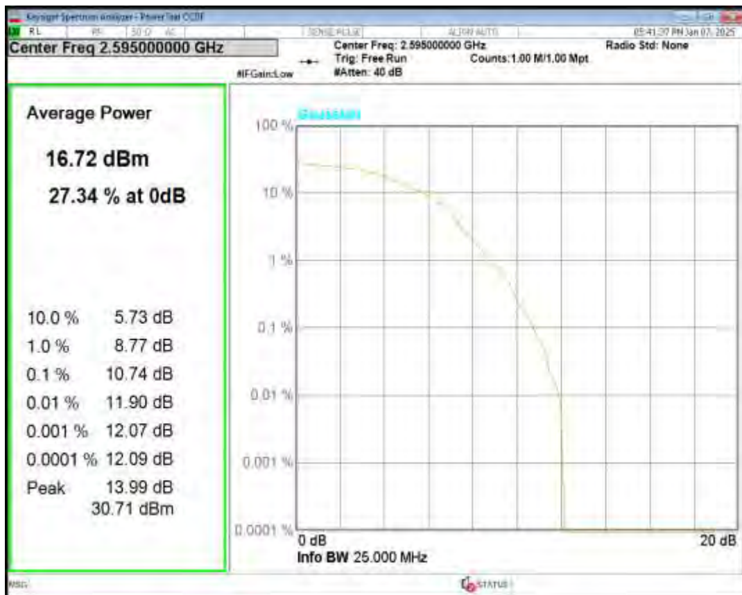
Band38 16QAM BW=15MHz Channel=38175 RB Size=1 Position=#0
