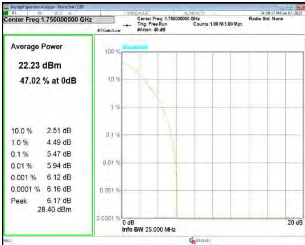
Band4 QPSK BW=20MHz Channel=20050 RB Size=1 Position=#0
