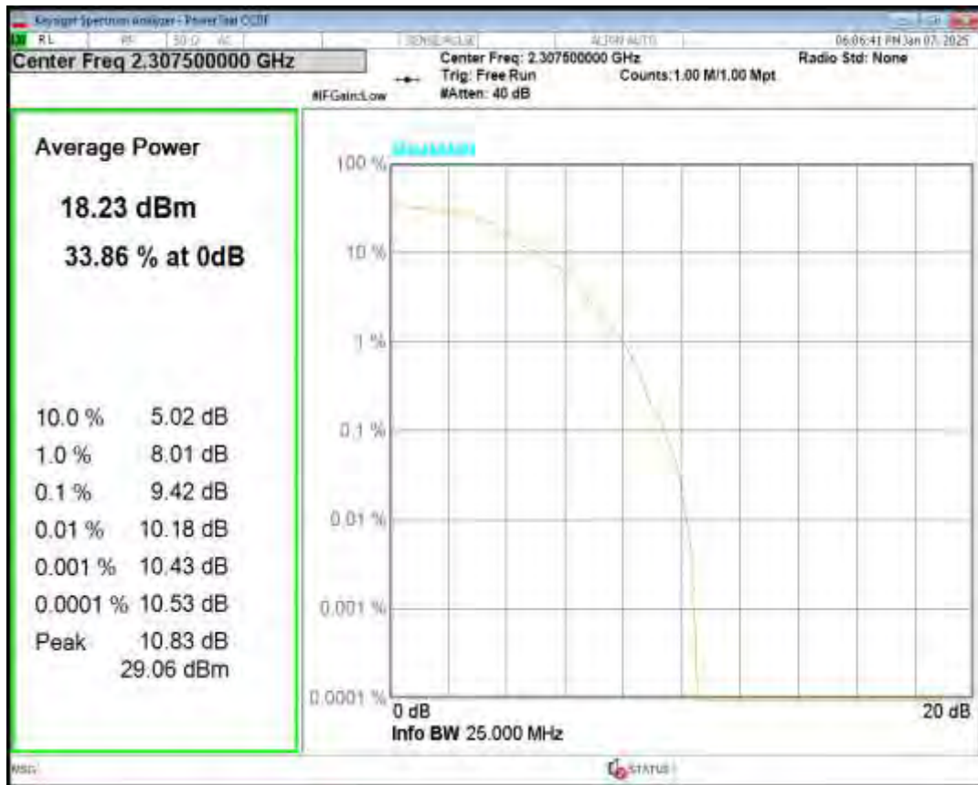
Band40(2305-2315) QPSK BW=5MHz Channel=38750 RB Size=1 Position=#0
