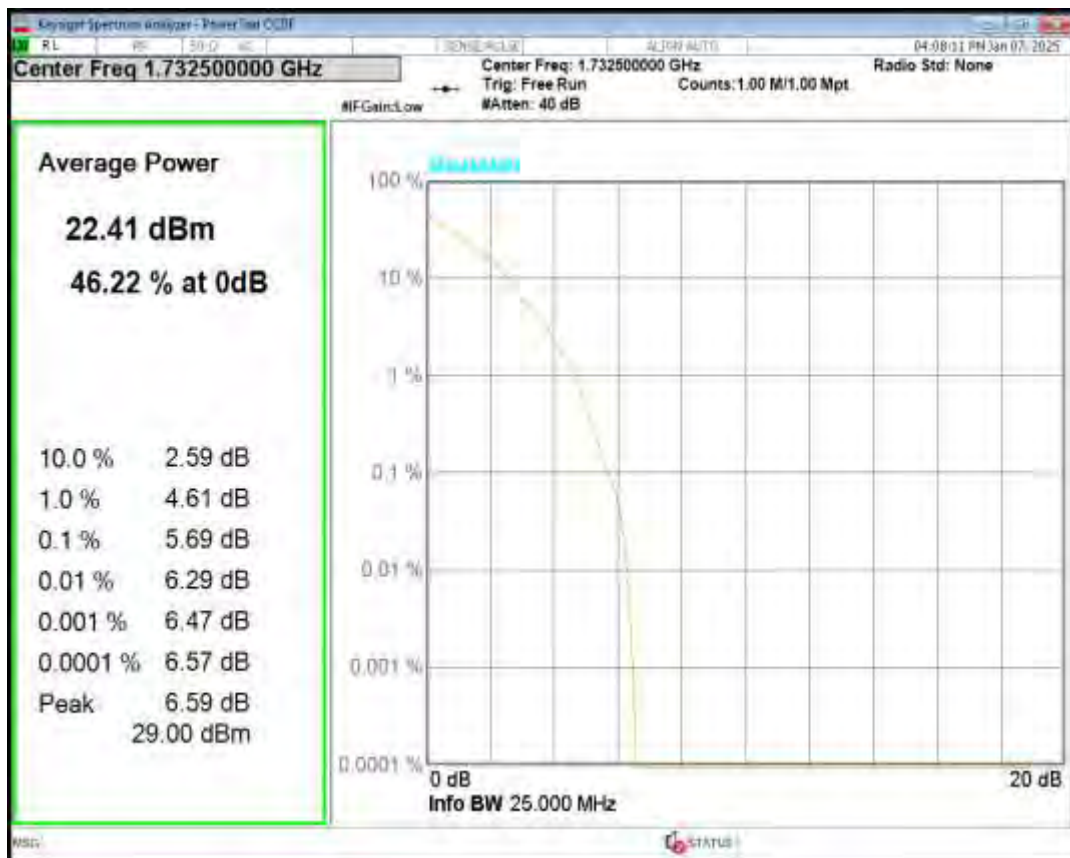
Band4 QPSK BW=3MHz Channel=20175 RB Size=1 Position=#0
