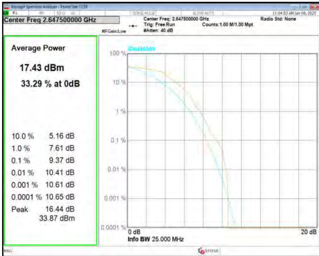
Band41(2555-2655) QPSK BW=20MHz Channel=40340 RB Size=1 Position=#0
