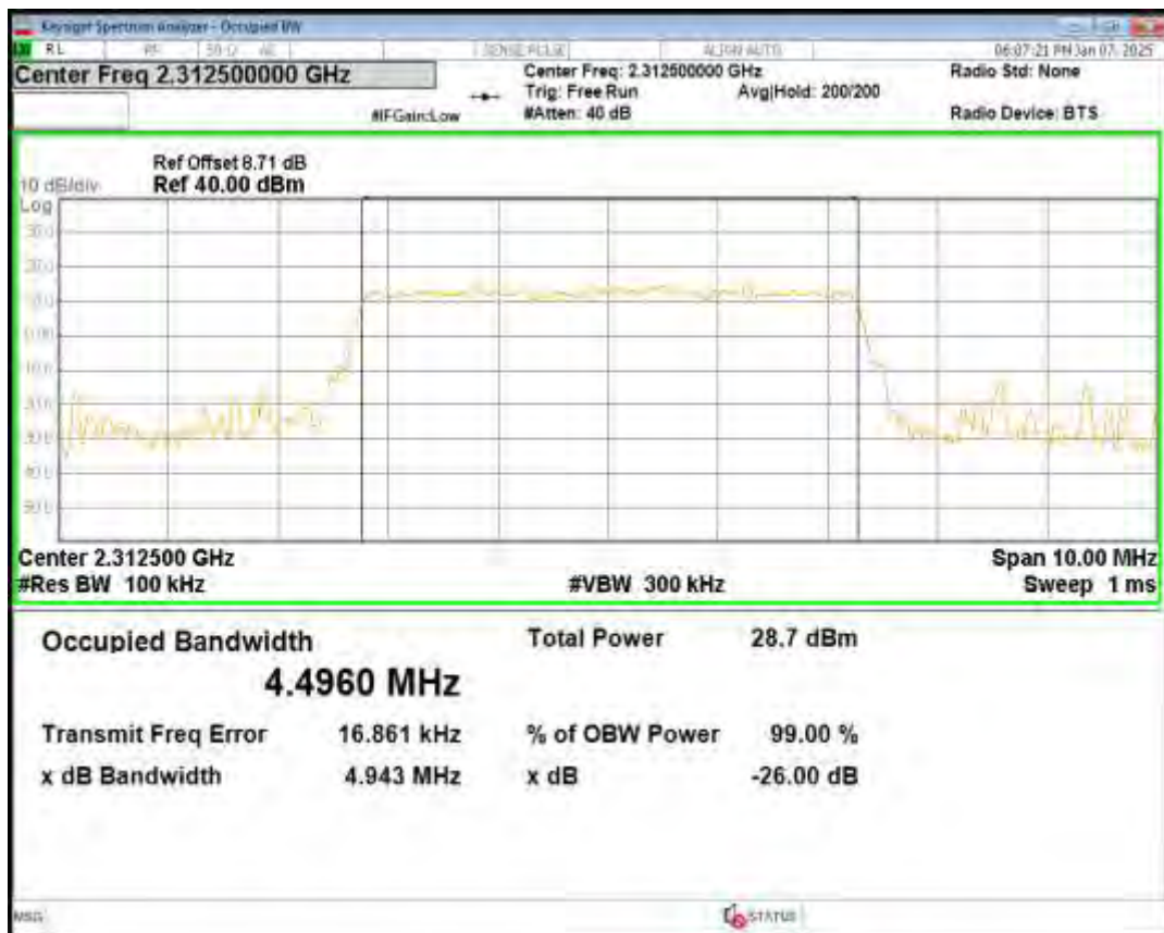
Band40(2350-2360) 16QAM BW=10MHz Channel=39200 RB Size=50 Position=#0
