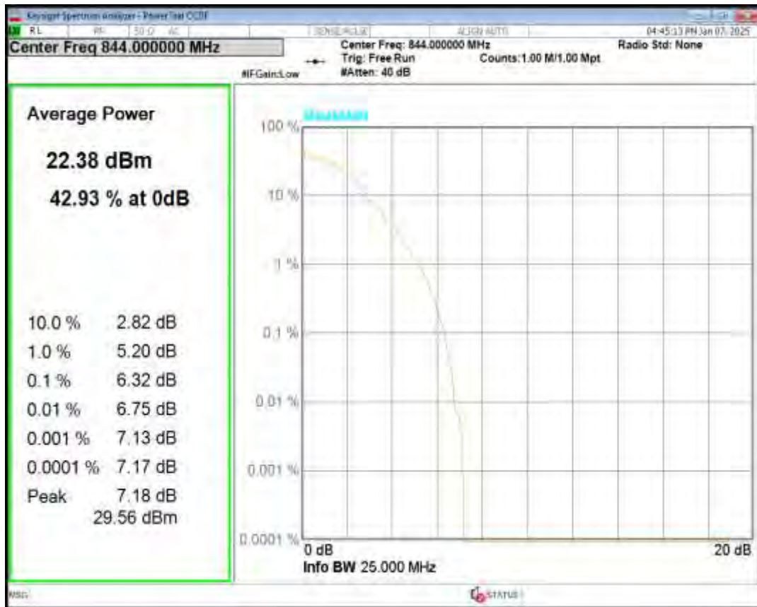
Band5 16QAM BW=10MHz Channel=20525 RB Size=1 Position=#0
