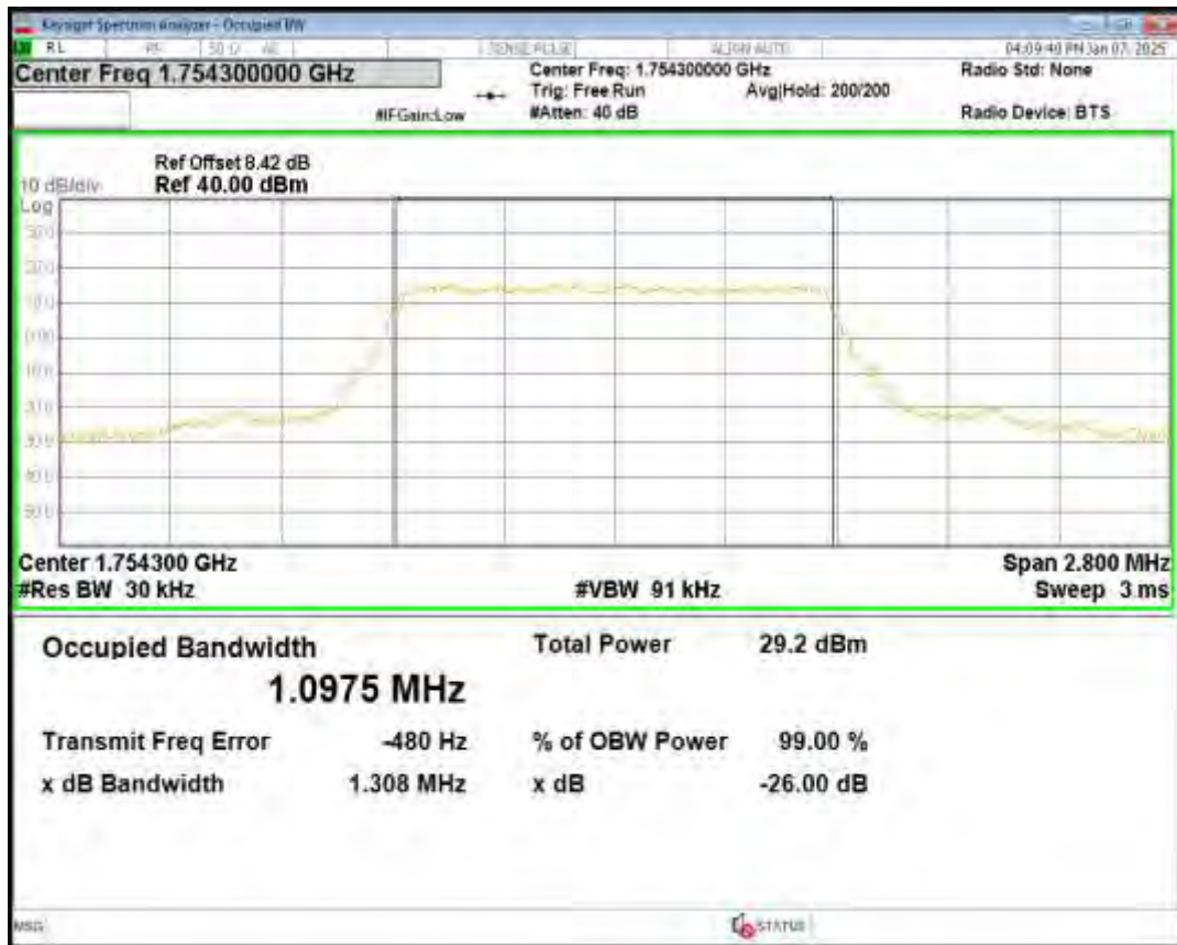
Band4 QPSK BW=10MHz Channel=20000 RB Size=50 Position=#0
