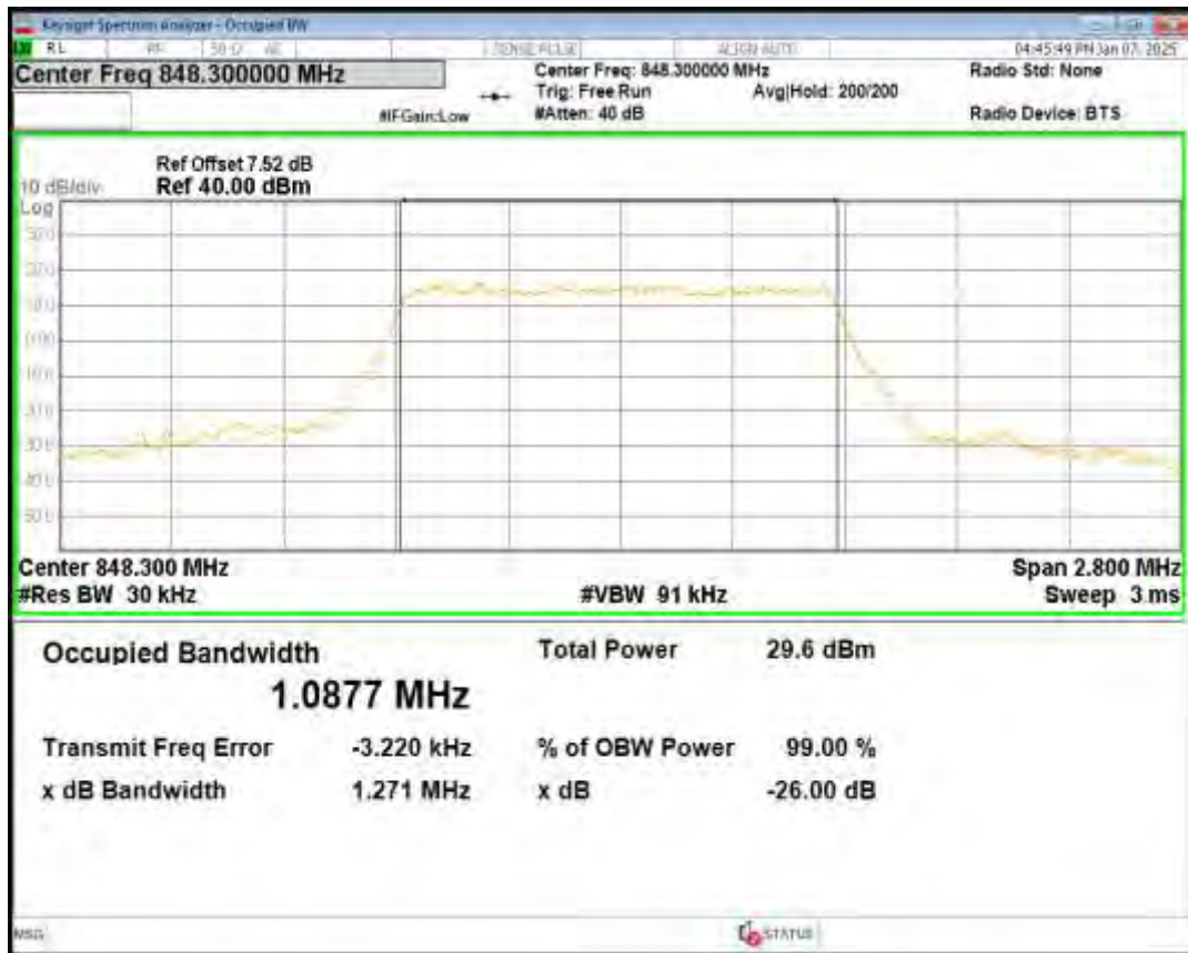
Band5 16QAM BW=10MHz Channel=20450 RB Size=50 Position=#0
