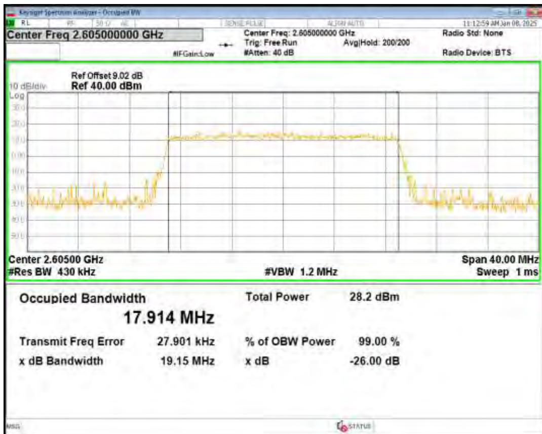
Band41(2555-2655) QPSK BW=20MHz Channel=41140 RB Size=100 Position=#0
