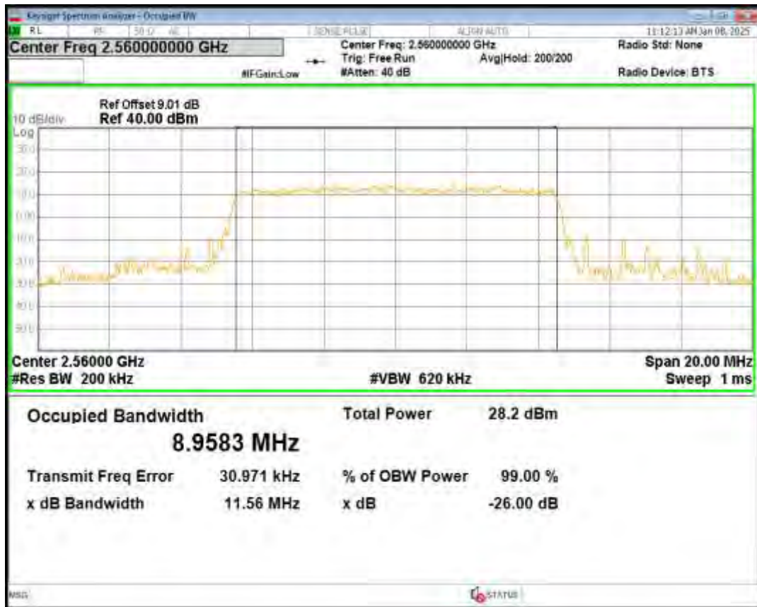
Band41(2555-2655) QPSK BW=10MHz Channel=40740 RB Size=50 Position=#0
