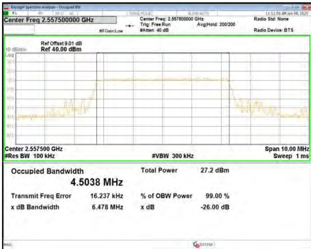
Band41(2555-2655) 16QAM BW=5MHz Channel=40740 RB Size=25 Position=#0
