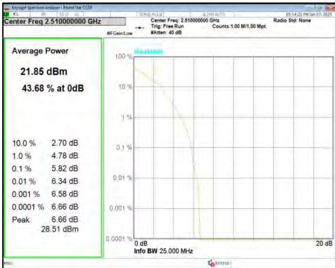
Band7 QPSK BW=20MHz Channel=21100 RB Size=1 Position=#0
