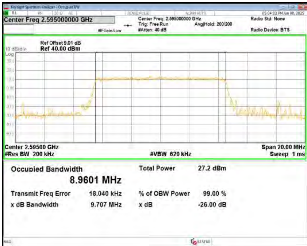
Band38 16QAM BW=10MHz Channel=38200 RB Size=50 Position=#0
