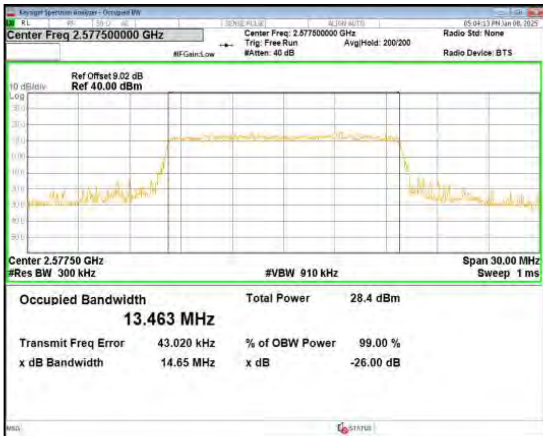
Band38 QPSK BW=15MHz Channel=38000 RB Size=75 Position=#0
