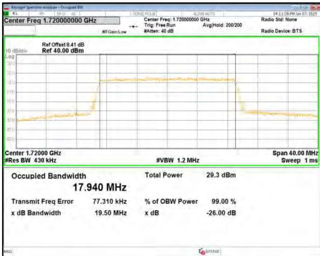
Band4 QPSK BW=20MHz Channel=20175 RB Size=100 Position=#0
