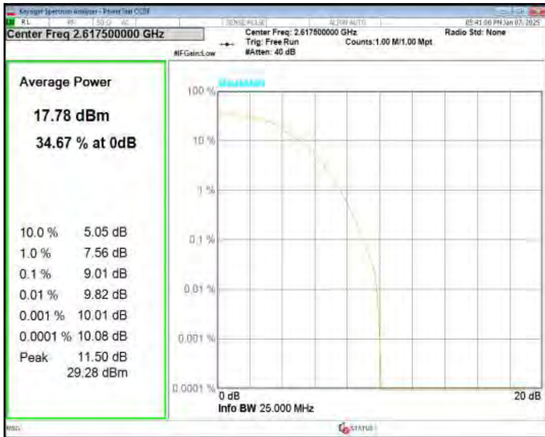
Band4 16QAM BW=1.4MHz Channel=19957 RB Size=1 Position=#0
