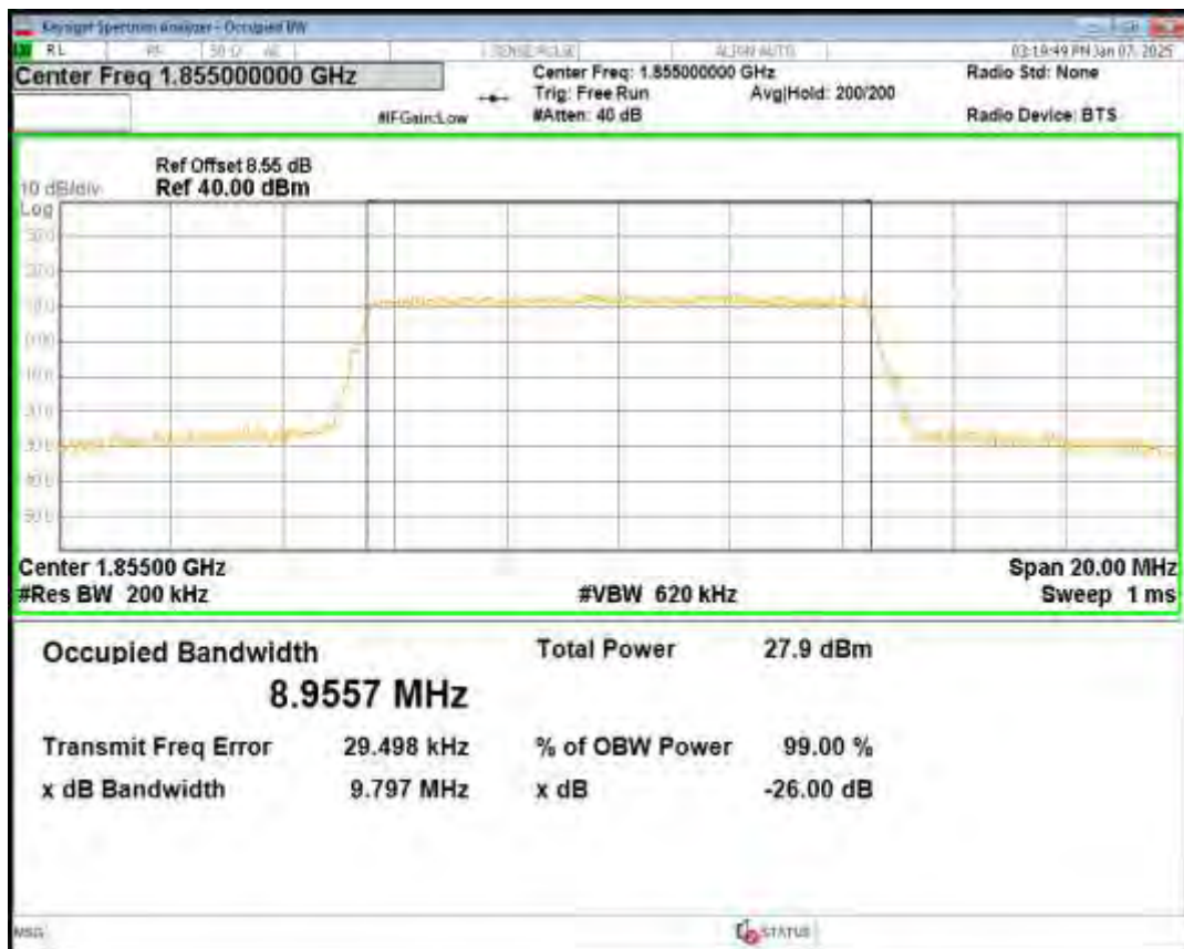
Band2 16QAM BW=10MHz Channel=18900 RB Size=50 Position=#0
