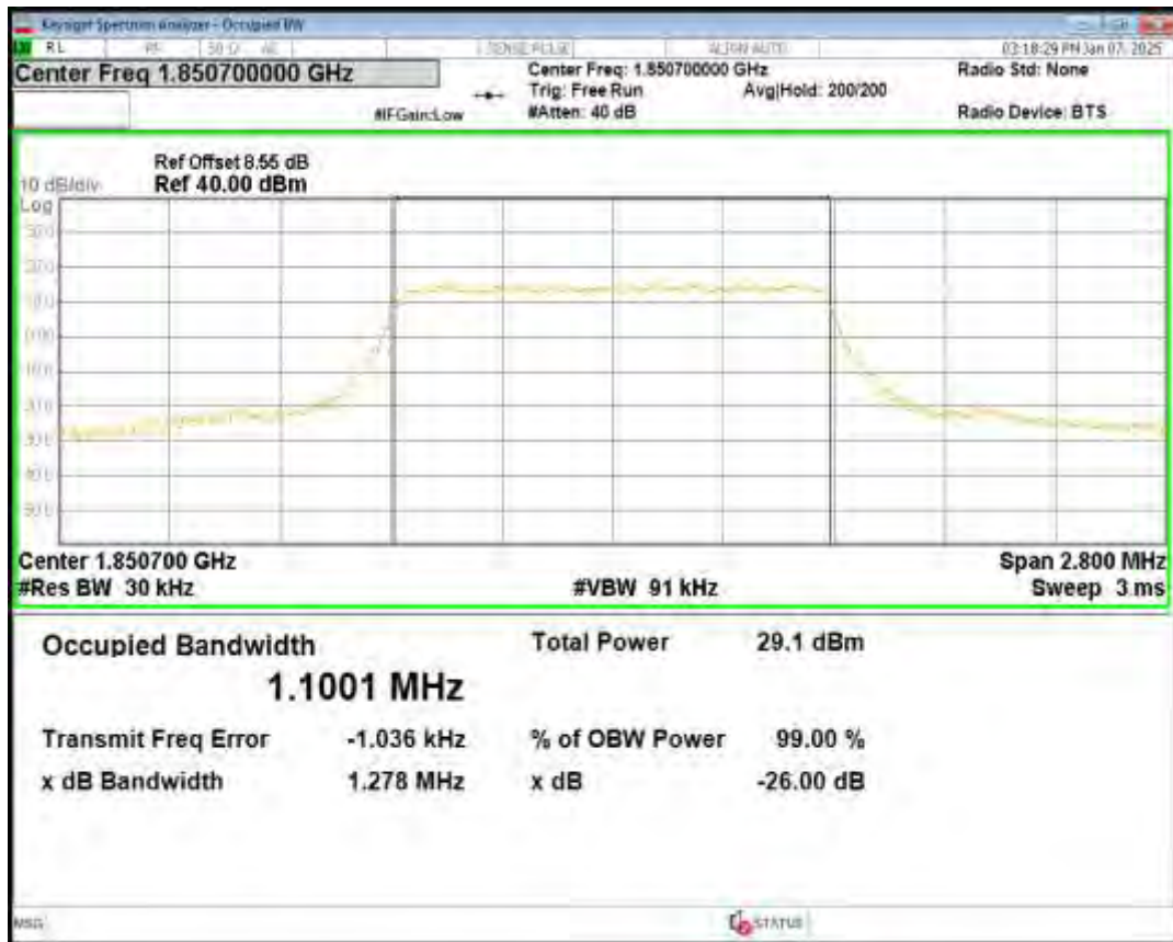
Band2 16QAM BW=5MHz Channel=18900 RB Size=25 Position=#0
