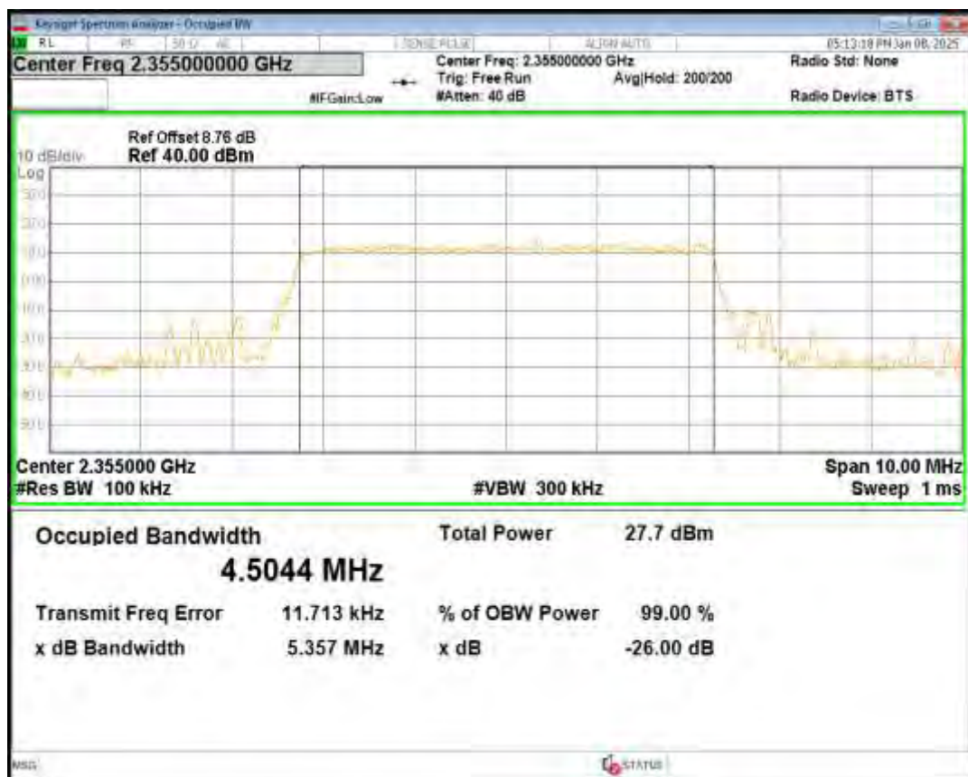
Band40(2350-2360) 16QAM BW=5MHz Channel=39225 RB Size=25 Position=#0
