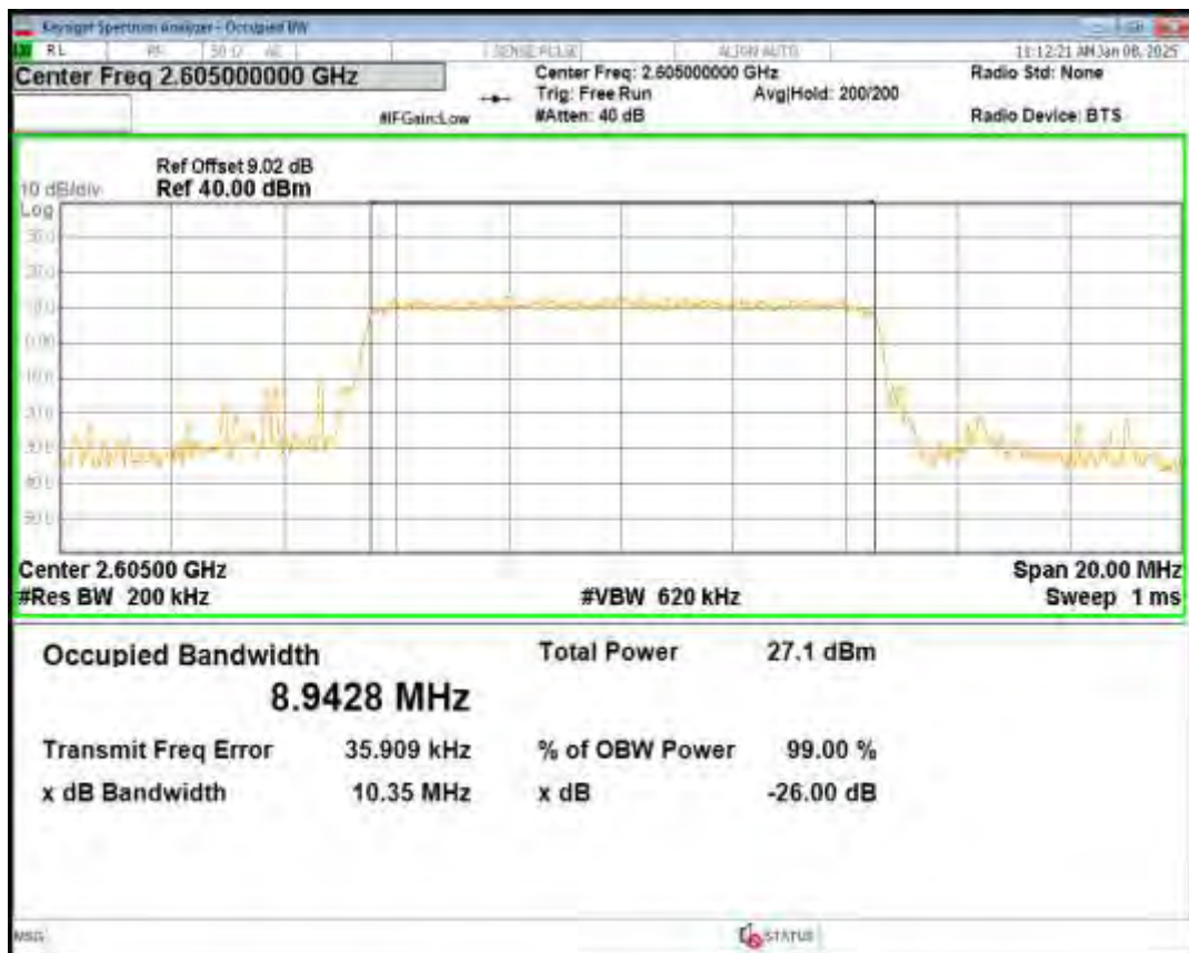
Band41(2555-2655) 16QAM BW=10MHz Channel=41190 RB Size=50 Position=#0
