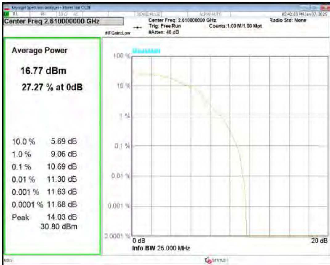
Band38 16QAM BW=5MHz Channel=37775 RB Size=1 Position=#0
