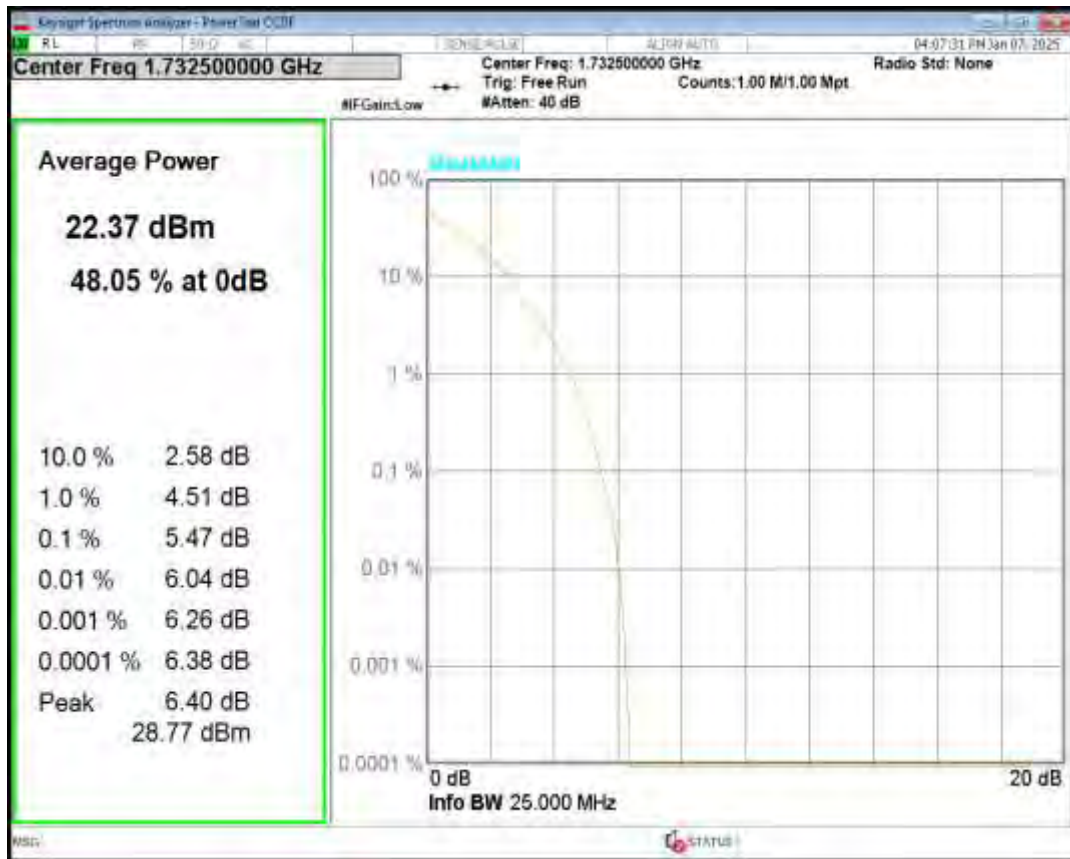
Band4 QPSK BW=3MHz Channel=19965 RB Size=1 Position=#0
