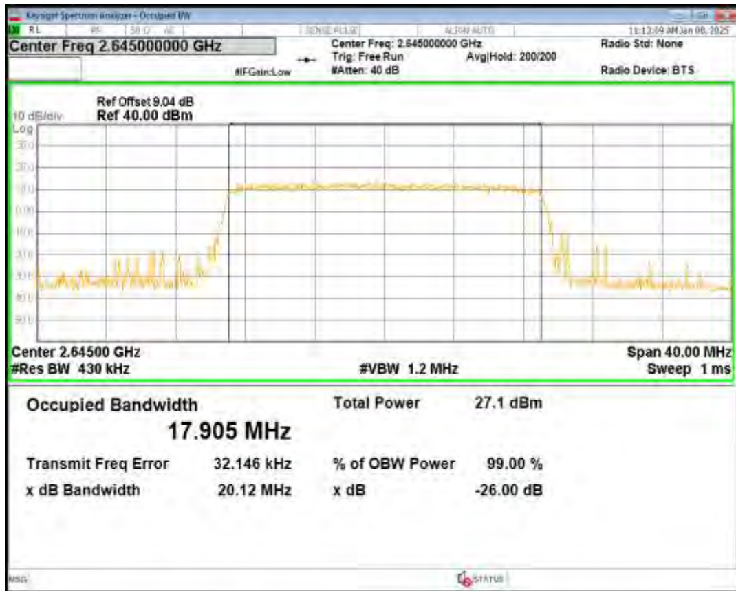
Band41(2555-2655) 16QAM BW=5MHz Channel=40265 RB Size=25 Position=#0
