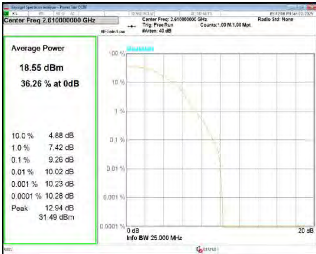
Band38 QPSK BW=5MHz Channel=37775 RB Size=1 Position=#0
