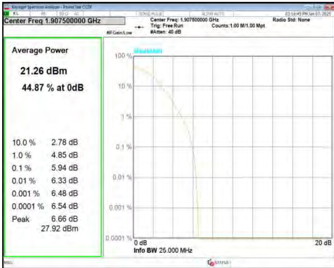
Band2 16QAM BW=5MHz Channel=18900 RB Size=1 Position=#0
