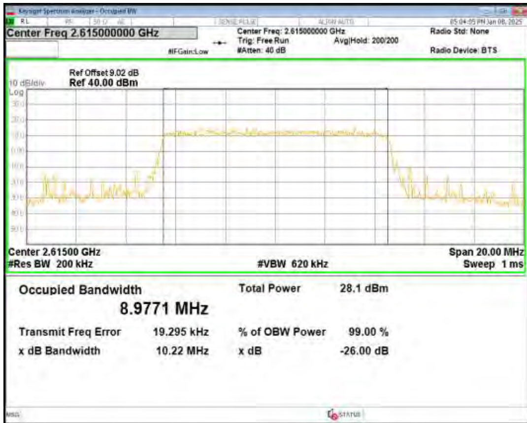
Band38 QPSK BW=15MHz Channel=37825 RB Size=75 Position=#0
