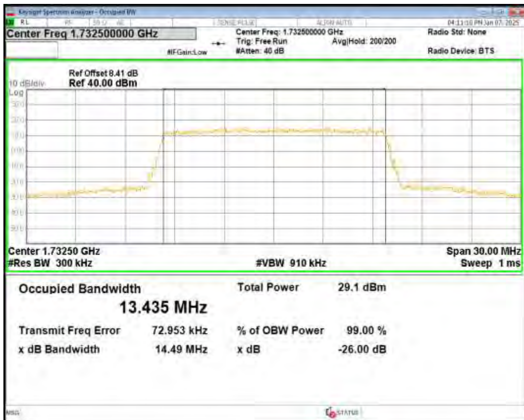
Band4 QPSK BW=15MHz Channel=20325 RB Size=75 Position=#0
