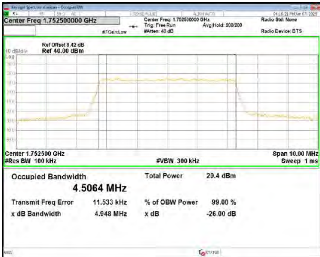
Band40(2305-2315) 16QAM BW=10MHz Channel=38750 RB Size=50 Position=#0
