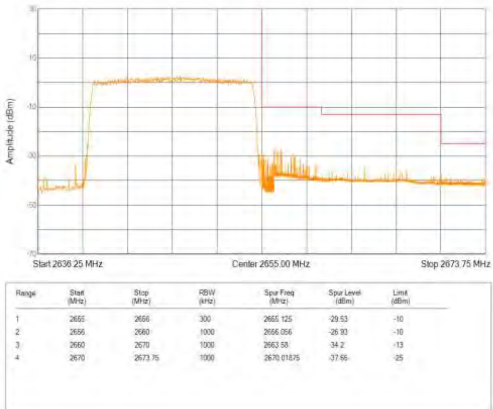
Band41(2555-2655) QPSK BW=20MHz Channel=40340 RB Size=100 Position=#0
