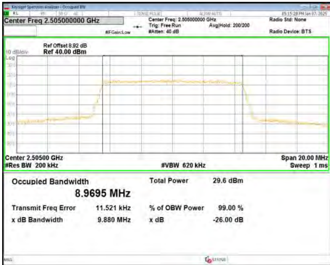
Band7 16QAM BW=5MHz Channel=21100 RB Size=25 Position=#0
