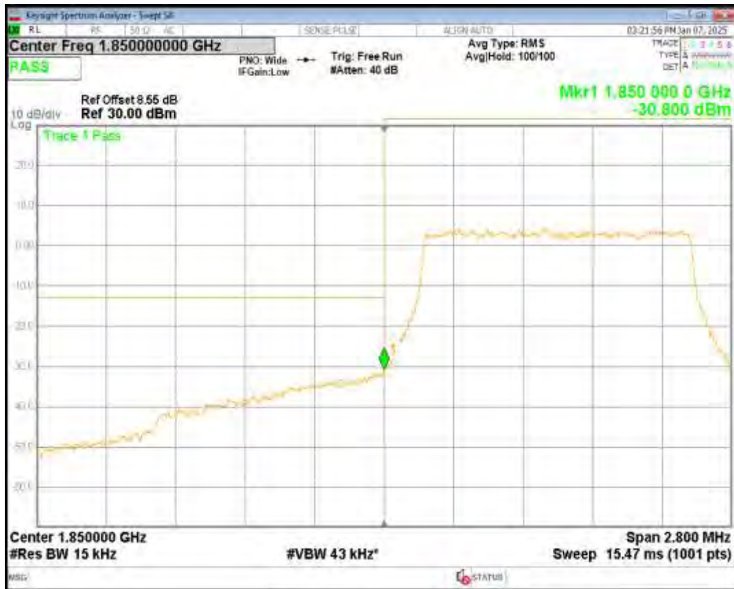
Band2 QPSK BW=1.4MHz Channel=19193 RB Size=6 Position=#0
