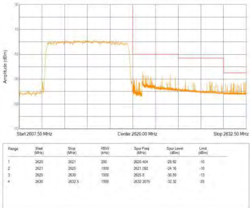
Band38 16QAM BW=15MHz Channel=37825 RB Size=75 Position=#0
