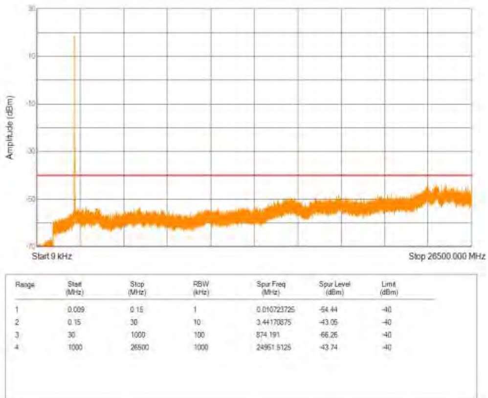
Band40(2305-2315) QPSK BW=5MHz Channel=38725 RB Size=25 Position=#0
