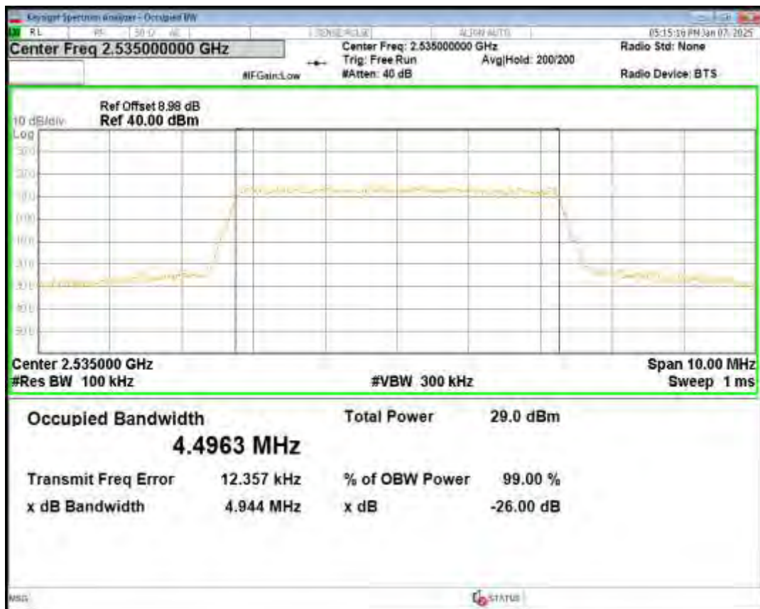
Band7 16QAM BW=5MHz Channel=20775 RB Size=25 Position=#0
