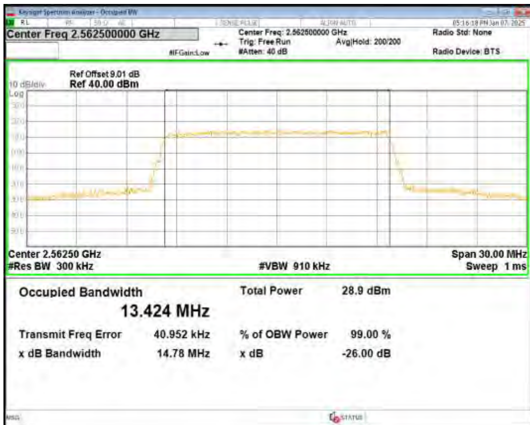
Band7 16QAM BW=20MHz Channel=20850 RB Size=100 Position=#0
