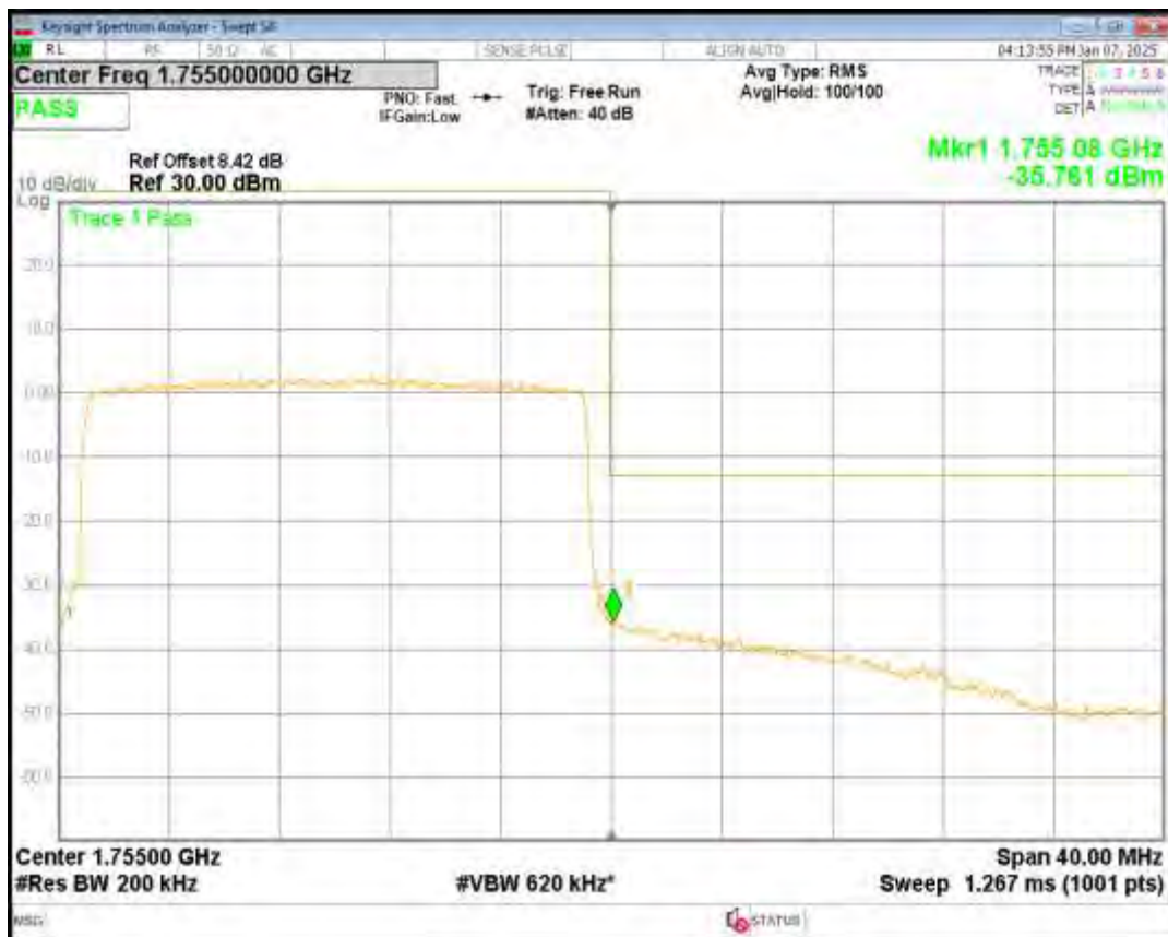
Band4 16QAM BW=3MHz Channel=19965 RB Size=15 Position=#0
