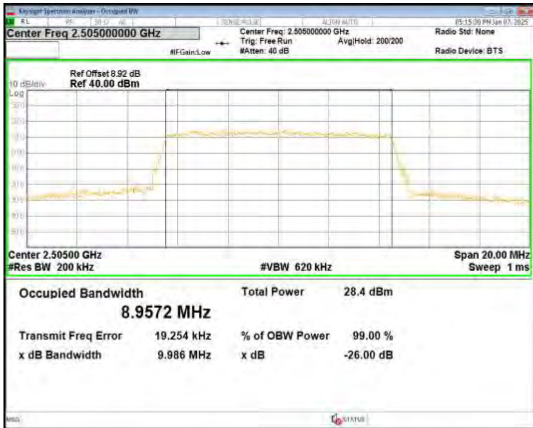
Band7 16QAM BW=10MHz Channel=21100 RB Size=50 Position=#0
