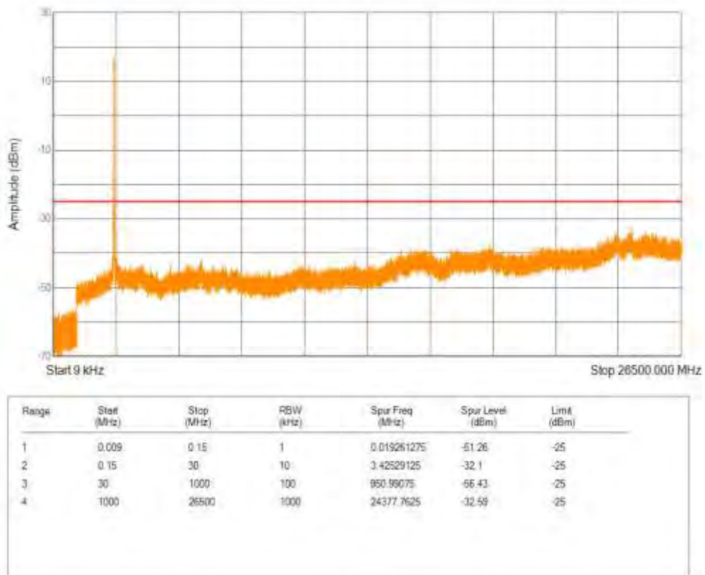
Band41(2555-2655) QPSK BW=20MHz Channel=40740 RB Size=100 Position=#0
