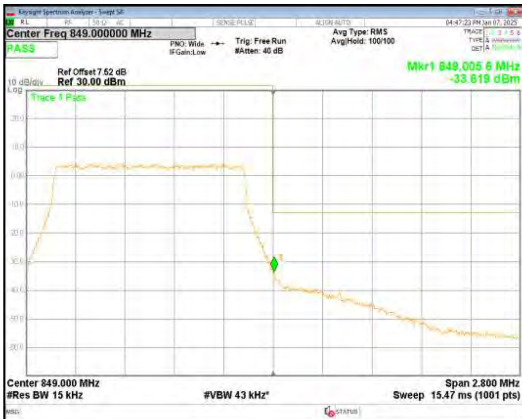
Band5 16QAM BW=10MHz Channel=20450 RB Size=50 Position=#0
