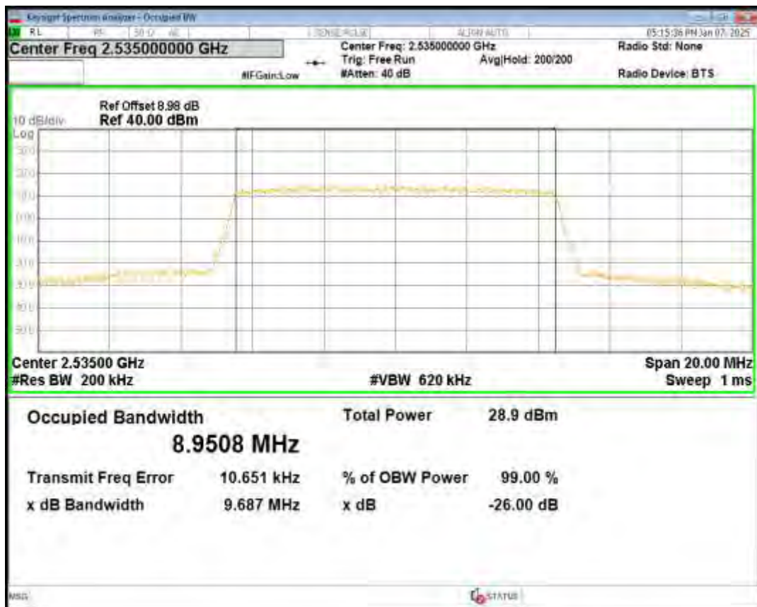
Band7 16QAM BW=10MHz Channel=21400 RB Size=50 Position=#0
