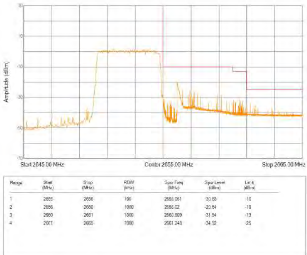
Band5 16QAM BW=1.4MHz Channel=20407 RB Size=6 Position=#0
