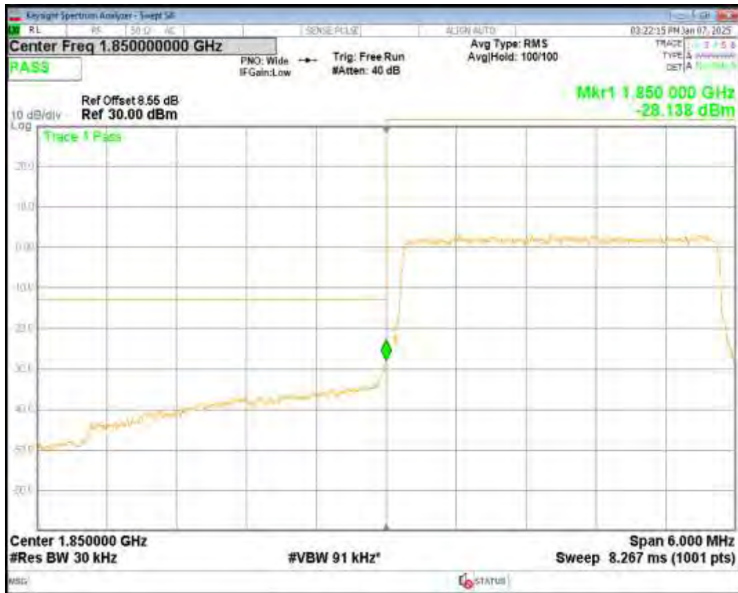
Band2 QPSK BW=3MHz Channel=19185 RB Size=15 Position=#0
