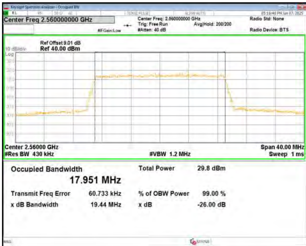
Band7 QPSK BW=5MHz Channel=20775 RB Size=25 Position=#0
