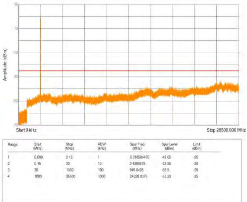
Band38 QPSK BW=15MHz Channel=37825 RB Size=75 Position=#0
