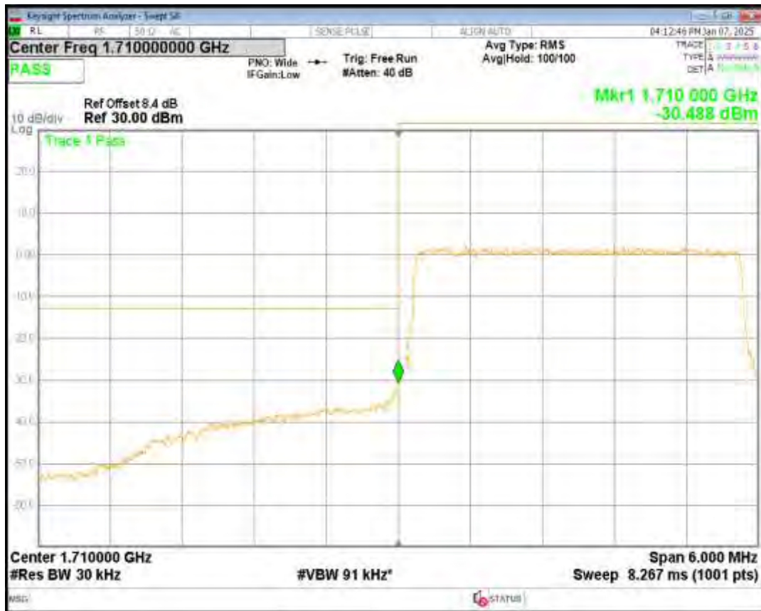
Band4 16QAM BW=3MHz Channel=20385 RB Size=15 Position=#0
