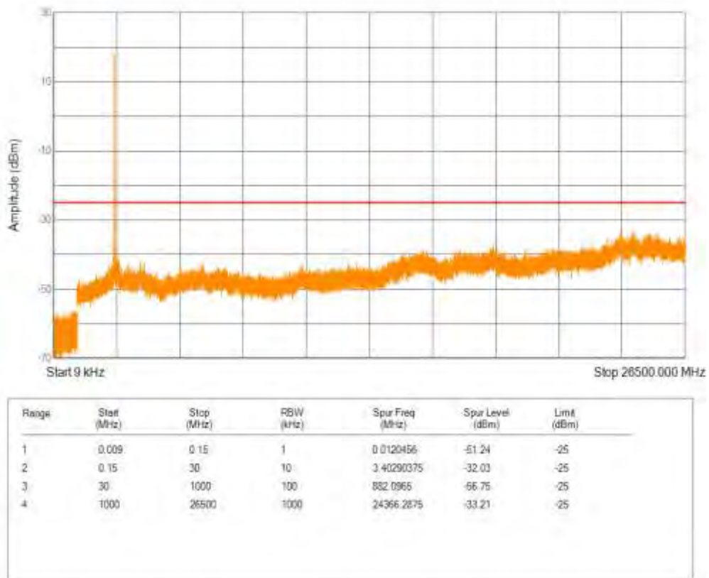
Band41(2555-2655) 16QAM BW=10MHz Channel=40740 RB Size=50 Position=#0
