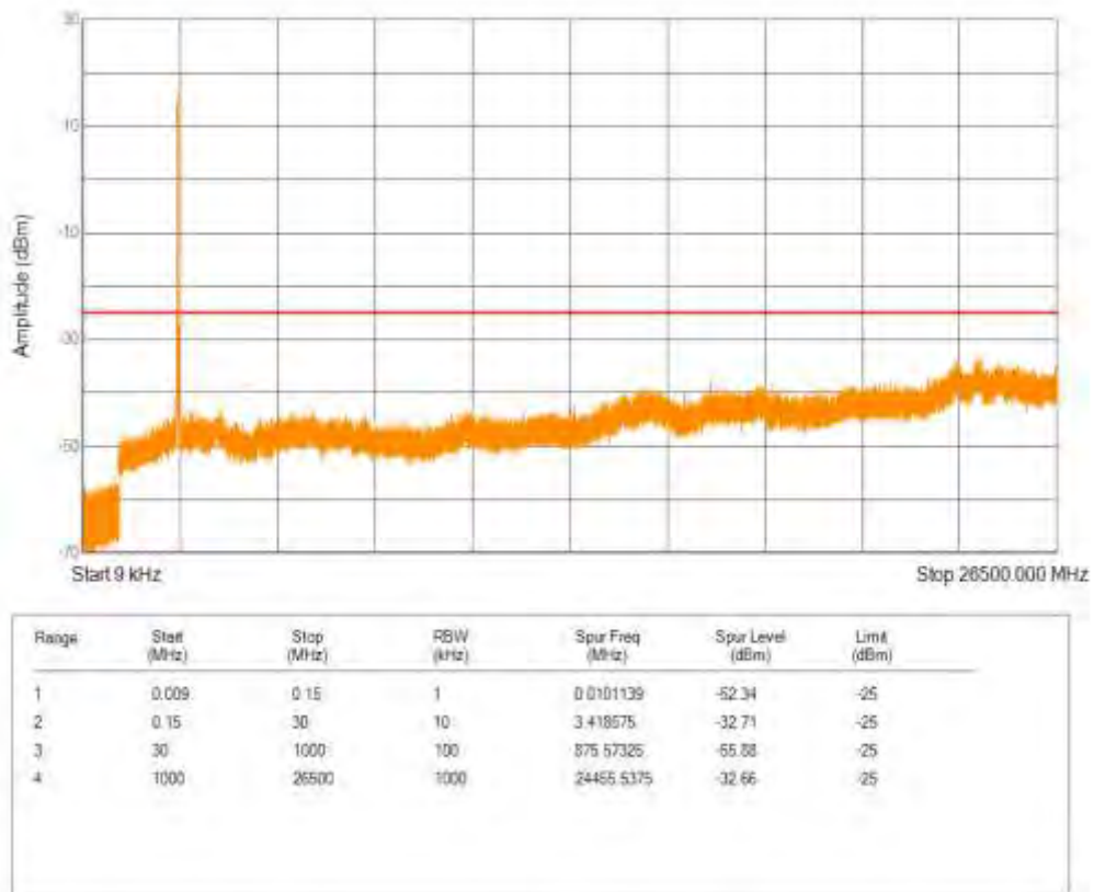
Band38 QPSK BW=20MHz Channel=38150 RB Size=100 Position=#0
