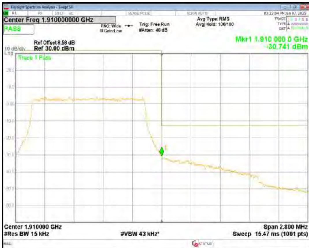
Band2 QPSK BW=10MHz Channel=18650 RB Size=50 Position=#0
