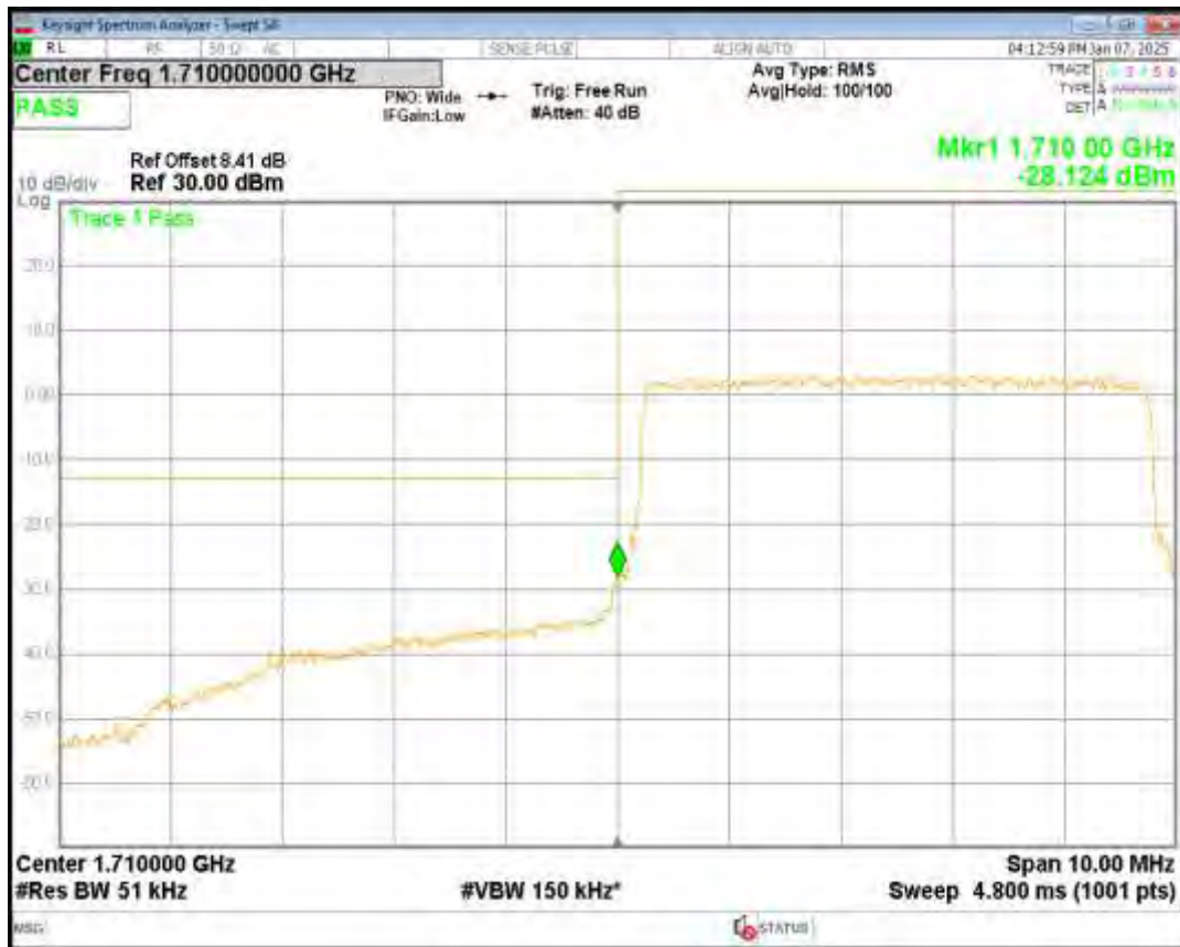
Band4 QPSK BW=5MHz Channel=20375 RB Size=25 Position=#0
