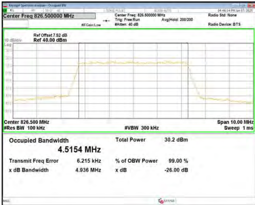
Band5 QPSK BW=5MHz Channel=20625 RB Size=25 Position=#0
