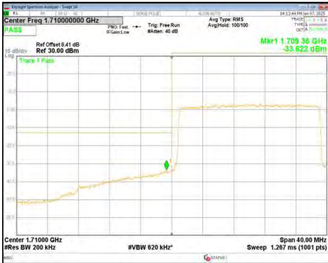
Band4 QPSK BW=20MHz Channel=20300 RB Size=100 Position=#0
