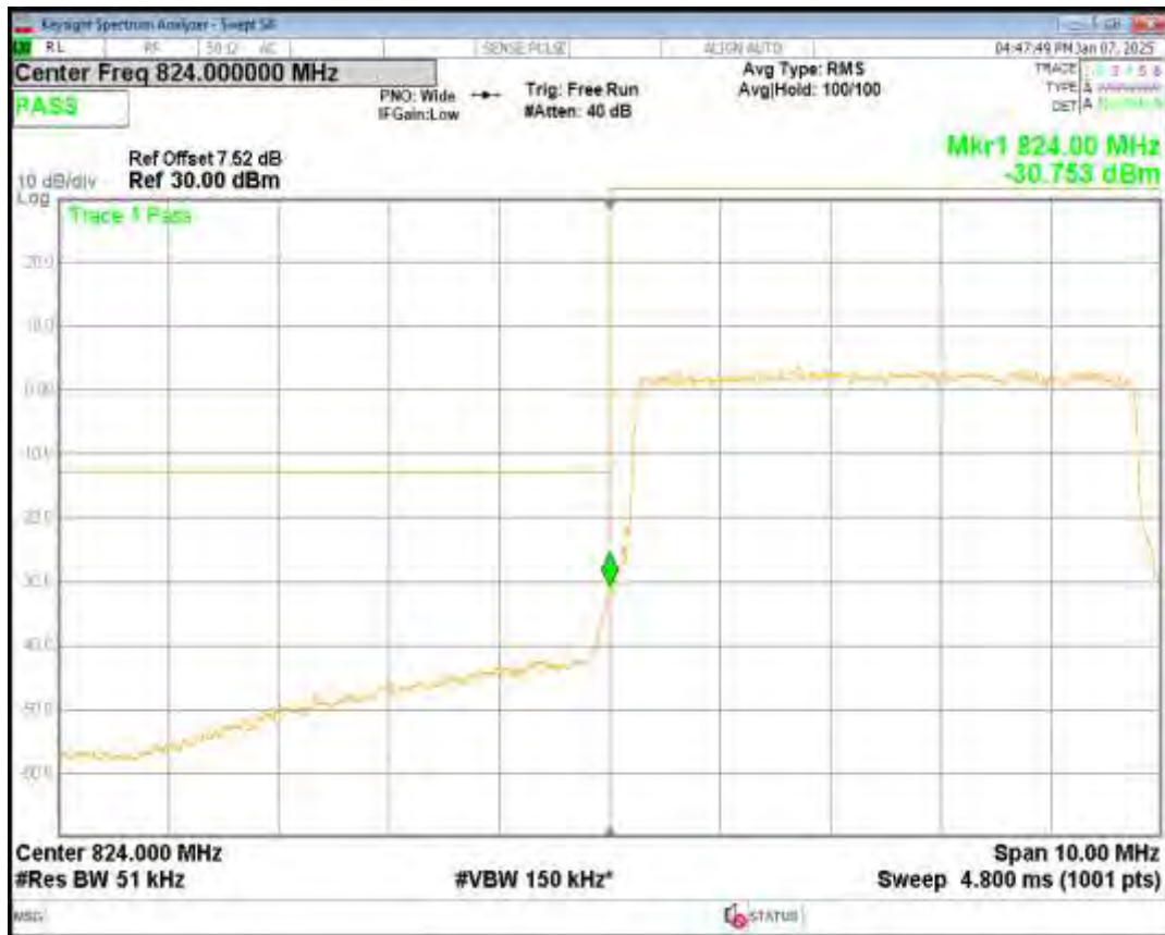
Band5 16QAM BW=5MHz Channel=20625 RB Size=25 Position=#0
