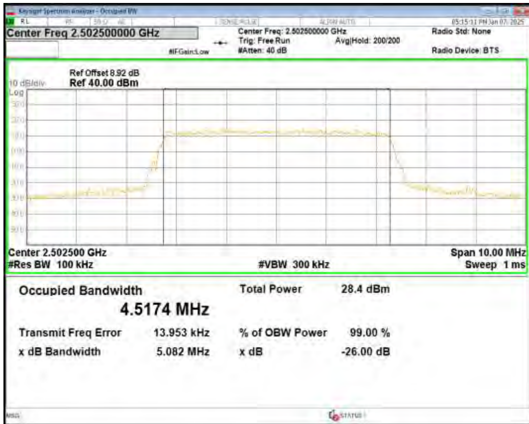
Band7 QPSK BW=10MHz Channel=21100 RB Size=50 Position=#0
