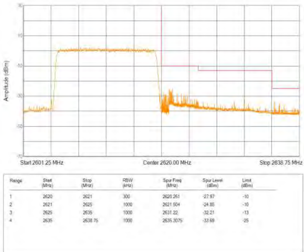
Band38 QPSK BW=20MHz Channel=37850 RB Size=100 Position=#0
