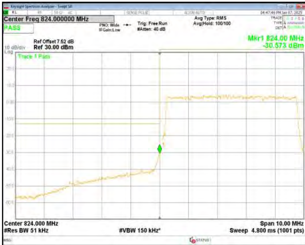
Band5 QPSK BW=5MHz Channel=20625 RB Size=25 Position=#0
