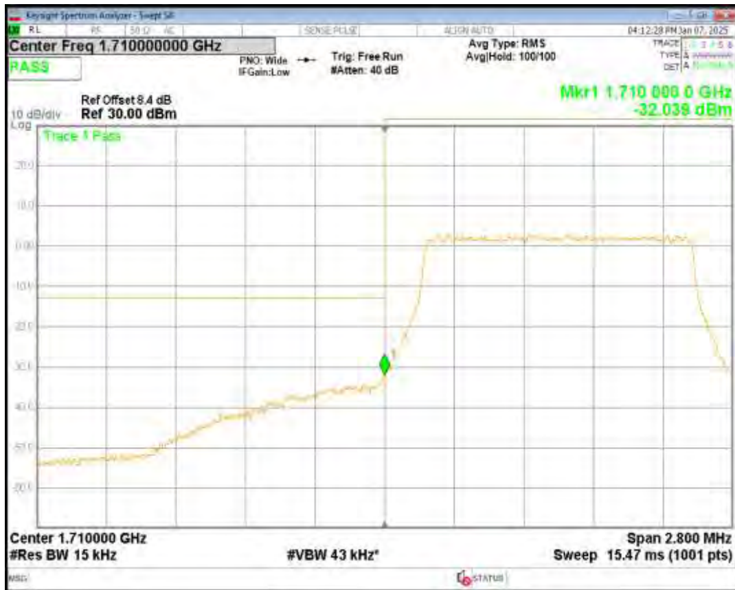
Band4 16QAM BW=1.4MHz Channel=20393 RB Size=6 Position=#0
