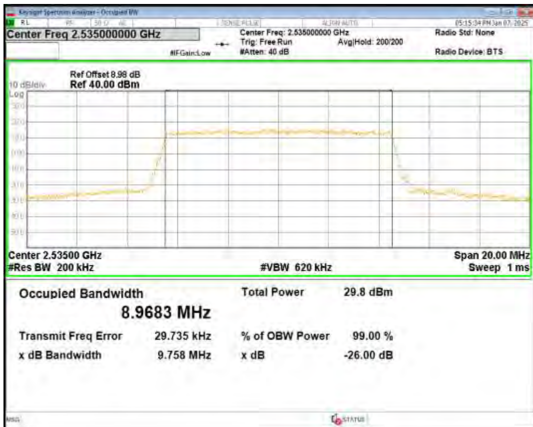
Band7 QPSK BW=5MHz Channel=21100 RB Size=25 Position=#0
