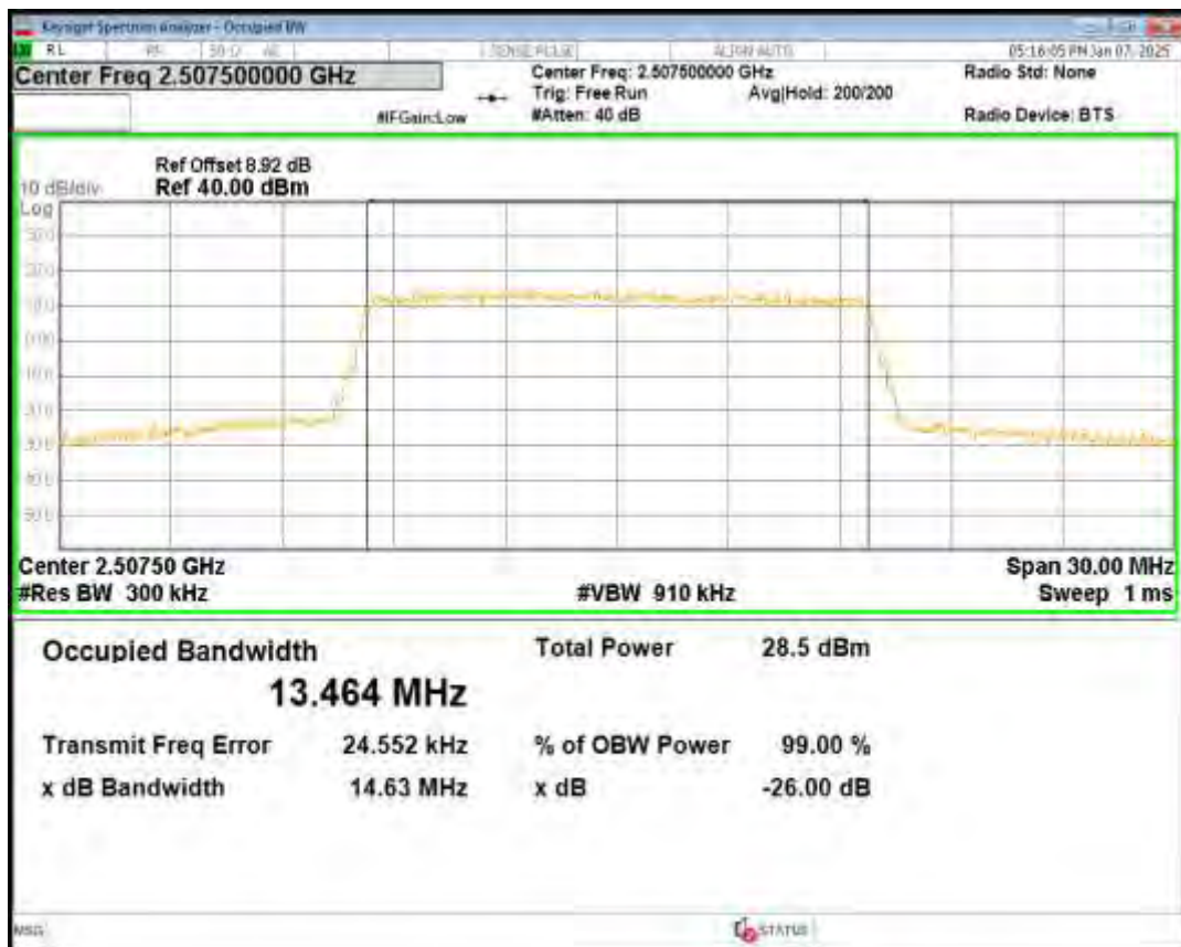
Band7 16QAM BW=15MHz Channel=21100 RB Size=75 Position=#0
