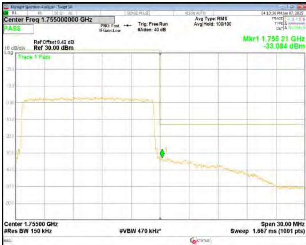
Band4 QPSK BW=20MHz Channel=20050 RB Size=100 Position=#0
