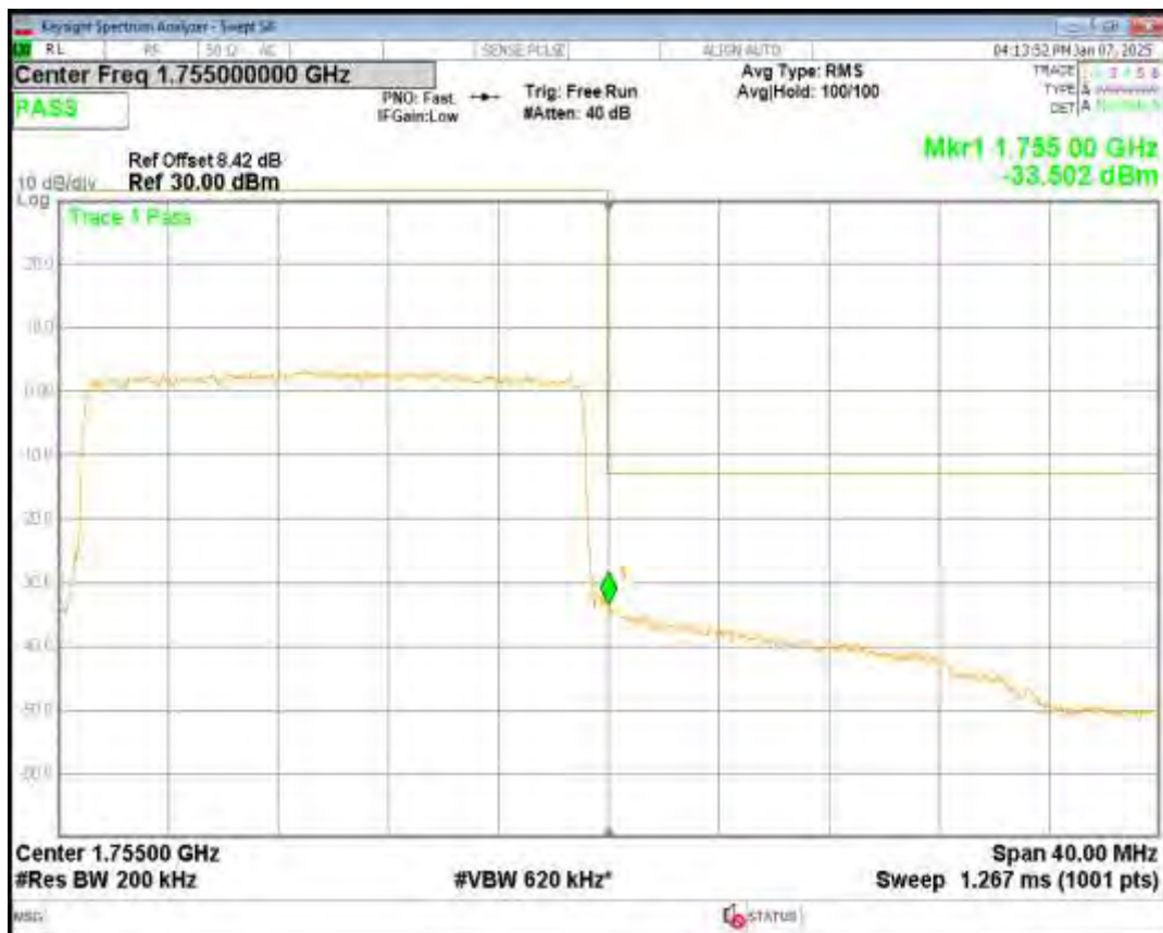
Band4 QPSK BW=3MHz Channel=19965 RB Size=15 Position=#0
