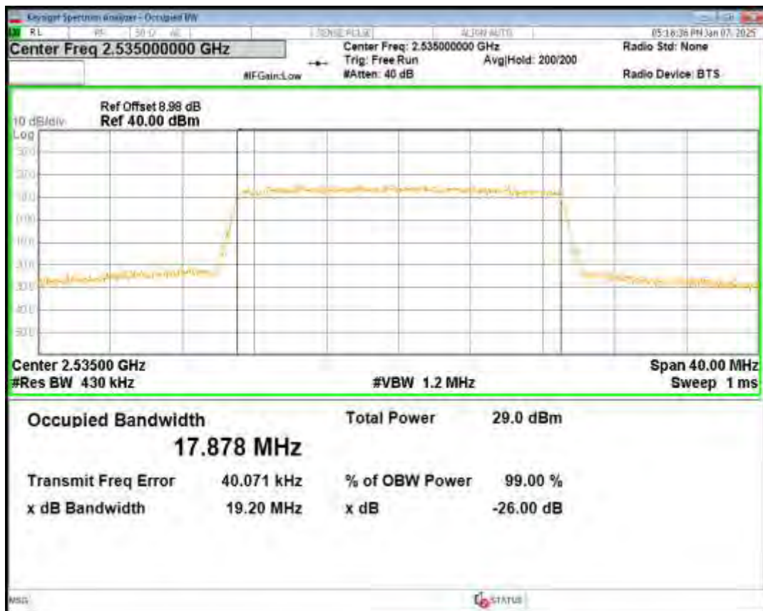
Band7 16QAM BW=20MHz Channel=21350 RB Size=100 Position=#0
