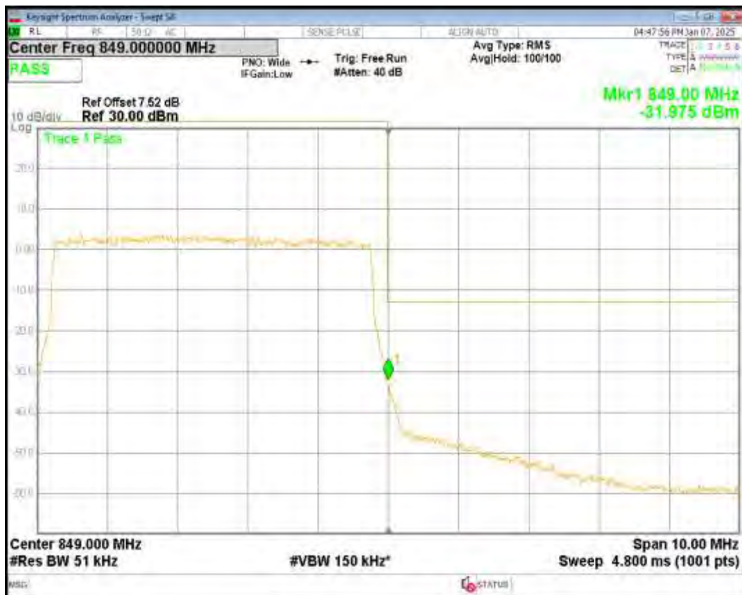
Band5 QPSK BW=1.4MHz Channel=20407 RB Size=6 Position=#0
