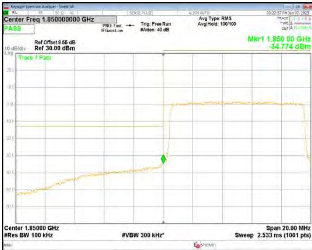
Band2 16QAM BW=10MHz Channel=19150 RB Size=50 Position=#0
