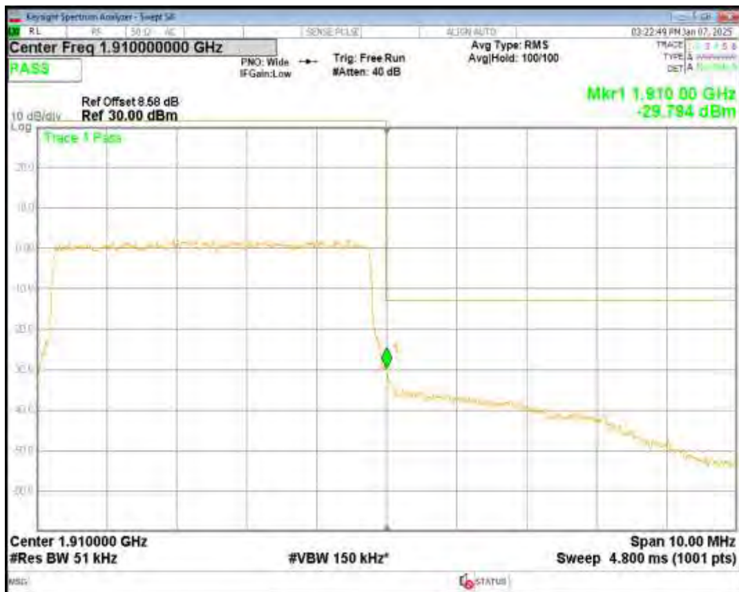
Band2 QPSK BW=1.4MHz Channel=18607 RB Size=6 Position=#0
