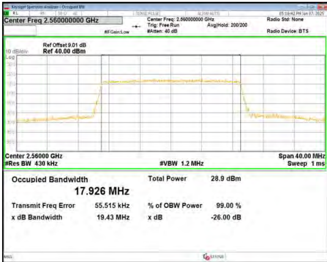
Band7 QPSK BW=15MHz Channel=21375 RB Size=75 Position=#0
