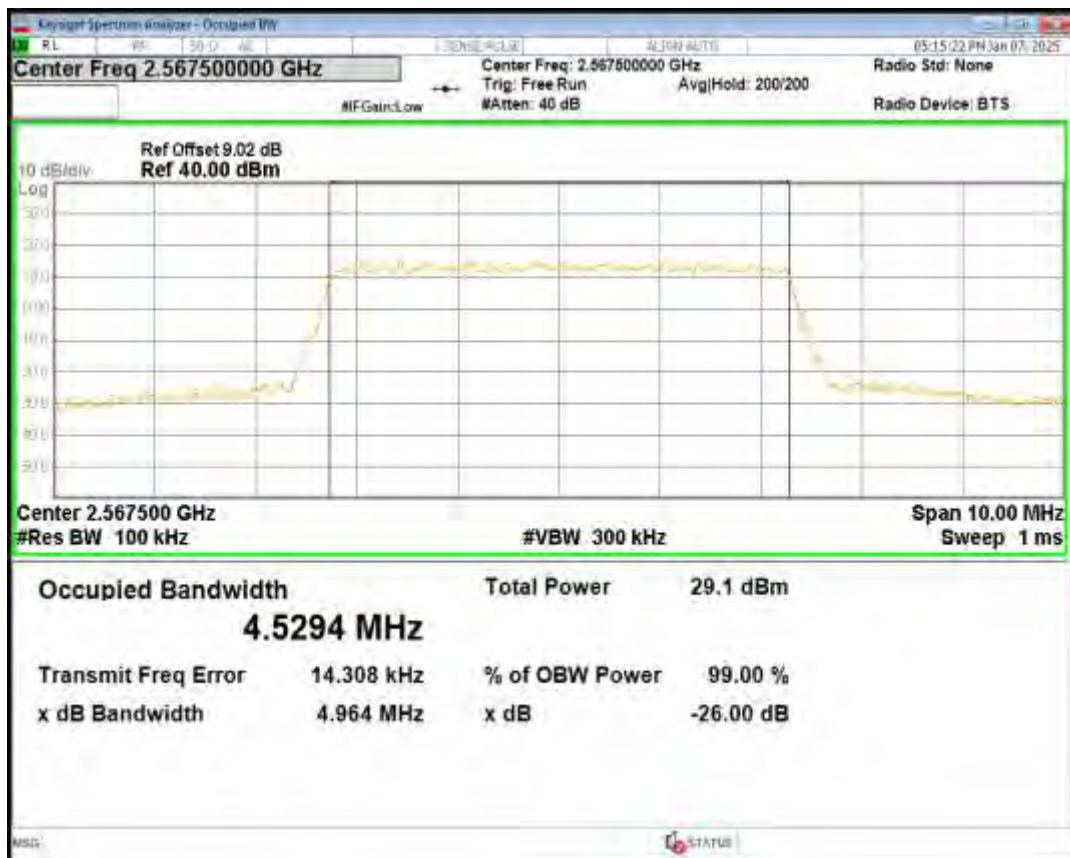
Band7 QPSK BW=10MHz Channel=20800 RB Size=50 Position=#0
