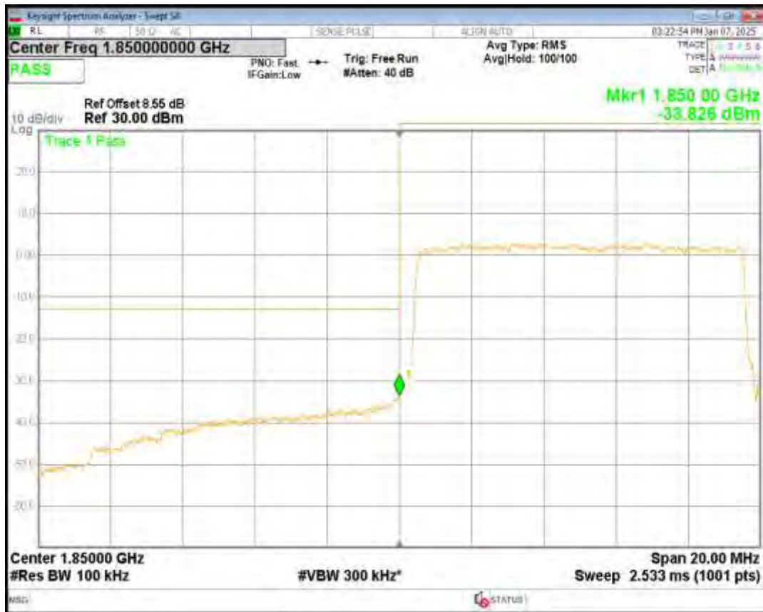
Band2 QPSK BW=10MHz Channel=19150 RB Size=50 Position=#0
