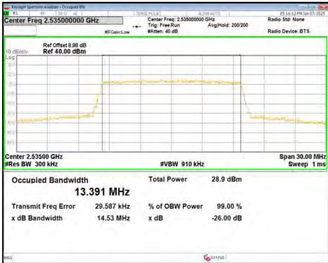
Band7 16QAM BW=15MHz Channel=21375 RB Size=75 Position=#0
