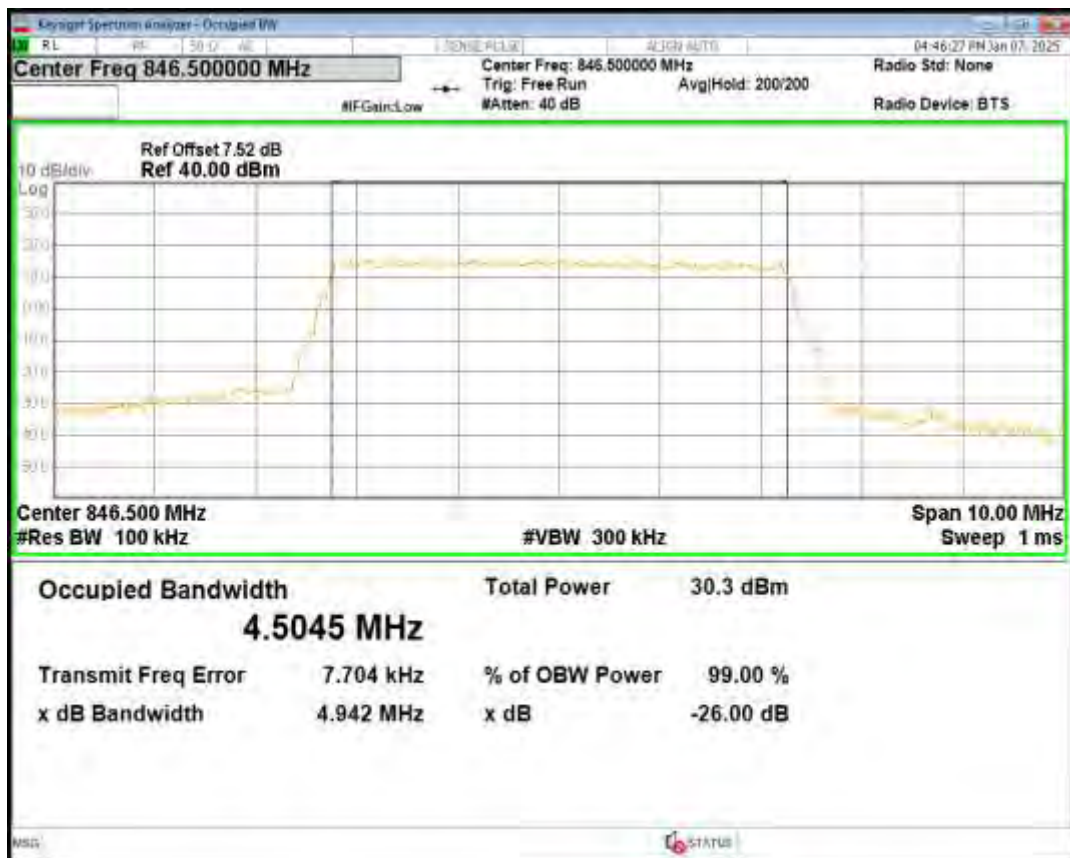
Band7 16QAM BW=10MHz Channel=20800 RB Size=50 Position=#0
