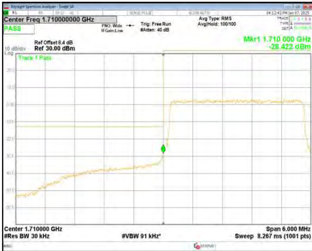
Band4 QPSK BW=3MHz Channel=20385 RB Size=15 Position=#0
