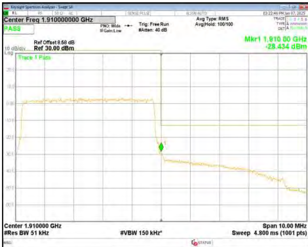
Band38 16QAM BW=10MHz Channel=37800 RB Size=50 Position=#0
