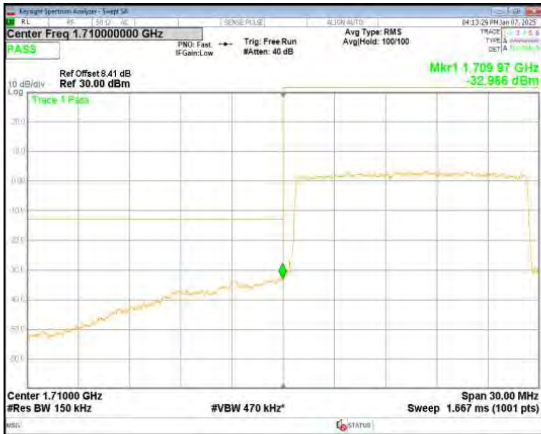
Band4 QPSK BW=15MHz Channel=20325 RB Size=75 Position=#0
