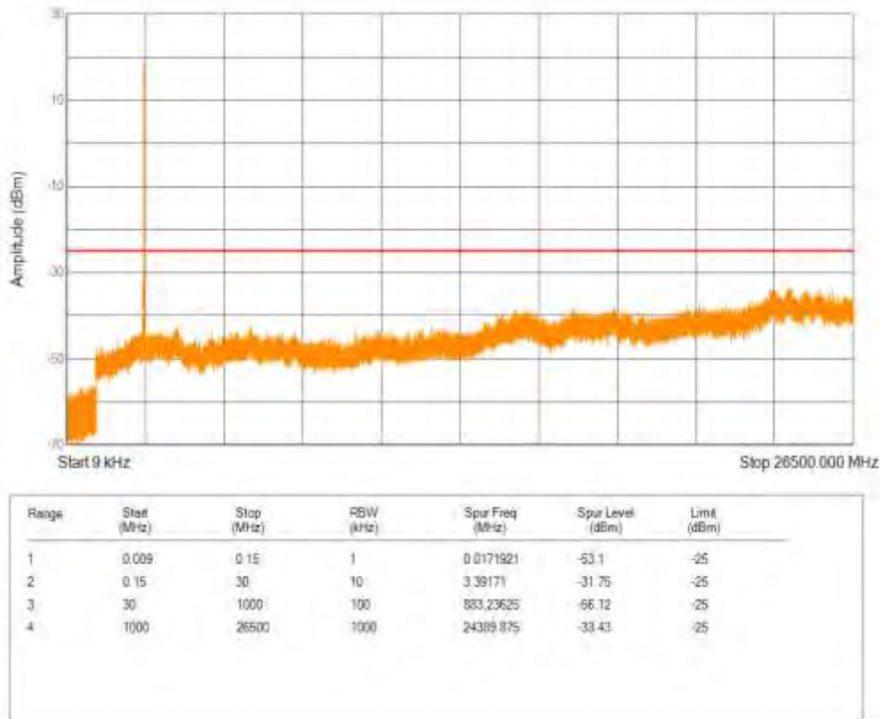
Band41(2555-2655) QPSK BW=10MHz Channel=41190 RB Size=50 Position=#0
