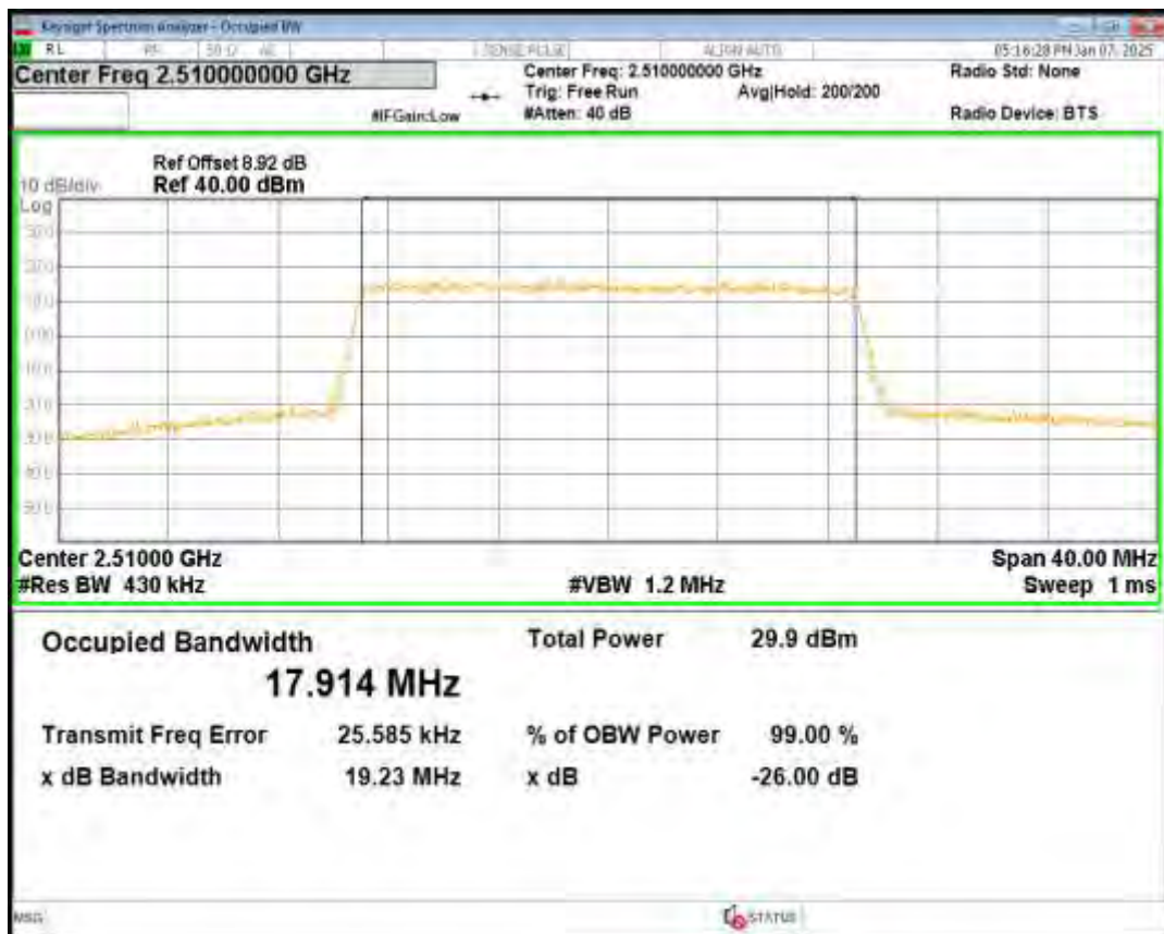
Band7 QPSK BW=20MHz Channel=21100 RB Size=100 Position=#0
