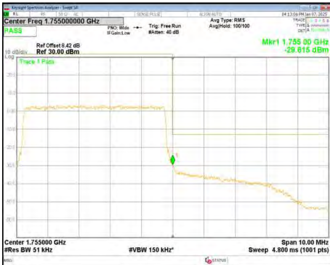
Band40(2305-2315) 16QAM BW=10MHz Channel=38750 RB Size=50 Position=#0
