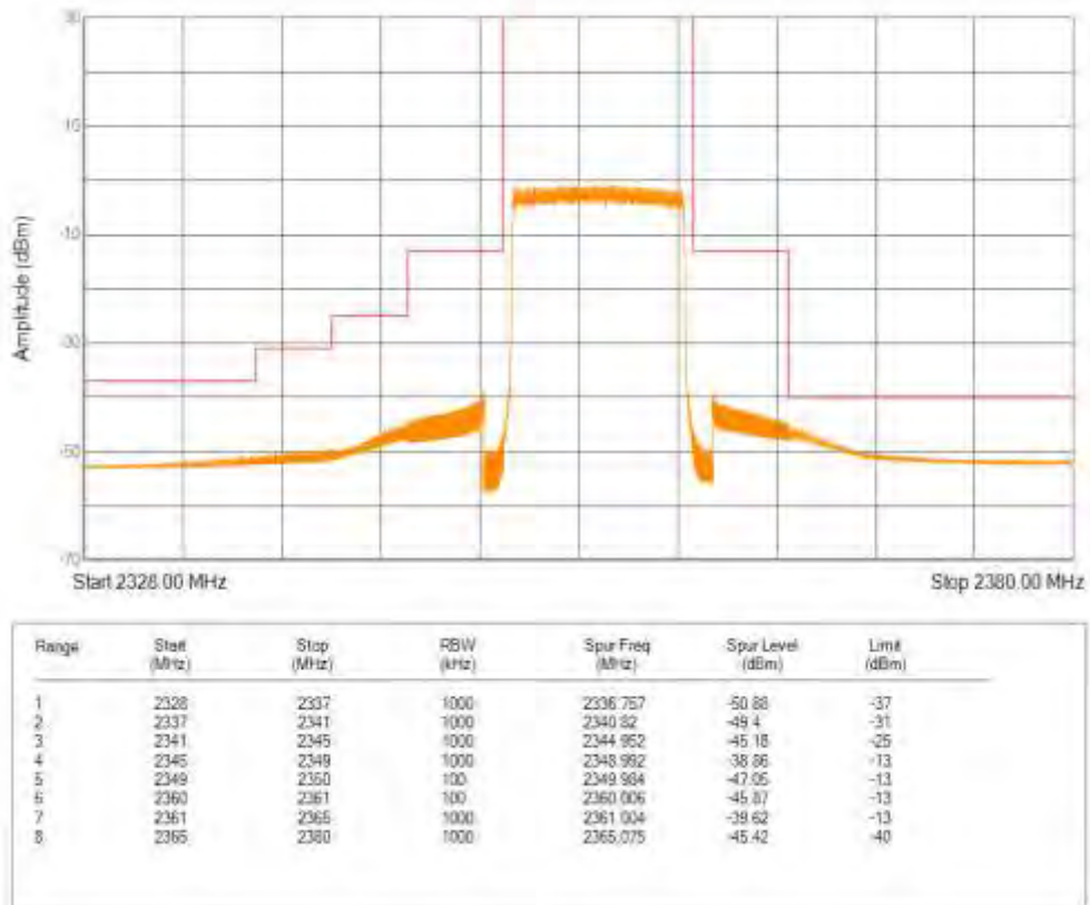
Band40(2350-2360) 16QAM BW=5MHz Channel=39175 RB Size=25 Position=#0
