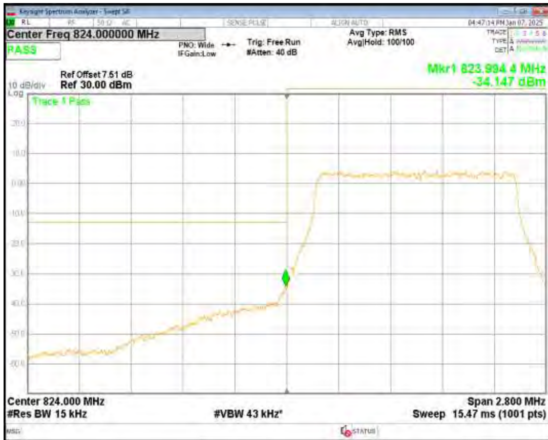
Band5 16QAM BW=1.4MHz Channel=20643 RB Size=6 Position=#0
