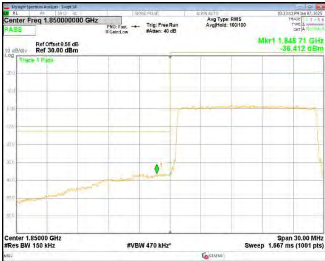
Band2 16QAM BW=15MHz Channel=19125 RB Size=75 Position=#0
