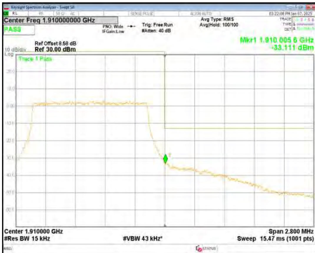
Band2 16QAM BW=10MHz Channel=18650 RB Size=50 Position=#0
