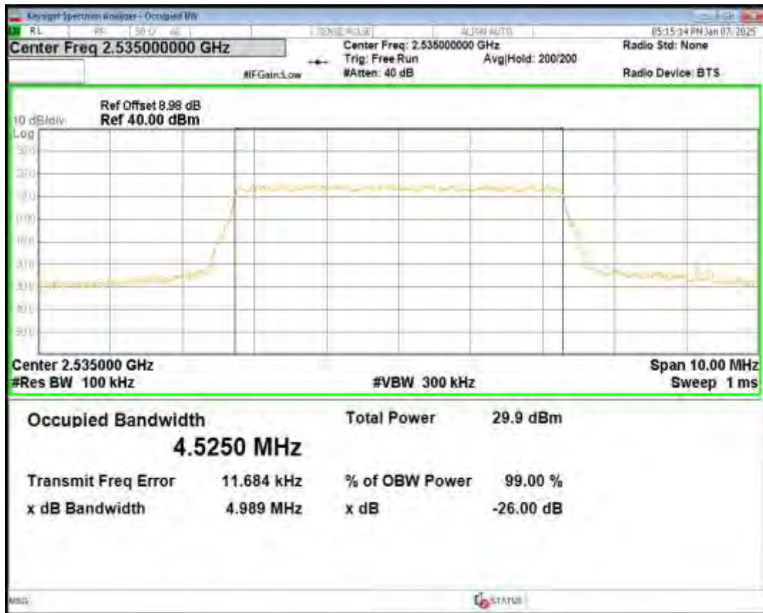
Band7 QPSK BW=20MHz Channel=20850 RB Size=100 Position=#0
