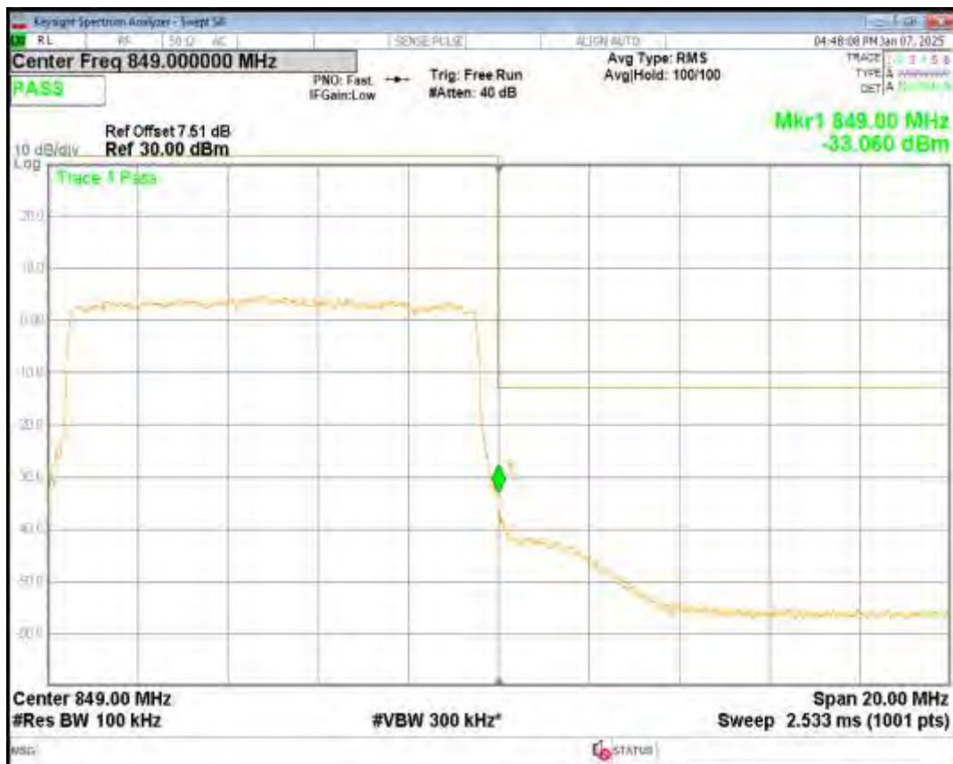
Band5 QPSK BW=3MHz Channel=20415 RB Size=15 Position=#0
