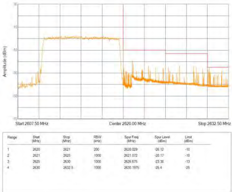
Band38 QPSK BW=15MHz Channel=37825 RB Size=75 Position=#0
