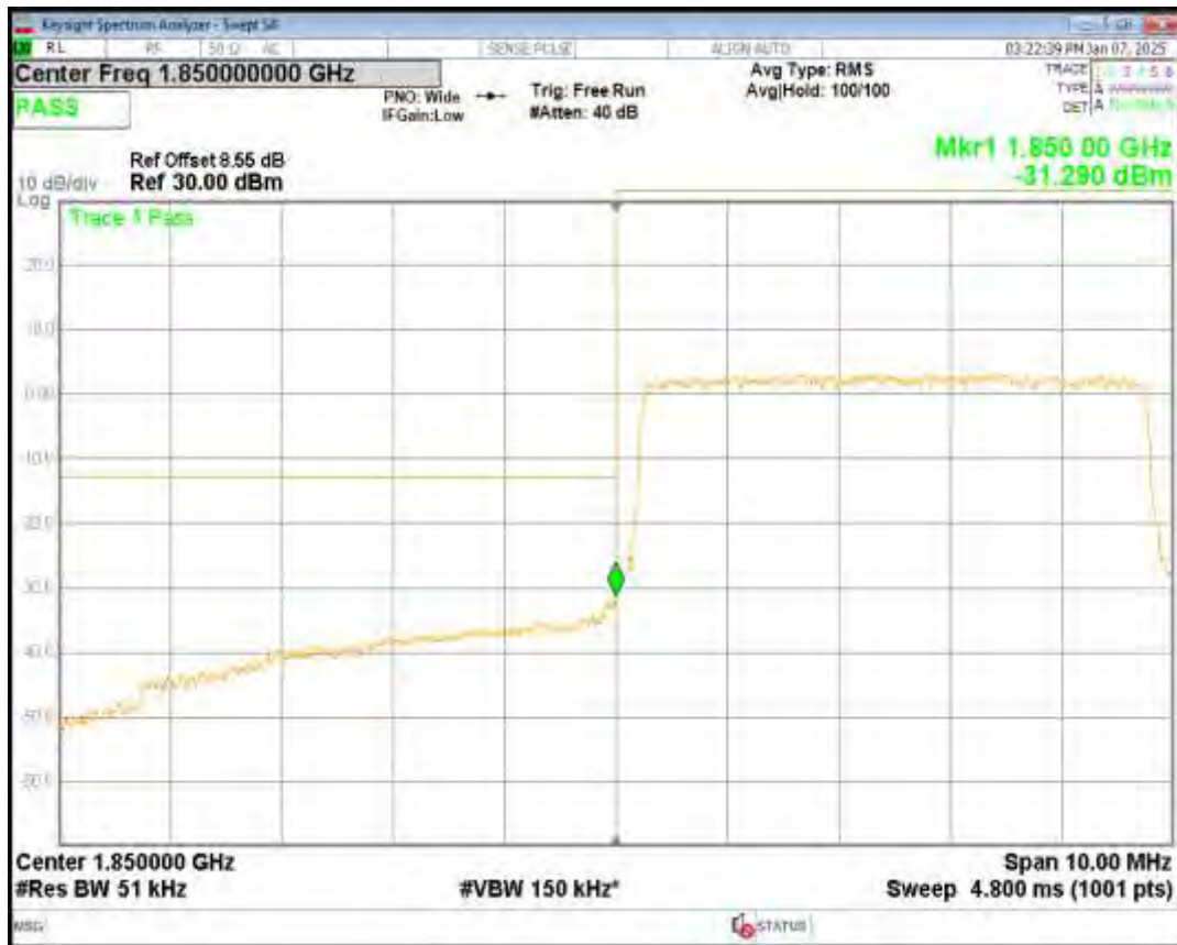
Band2 QPSK BW=5MHz Channel=19175 RB Size=25 Position=#0
