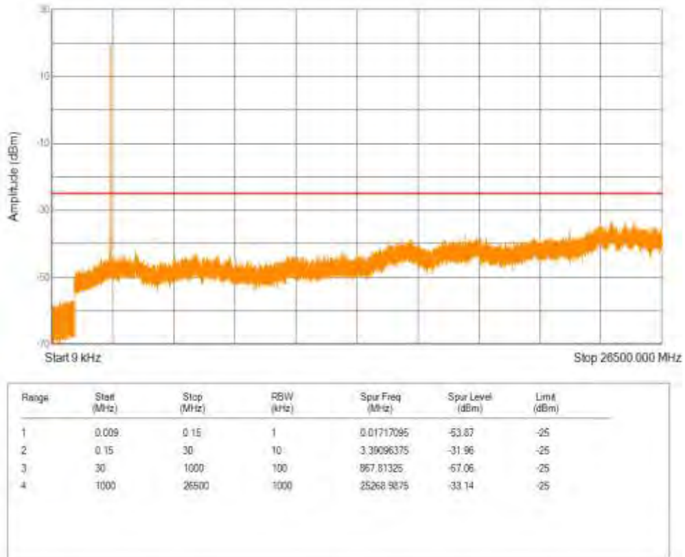
Band41(2555-2655) 16QAM BW=5MHz Channel=41215 RB Size=25 Position=#0
