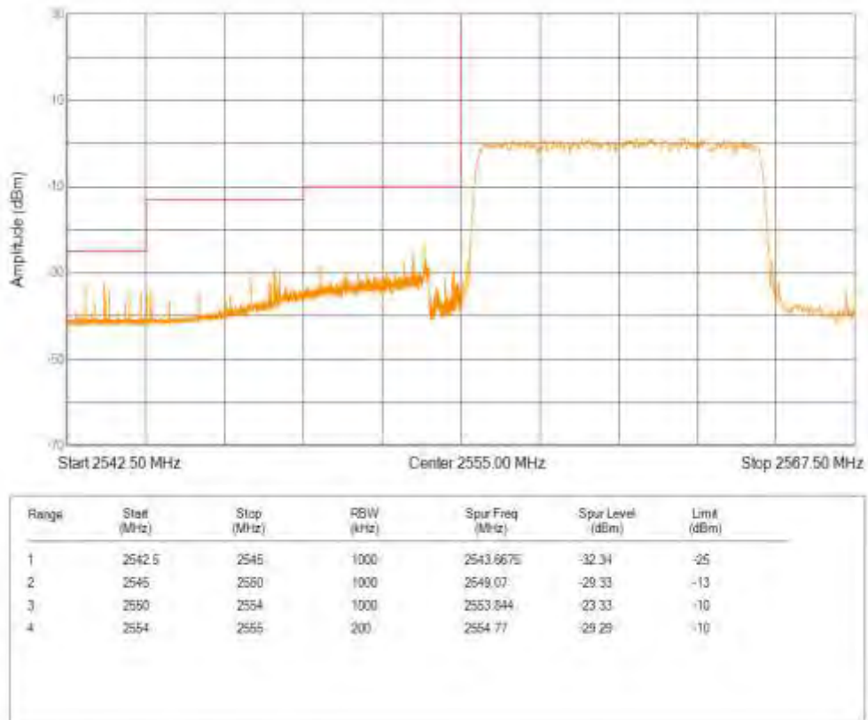
Band41(2555-2655) 16QAM BW=10MHz Channel=41190 RB Size=50 Position=#0
