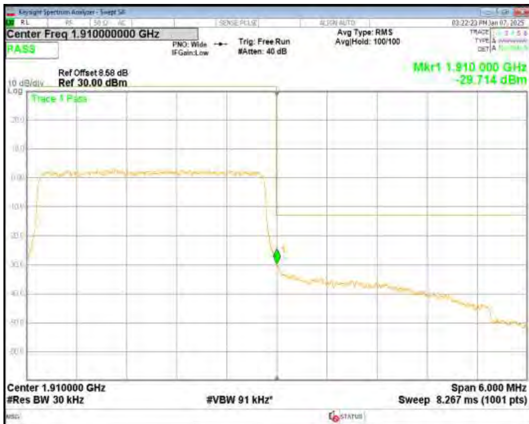
Band2 QPSK BW=5MHz Channel=18625 RB Size=25 Position=#0
