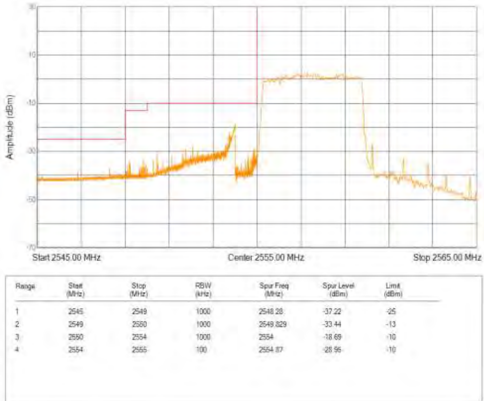
Band41(2555-2655) QPSK BW=5MHz Channel=41215 RB Size=25 Position=#0
