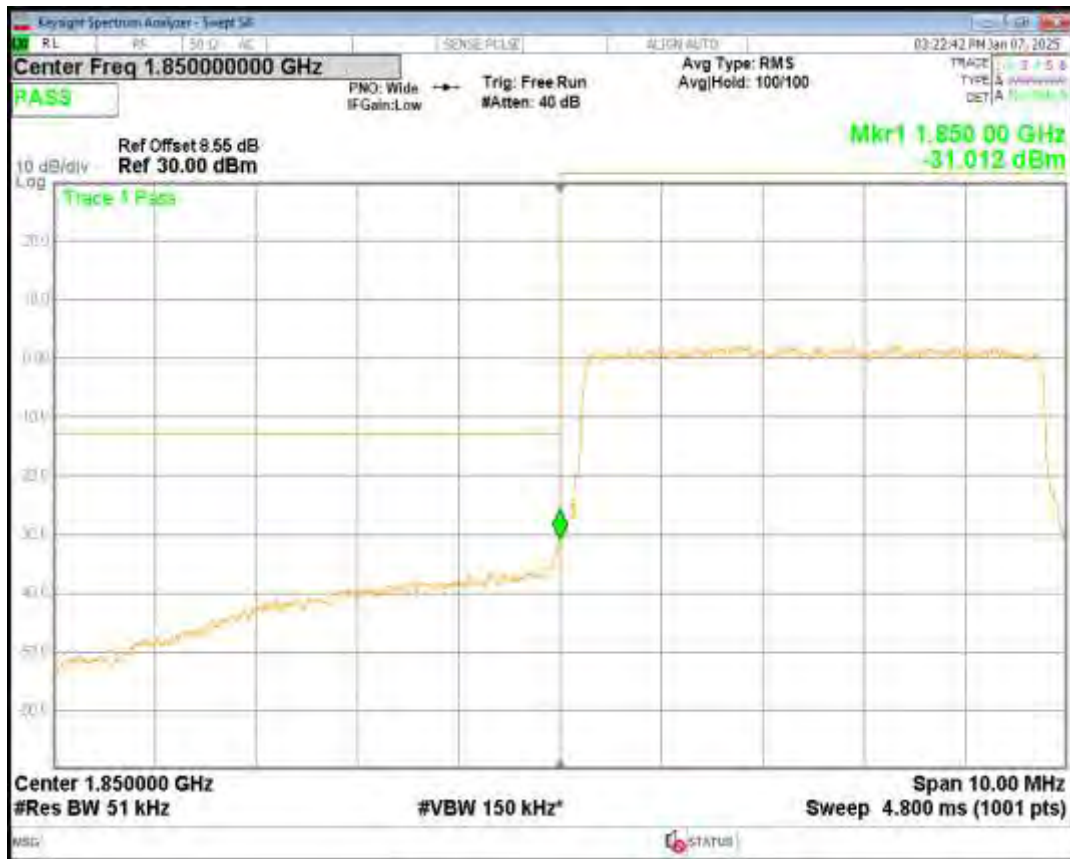
Band2 16QAM BW=5MHz Channel=19175 RB Size=25 Position=#0
