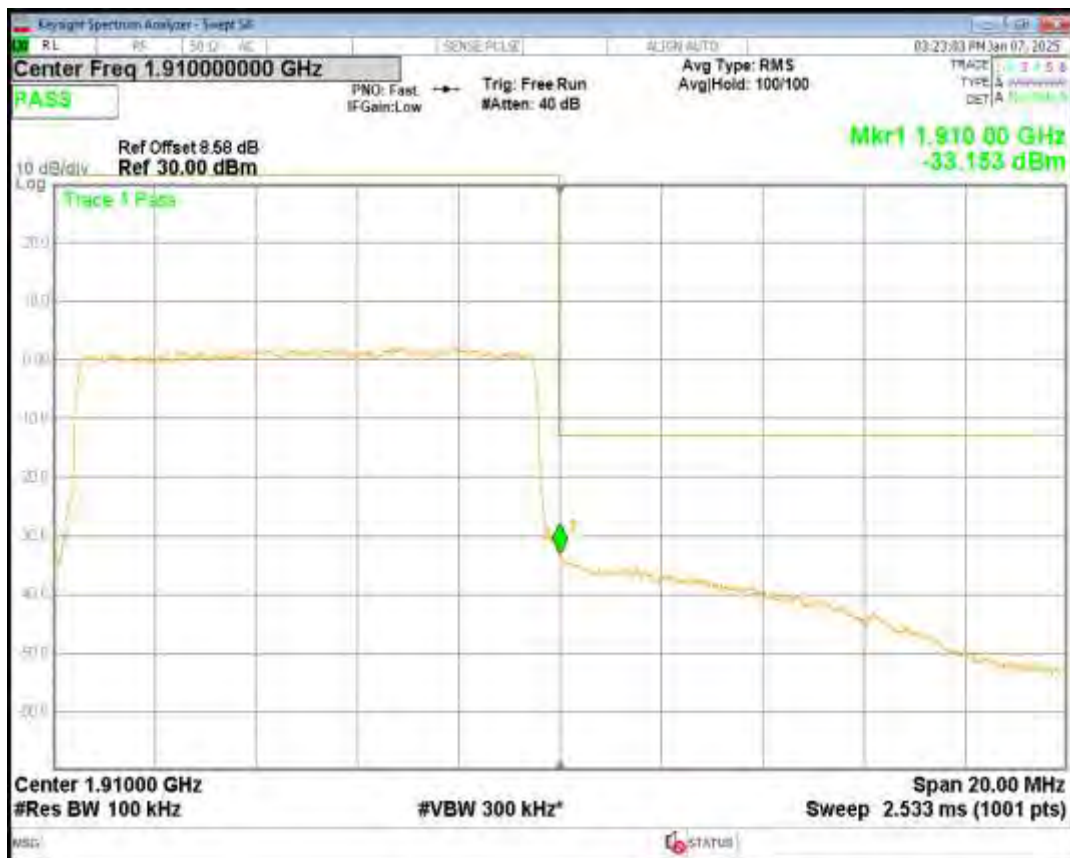
Band2 16QAM BW=15MHz Channel=18675 RB Size=75 Position=#0
