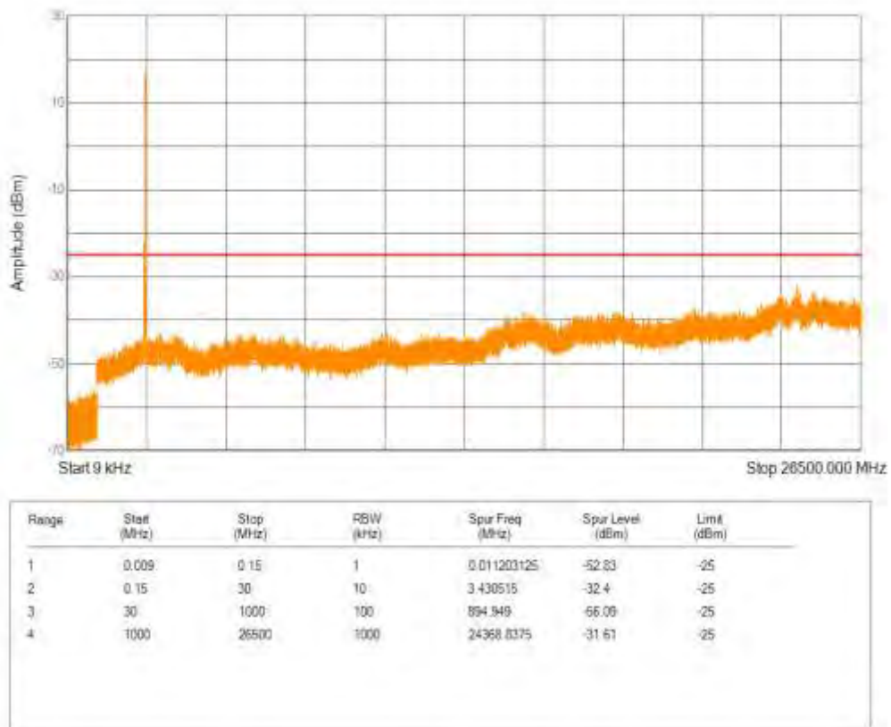
Band41(2555-2655) QPSK BW=10MHz Channel=40290 RB Size=50 Position=#0
