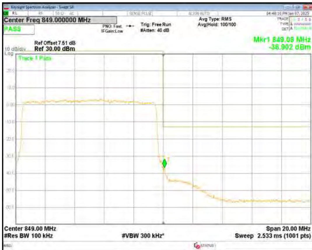
Band5 16QAM BW=3MHz Channel=20415 RB Size=15 Position=#0
