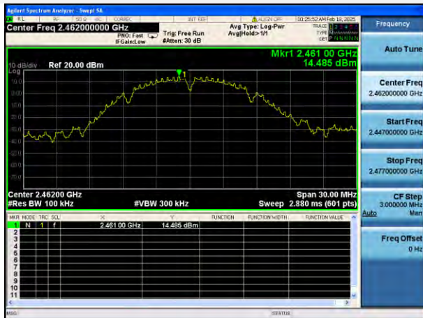
802.11b HIGH CHANNEL, CARRIER LEVEL
