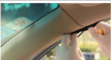
c. then insert the cable to the door's sealing tape.
