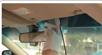
a. hide the cable into to the top panel as the photo
