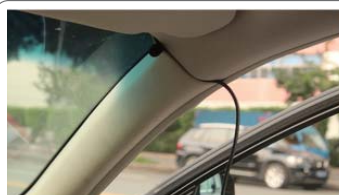
b. Break the side panel slightly and insert the cable, please be careful if there is a airbag
