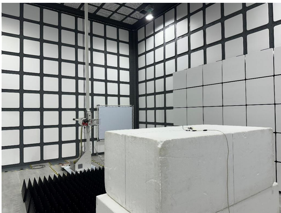
Set-up for Spurious Emissions Rear View
