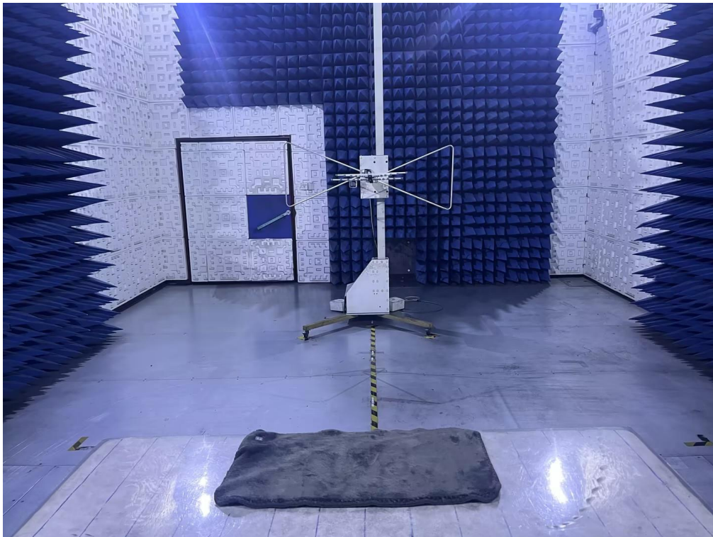
RADIATED EMISSION TEST SETUP ABOVE 1GHz
