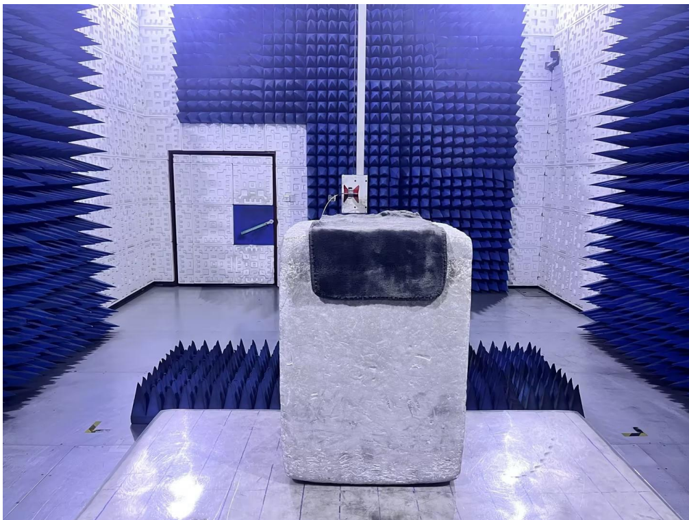
RADIATED EMISSION TEST SETUP ABOVE 1GHz
