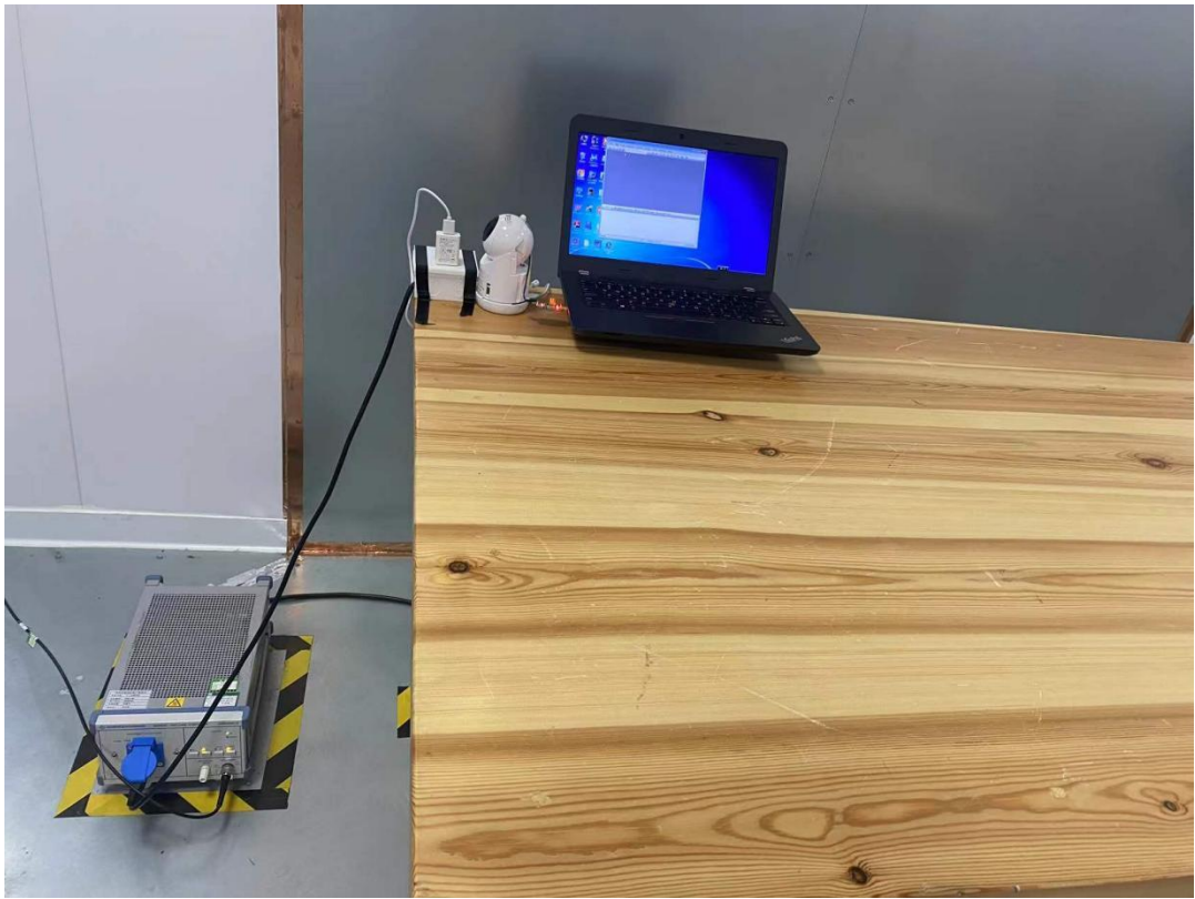
Photo of Conducted emission Test
