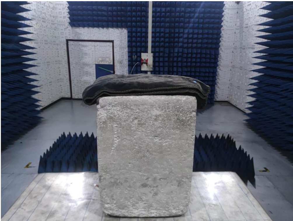
RADIATED EMISSION TEST SETUP ABOVE 1GHz
