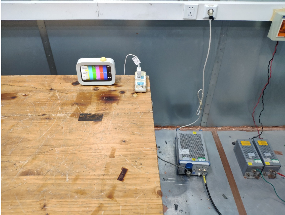
Picture 2: Conducted Emissions Test Setup
