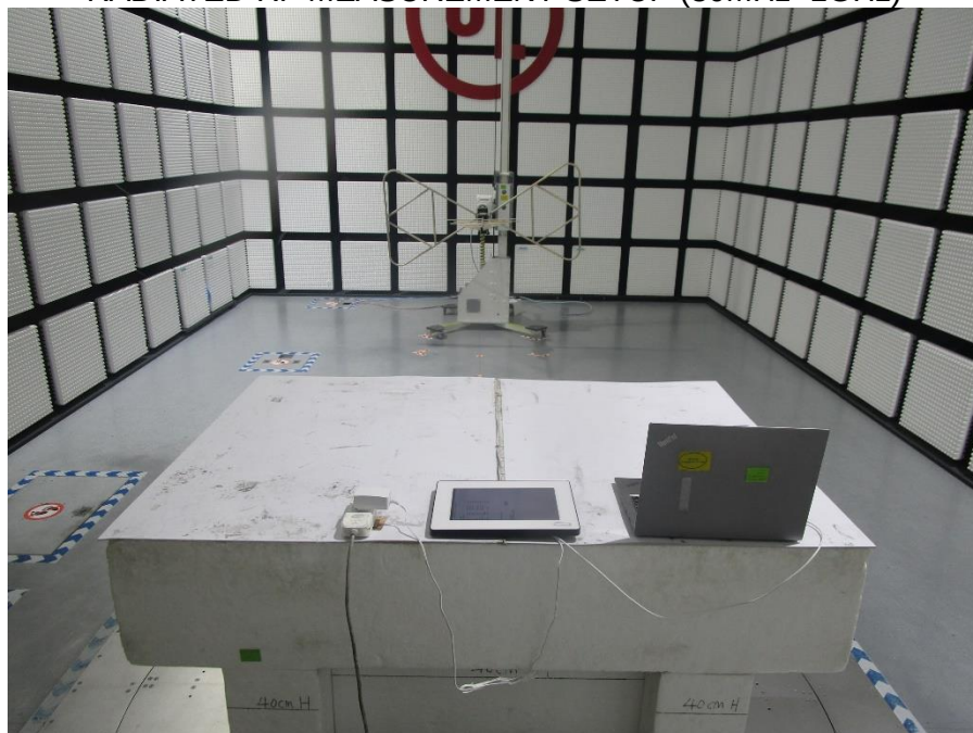
RADIATED RF MEASUREMENT SETUP (Below 30MHz)
