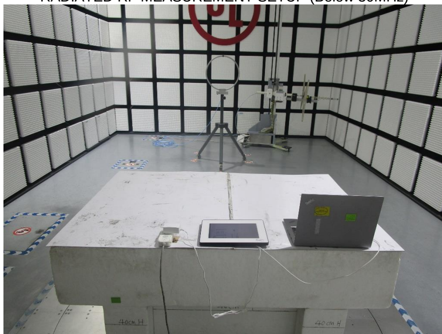
RADIATED RF MEASUREMENT SETUP (Below 30MHz)
