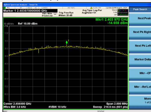
GFSK (BLE 2Mbps) LOW CHANNEL
