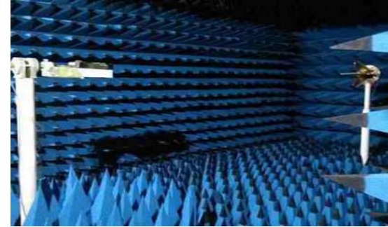
7*4*3M ETS microwave anechoic chamber
