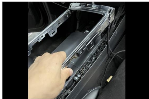
2. Remove the original central console trim
