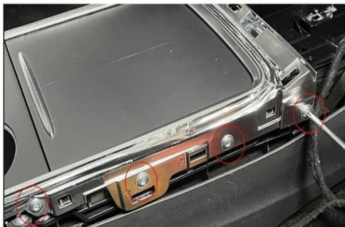
2. Remove the original central console trim
