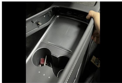
1. Pry open and remove the original central console cover plate
