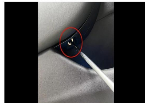
6. Remove the setscrew of rear door panel
