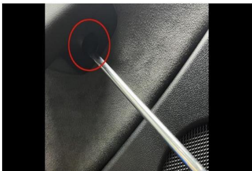
7. Remove the setscrew of rear door panel
