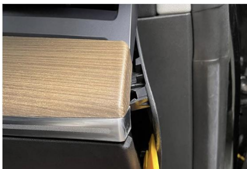
1. Pry open the cover plate of both side dashboard
