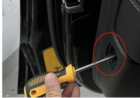
1. Remove the door panel setscrews
