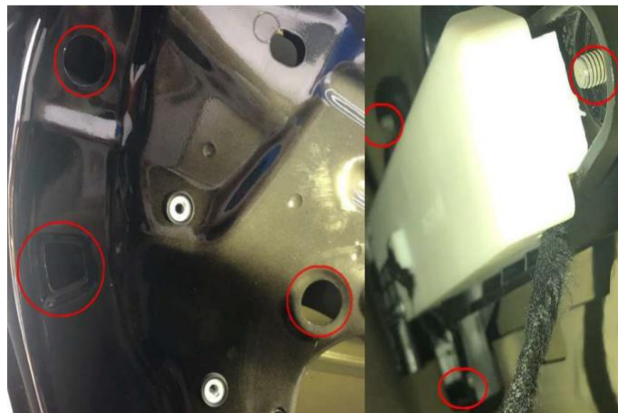
(8).取出上图三颗螺丝，拆下原车把手 Take out the three screws in the picture above and remove the original handlebar
