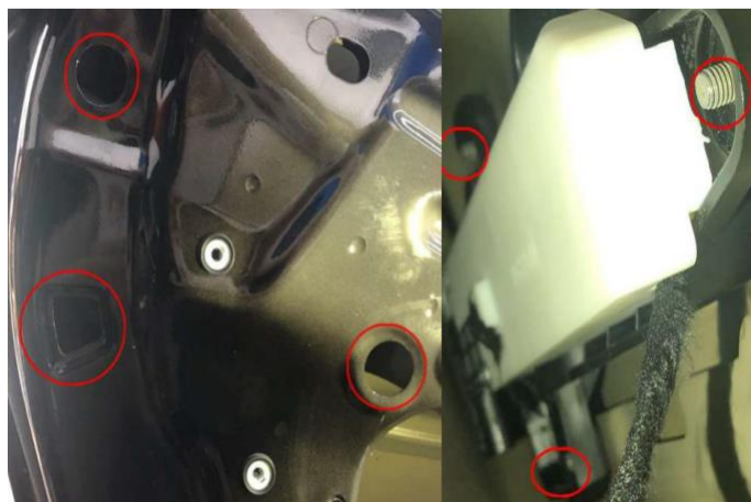
(6).取出上图三颗螺丝，拆下原车把手 Take out the three screws in the picture above and remove the original handlebar
