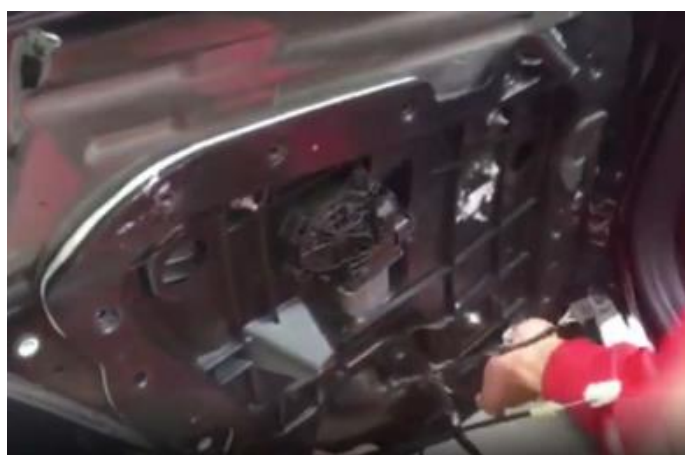
(8).把与固定饰板上连接的所有线取下,用手从固定饰板下端用力往上提的同时 往外拉出即可取下饰板 Remove all the wires connected with the fixed plate and pull out the lower plate by hand while lifting the lower end of the fixed plate forcefully
