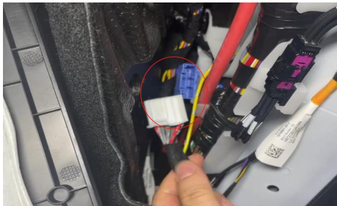
(2) 拆下副驾 A 柱饰板 CAN 线直接与蓝色插座对插 Remove co-pilot's A-pillar trim panel and plug the CAN cable directly into the blue socket
