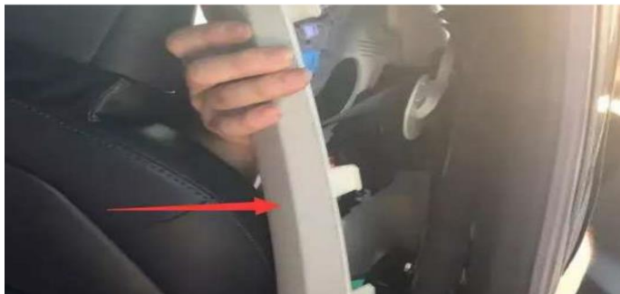
(12).拆下 B 柱上边饰板 用穿线绳将把手线从波纹管穿到车内，线材隐藏在车边沿饰板内 Remove the upper edge panel of pillar B and thread the handle line from the bellows to the inside of the car with the string, the wire is hidden in the edge panel of the car
