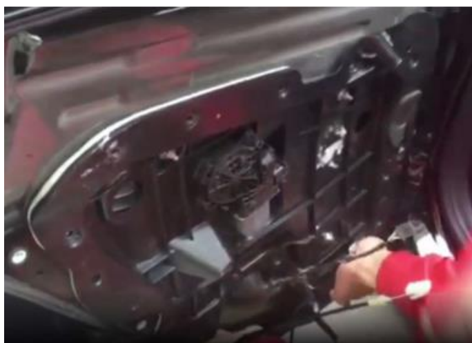
(8).把与固定饰板上连接的所有线取下，用手从固定饰板下端用力往上提的同时往外拉出即可取下饰板 (8). Remove all the wires connected with the fixed plate and pull out the lower plate by hand while lifting the lower end of the fixed plate forcefully
