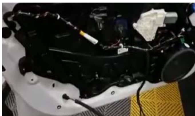
(6).拔掉与饰板相连的插头 Remove the plug connected to the trim plate
