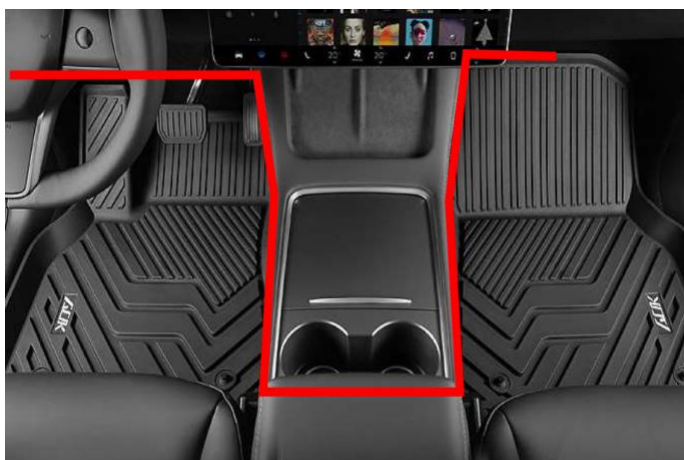
(3) 拆下马鞍两侧饰板，左侧前后门把手线材按照上图走线至副驾驶控制盒放置位置，控制盒隐藏在饰板里面 Remove the decorative plates on both sides of the saddle, and route the left front and rear door handle wire to the position of the copilot control box according to the figure above. The control box is hidden inside the decorative plate
