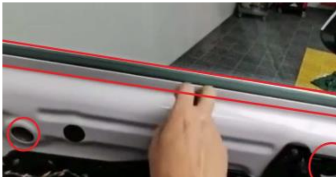
(3).拿出标示处胶条和胶塞把玻璃螺丝对上孔位 Take out the rubber strip and rubber plug at the marking point and align the glass screw with the hole
