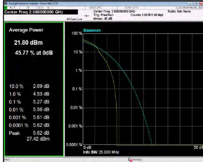
Band7 16QAM BW=5MHz Channel=20775 RB Size=1 Position=#0
