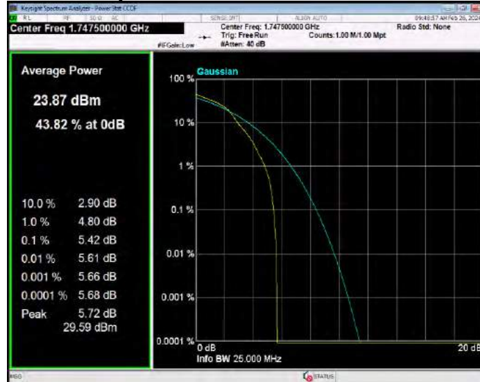
Band4 16QAM BW=20MHz Channel=20050 RB Size=1 Position=#0
