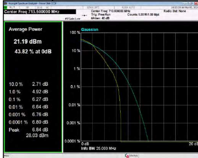
Band12 QPSK BW=1.4MHz Channel=23017 RB Size=1 Position=#0
