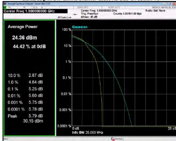
Band2 16QAM BW=3MHz Channel=18615 RB Size=1 Position=#0
