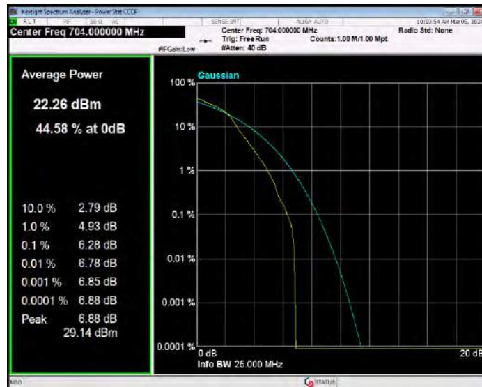
Band12 16QAM BW=10MHz Channel=23095 RB Size=1 Position=#0
