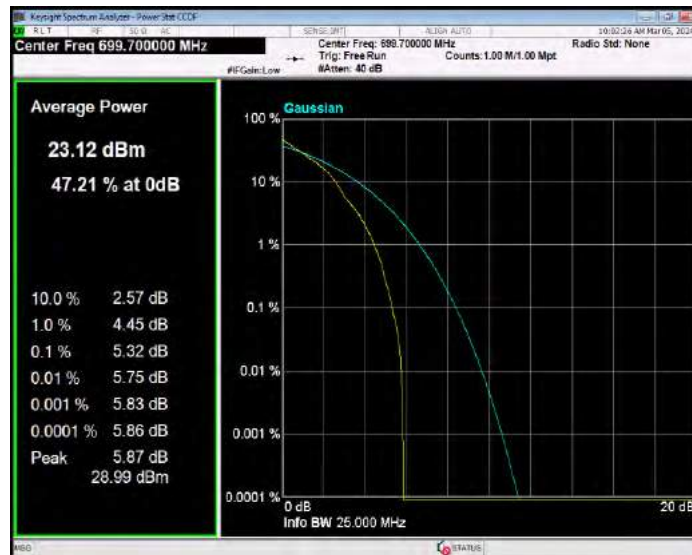
Band12 QPSK BW=1.4MHz Channel=23095 RB Size=1 Position=#0
