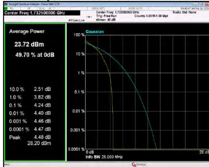
Band4 QPSK BW=15MHz Channel=20325 RB Size=1 Position=#0
