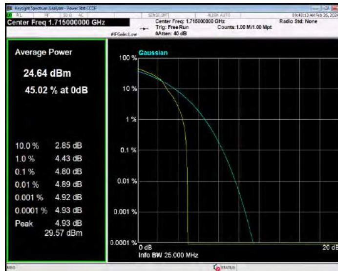
Band4 16QAM BW=10MHz Channel=20175 RB Size=1 Position=#0
