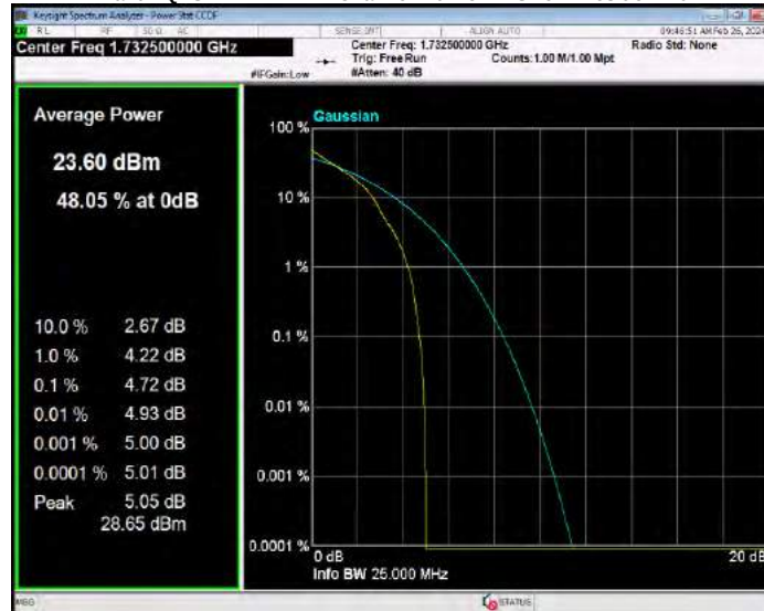
Band4 QPSK BW=1.4MHz Channel=20393 RB Size=1 Position=#0
