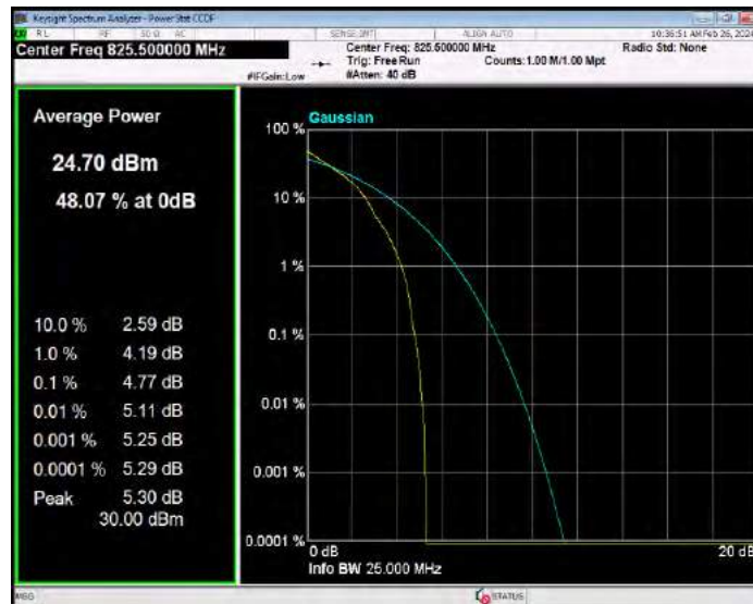
Band5 QPSK BW=3MHz Channel=20525 RB Size=1 Position=#0
