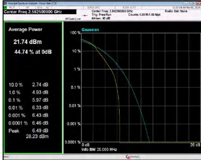
Band7 16QAM BW=20MHz Channel=20850 RB Size=1 Position=#0
