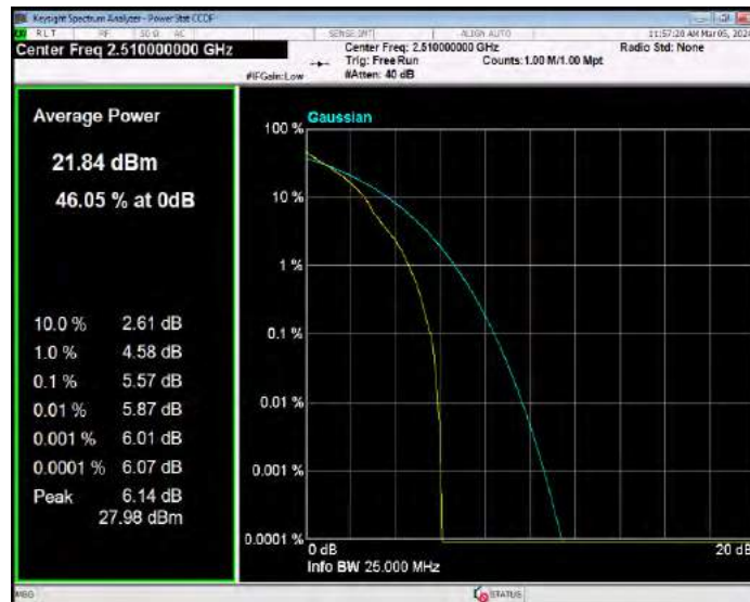
Band7 QPSK BW=20MHz Channel=21100 RB Size=1 Position=#0
