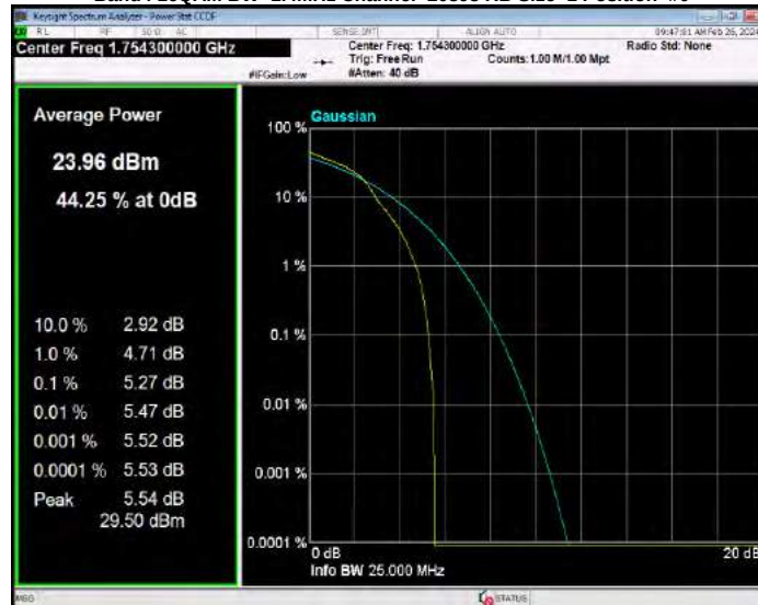
Band4 16QAM BW=10MHz Channel=20000 RB Size=1 Position=#0
