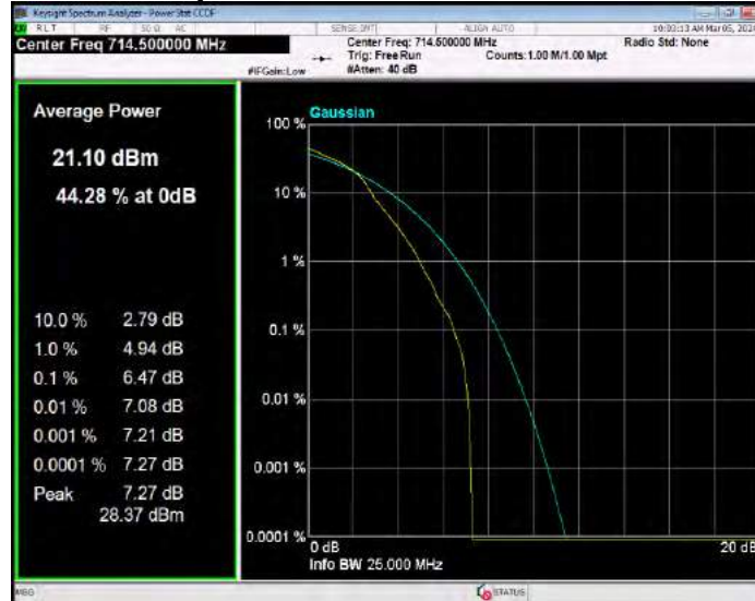
Band12 16QAM BW=5MHz Channel=23035 RB Size=1 Position=#0
