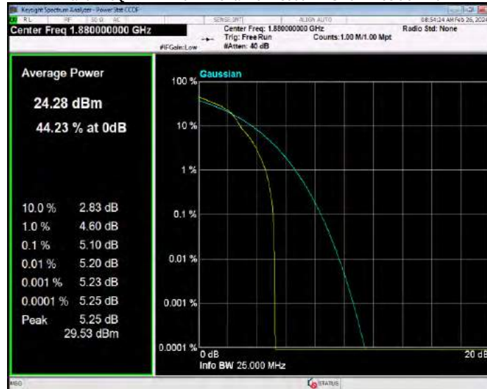
Band2 16QAM BW=20MHz Channel=19100 RB Size=1 Position=#0
