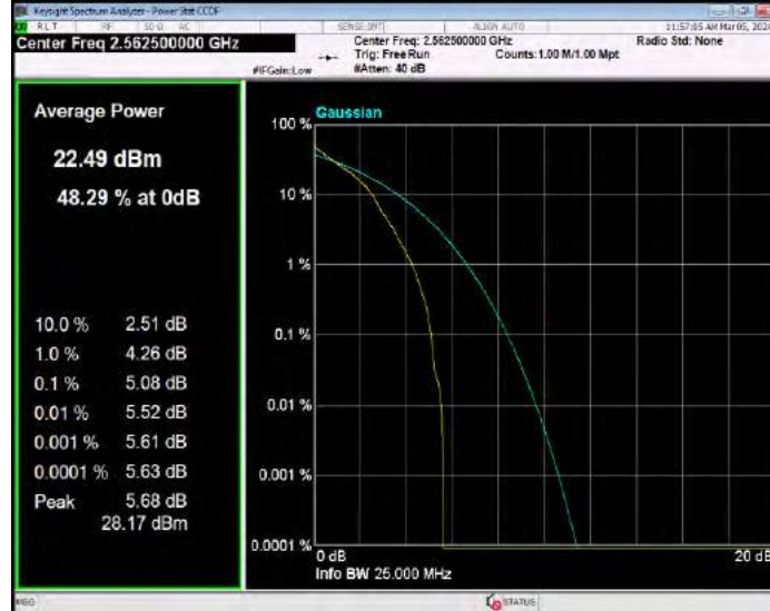
Band7 QPSK BW=20MHz Channel=20850 RB Size=1 Position=#0
