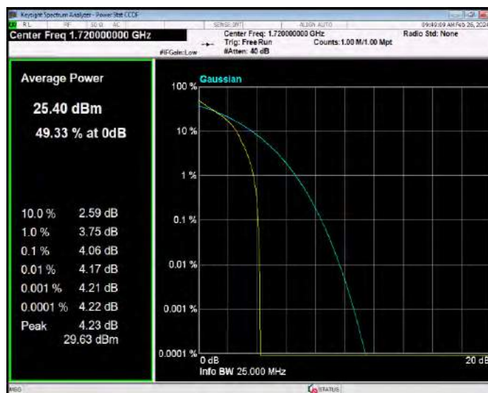
Band4 QPSK BW=20MHz Channel=20175 RB Size=1 Position=#0
