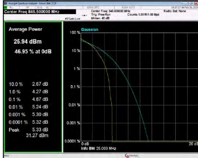
Band7 16QAM BW=10MHz Channel=20800 RB Size=1 Position=#0
