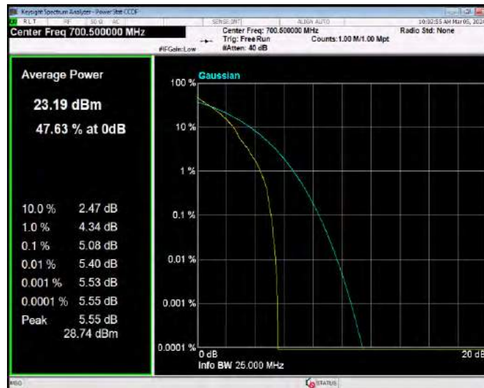
Band12 QPSK BW=3MHz Channel=23095 RB Size=1 Position=#0
