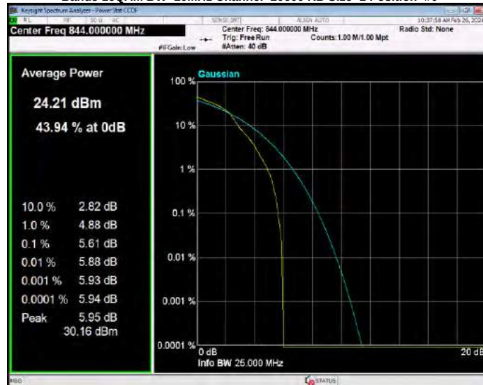
Band5 16QAM BW=3MHz Channel=20415 RB Size=1 Position=#0
