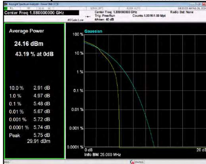
Band2 16QAM BW=15MHz Channel=19125 RB Size=1 Position=#0
