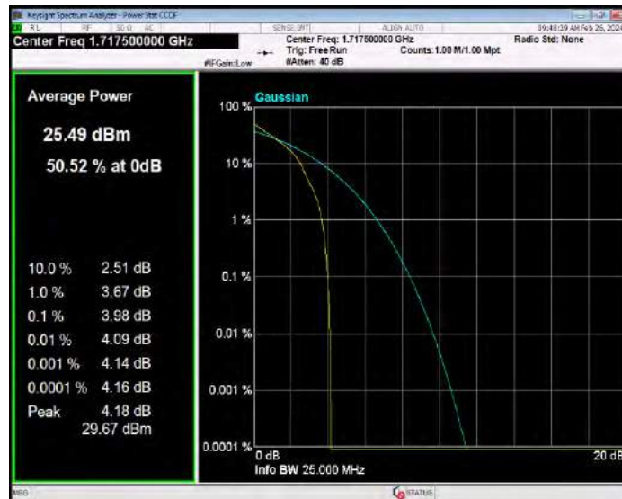
Band4 QPSK BW=15MHz Channel=20175 RB Size=1 Position=#0
