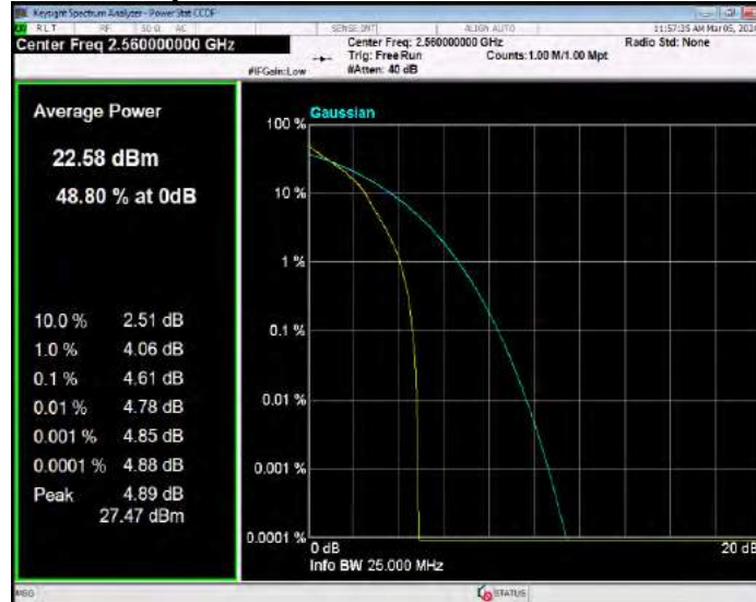
Band7 QPSK BW=5MHz Channel=20775 RB Size=1 Position=#0
