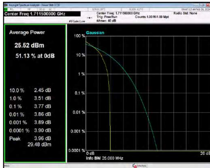
Band4 QPSK BW=3MHz Channel=20175 RB Size=1 Position=#0
