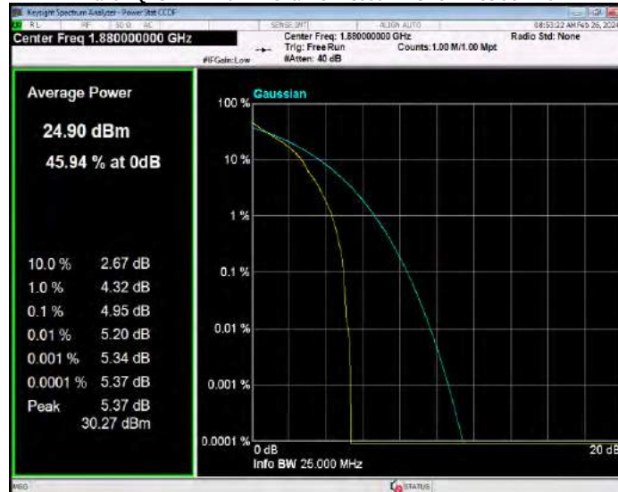
Band2 QPSK BW=10MHz Channel=19150 RB Size=1 Position=#0
