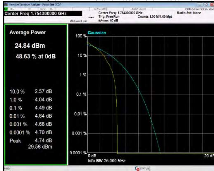
Band4 QPSK BW=10MHz Channel=20000 RB Size=1 Position=#0
