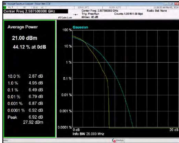
Band7 16QAM BW=15MHz Channel=21100 RB Size=1 Position=#0
