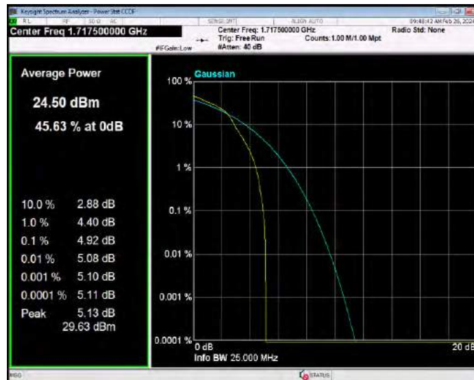
Band4 16QAM BW=15MHz Channel=20175 RB Size=1 Position=#0
