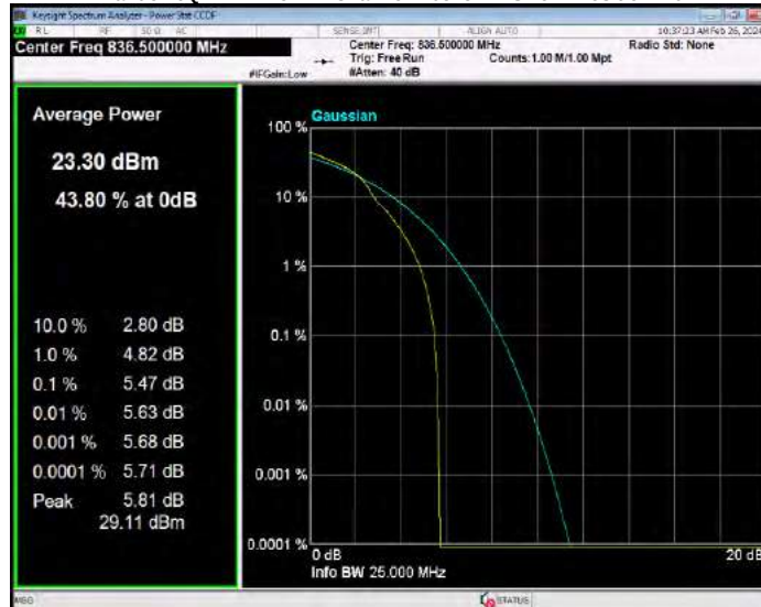
Band5 16QAM BW=5MHz Channel=20625 RB Size=1 Position=#0
