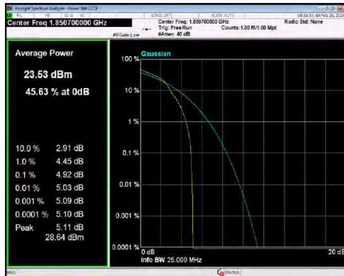
Band2 16QAM BW=1.4MHz Channel=18900 RB Size=1 Position=#0
