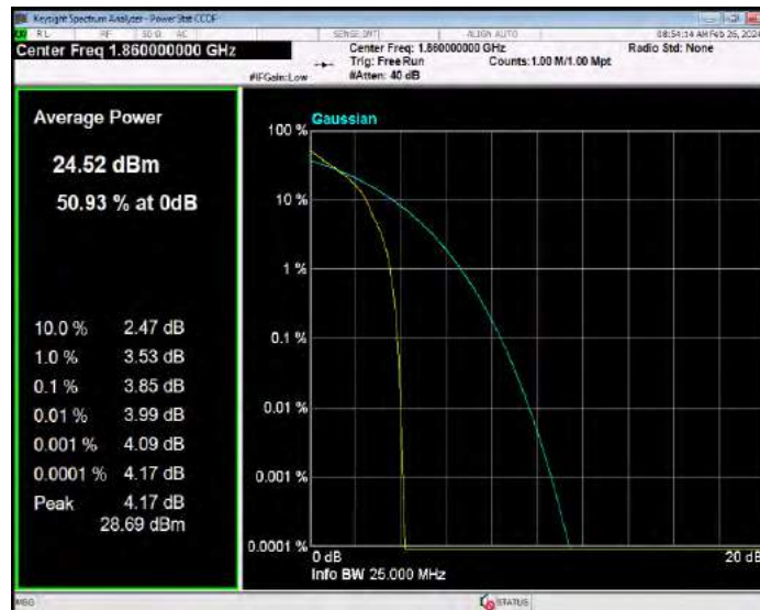
Band2 QPSK BW=20MHz Channel=18900 RB Size=1 Position=#0
