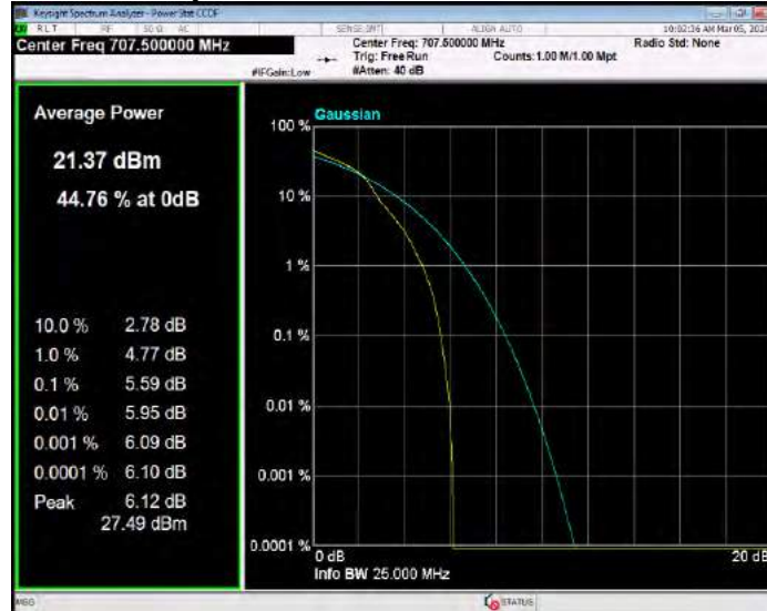
Band12 16QAM BW=1.4MHz Channel=23173 RB Size=1 Position=#0
