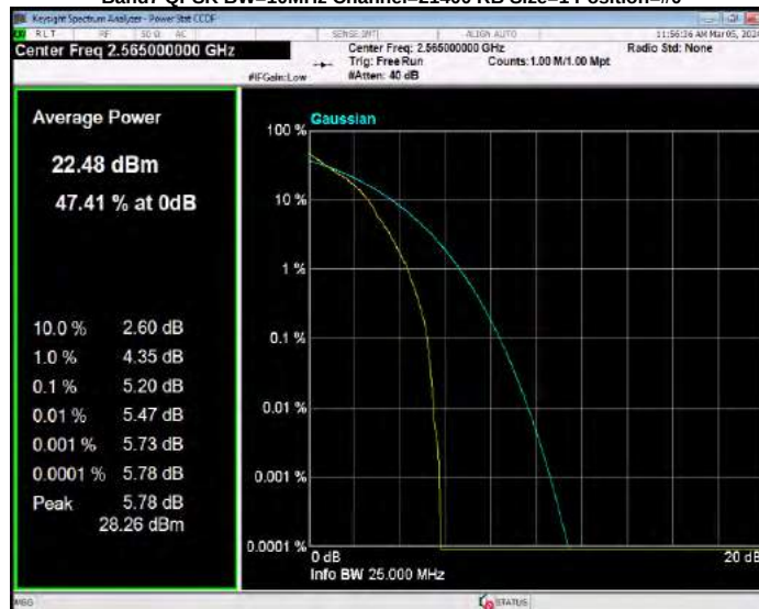
Band7 QPSK BW=15MHz Channel=20825 RB Size=1 Position=#0
