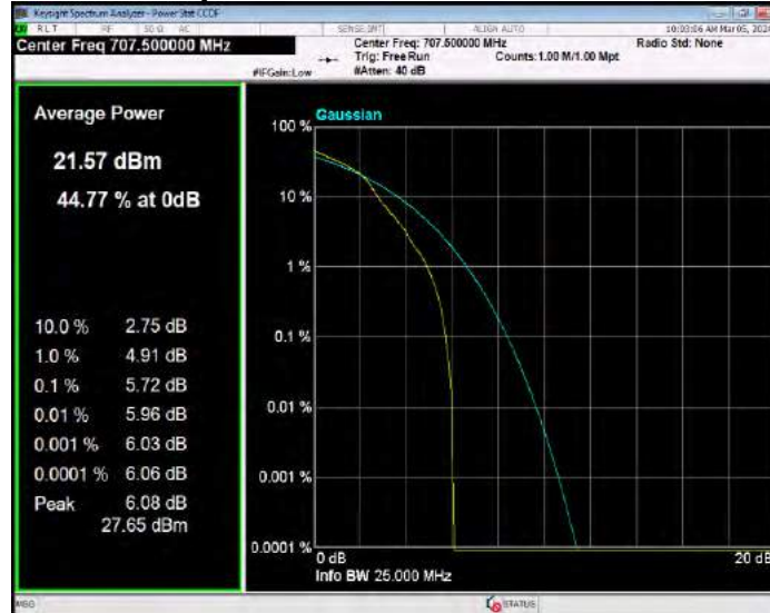
Band12 16QAM BW=3MHz Channel=23165 RB Size=1 Position=#0
