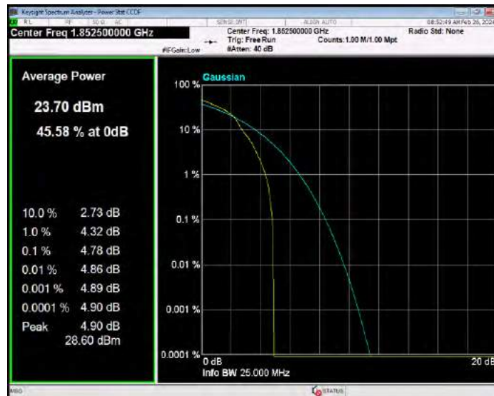
Band2 16QAM BW=5MHz Channel=18900 RB Size=1 Position=#0
