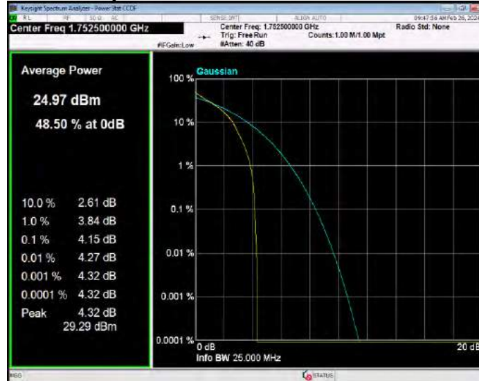
Band5 16QAM BW=1.4MHz Channel=20407 RB Size=1 Position=#0
