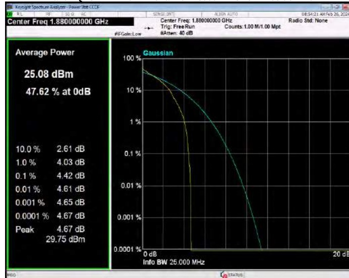
Band2 QPSK BW=20MHz Channel=19100 RB Size=1 Position=#0
