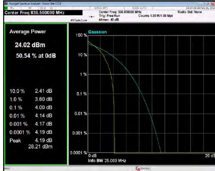
Band5 QPSK BW=10MHz Channel=20600 RB Size=1 Position=#0
