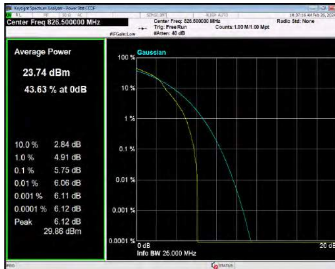
Band5 16QAM BW=5MHz Channel=20525 RB Size=1 Position=#0
