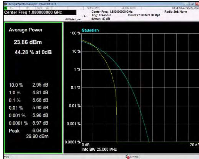
Band2 16QAM BW=1.4MHz Channel=19193 RB Size=1 Position=#0
