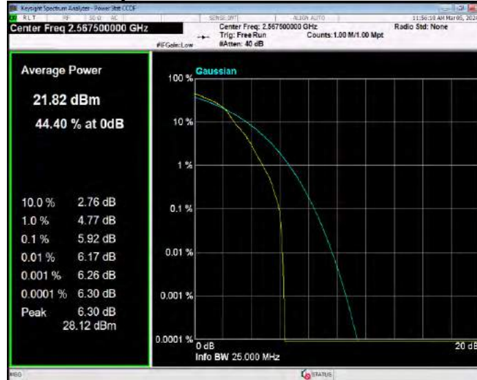
Band7 QPSK BW=10MHz Channel=20800 RB Size=1 Position=#0
