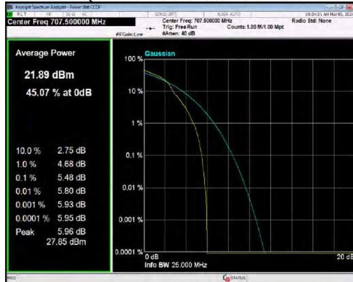
Band12 16QAM BW=10MHz Channel=23130 RB Size=1 Position=#0
