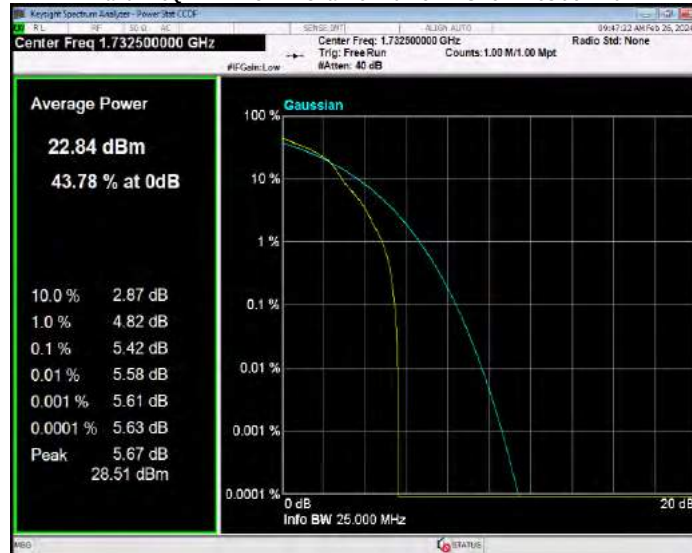
Band4 16QAM BW=3MHz Channel=20385 RB Size=1 Position=#0
