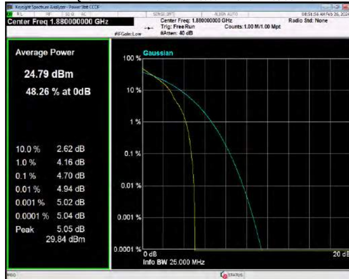
Band2 QPSK BW=1.4MHz Channel=19193 RB Size=1 Position=#0
