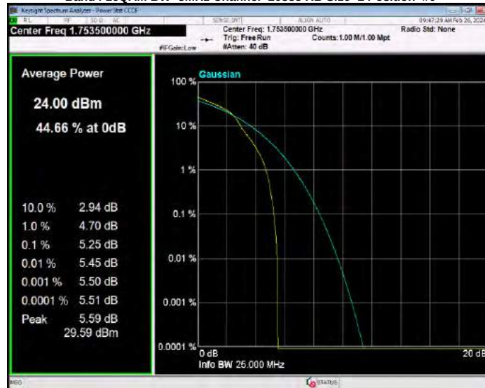
Band4 16QAM BW=5MHz Channel=19975 RB Size=1 Position=#0
