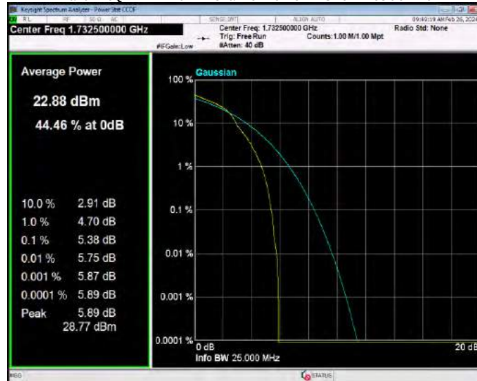
Band4 16QAM BW=20MHz Channel=20300 RB Size=1 Position=#0
