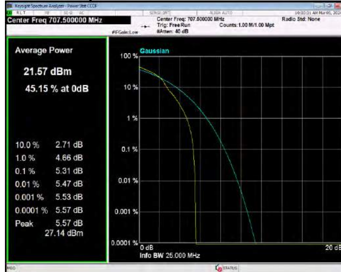
Band12 16QAM BW=5MHz Channel=23155 RB Size=1 Position=#0
