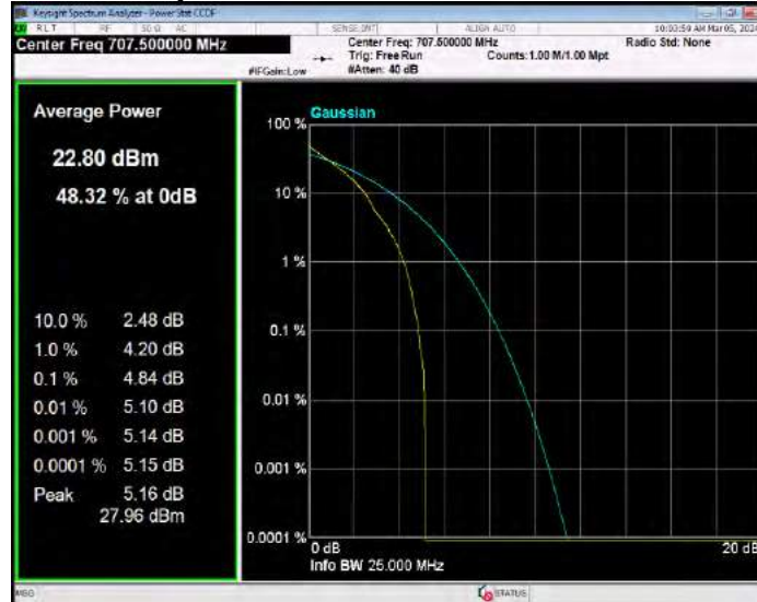
Band12 QPSK BW=10MHz Channel=23130 RB Size=1 Position=#0
