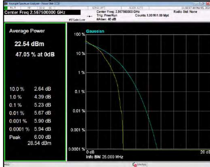
Band12 16QAM BW=1.4MHz Channel=23017 RB Size=1 Position=#0
