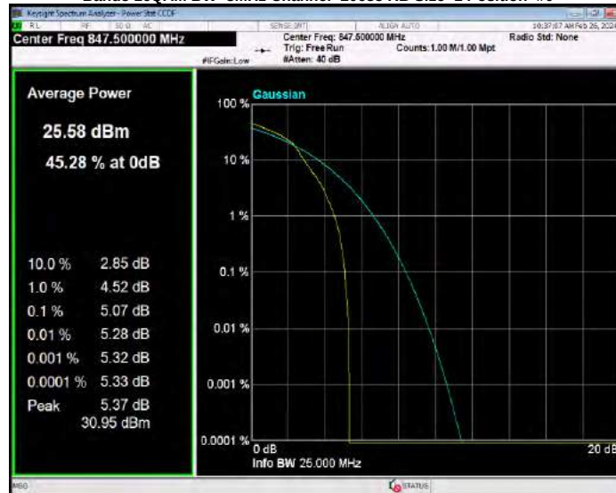
Band5 16QAM BW=5MHz Channel=20425 RB Size=1 Position=#0
