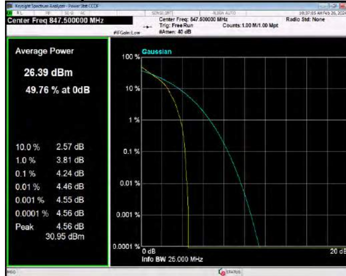
Band5 QPSK BW=5MHz Channel=20425 RB Size=1 Position=#0
