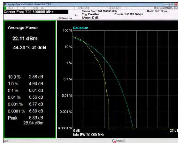
Band12 16QAM BW=5MHz Channel=23095 RB Size=1 Position=#0
