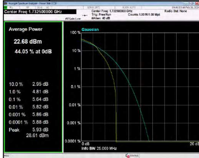
Band4 16QAM BW=1.4MHz Channel=20393 RB Size=1 Position=#0
