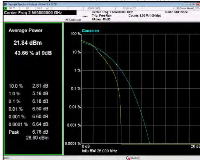
Band7 16QAM BW=15MHz Channel=20825 RB Size=1 Position=#0
