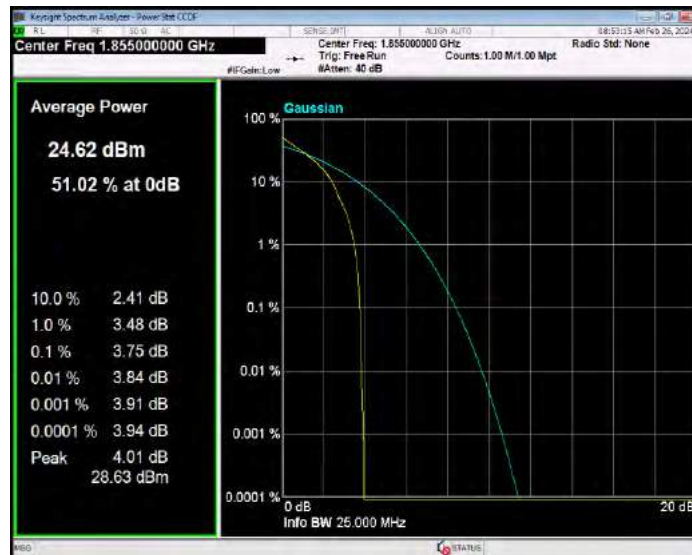
Band2 QPSK BW=10MHz Channel=18900 RB Size=1 Position=#0
