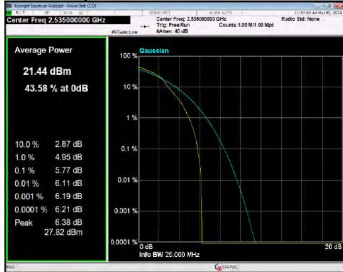
Band7 16QAM BW=15MHz Channel=21375 RB Size=1 Position=#0
