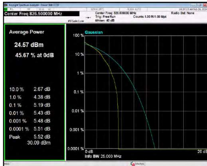
Band5 QPSK BW=5MHz Channel=20525 RB Size=1 Position=#0
