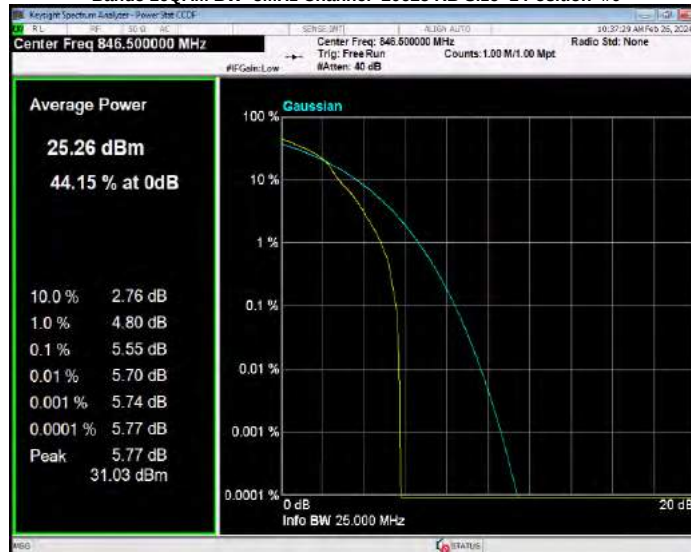
Band5 QPSK BW=1.4MHz Channel=20407 RB Size=1 Position=#0
