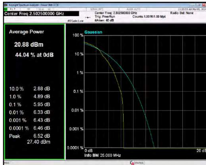
Band7 16QAM BW=5MHz Channel=21100 RB Size=1 Position=#0
