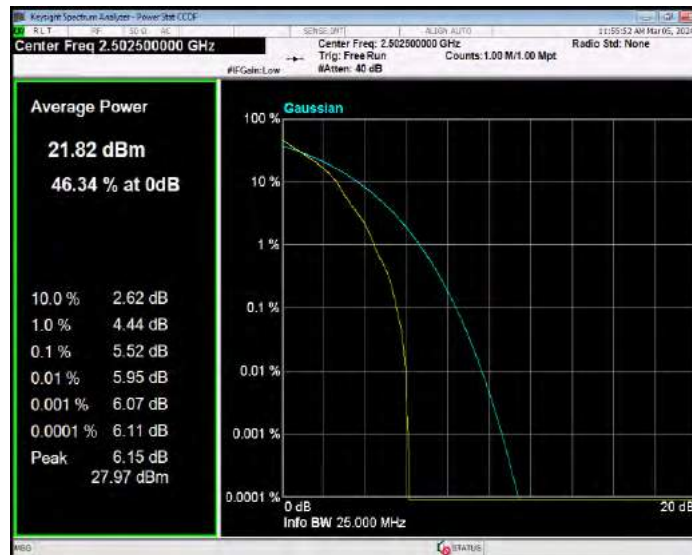
Band7 QPSK BW=5MHz Channel=21100 RB Size=1 Position=#0
