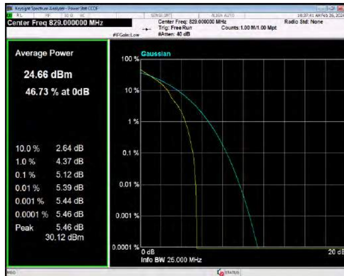
Band5 QPSK BW=10MHz Channel=20525 RB Size=1 Position=#0
