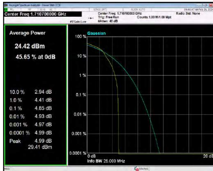
Band4 16QAM BW=1.4MHz Channel=20175 RB Size=1 Position=#0
