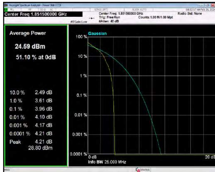
Band2 QPSK BW=3MHz Channel=18900 RB Size=1 Position=#0
