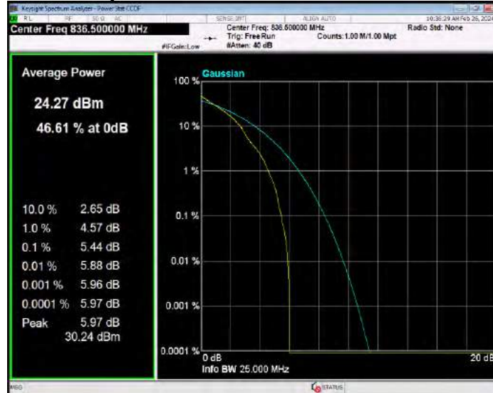
Band5 QPSK BW=1.4MHz Channel=20643 RB Size=1 Position=#0
