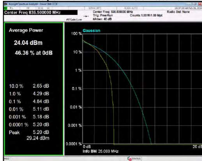
Band5 QPSK BW=5MHz Channel=20625 RB Size=1 Position=#0
