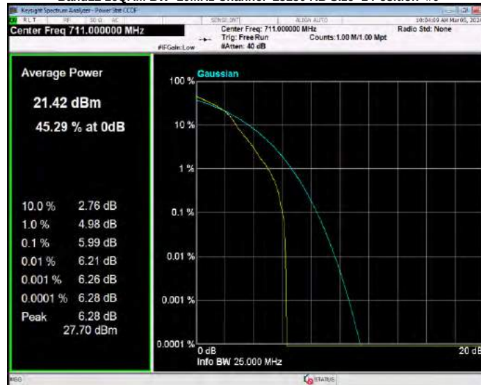
Band12 16QAM BW=3MHz Channel=23025 RB Size=1 Position=#0
