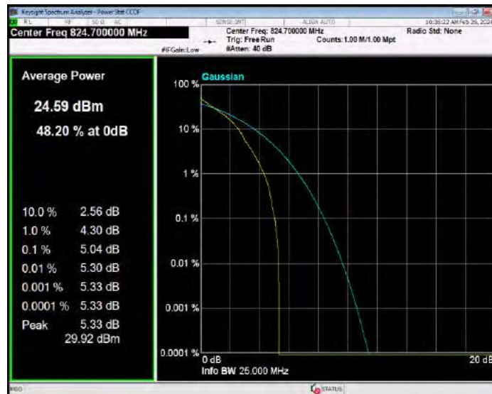
Band5 QPSK BW=1.4MHz Channel=20525 RB Size=1 Position=#0
