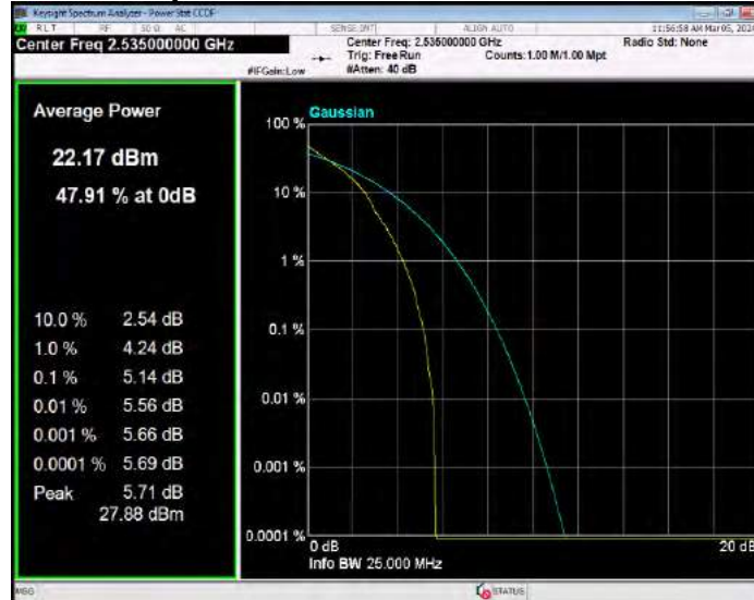
Band7 QPSK BW=15MHz Channel=21375 RB Size=1 Position=#0
