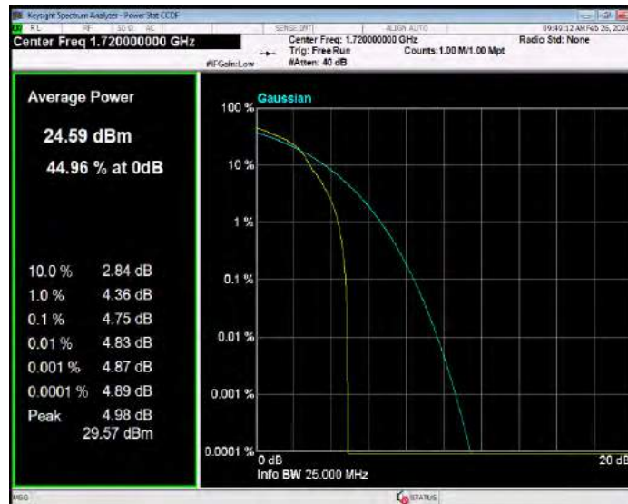
Band4 16QAM BW=20MHz Channel=20175 RB Size=1 Position=#0
