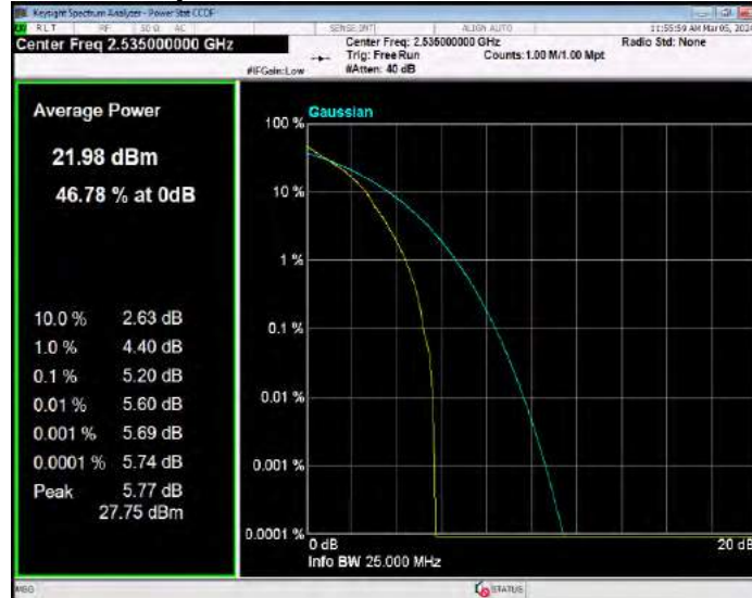
Band7 QPSK BW=5MHz Channel=21425 RB Size=1 Position=#0
