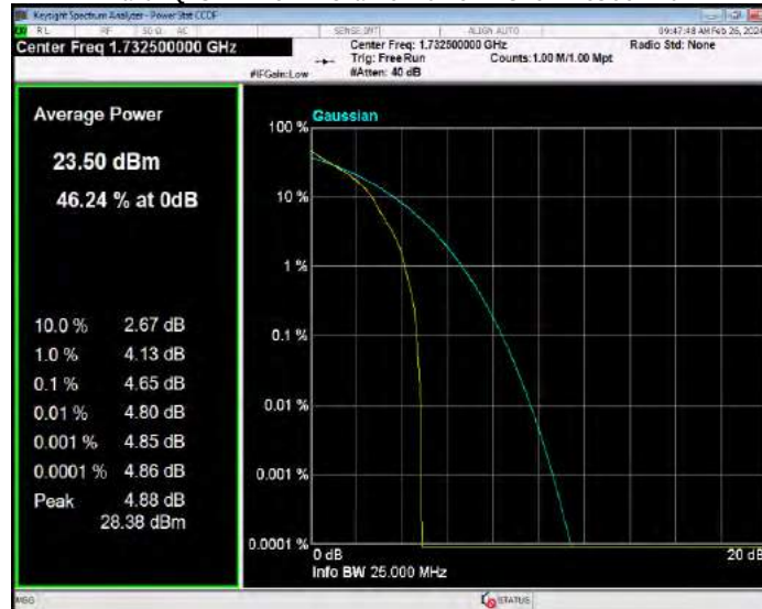
Band4 QPSK BW=5MHz Channel=20375 RB Size=1 Position=#0
