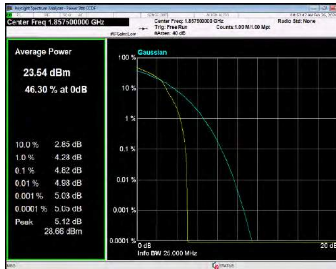
Band2 16QAM BW=15MHz Channel=18900 RB Size=1 Position=#0
