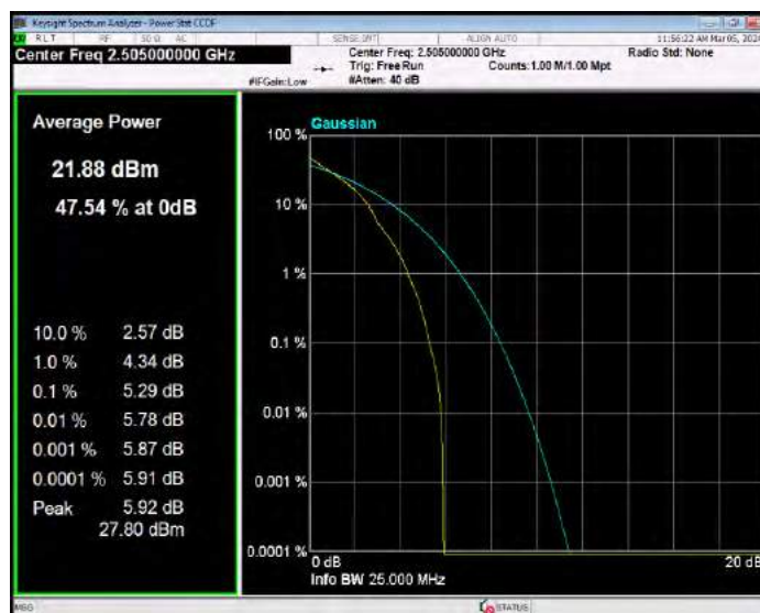
Band7 QPSK BW=10MHz Channel=21100 RB Size=1 Position=#0
