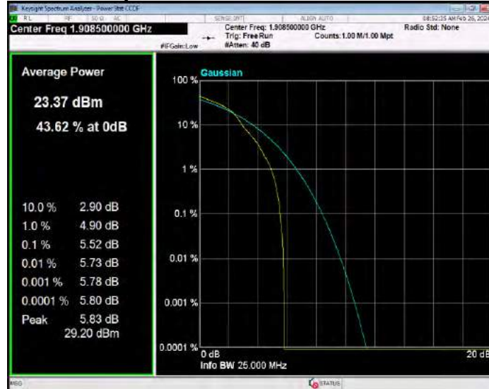
Band2 16QAM BW=5MHz Channel=18625 RB Size=1 Position=#0
