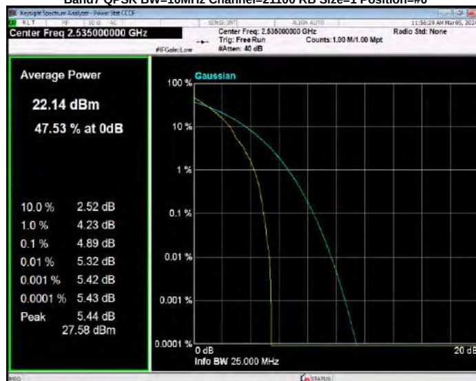
Band7 QPSK BW=10MHz Channel=21400 RB Size=1 Position=#0
