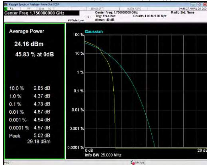
Band4 16QAM BW=15MHz Channel=20025 RB Size=1 Position=#0
