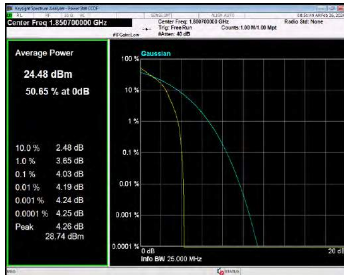
Band2 QPSK BW=1.4MHz Channel=18900 RB Size=1 Position=#0
