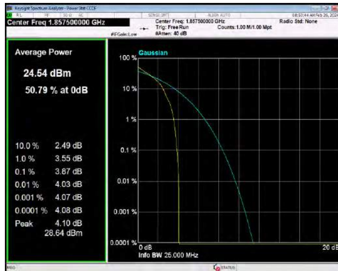
Band2 QPSK BW=15MHz Channel=18900 RB Size=1 Position=#0
