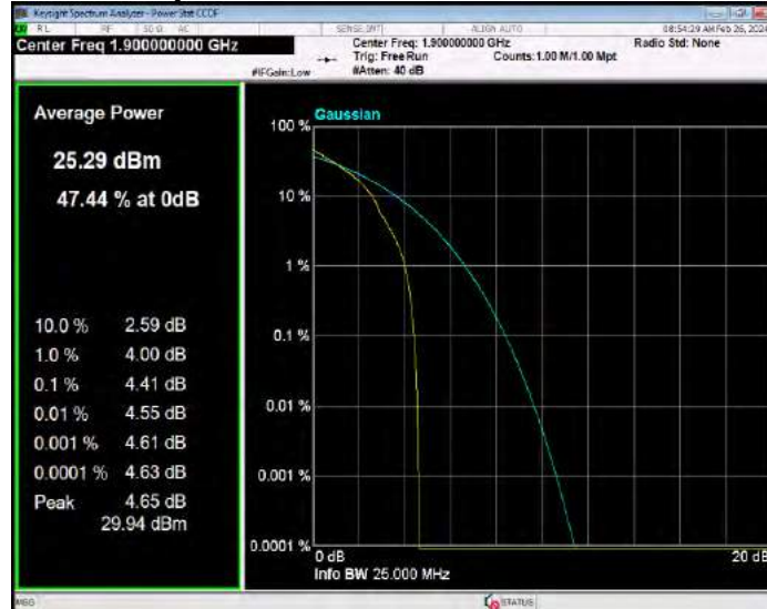
Band2 QPSK BW=3MHz Channel=18615 RB Size=1 Position=#0
