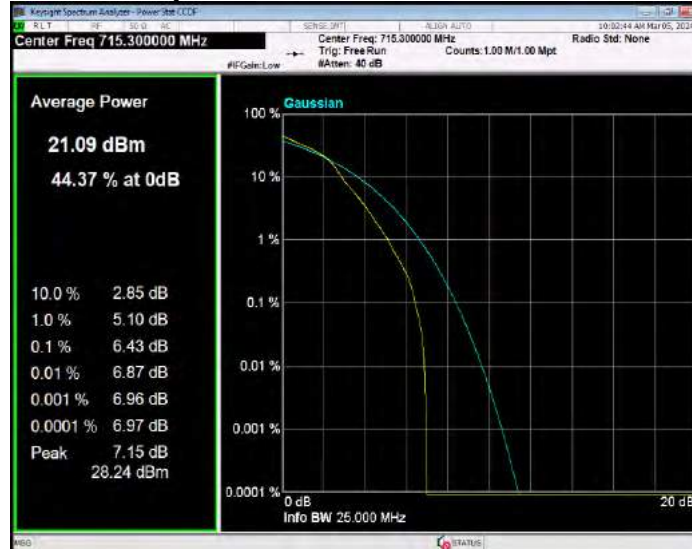
Band12 16QAM BW=10MHz Channel=23060 RB Size=1 Position=#0
