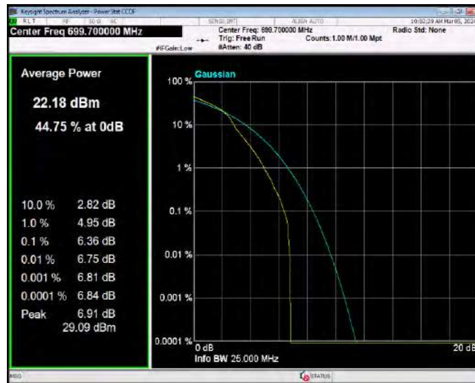
Band12 16QAM BW=1.4MHz Channel=23095 RB Size=1 Position=#0
