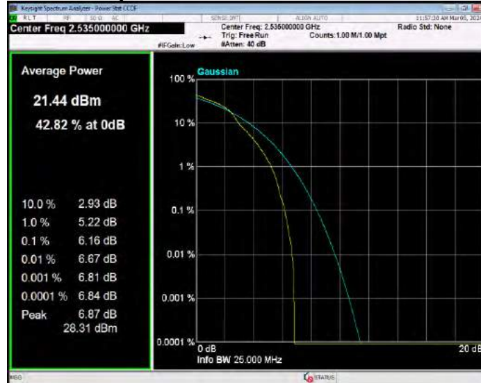
Band7 16QAM BW=20MHz Channel=21350 RB Size=1 Position=#0
