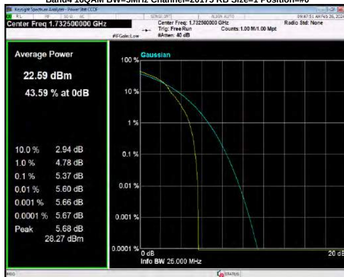
Band4 16QAM BW=5MHz Channel=20375 RB Size=1 Position=#0
