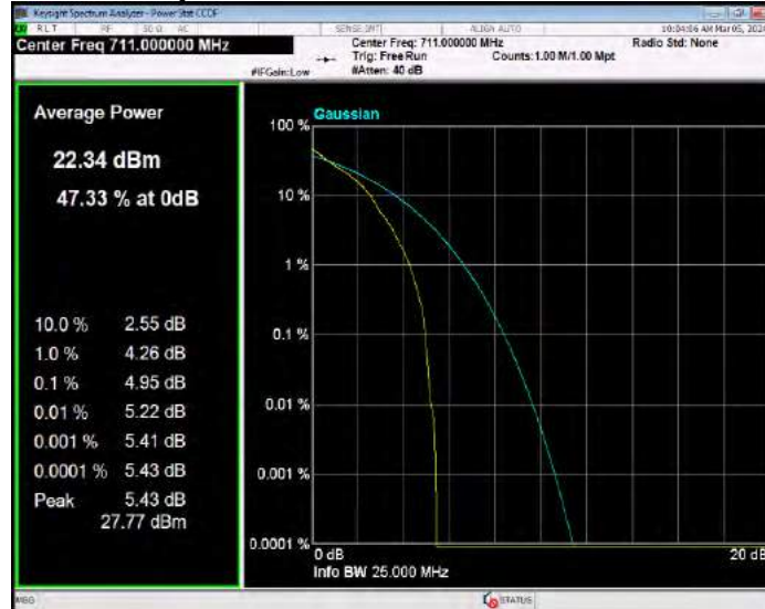
Band12 QPSK BW=3MHz Channel=23025 RB Size=1 Position=#0
