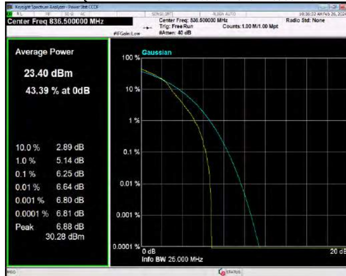
Band5 16QAM BW=1.4MHz Channel=20643 RB Size=1 Position=#0
