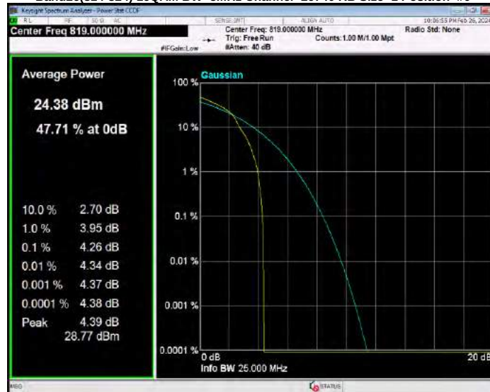
Band26(814-824) 16QAM BW=5MHz Channel=26765 RB Size=1 Position=#0
