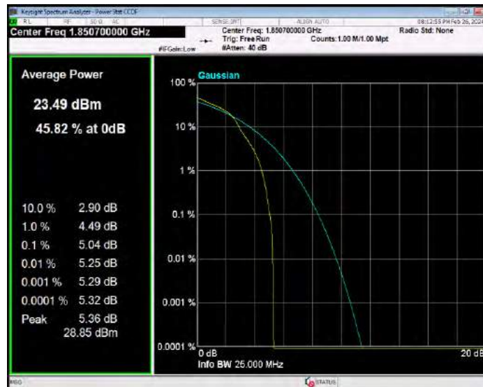
Band25 16QAM BW=1.4MHz Channel=26365 RB Size=1 Position=#0
