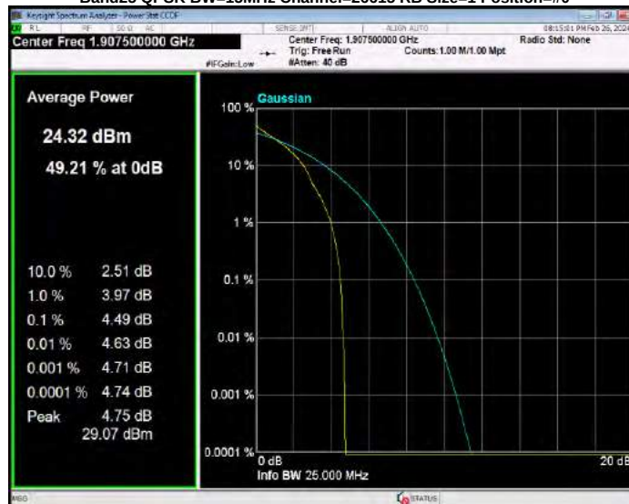
Band25 QPSK BW=20MHz Channel=26140 RB Size=1 Position=#0
