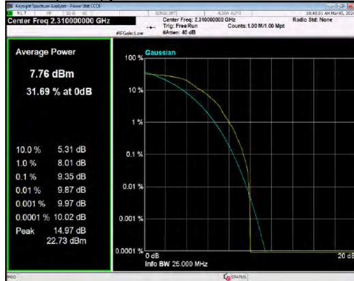
Band40(2305-2315) QPSK BW=5MHz Channel=38775 RB Size=1 Position=#0
