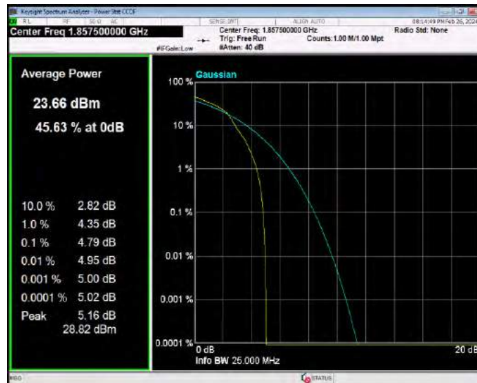
Band25 16QAM BW=15MHz Channel=26365 RB Size=1 Position=#0
