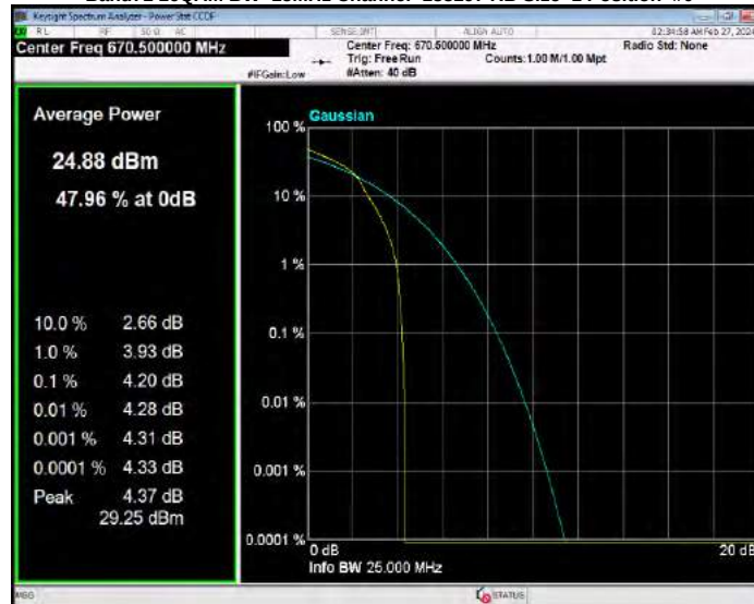
Band71 16QAM BW=15MHz Channel=133297 RB Size=1 Position=#0
