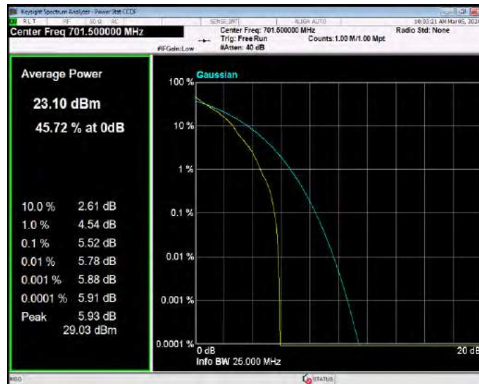
Band12 QPSK BW=5MHz Channel=23095 RB Size=1 Position=#0
