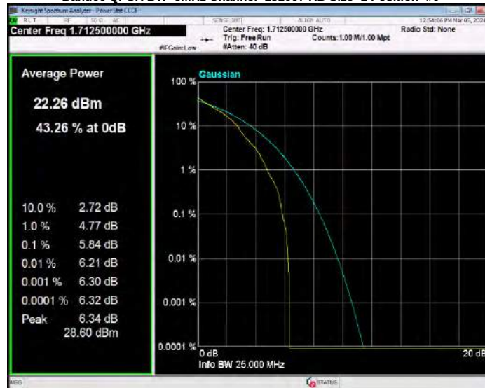
Band66 QPSK BW=5MHz Channel=132322 RB Size=1 Position=#0
