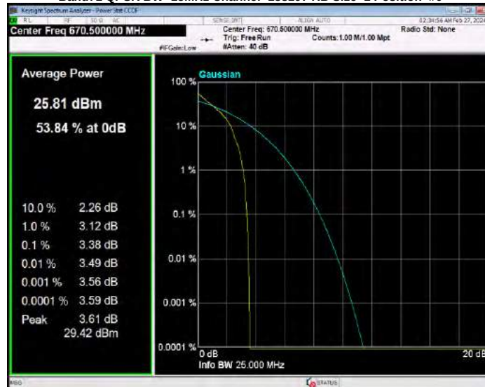
Band71 QPSK BW=15MHz Channel=133297 RB Size=1 Position=#0
