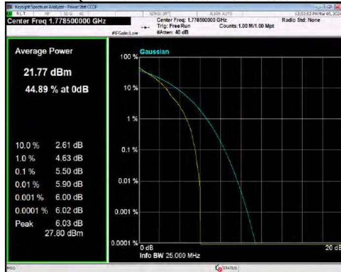
Band66 QPSK BW=5MHz Channel=131997 RB Size=1 Position=#0
