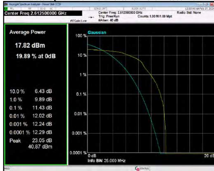
Band38 16QAM BW=20MHz Channel=37850 RB Size=1 Position=#0
