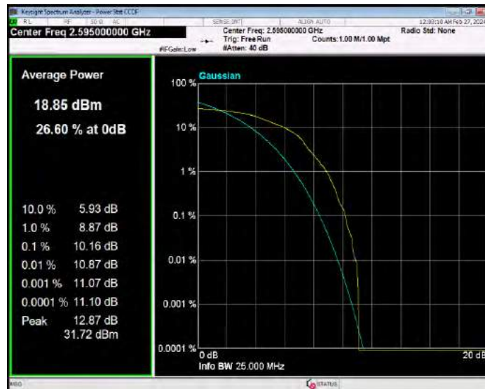
Band38 16QAM BW=10MHz Channel=38200 RB Size=1 Position=#0
