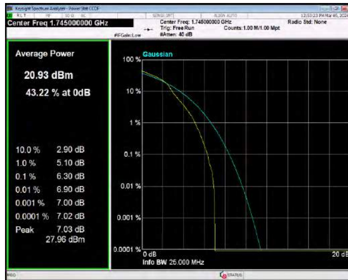
Band66 16QAM BW=1.4MHz Channel=132665 RB Size=1 Position=#0
