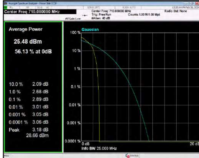
Band17 QPSK BW=10MHz Channel=23800 RB Size=1 Position=#0
