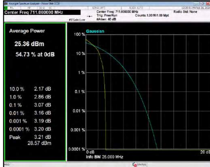
Band17 QPSK BW=5MHz Channel=23755 RB Size=1 Position=#0
