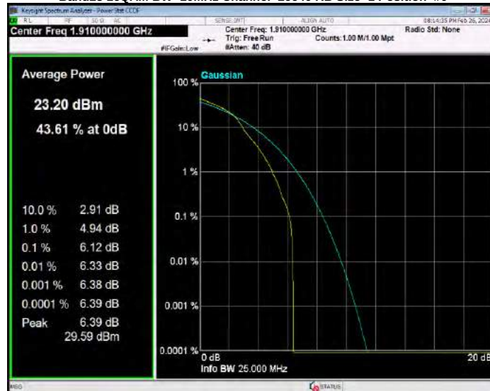
Band25 16QAM BW=15MHz Channel=26115 RB Size=1 Position=#0
