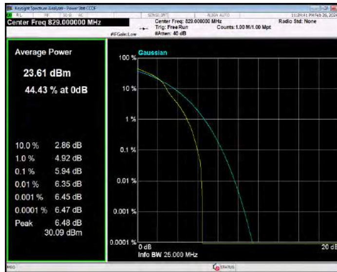
Band26(824-849) 16QAM BW=10MHz Channel=26915 RB Size=1 Position=#0
