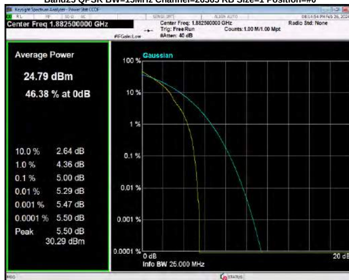
Band25 QPSK BW=15MHz Channel=26615 RB Size=1 Position=#0
