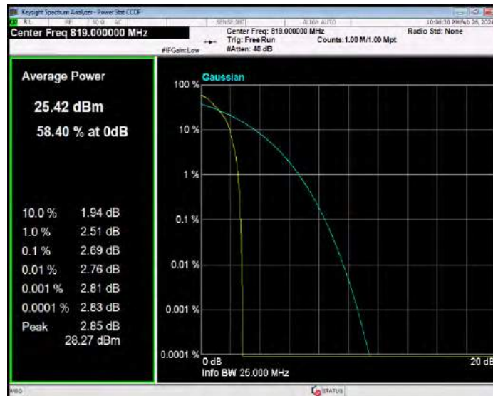
Band26(814-824) QPSK BW=3MHz Channel=26775 RB Size=1 Position=#0
