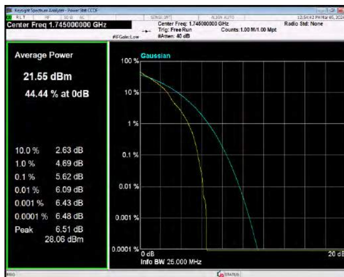
Band66 QPSK BW=10MHz Channel=132622 RB Size=1 Position=#0
