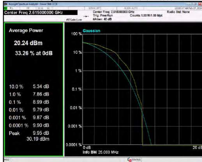
Band38 16QAM BW=15MHz Channel=37825 RB Size=1 Position=#0
