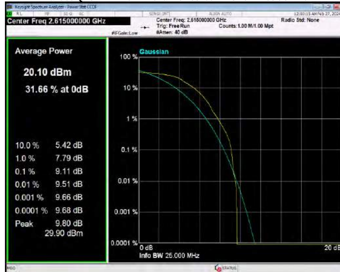
Band38 QPSK BW=15MHz Channel=37825 RB Size=1 Position=#0
