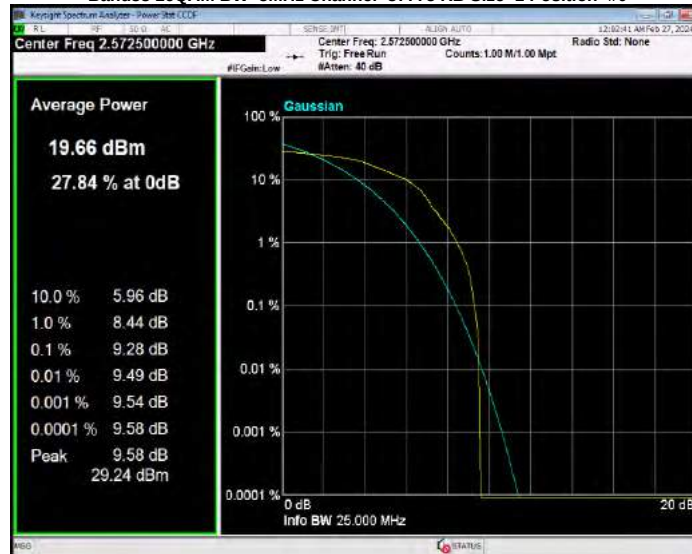
Band38 16QAM BW=5MHz Channel=38000 RB Size=1 Position=#0
