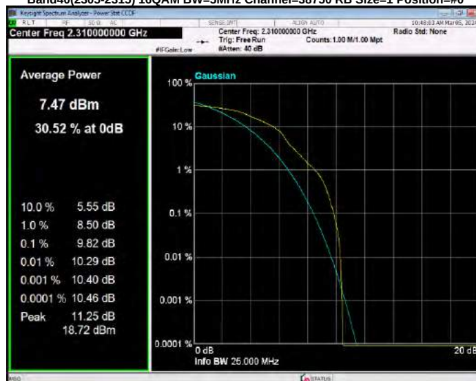
Band40(2305-2315) 16QAM BW=5MHz Channel=38775 RB Size=1 Position=#0
