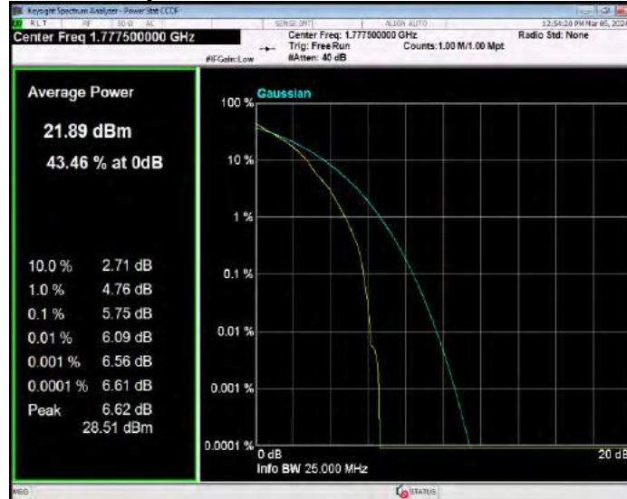
Band71 16QAM BW=10MHz Channel=133172 RB Size=1 Position=#0
