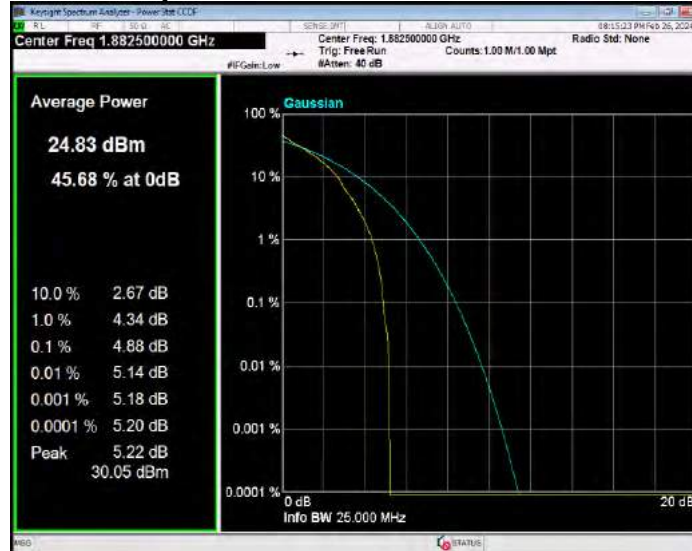
Band25 QPSK BW=20MHz Channel=26590 RB Size=1 Position=#0
