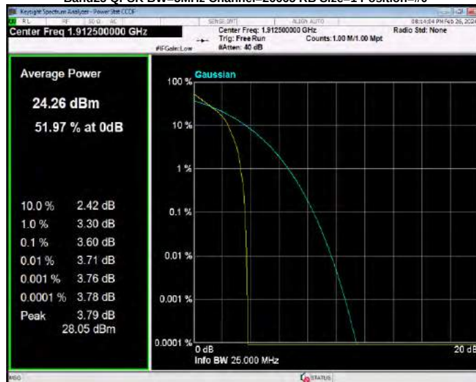
Band26(824-849) 16QAM BW=1.4MHz Channel=26797 RB Size=1 Position=#0
