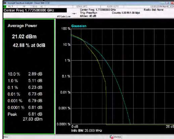
Band66 16QAM BW=20MHz Channel=132072 RB Size=1 Position=#0
