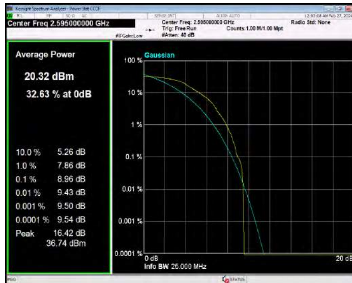
Band38 QPSK BW=10MHz Channel=38200 RB Size=1 Position=#0
