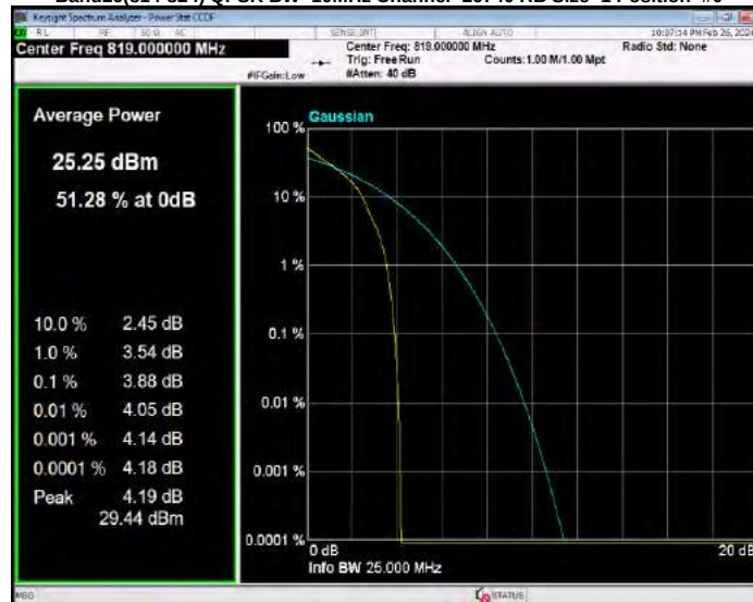
Band26(814-824) QPSK BW=3MHz Channel=26705 RB Size=1 Position=#0
