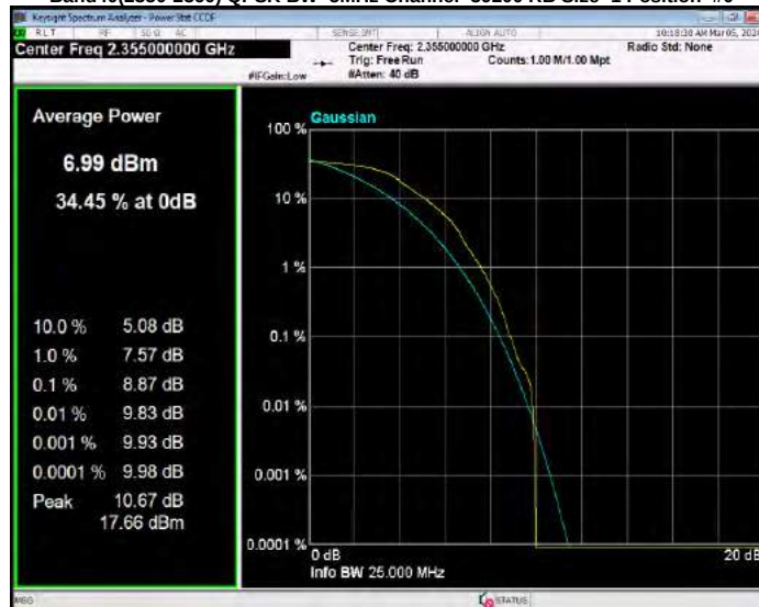
Band40(2350-2360) QPSK BW=5MHz Channel=39225 RB Size=1 Position=#0
