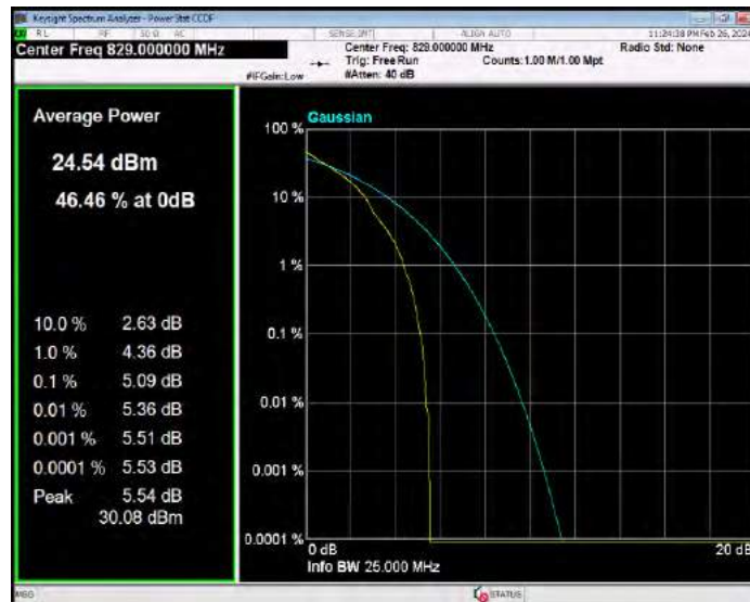
Band26(824-849) QPSK BW=10MHz Channel=26915 RB Size=1 Position=#0
