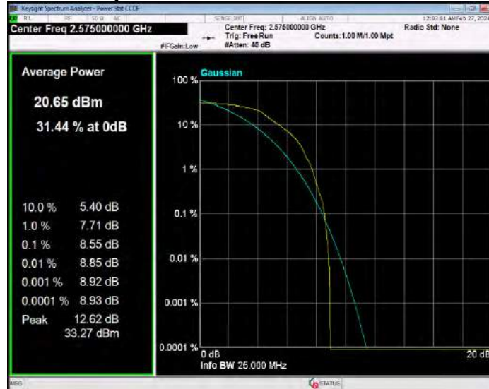
Band38 QPSK BW=10MHz Channel=38000 RB Size=1 Position=#0
