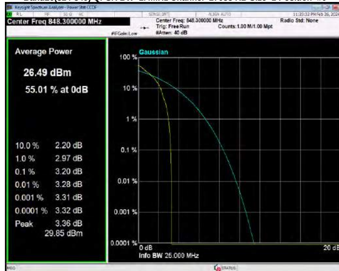
Band26(824-849) QPSK BW=10MHz Channel=26840 RB Size=1 Position=#0
