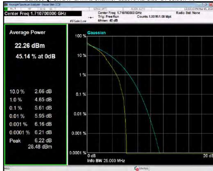
Band66 QPSK BW=1.4MHz Channel=132322 RB Size=1 Position=#0
