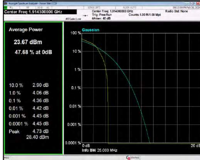
Band25 16QAM BW=10MHz Channel=26090 RB Size=1 Position=#0
