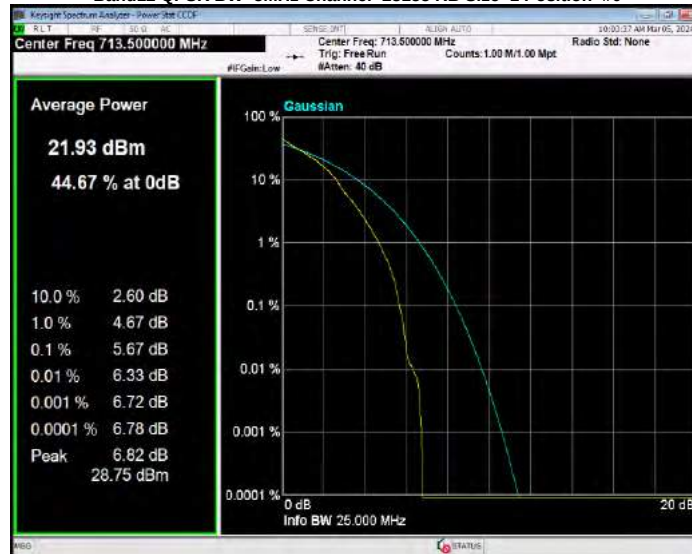
Band17 16QAM BW=10MHz Channel=23780 RB Size=1 Position=#0
