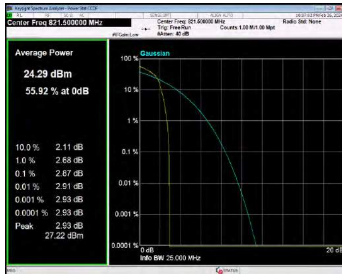
Band26(814-824) QPSK BW=1.4MHz Channel=26697 RB Size=1 Position=#0
