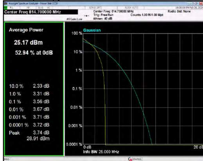
Band26(814-824) QPSK BW=1.4MHz Channel=26740 RB Size=1 Position=#0
