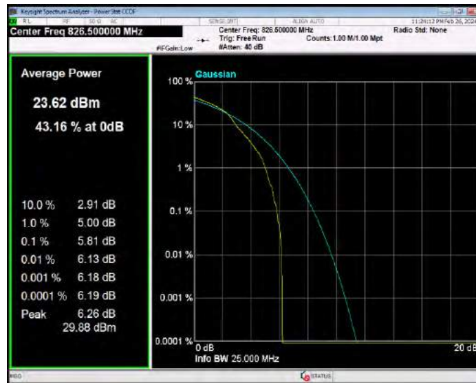
Band26(824-849) 16QAM BW=5MHz Channel=26915 RB Size=1 Position=#0
