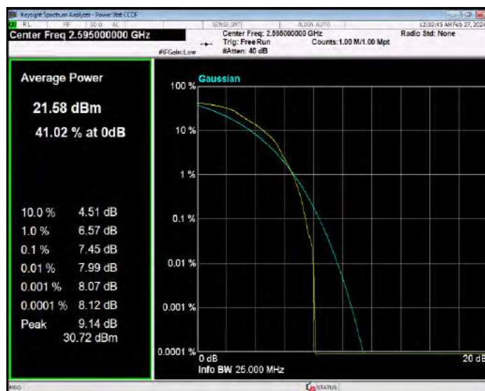
Band38 QPSK BW=5MHz Channel=38225 RB Size=1 Position=#0
