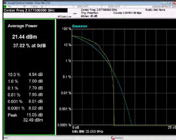
Band38 16QAM BW=15MHz Channel=38000 RB Size=1 Position=#0
