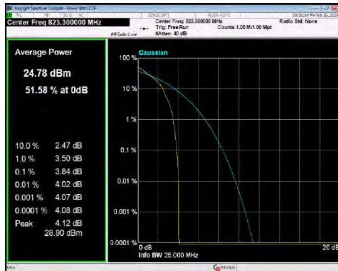
Band26(814-824) QPSK BW=10MHz Channel=26740 RB Size=1 Position=#0
