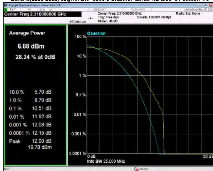
Band40(2305-2315) 16QAM BW=5MHz Channel=38725 RB Size=1 Position=#0
