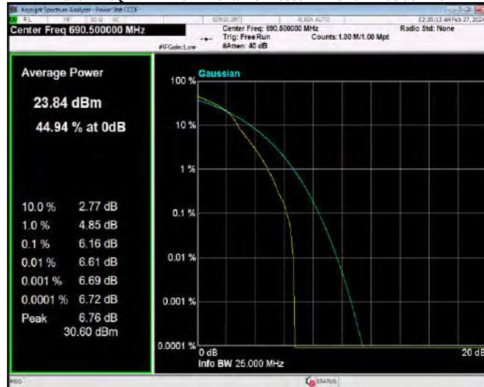
Band71 16QAM BW=20MHz Channel=133222 RB Size=1 Position=#0
