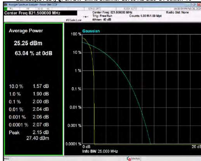
Band38 16QAM BW=10MHz Channel=37800 RB Size=1 Position=#0
