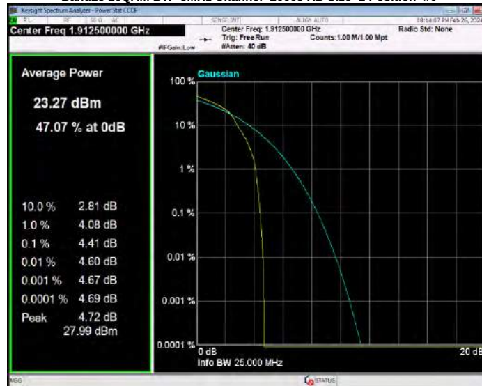
Band25 QPSK BW=1.4MHz Channel=26047 RB Size=1 Position=#0
