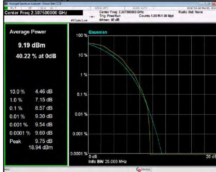
Band40(2305-2315) QPSK BW=5MHz Channel=38750 RB Size=1 Position=#0
