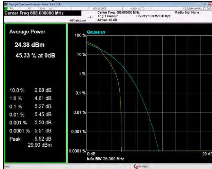
Band71 16QAM BW=5MHz Channel=133147 RB Size=1 Position=#0
