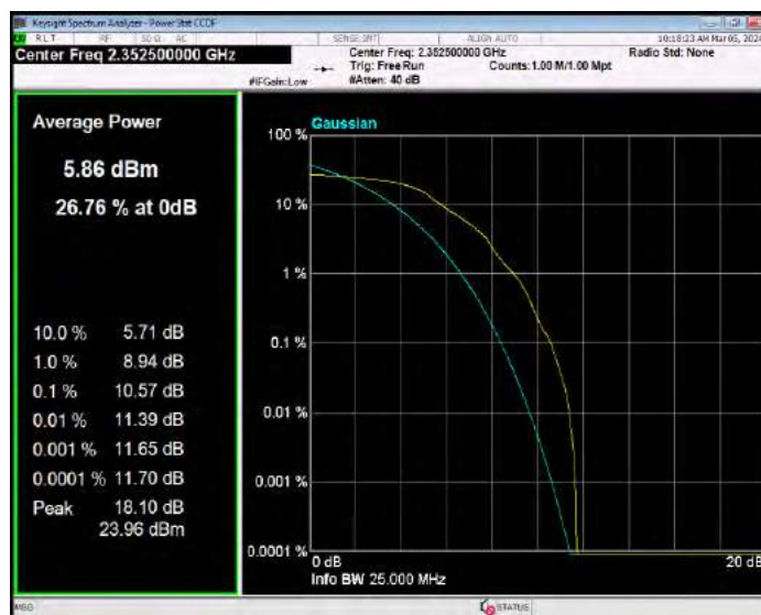
Band40(2350-2360) QPSK BW=5MHz Channel=39200 RB Size=1 Position=#0
