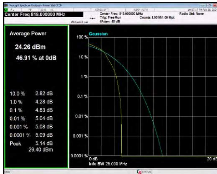
Band26(814-824) 16QAM BW=3MHz Channel=26705 RB Size=1 Position=#0
