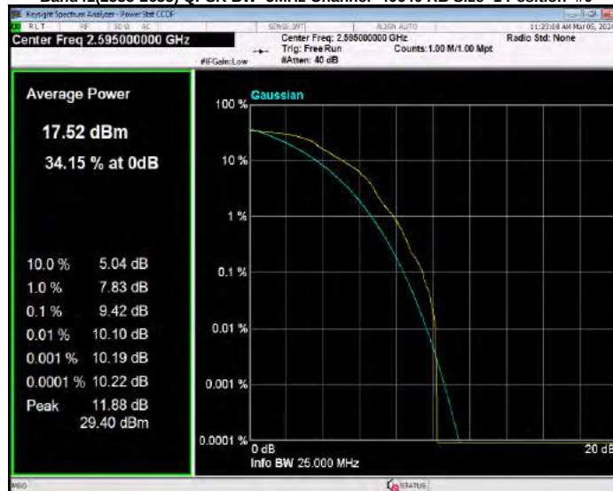
Band66 16QAM BW=1.4MHz Channel=131979 RB Size=1 Position=#0
