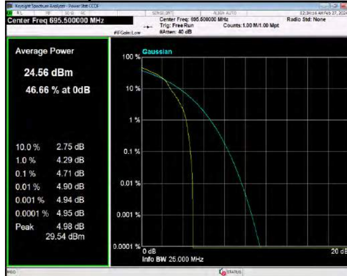
Band71 QPSK BW=10MHz Channel=133172 RB Size=1 Position=#0
