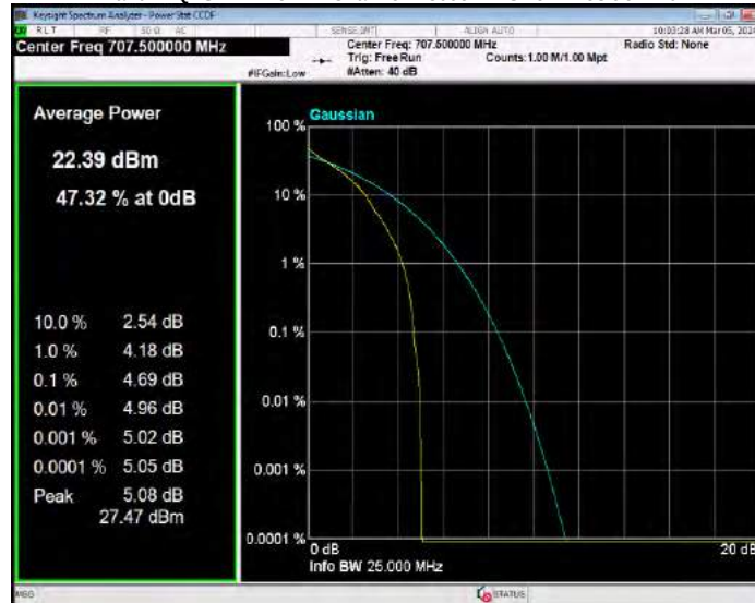
Band12 QPSK BW=5MHz Channel=23155 RB Size=1 Position=#0
