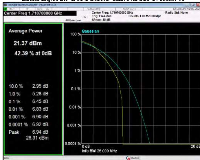
Band66 16QAM BW=1.4MHz Channel=132322 RB Size=1 Position=#0
