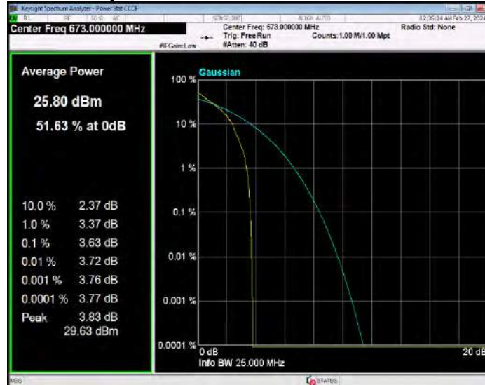
Band71 QPSK BW=20MHz Channel=133297 RB Size=1 Position=#0
