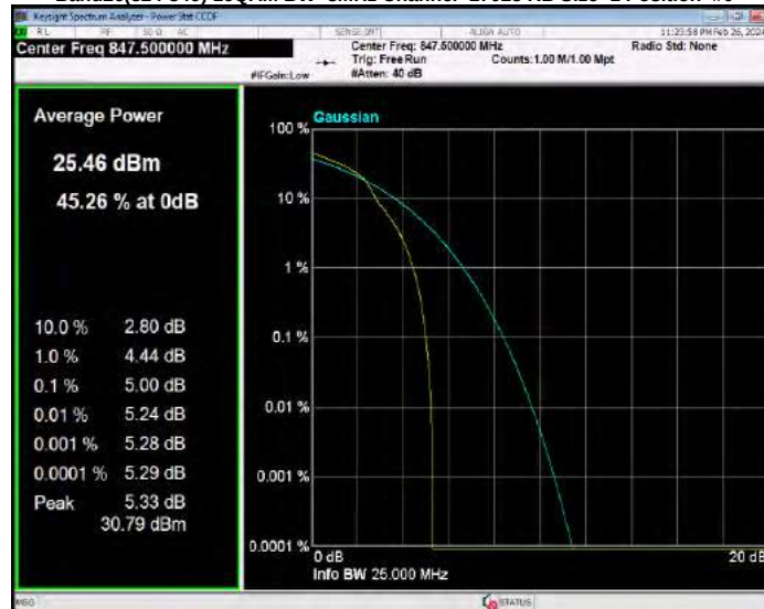
Band26(824-849) 16QAM BW=5MHz Channel=26815 RB Size=1 Position=#0
