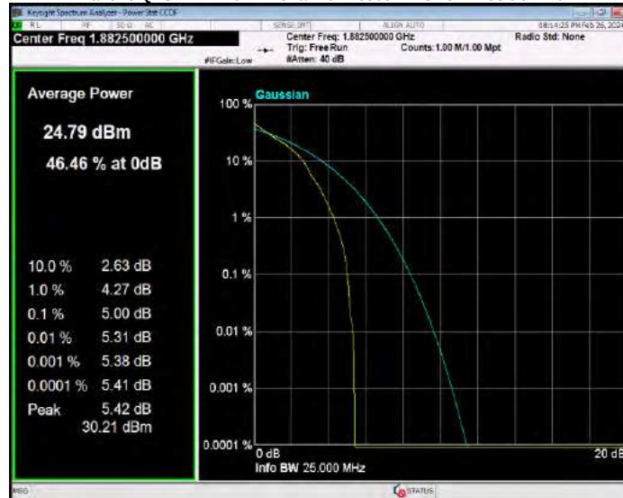
Band25 QPSK BW=10MHz Channel=26640 RB Size=1 Position=#0
