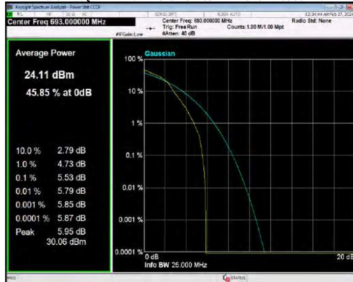
Band71 16QAM BW=15MHz Channel=133197 RB Size=1 Position=#0
