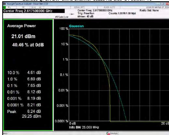
Band40(2305-2315) 16QAM BW=10MHz Channel=38750 RB Size=1 Position=#0
