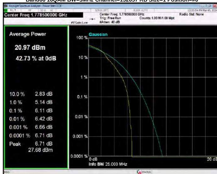
Band66 16QAM BW=5MHz Channel=131997 RB Size=1 Position=#0
