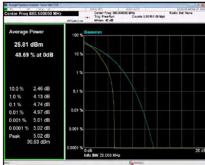
Band71 QPSK BW=10MHz Channel=133422 RB Size=1 Position=#0
