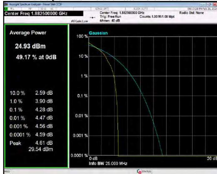
Band25 QPSK BW=3MHz Channel=26675 RB Size=1 Position=#0
