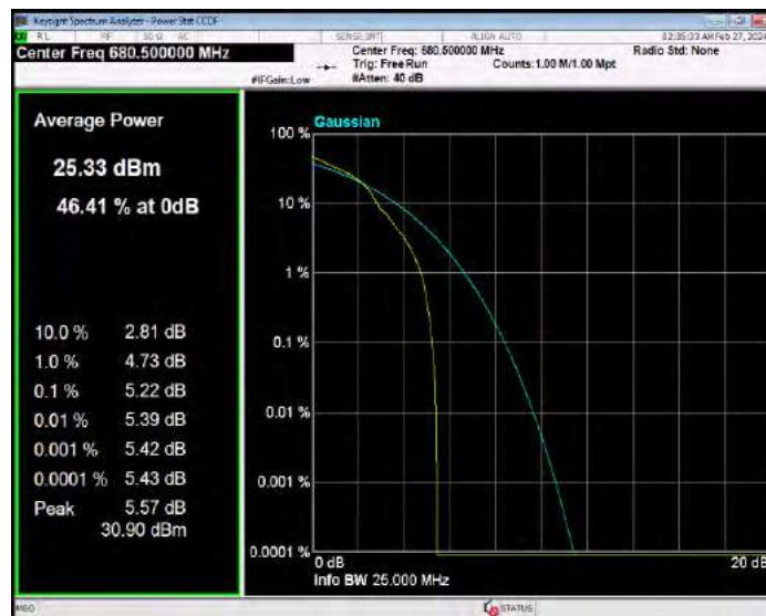
Band71 16QAM BW=20MHz Channel=133372 RB Size=1 Position=#0
