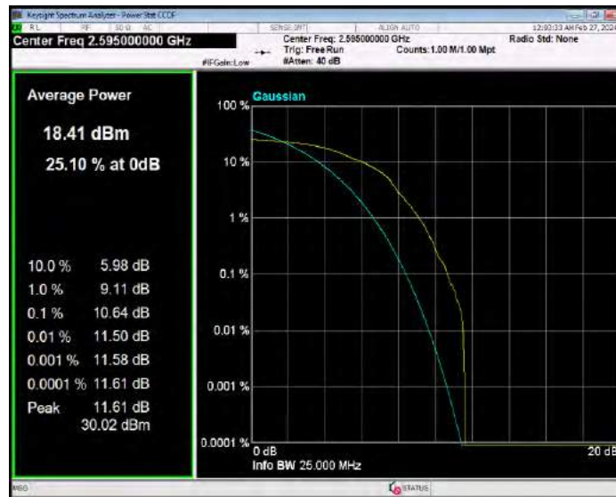
Band38 16QAM BW=15MHz Channel=38175 RB Size=1 Position=#0
