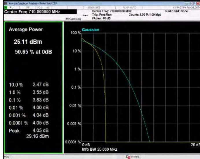
Band17 QPSK BW=5MHz Channel=23825 RB Size=1 Position=#0
