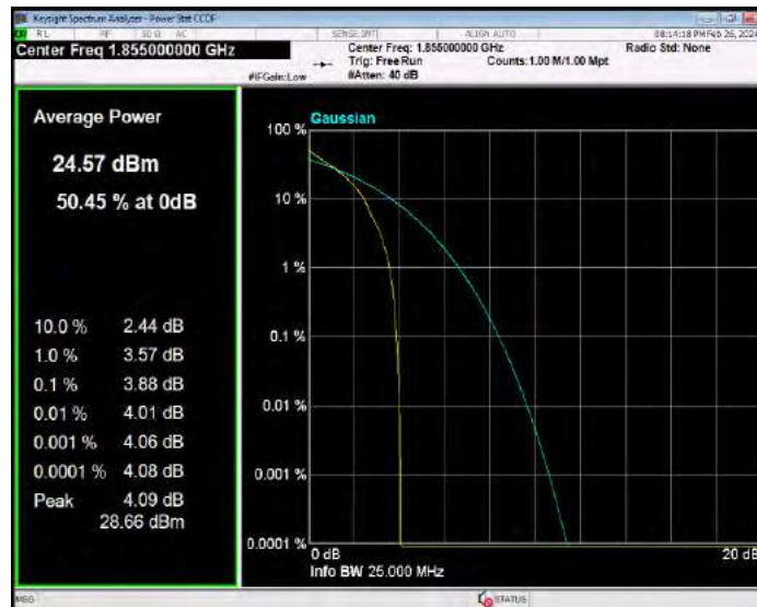
Band25 QPSK BW=10MHz Channel=26365 RB Size=1 Position=#0
