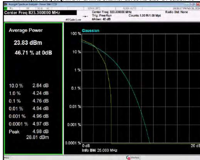
Band26(814-824) 16QAM BW=10MHz Channel=26740 RB Size=1 Position=#0
