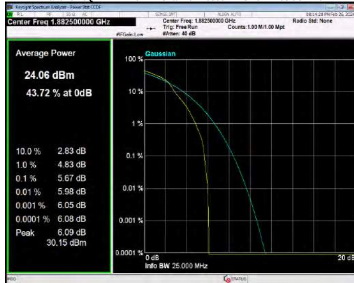
Band25 16QAM BW=10MHz Channel=26640 RB Size=1 Position=#0
