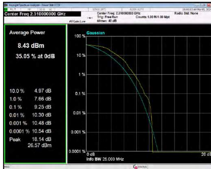
Band40(2305-2315) QPSK BW=5MHz Channel=38725 RB Size=1 Position=#0
