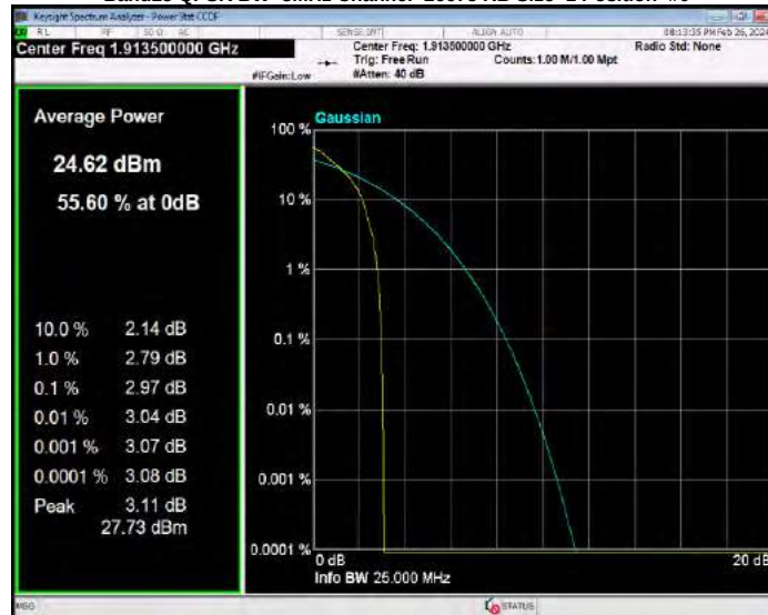
Band25 QPSK BW=5MHz Channel=26065 RB Size=1 Position=#0
