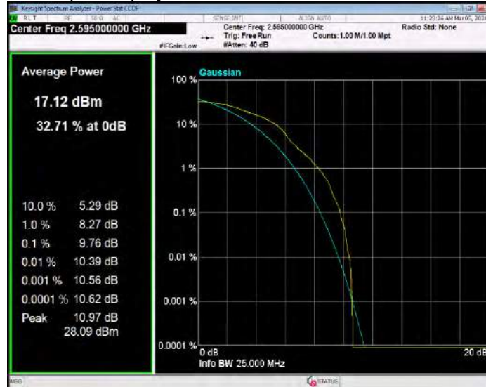
Band41(2535-2655) 16QAM BW=20MHz Channel=40640 RB Size=1 Position=#0
