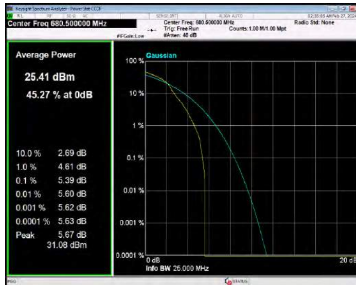
Band71 16QAM BW=15MHz Channel=133397 RB Size=1 Position=#0
