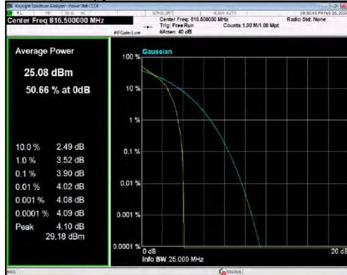
Band26(814-824) QPSK BW=5MHz Channel=26740 RB Size=1 Position=#0
