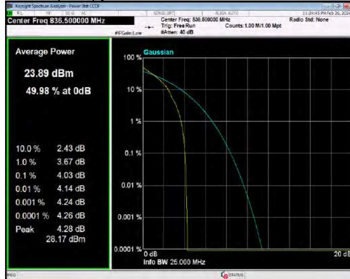
Band26(824-849) QPSK BW=10MHz Channel=26990 RB Size=1 Position=#0
