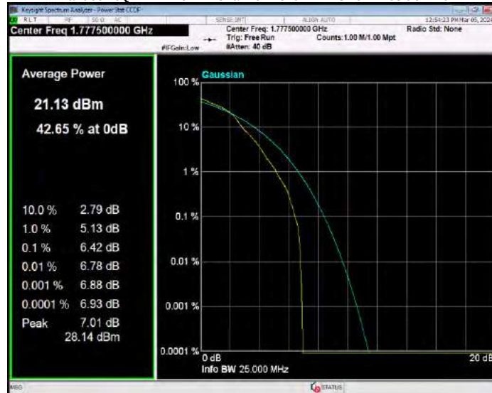
Band66 QPSK BW=1.4MHz Channel=131979 RB Size=1 Position=#0
