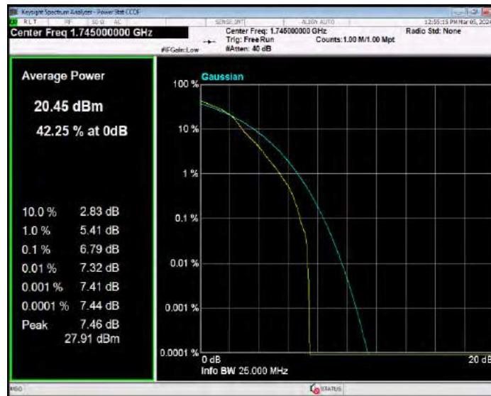
Band66 16QAM BW=15MHz Channel=132597 RB Size=1 Position=#0
