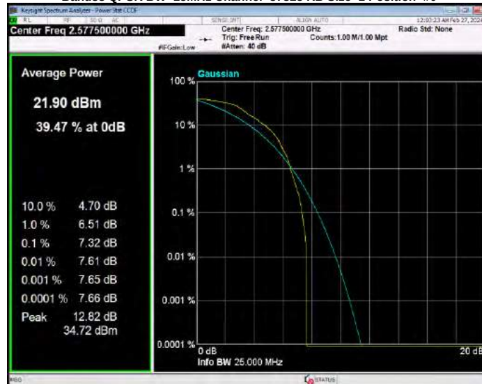
Band38 QPSK BW=15MHz Channel=38000 RB Size=1 Position=#0
