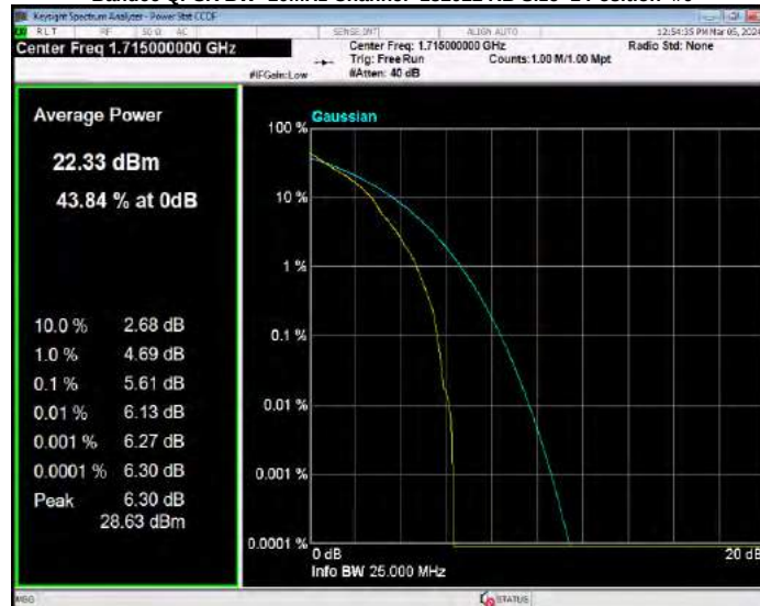
Band66 QPSK BW=10MHz Channel=132322 RB Size=1 Position=#0
