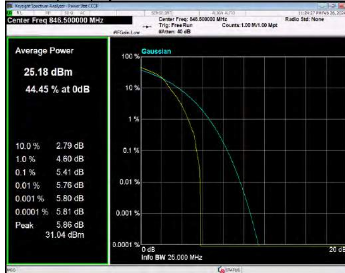
Band26(824-849) QPSK BW=1.4MHz Channel=26797 RB Size=1 Position=#0
