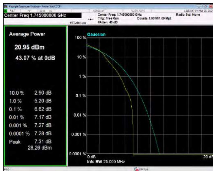
Band66 16QAM BW=3MHz Channel=132657 RB Size=1 Position=#0
