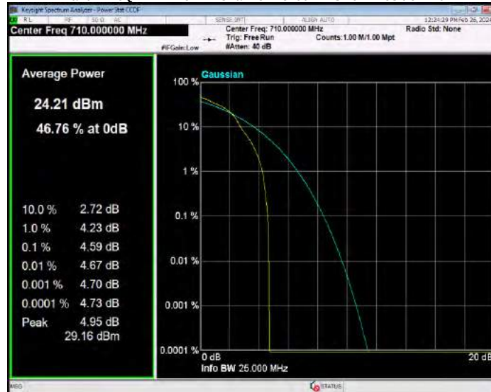
Band17 16QAM BW=5MHz Channel=23825 RB Size=1 Position=#0
