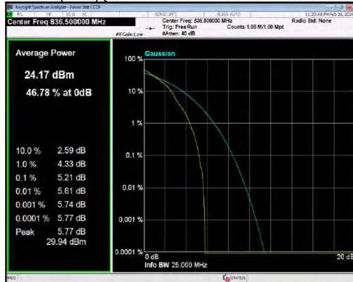
Band26(824-849) QPSK BW=3MHz Channel=27025 RB Size=1 Position=#0
