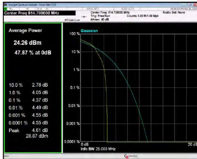
Band26(814-824) 16QAM BW=1.4MHz Channel=26740 RB Size=1 Position=#0
