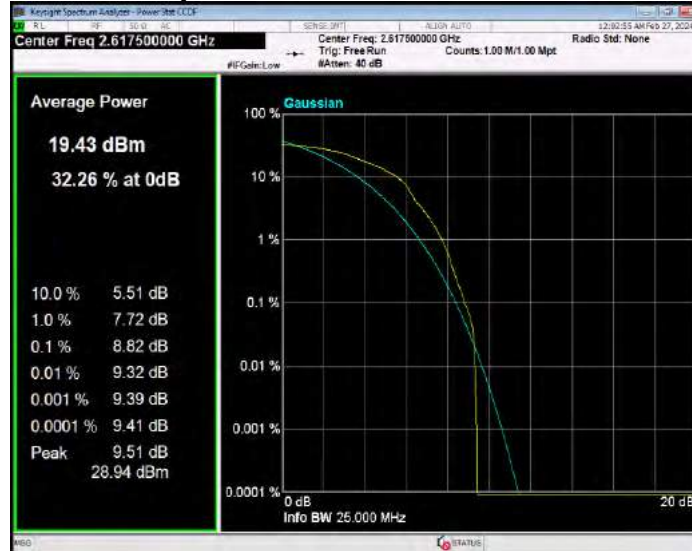
Band38 QPSK BW=10MHz Channel=37800 RB Size=1 Position=#0
