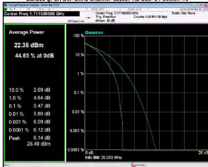
Band66 QPSK BW=3MHz Channel=132322 RB Size=1 Position=#0
