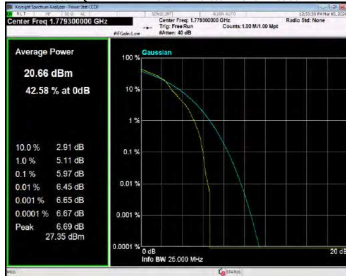
Band66 16QAM BW=10MHz Channel=132022 RB Size=1 Position=#0
