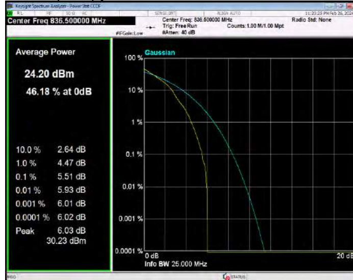
Band26(824-849) QPSK BW=1.4MHz Channel=27033 RB Size=1 Position=#0
