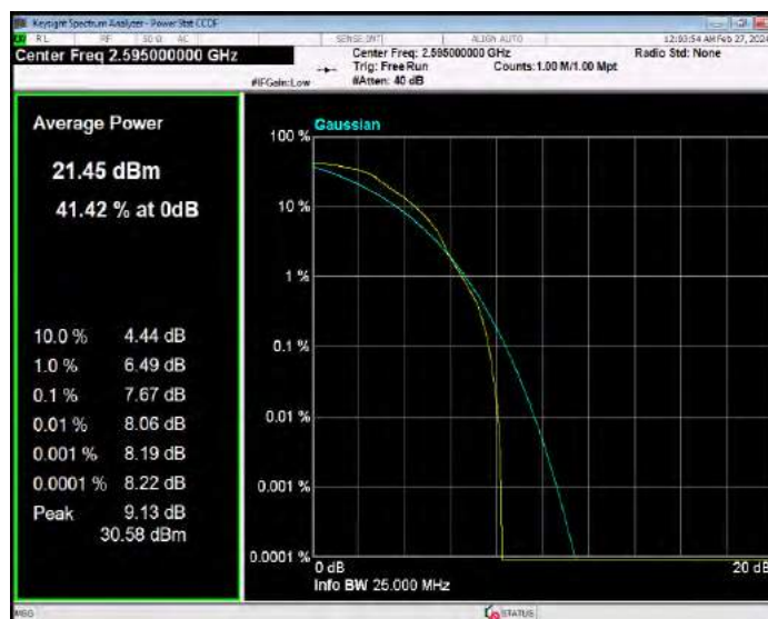
Band38 QPSK BW=20MHz Channel=38150 RB Size=1 Position=#0
