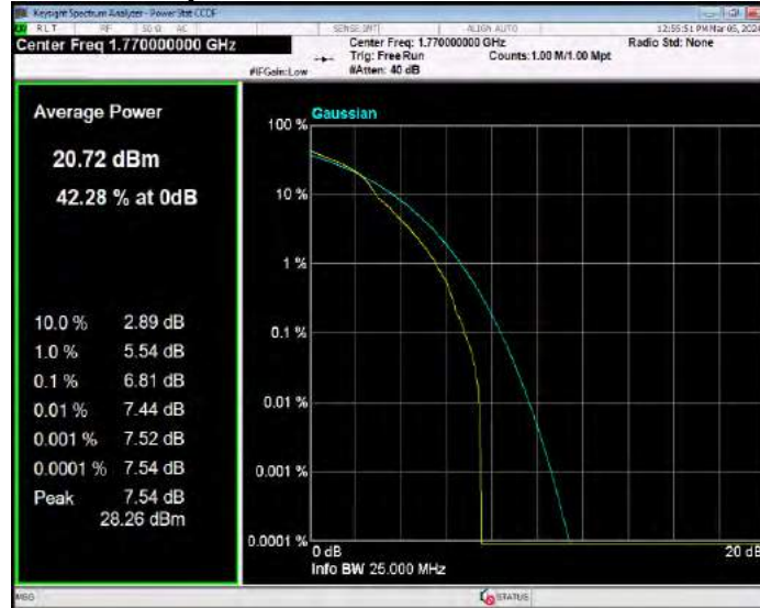
Band66 16QAM BW=3MHz Channel=131987 RB Size=1 Position=#0
