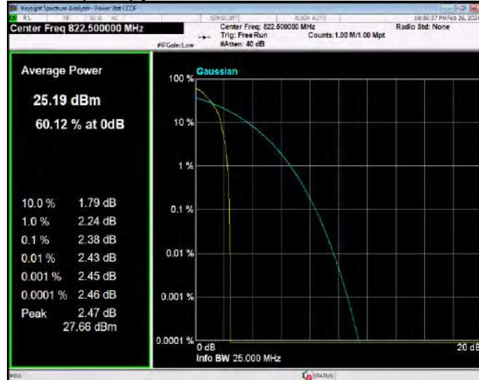
Band26(814-824) QPSK BW=5MHz Channel=26715 RB Size=1 Position=#0
