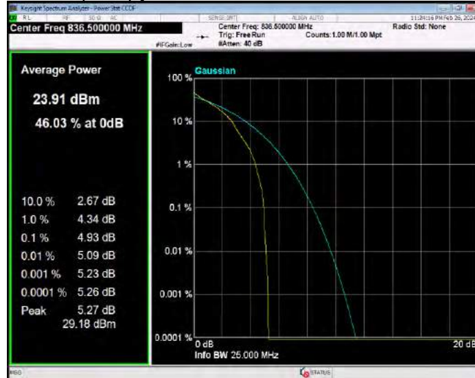
Band26(824-849) QPSK BW=5MHz Channel=27015 RB Size=1 Position=#0
