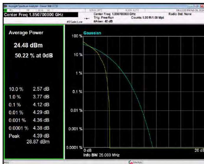
Band25 QPSK BW=1.4MHz Channel=26365 RB Size=1 Position=#0
