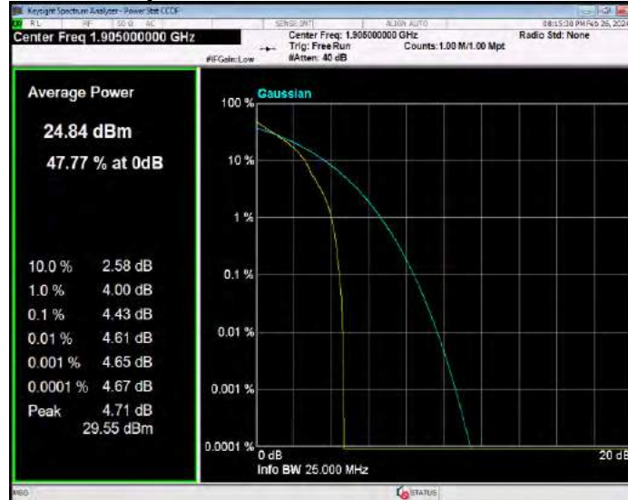
Band25 QPSK BW=3MHz Channel=26055 RB Size=1 Position=#0
