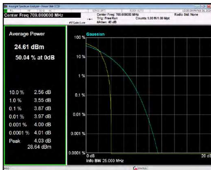
Band17 16QAM BW=10MHz Channel=23790 RB Size=1 Position=#0
