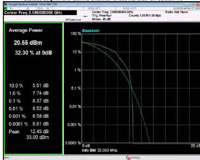
Band38 16QAM BW=20MHz Channel=38000 RB Size=1 Position=#0
