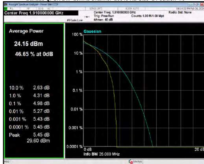
Band25 QPSK BW=15MHz Channel=26115 RB Size=1 Position=#0
