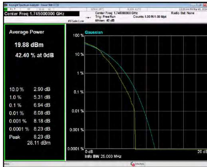
Band66 16QAM BW=20MHz Channel=132572 RB Size=1 Position=#0
