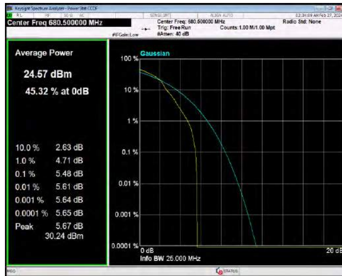
Band71 16QAM BW=5MHz Channel=133447 RB Size=1 Position=#0
