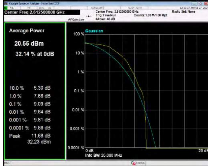
Band38 QPSK BW=20MHz Channel=37850 RB Size=1 Position=#0
