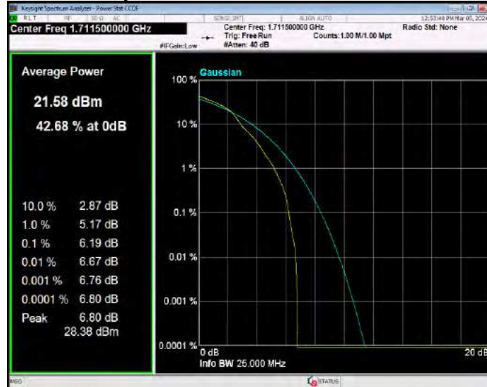
Band66 16QAM BW=3MHz Channel=132322 RB Size=1 Position=#0
