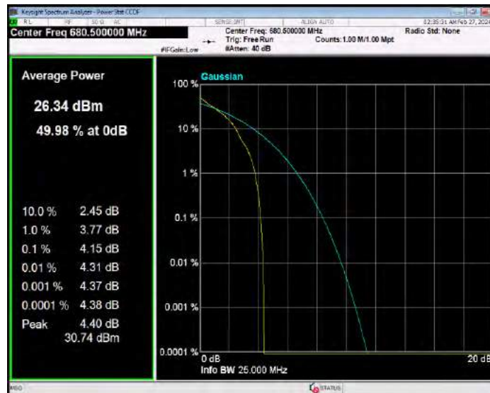
Band71 QPSK BW=20MHz Channel=133372 RB Size=1 Position=#0
