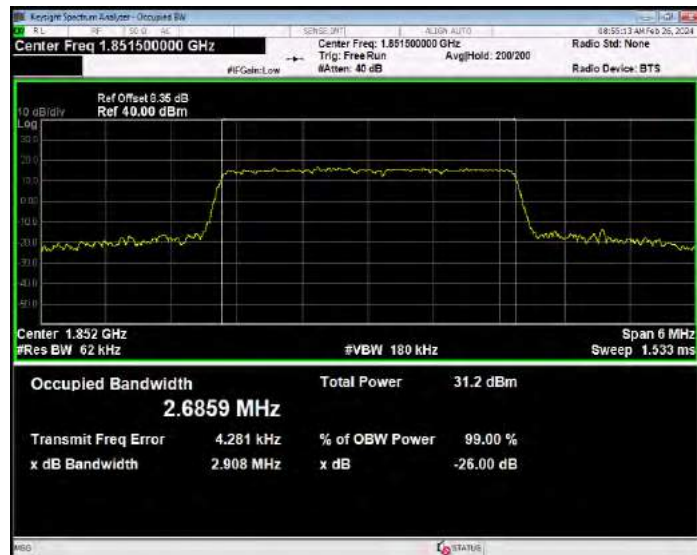
Band2 16QAM BW=3MHz Channel=18900 RB Size=15 Position=#0
