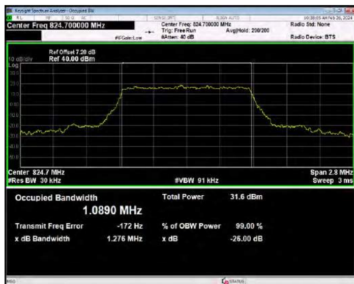
Band5 QPSK BW=1.4MHz Channel=20525 RB Size=6 Position=#0
