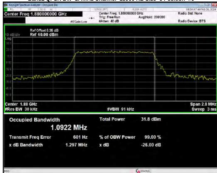
Band2 QPSK BW=1.4MHz Channel=19193 RB Size=6 Position=#0
