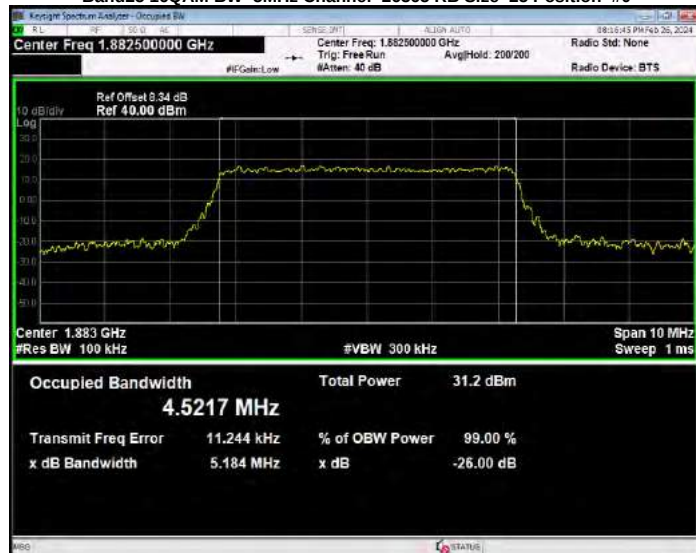
Band25 16QAM BW=5MHz Channel=26665 RB Size=25 Position=#0
