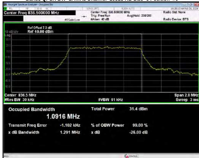
Band5 QPSK BW=1.4MHz Channel=20643 RB Size=6 Position=#0
