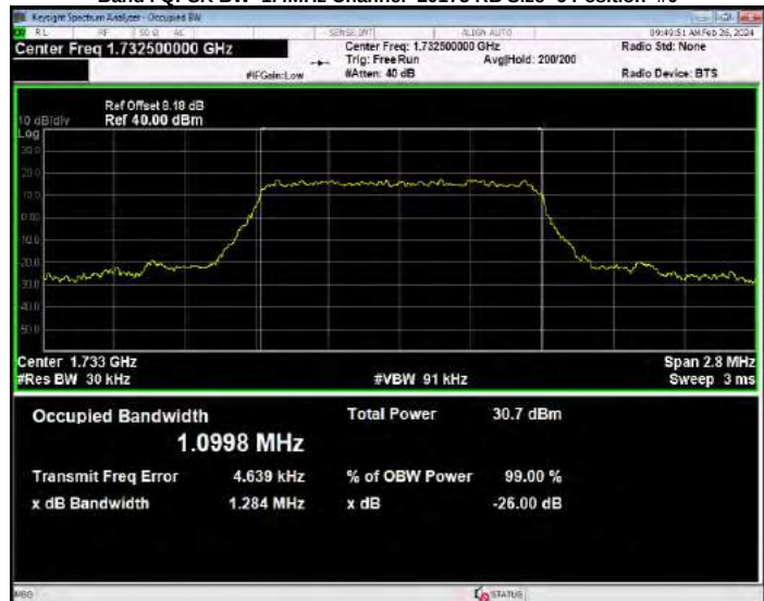
Band4 QPSK BW=1.4MHz Channel=20393 RB Size=6 Position=#0
