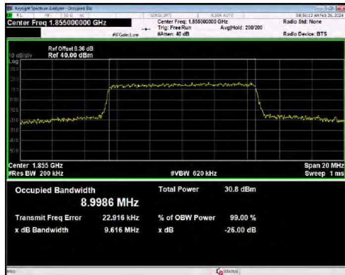
Band2 16QAM BW=10MHz Channel=18900 RB Size=50 Position=#0
