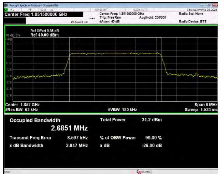
Band25 16QAM BW=3MHz Channel=26365 RB Size=15 Position=#0
