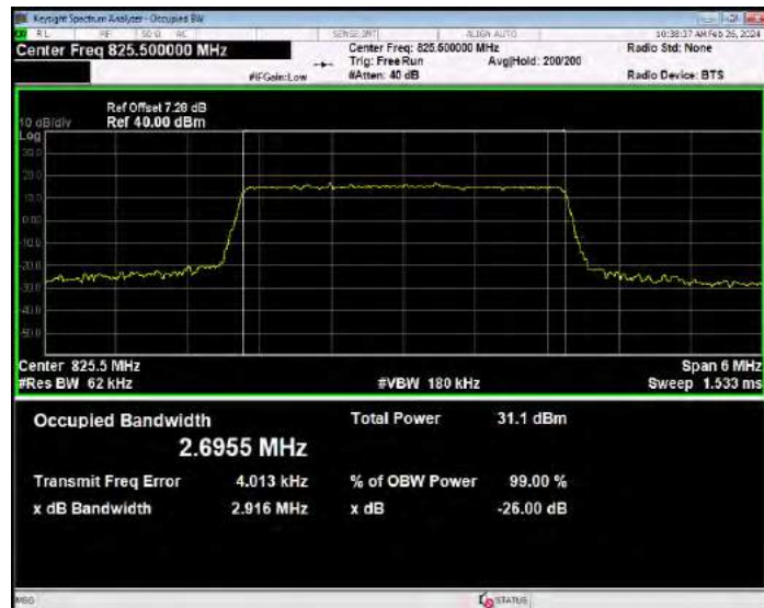
Band5 16QAM BW=3MHz Channel=20525 RB Size=15 Position=#0
