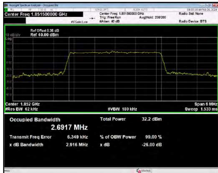
Band2 QPSK BW=3MHz Channel=18900 RB Size=15 Position=#0
