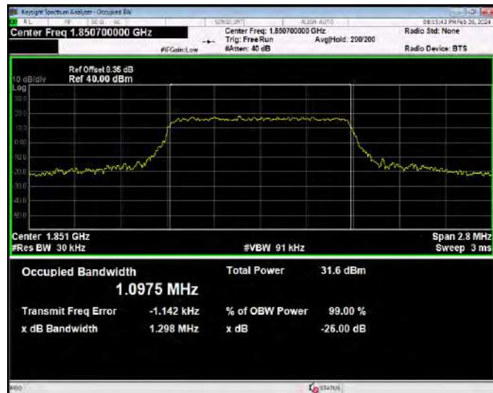
Band25 QPSK BW=1.4MHz Channel=26365 RB Size=6 Position=#0
