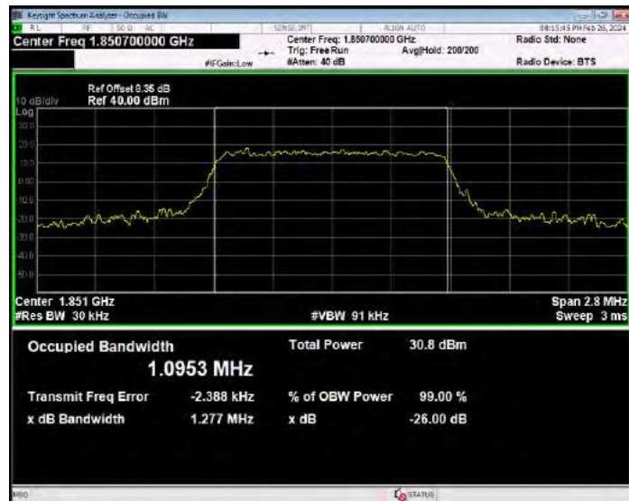
Band25 16QAM BW=1.4MHz Channel=26365 RB Size=6 Position=#0
