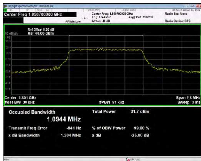
Band2 QPSK BW=1.4MHz Channel=18900 RB Size=6 Position=#0
