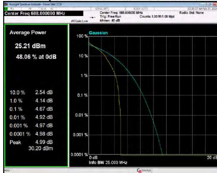
Band71 QPSK BW=5MHz Channel=133147 RB Size=1 Position=#0
