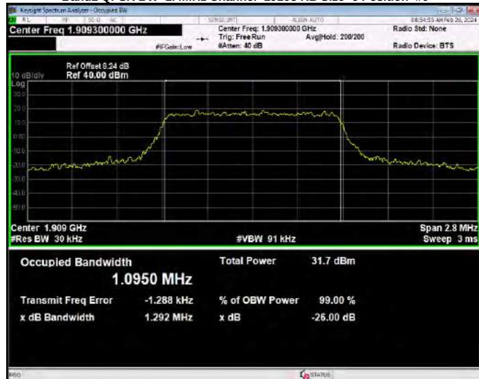
Band2 QPSK BW=10MHz Channel=18650 RB Size=50 Position=#0
