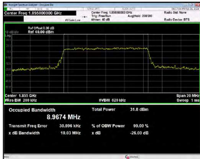
Band25 QPSK BW=10MHz Channel=26365 RB Size=50 Position=#0
