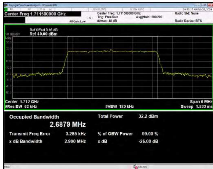
Band4 16QAM BW=3MHz Channel=20175 RB Size=15 Position=#0
