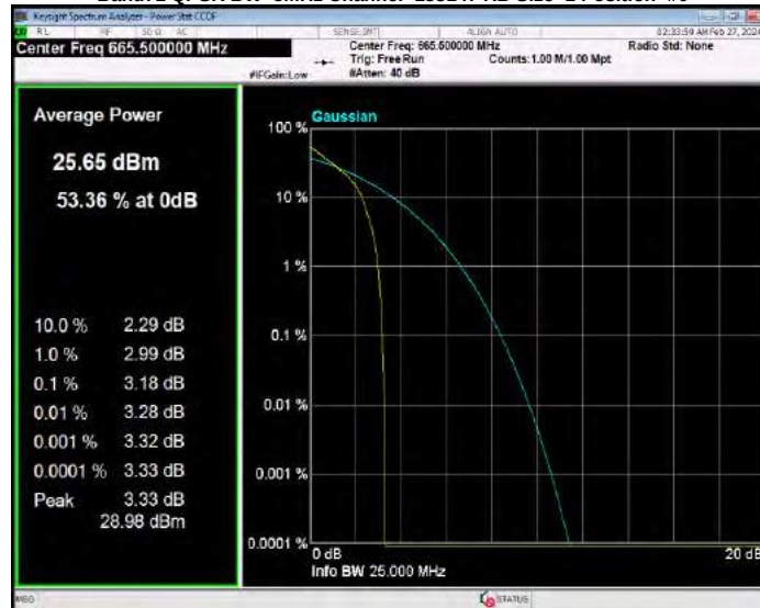
Band71 QPSK BW=5MHz Channel=133297 RB Size=1 Position=#0
