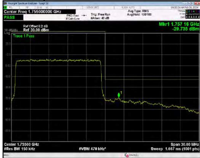
Band4 QPSK BW=20MHz Channel=20050 RB Size=1 Position=#0
