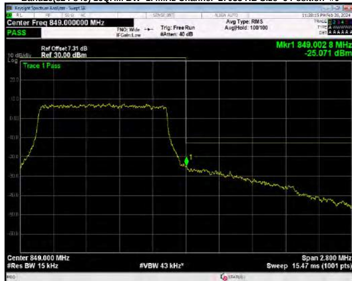
Band26(824-849) 16QAM BW=10MHz Channel=26840 RB Size=50 Position=#0
