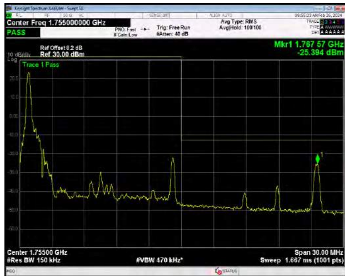
Band4 QPSK BW=15MHz Channel=20325 RB Size=75 Position=#0
