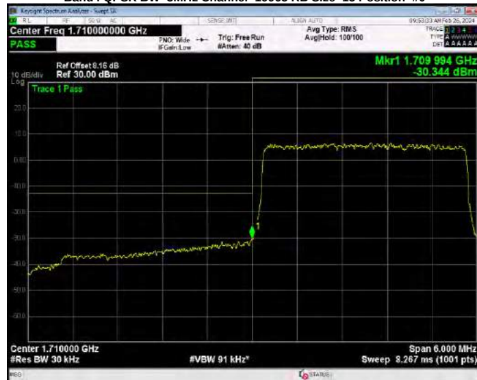
Band4 QPSK BW=3MHz Channel=20385 RB Size=1 Position=#0
