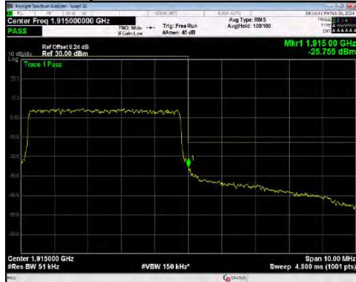
Band25 QPSK BW=1.4MHz Channel=26047 RB Size=6 Position=#0
