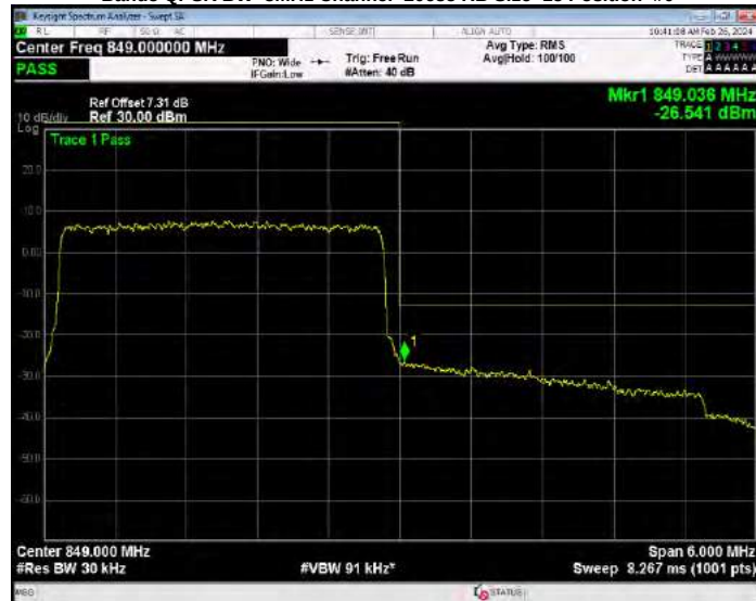
Band5 QPSK BW=5MHz Channel=20425 RB Size=1 Position=#0
