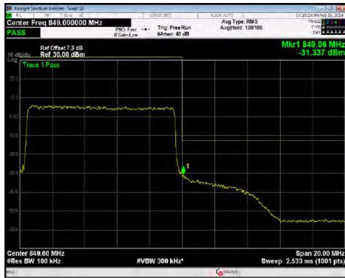
Band26(824-849) 16QAM BW=15MHz Channel=26865 RB Size=75 Position=#0
