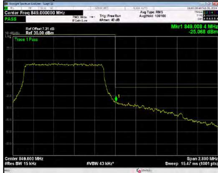
Band5 16QAM BW=10MHz Channel=20450 RB Size=1 Position=#0
