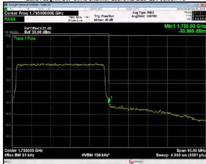
Band4 QPSK BW=1.4MHz Channel=19957 RB Size=1 Position=#0
