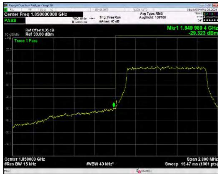
Band25 16QAM BW=1.4MHz Channel=26683 RB Size=6 Position=#0
