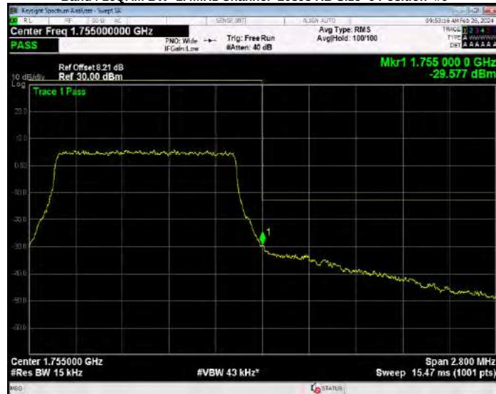
Band4 16QAM BW=10MHz Channel=20000 RB Size=1 Position=#0
