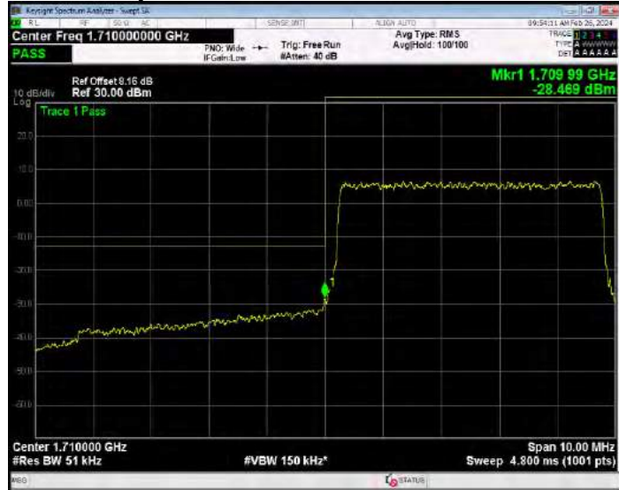
Band4 QPSK BW=5MHz Channel=20375 RB Size=1 Position=#0
