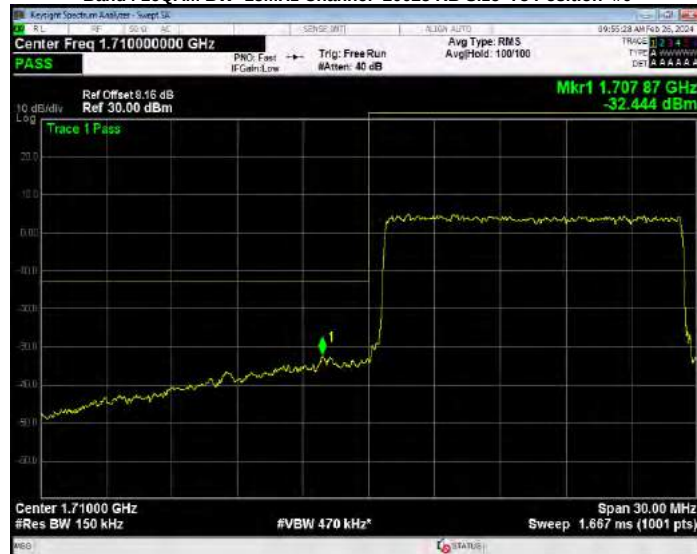
Band4 16QAM BW=15MHz Channel=20325 RB Size=1 Position=#0
