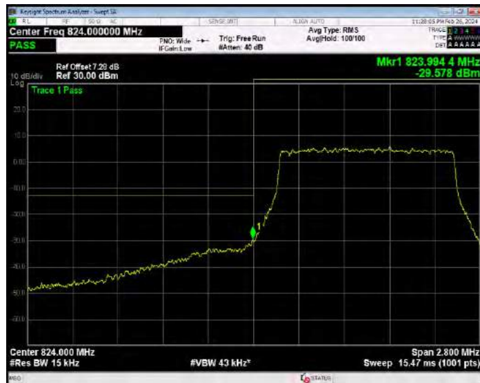
Band26(824-849) 16QAM BW=1.4MHz Channel=27033 RB Size=6 Position=#0
