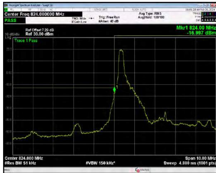
Band5 QPSK BW=5MHz Channel=20425 RB Size=25 Position=#0
