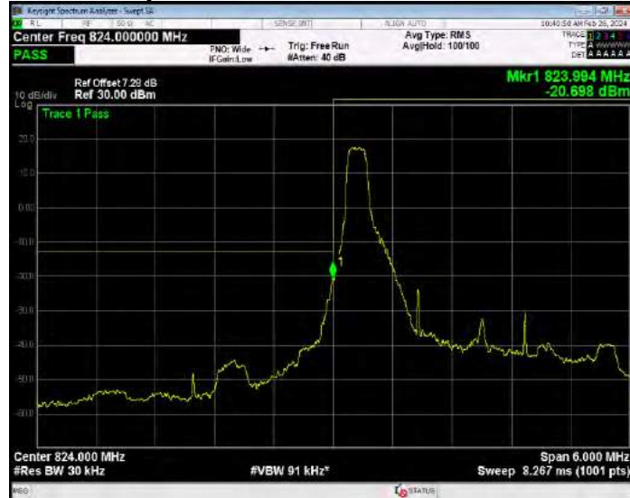
Band5 QPSK BW=3MHz Channel=20415 RB Size=15 Position=#0
