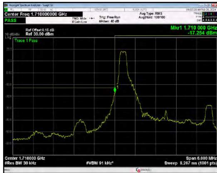
Band4 QPSK BW=3MHz Channel=19965 RB Size=15 Position=#0
