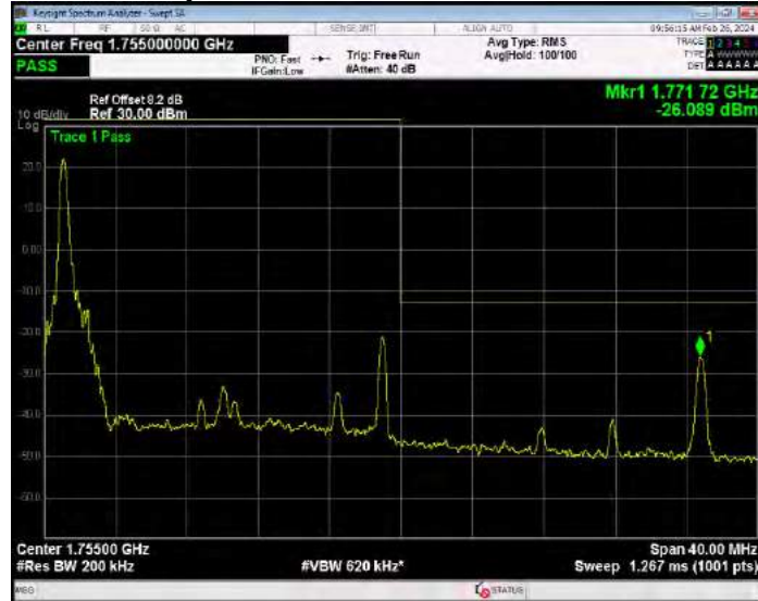
Band4 16QAM BW=20MHz Channel=20300 RB Size=100 Position=#0
