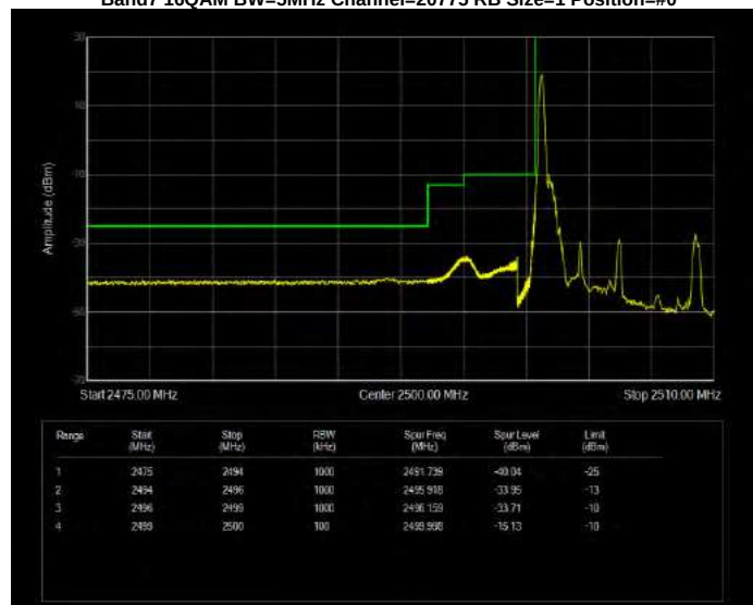
Band7 16QAM BW=5MHz Channel=20775 RB Size=25 Position=#0
