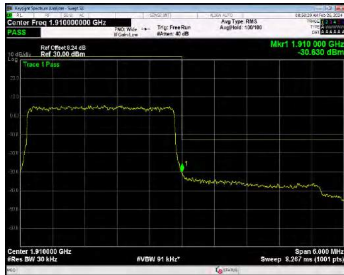
Band2 QPSK BW=5MHz Channel=18625 RB Size=1 Position=#0
