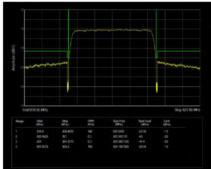
Band26(814-824) 16QAM BW=5MHz Channel=26715 RB Size=25 Position=#0
