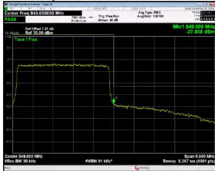
Band5 16QAM BW=5MHz Channel=20425 RB Size=1 Position=#0
