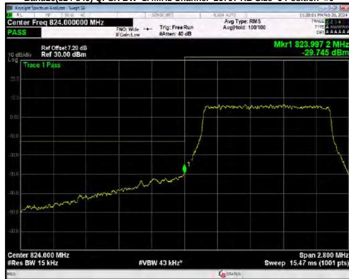
Band26(824-849) QPSK BW=1.4MHz Channel=27033 RB Size=6 Position=#0
