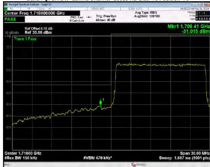
Band4 QPSK BW=15MHz Channel=20325 RB Size=1 Position=#0
