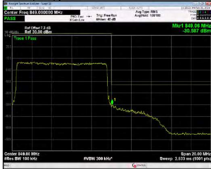
Band26(824-849) QPSK BW=15MHz Channel=26865 RB Size=75 Position=#0
