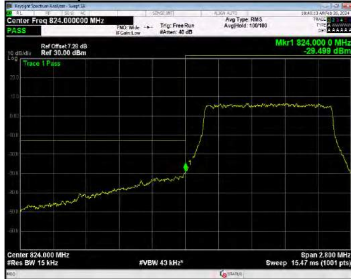
Band5 QPSK BW=1.4MHz Channel=20643 RB Size=1 Position=#0
