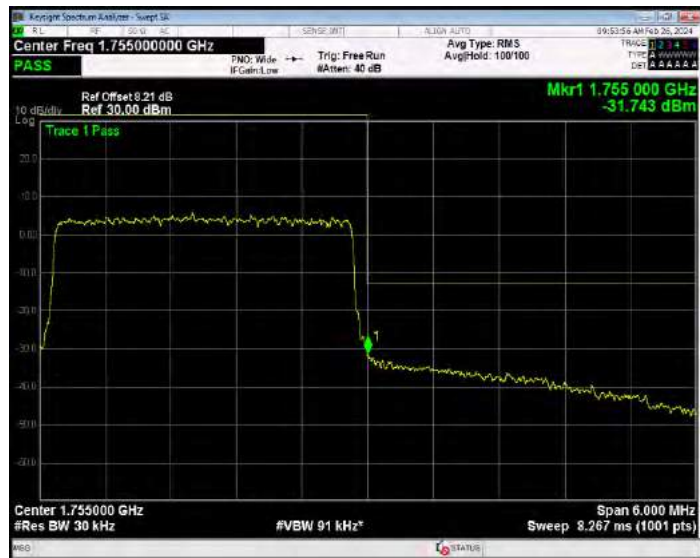
Band4 16QAM BW=5MHz Channel=19975 RB Size=1 Position=#0
