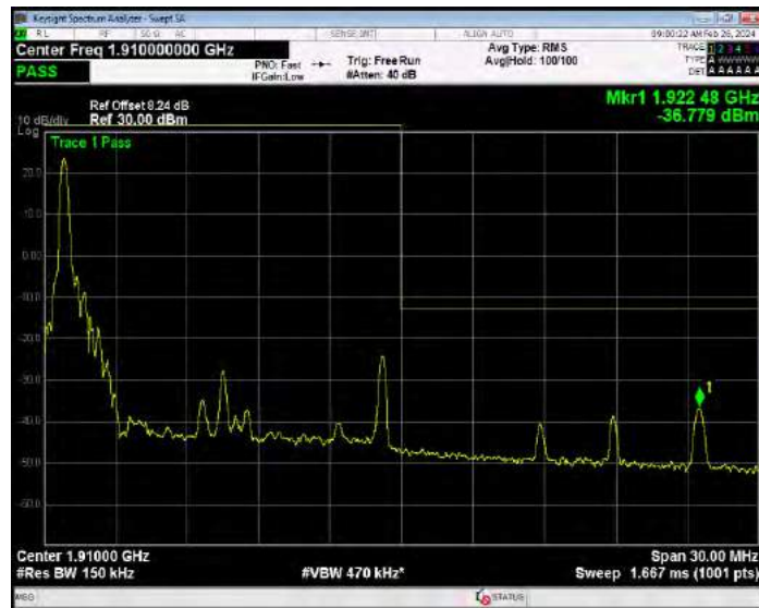
Band2 QPSK BW=15MHz Channel=19125 RB Size=75 Position=#0
