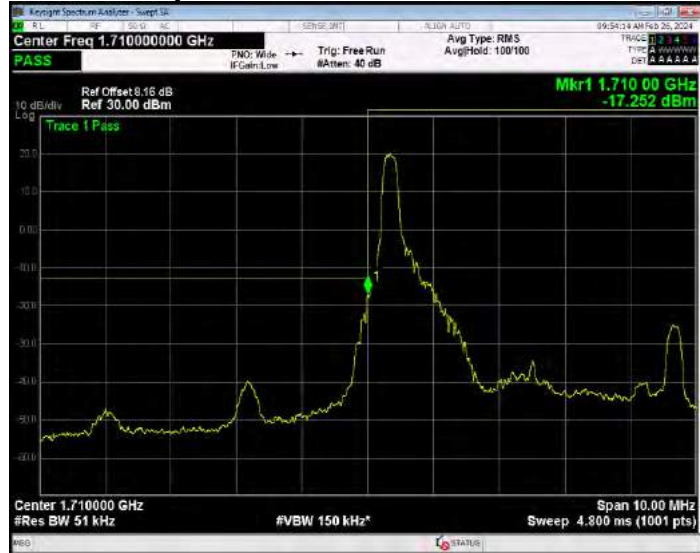
Band4 16QAM BW=5MHz Channel=19975 RB Size=25 Position=#0
