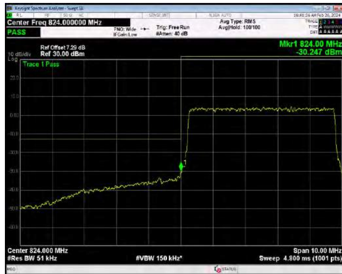
Band5 16QAM BW=5MHz Channel=20625 RB Size=1 Position=#0
