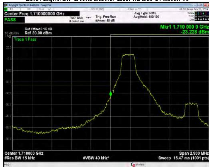
Band4 16QAM BW=1.4MHz Channel=19957 RB Size=6 Position=#0
