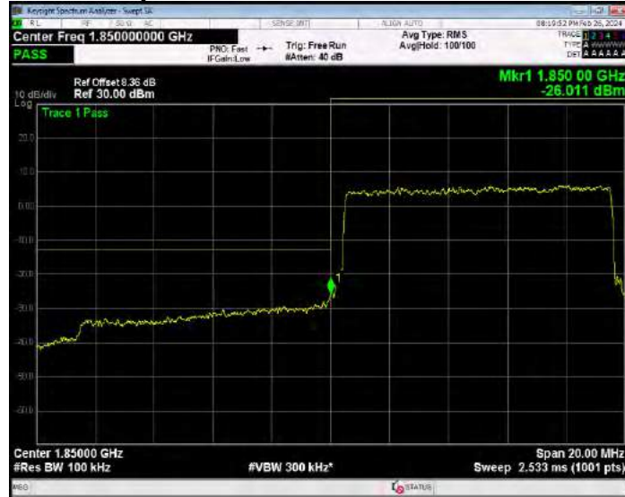
Band25 QPSK BW=10MHz Channel=26640 RB Size=50 Position=#0
