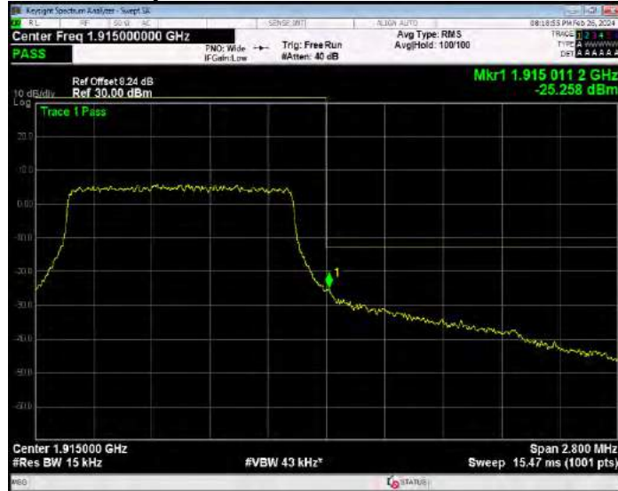
Band25 16QAM BW=10MHz Channel=26090 RB Size=50 Position=#0
