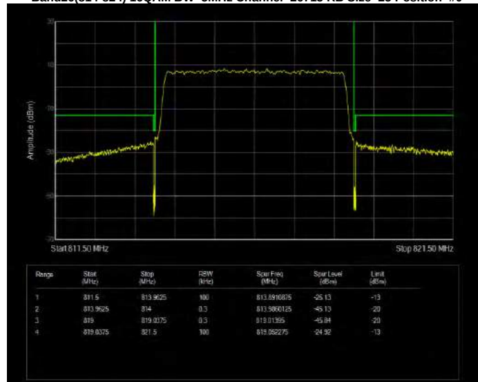
Band26(814-824) 16QAM BW=5MHz Channel=26765 RB Size=25 Position=#0
