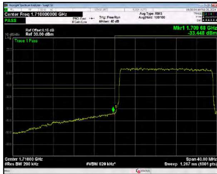
Band4 16QAM BW=20MHz Channel=20300 RB Size=1 Position=#0
