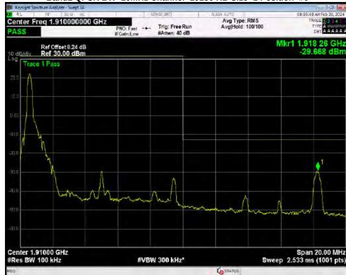
Band2 QPSK BW=10MHz Channel=19150 RB Size=50 Position=#0
