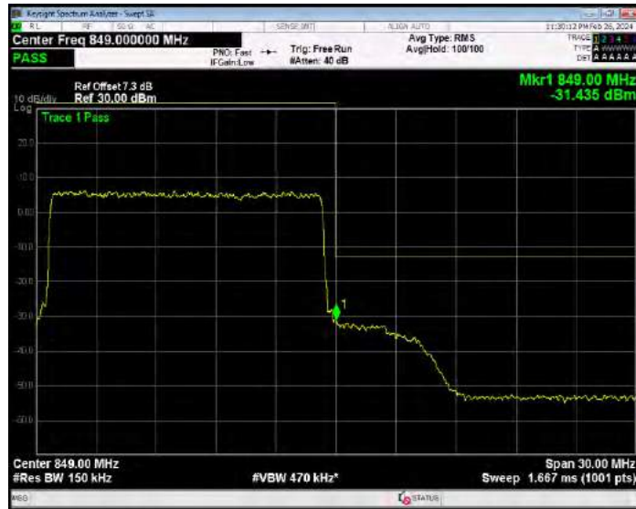
Band26(824-849) QPSK BW=3MHz Channel=26805 RB Size=15 Position=#0
