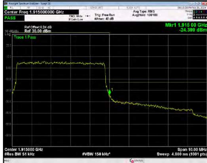
Band26(824-849) 16QAM BW=1.4MHz Channel=26797 RB Size=6 Position=#0
