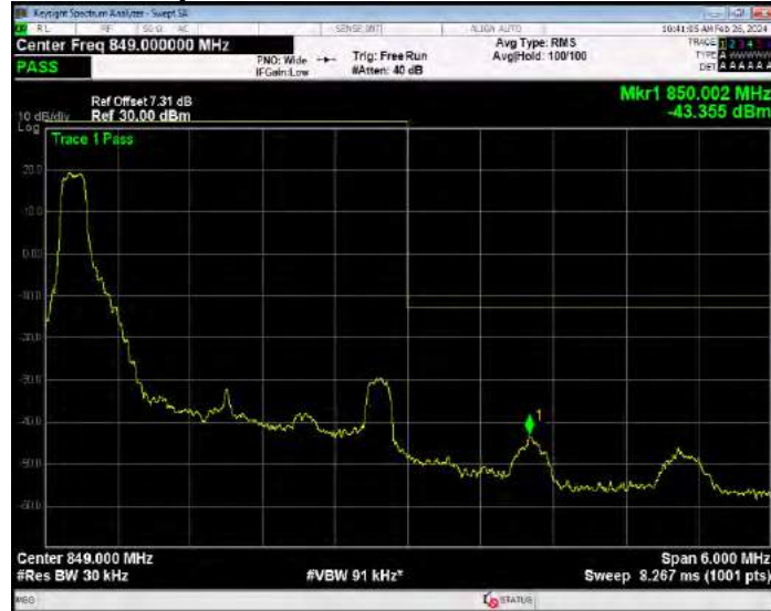
Band5 QPSK BW=3MHz Channel=20635 RB Size=15 Position=#0
