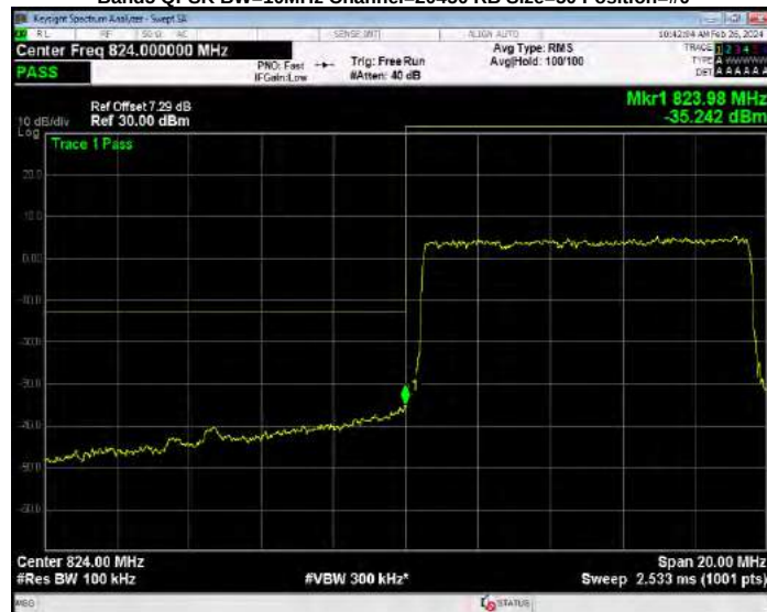
Band5 QPSK BW=10MHz Channel=20600 RB Size=1 Position=#0
