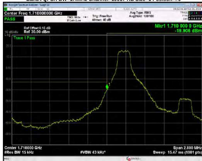
Band4 QPSK BW=1.4MHz Channel=19957 RB Size=6 Position=#0
