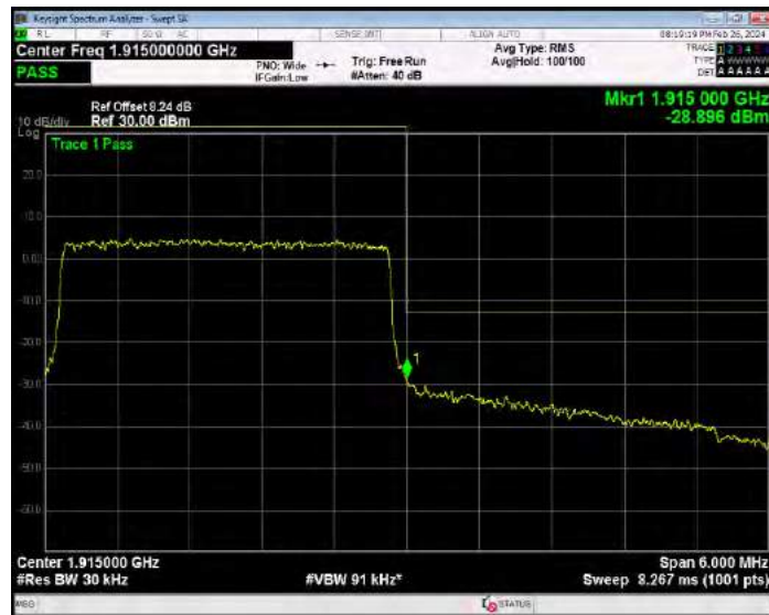
Band25 16QAM BW=5MHz Channel=26065 RB Size=25 Position=#0
