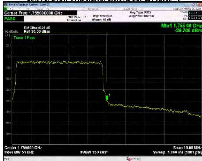
Band5 16QAM BW=1.4MHz Channel=20407 RB Size=1 Position=#0
