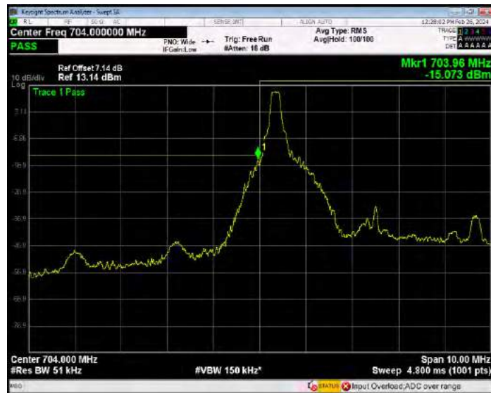
Band17 16QAM BW=5MHz Channel=23755 RB Size=25 Position=#0
