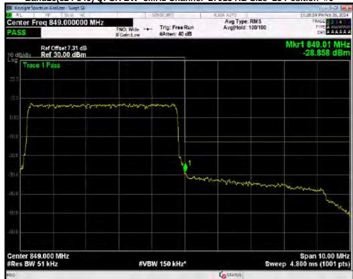
Band26(814-824) 16QAM BW=1.4MHz Channel=26697 RB Size=6 Position=#0
