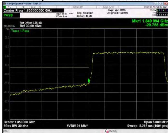
Band25 16QAM BW=3MHz Channel=26675 RB Size=15 Position=#0
