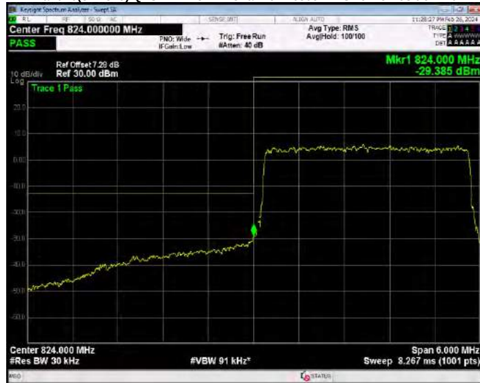
Band26(824-849) QPSK BW=3MHz Channel=27025 RB Size=15 Position=#0
