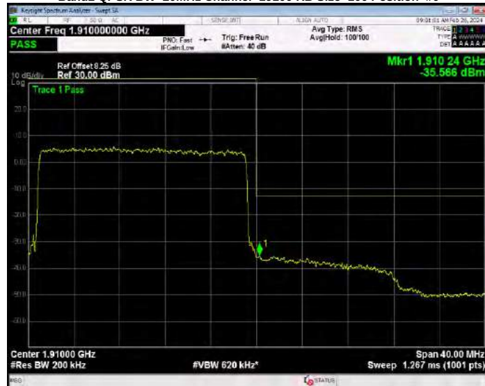
Band2 QPSK BW=3MHz Channel=18615 RB Size=1 Position=#0
