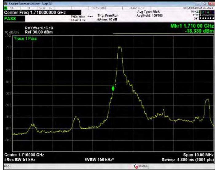
Band4 QPSK BW=5MHz Channel=19975 RB Size=25 Position=#0
