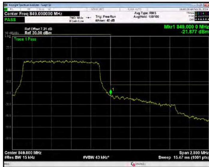
Band5 QPSK BW=10MHz Channel=20450 RB Size=1 Position=#0
