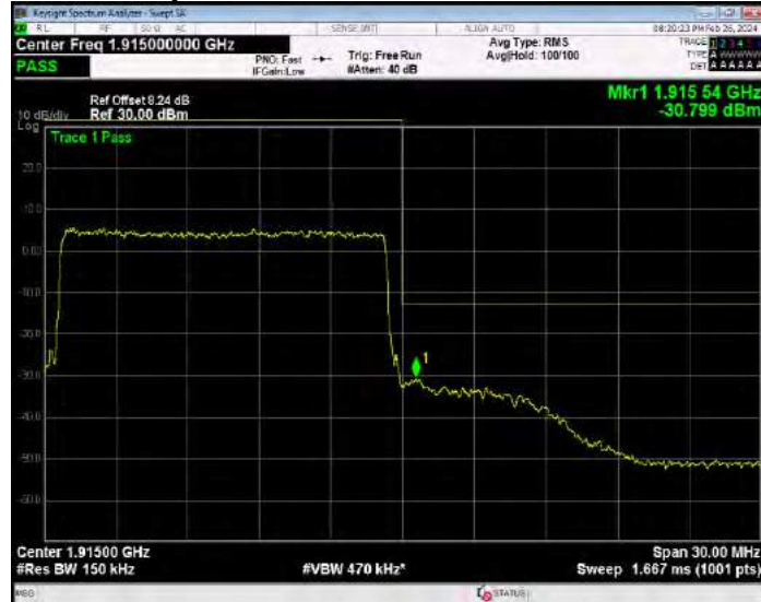
Band25 QPSK BW=20MHz Channel=26140 RB Size=100 Position=#0
