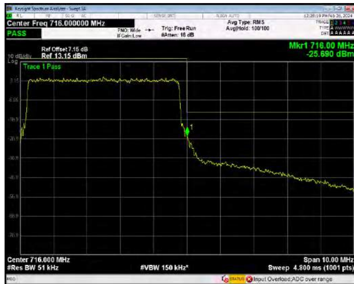
Band17 QPSK BW=10MHz Channel=23780 RB Size=1 Position=#0
