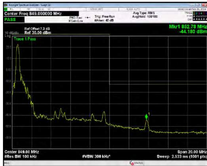
Band5 QPSK BW=10MHz Channel=20600 RB Size=50 Position=#0
