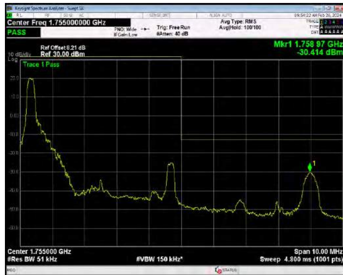
Band4 QPSK BW=5MHz Channel=20375 RB Size=25 Position=#0
