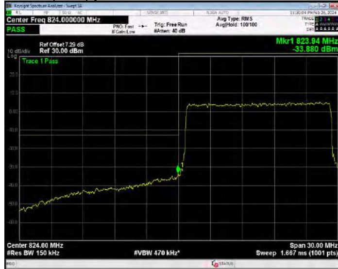
Band26(824-849) QPSK BW=15MHz Channel=26965 RB Size=75 Position=#0
