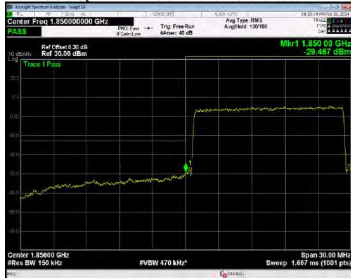
Band25 16QAM BW=15MHz Channel=26115 RB Size=75 Position=#0
