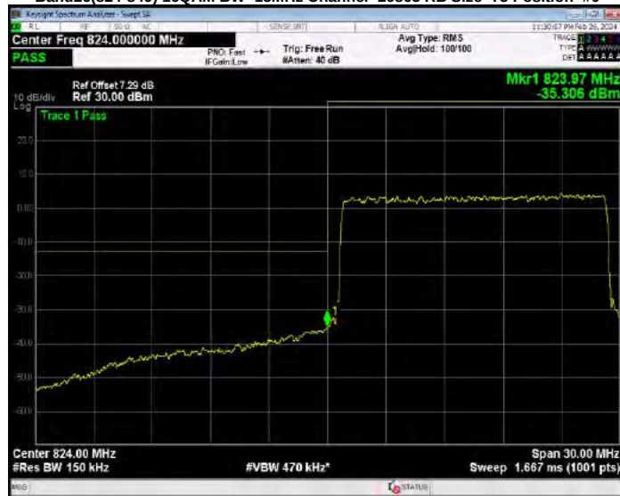
Band26(824-849) 16QAM BW=15MHz Channel=26965 RB Size=75 Position=#0
