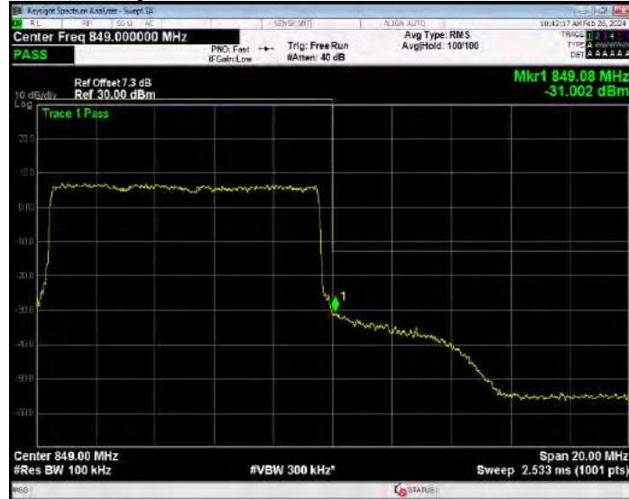
Band5 QPSK BW=3MHz Channel=20415 RB Size=1 Position=#0
