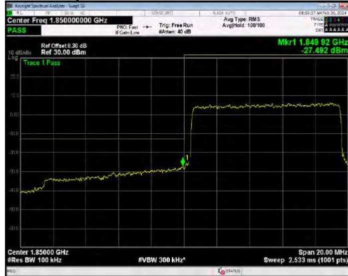
Band2 QPSK BW=10MHz Channel=19150 RB Size=1 Position=#0
