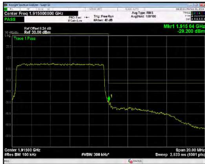
Band25 QPSK BW=15MHz Channel=26115 RB Size=75 Position=#0
