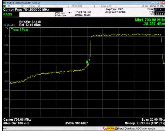
Band17 QPSK BW=10MHz Channel=23800 RB Size=1 Position=#0
