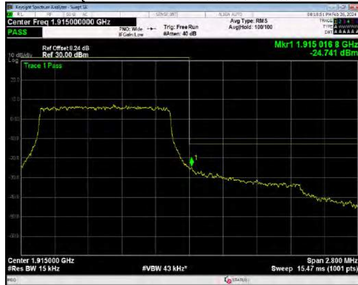
Band25 QPSK BW=10MHz Channel=26090 RB Size=50 Position=#0
