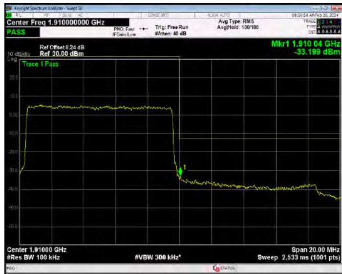
Band2 QPSK BW=15MHz Channel=18675 RB Size=1 Position=#0
