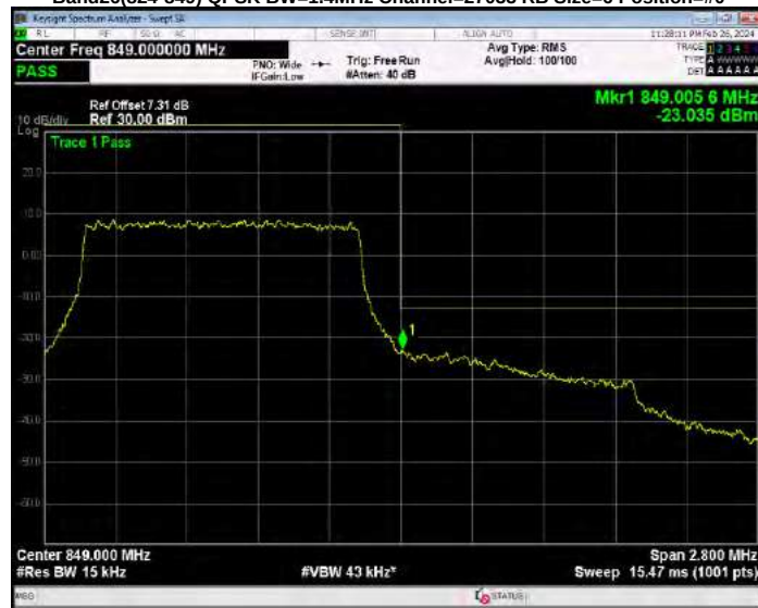
Band26(824-849) QPSK BW=10MHz Channel=26840 RB Size=50 Position=#0
