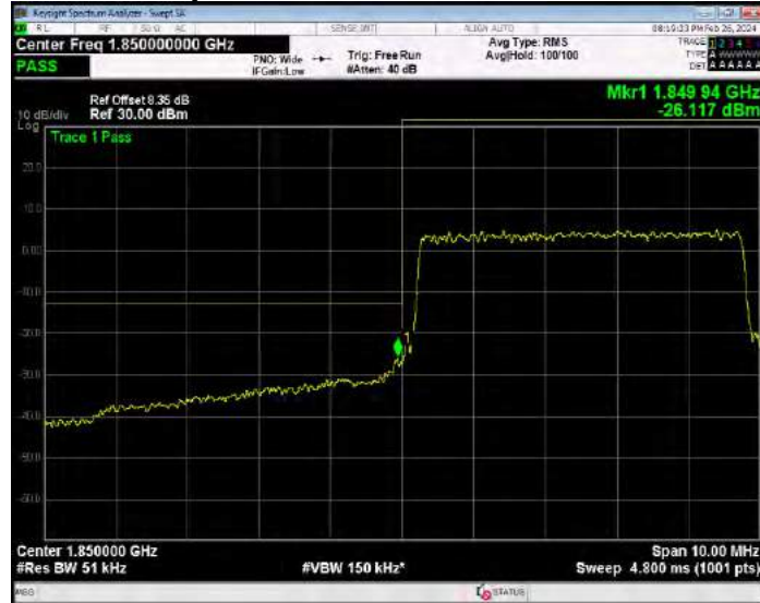
Band25 16QAM BW=5MHz Channel=26665 RB Size=25 Position=#0
