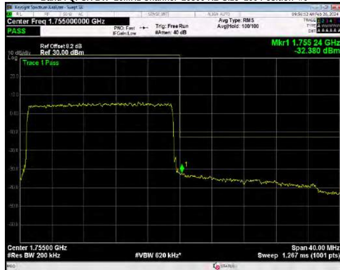
Band4 QPSK BW=3MHz Channel=19965 RB Size=1 Position=#0
