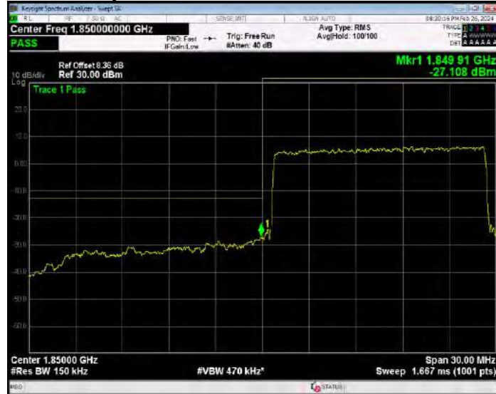
Band25 QPSK BW=15MHz Channel=26615 RB Size=75 Position=#0
