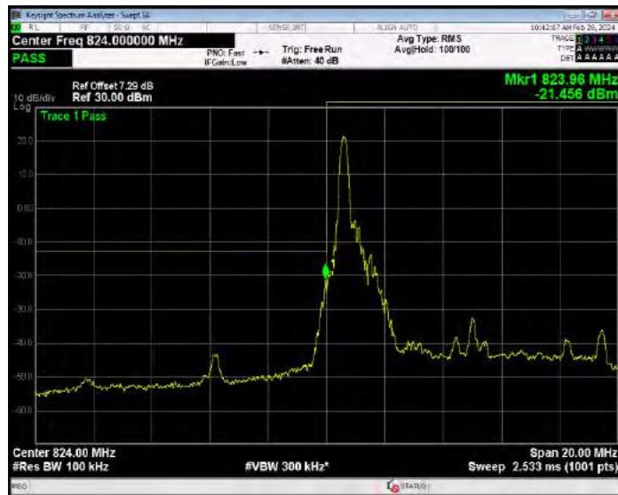
Band5 16QAM BW=10MHz Channel=20450 RB Size=50 Position=#0
