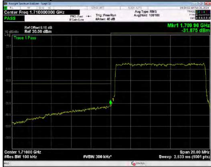
Band4 16QAM BW=10MHz Channel=20350 RB Size=1 Position=#0
