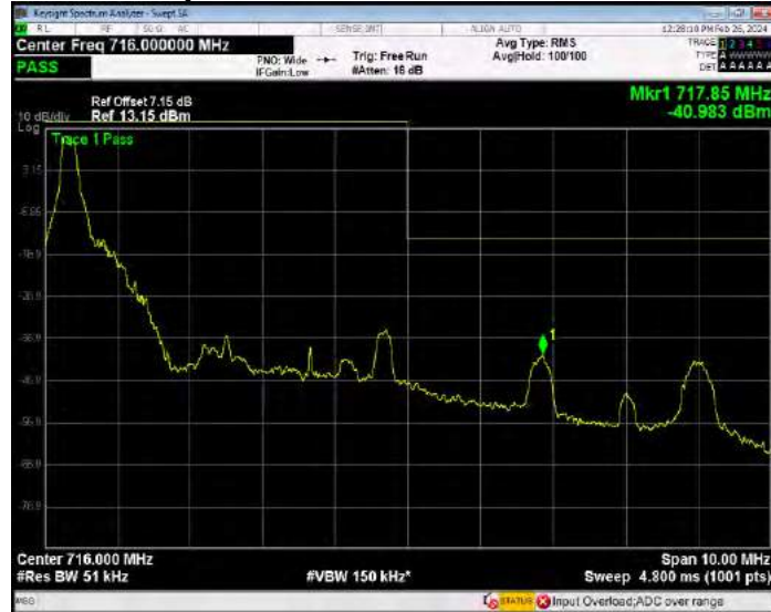
Band17 QPSK BW=5MHz Channel=23825 RB Size=25 Position=#0
