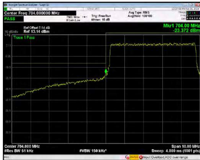
Band17 QPSK BW=5MHz Channel=23825 RB Size=1 Position=#0
