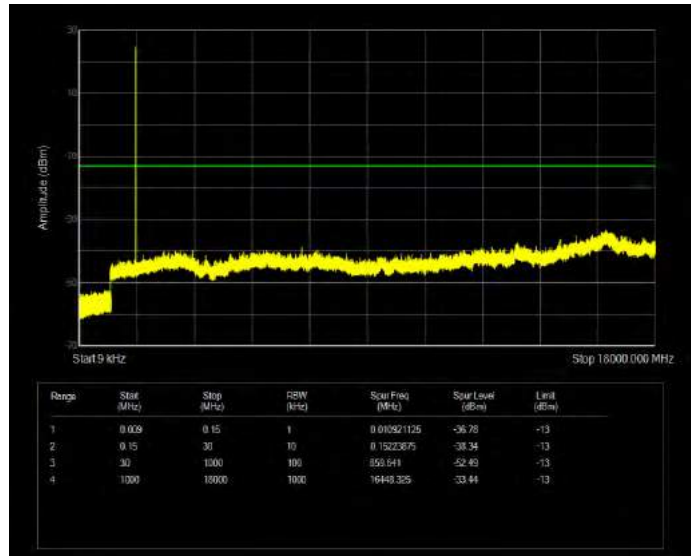
Band66 16QAM BW=10MHz Channel=132022 RB Size=50 Position=#0
