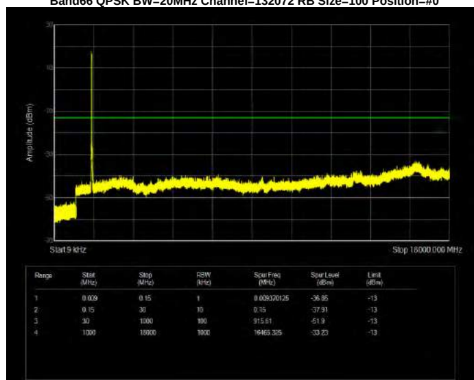
Band66 QPSK BW=20MHz Channel=132322 RB Size=100 Position=#0
