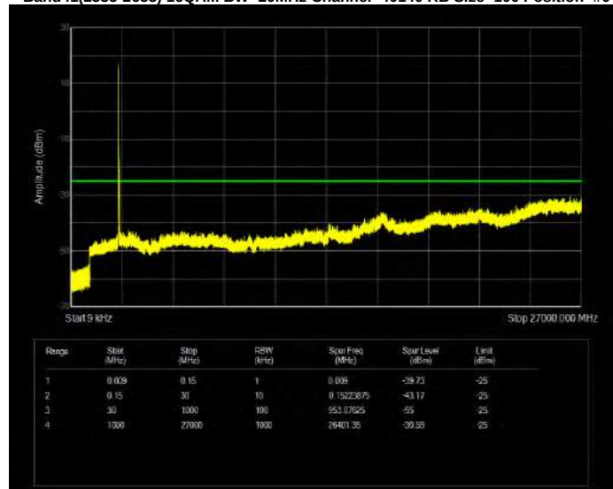
Band41(2535-2655) 16QAM BW=20MHz Channel=41140 RB Size=100 Position=#0
