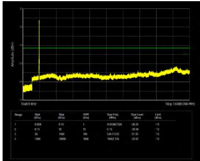
Band66 QPSK BW=3MHz Channel=131987 RB Size=15 Position=#0
