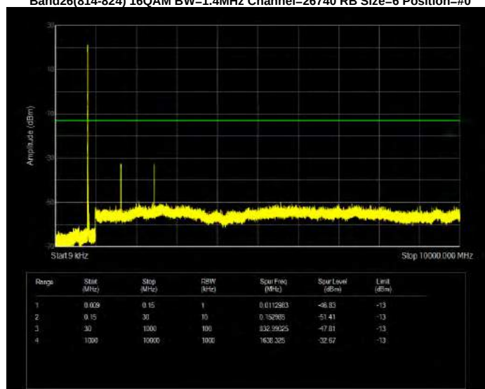
Band26(814-824) 16QAM BW=1.4MHz Channel=26783 RB Size=6 Position=#0
