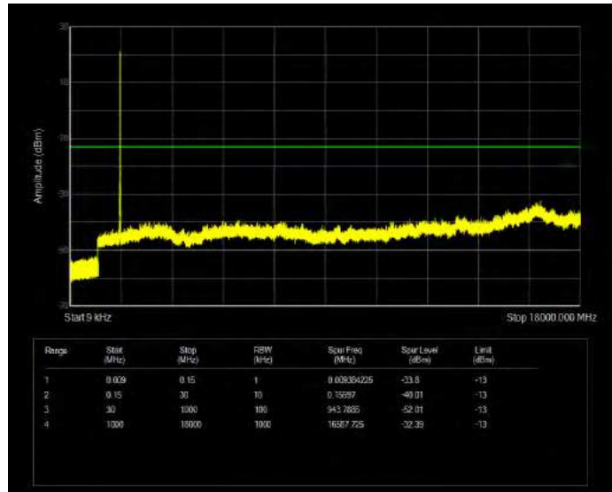
Band66 QPSK BW=1.4MHz Channel=131979 RB Size=6 Position=#0
