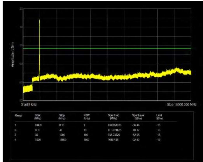
Band66 16QAM BW=20MHz Channel=132072 RB Size=100 Position=#0
