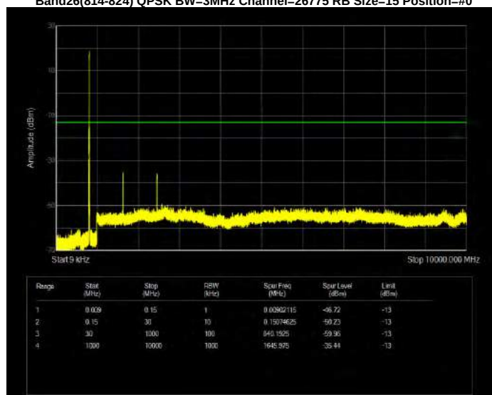
Band26(814-824) QPSK BW=5MHz Channel=26715 RB Size=25 Position=#0
