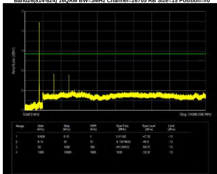
Band26(814-824) 16QAM BW=3MHz Channel=26740 RB Size=15 Position=#0
