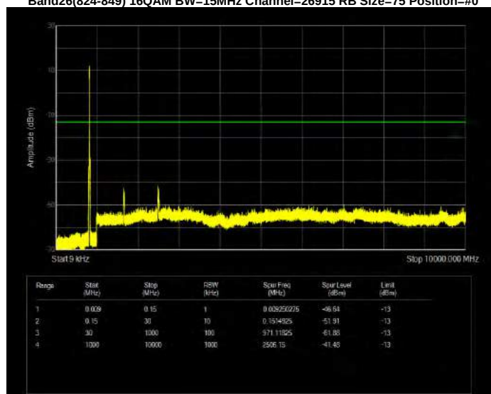
Band26(824-849) 16QAM BW=15MHz Channel=26965 RB Size=75 Position=#0
