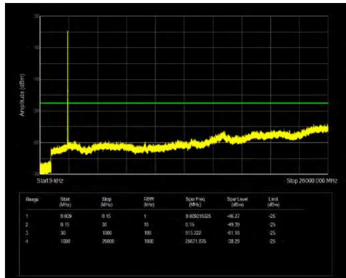
Band7 QPSK BW=5MHz Channel=21100 RB Size=25 Position=#0
