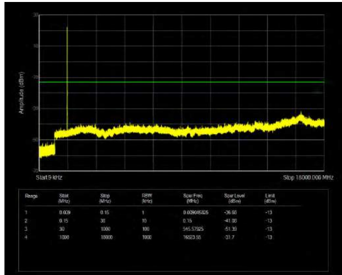
Band66 16QAM BW=5MHz Channel=131997 RB Size=25 Position=#0
