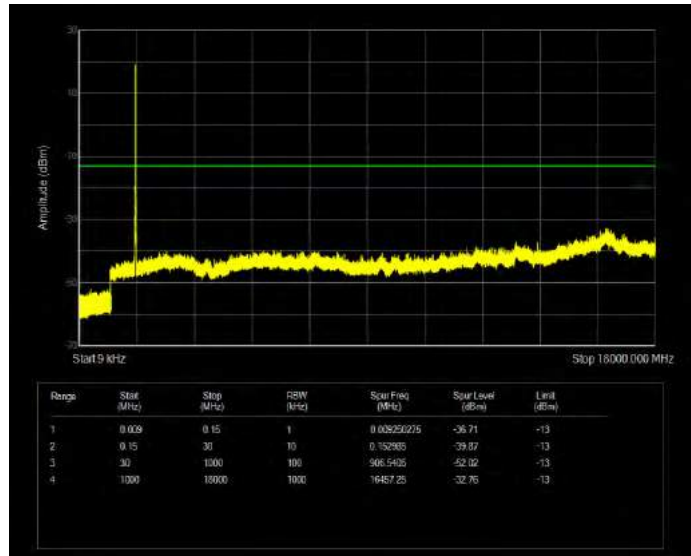
Band66 16QAM BW=15MHz Channel=132047 RB Size=75 Position=#0
